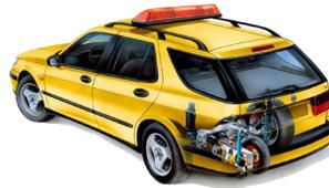
**Figure 18. SAAB Friction Tester**
