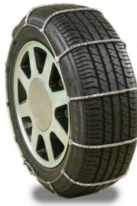
**Figure 1. Typical Cable Chain**
