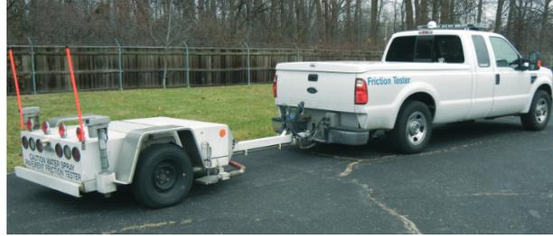
**Figure 19. Dynatest 1295 Pavement Friction Tester (PFT)**
