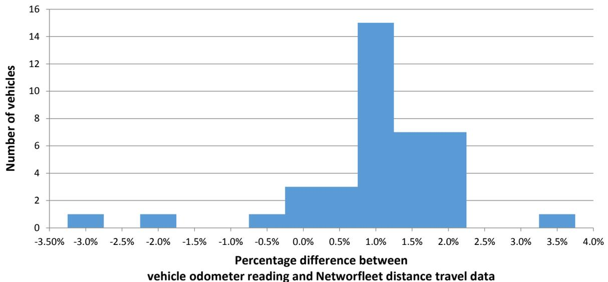
**Figure 4.10 – Pilot study fleet odometer error distribution**
