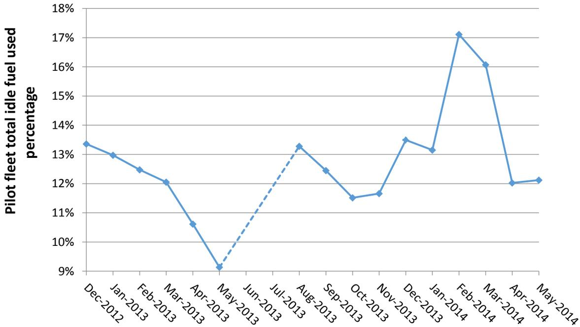
Figure 4.21 – Percentage of idle fuel usage over total fuel usage per month
