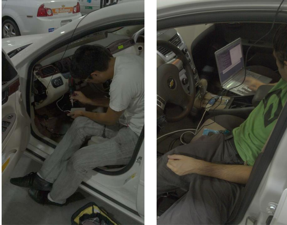
Figure 5.3. Telematic units were installed (left) and programmed for specific vehicle requirements (right).
