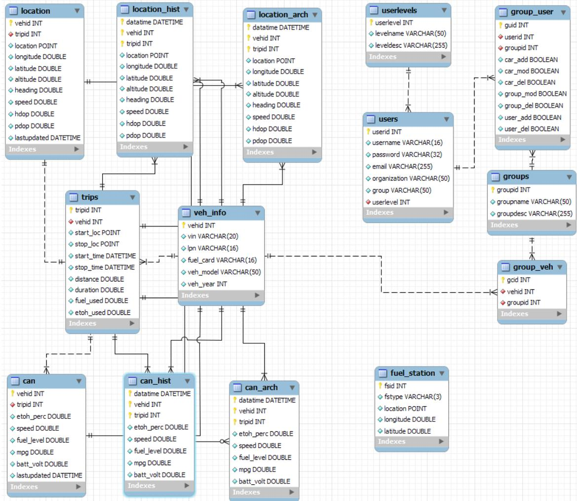
Figure 4.1. Database structure for the E85 alt fuel server.
