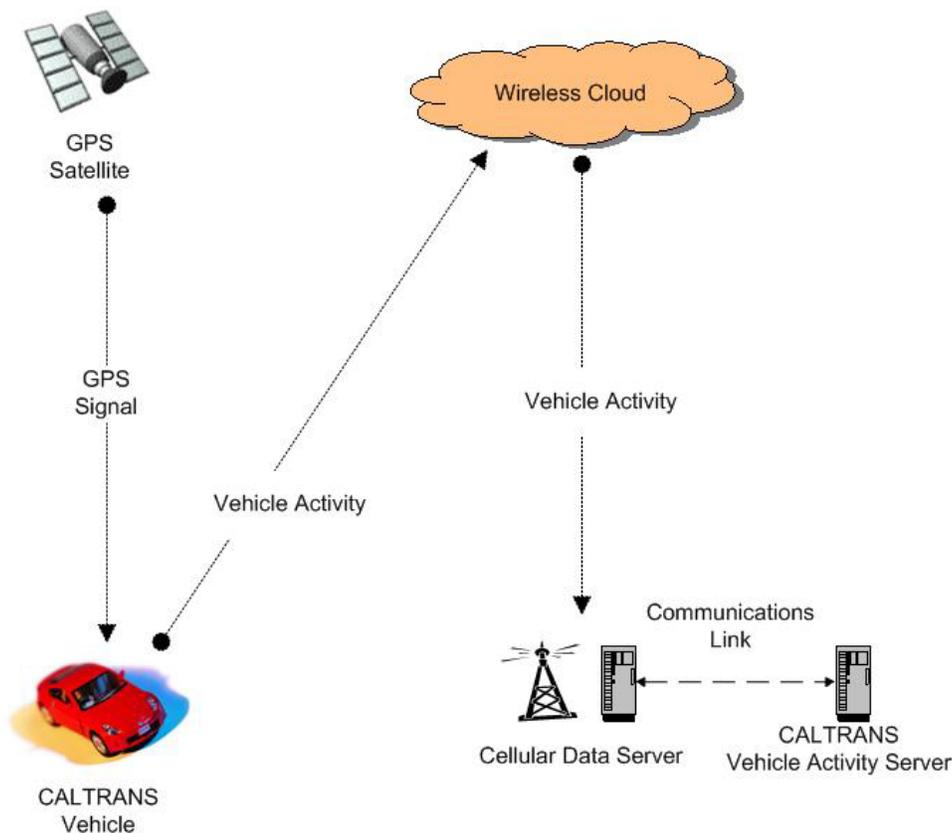
Figure 1. Caltrans E85 fuel monitoring system architecture.
