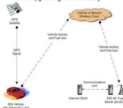
Figure 1 Caltrans E85 Monitoring System Architecture.
