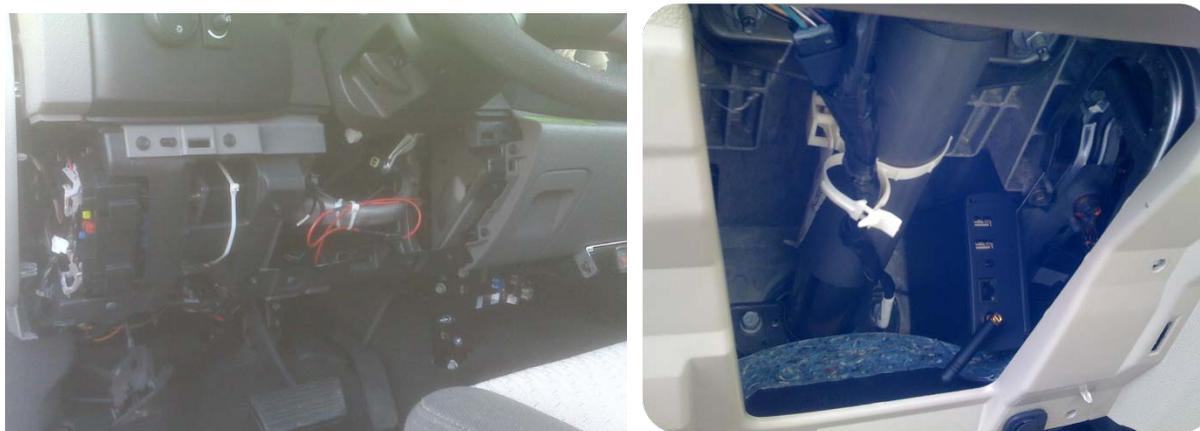
Figure 2.5. Telematic units were installed within the dashboard on Silverado (left) and Impala (right).
