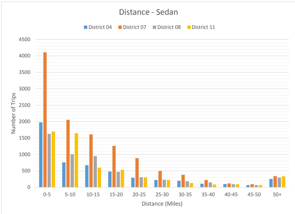
Figure 6.15. Trip distance histogram for sedans operating in the deployment program.
