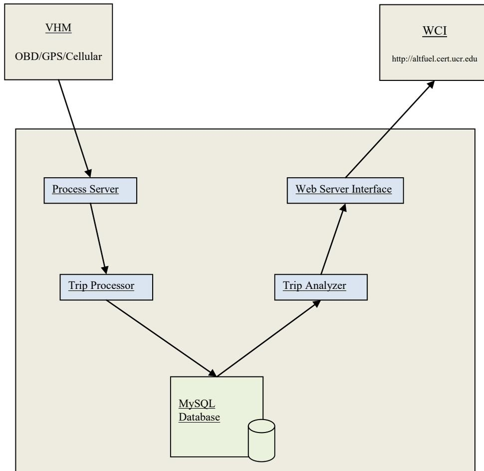
Figure 7.2. Server data flow diagram for telematics and web client programs.
