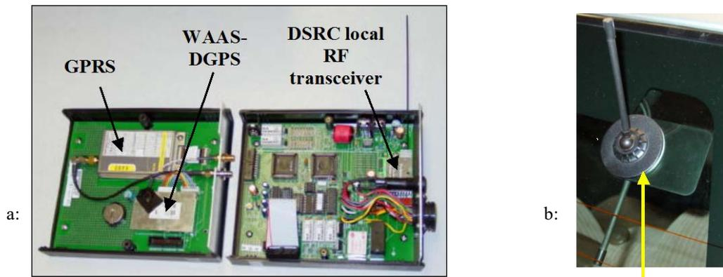
Figure 2.2. a) On-Board Telematics Hardware: GPRS - General Packet Radio Service cellular modem; WAAS-DGPS – Wide Area Augmentation System enabled Differential Global Position System receiver; DSRC – Dedicated Short Range Communications. b) Dual GPRS/GPS antenna.
