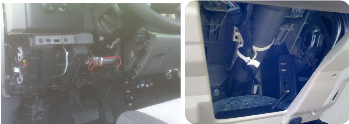
Figure 2.5. Telematic units were installed within the dashboard on Silverado (left) and Impala (right).
