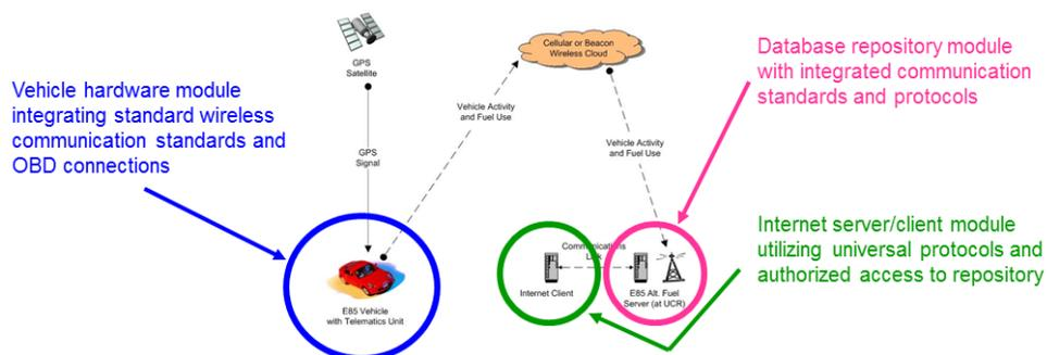
**Figure ES.1.** E85 alt-fuel system monitoring architecture with combined cellular and Wi-Fi.
