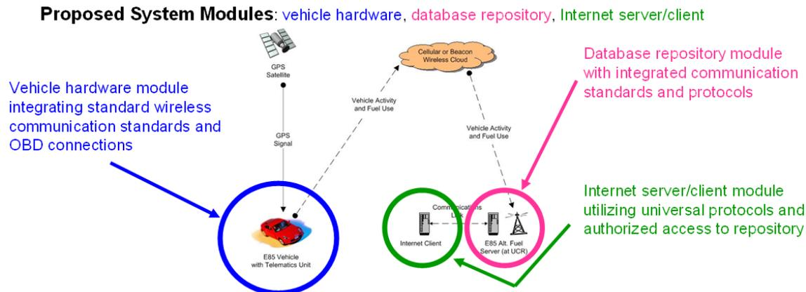
Figure 2. Proposed architecture for future deployment.
