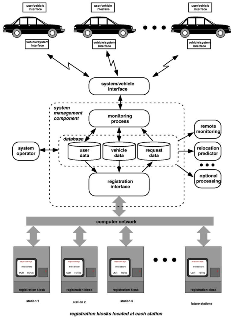
Figure 2.1. UCR IntelliShare carsharing system architecture.
