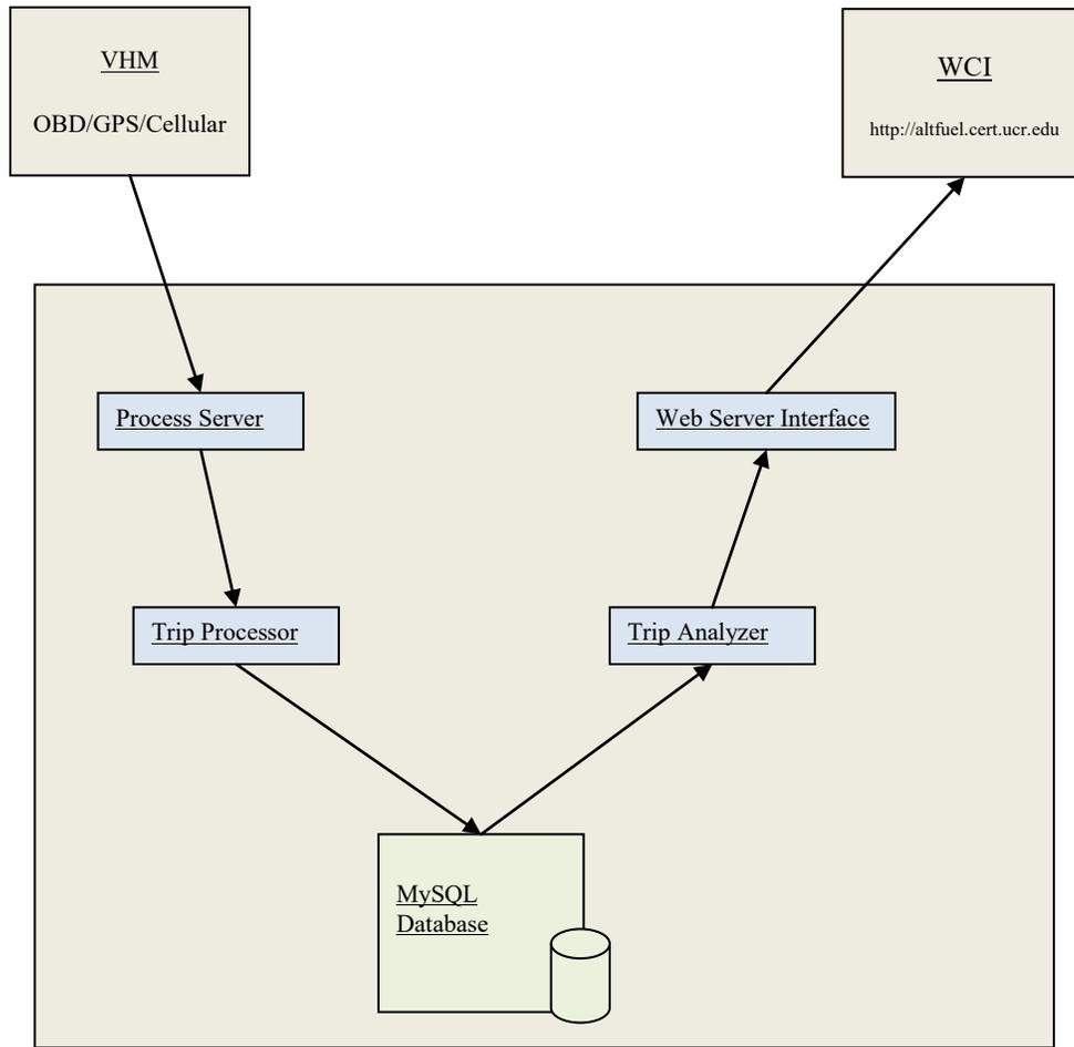
**Figure 3.** Server data flow diagram for telematics and web client programs.
