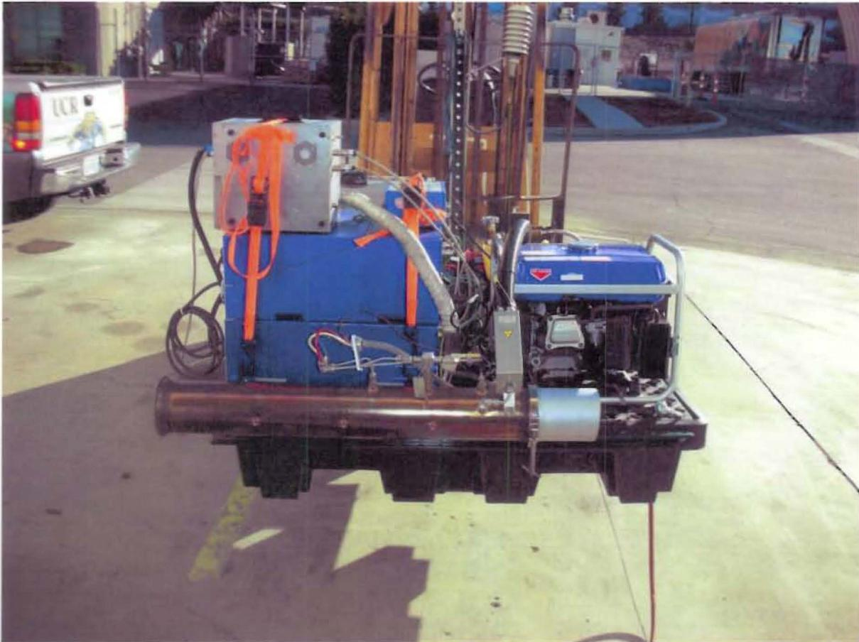
**Figure 2-5: Emission Analyzers, Generator, and Flow Meter on a 4' by 4' Plastic Pallet**
