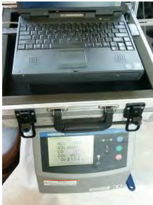
Figure 1 - In-Field Illustration of Continuous Gas Analyzer and Computer for Data Logging
