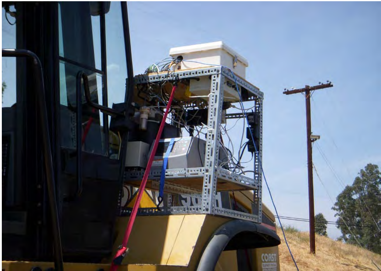
Figure 3 - Installation of the Real-Time Emissions Measurement System on the Front-End Loader
