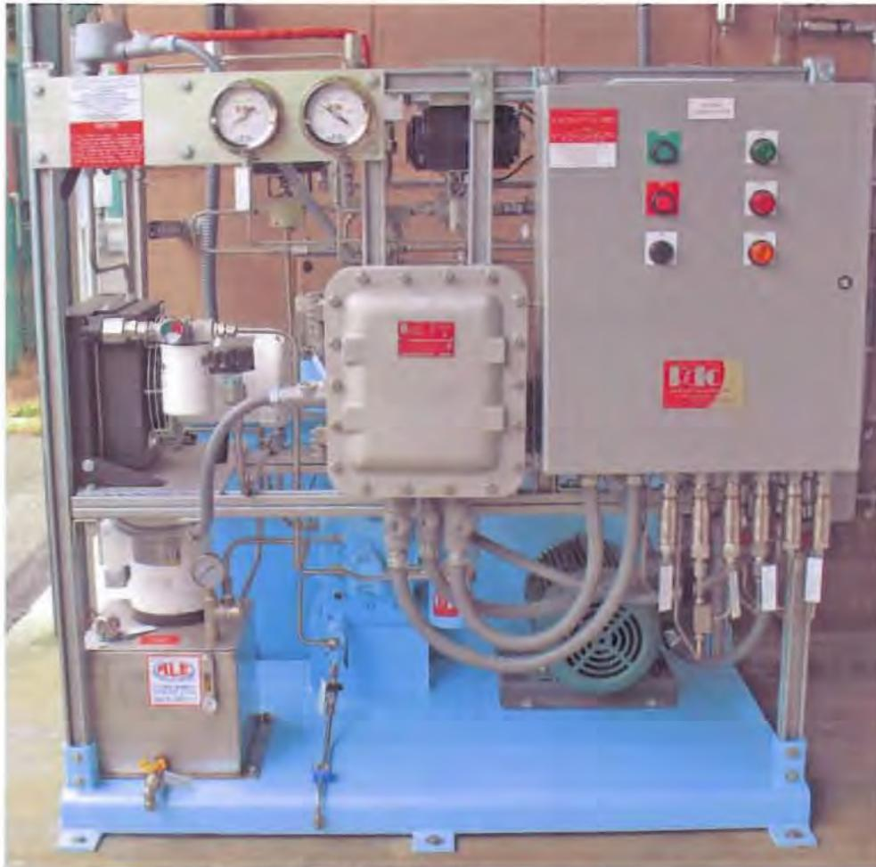
**Figure 3: 700 bar hydrogen compressor**
