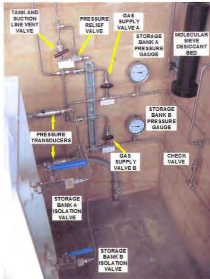
**Figure 2. Gas supply plumbing**
