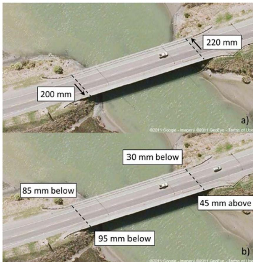
**Figure 2.9 South Brighton bridge; a) horizontal movement of abutments compared to bridge deck; b) vertical position of abutment compared to bridge deck (NZ-GEER 2011)**
