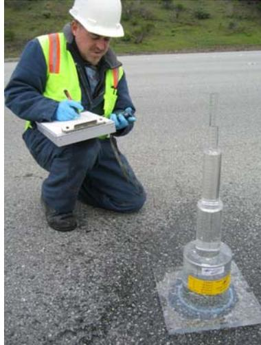
**Figure 1: Falling-head permeameter.**
