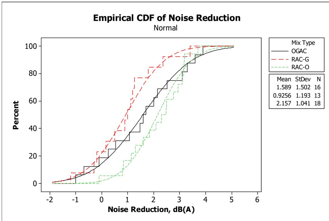
**Figure 7: Cumulative distribution function of noise reduction of OGAC, RAC-O, and RAC-G mixes compared to DGAC (104 dB(A) average across all ages) across an eight-year range of ages (positive value indicates a reduction in noise).**
