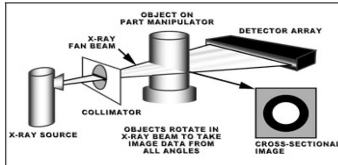
Figure 6: Computed tomography (CT) scanner (5).
