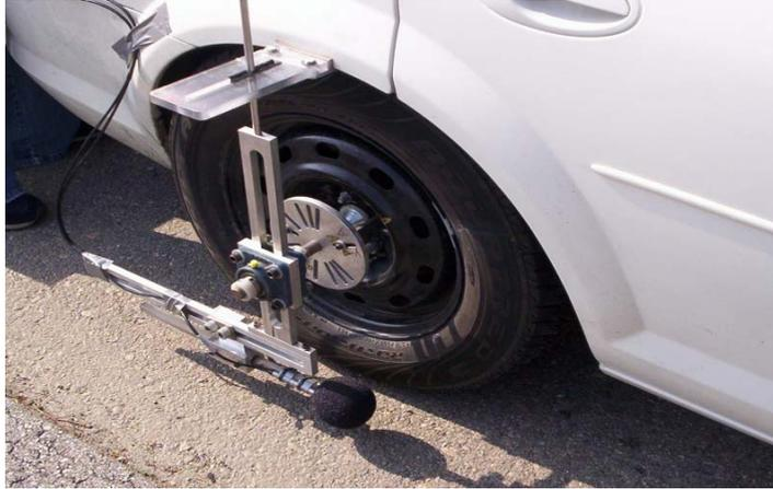
**Figure 3: On-board sound intensity (OBSI) microphone setup.**
