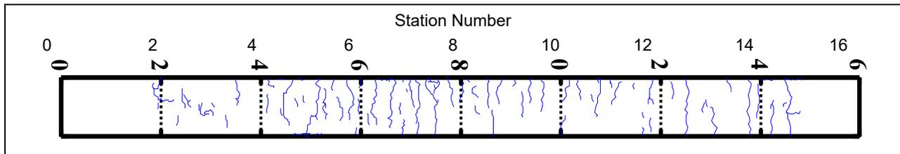
**Figure 4.42: 606FD: Final crack pattern.**
