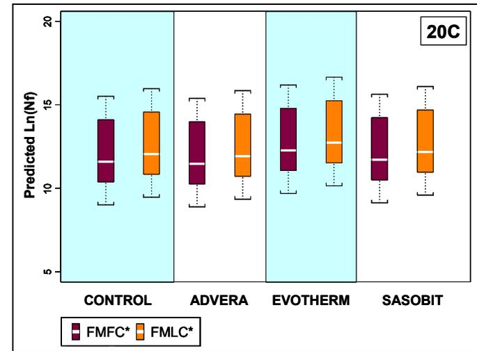
Figure 6.28: Comparison of predicted fatigue life at same air-void content.
