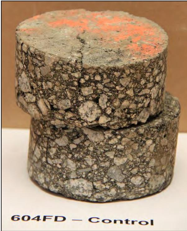
Figure 5.6: 604FD: Core from Trafficked Area.
