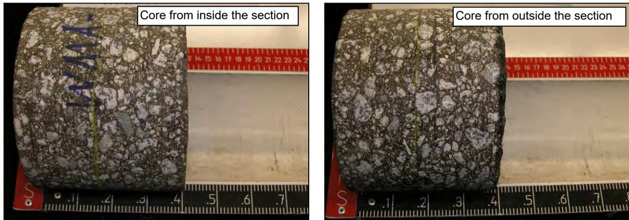
**Figure 4.27: 605FD: Cores for moisture content determination.**
