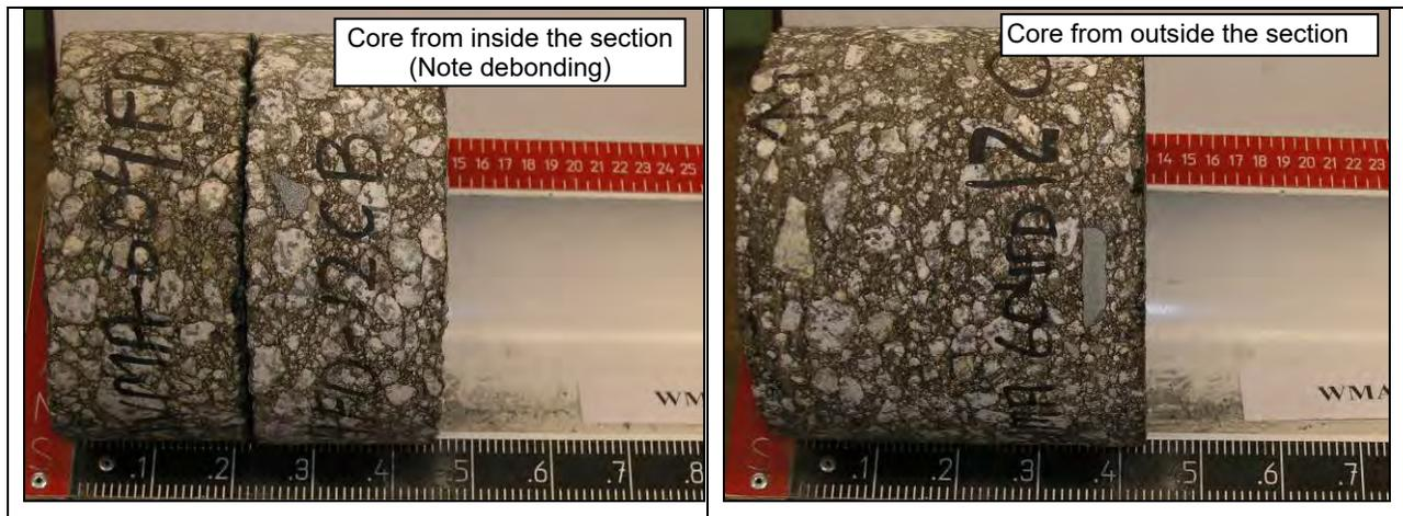
**Figure 4.13: 604FD: Cores for moisture content determination.**
