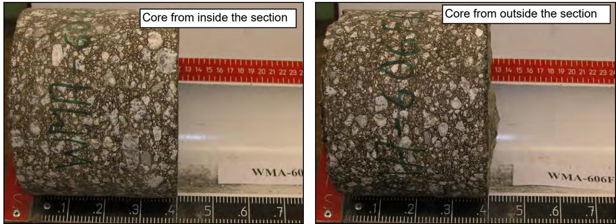
**Figure 4.41: 606FD: Cores for moisture content determination.**
