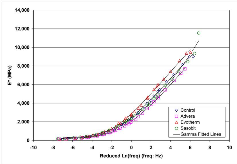
Figure 6.14: Complex modulus ( $E^*$ ) master curves (wet).
