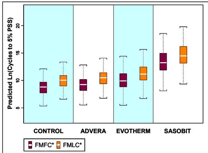
Figure 6.27: Comparison of predicted cycles to 5% permanent shear strain at same air-void content.
