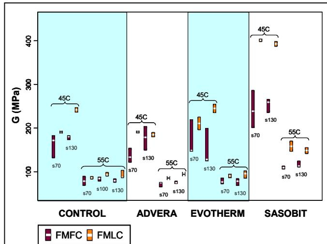
Figure 6.19: Resilient shear modulus comparison between FMFC and FMLC shear tests.
