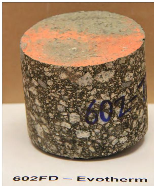
Figure 5.4: 602FD: Core from Trafficked Area.
