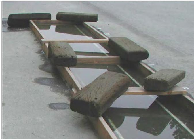
**Figure 3.5: Soaking dam with water.**
