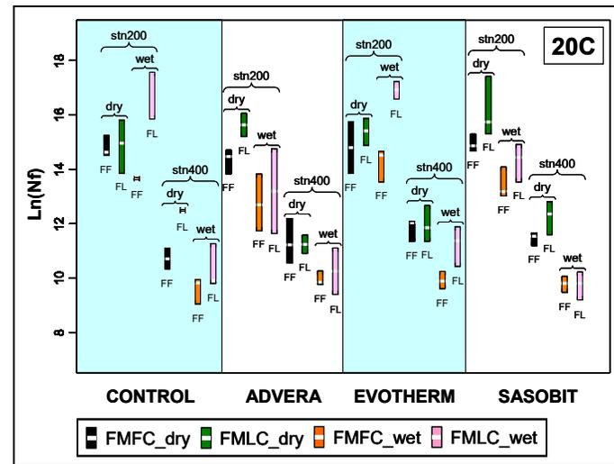
Figure 6.24: Fatigue life comparison between FMFC and FMLC fatigue tests.
