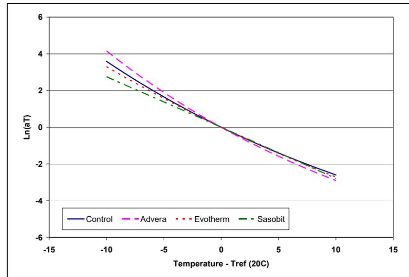
Figure 6.15: Temperature-shifting relationship (wet).
