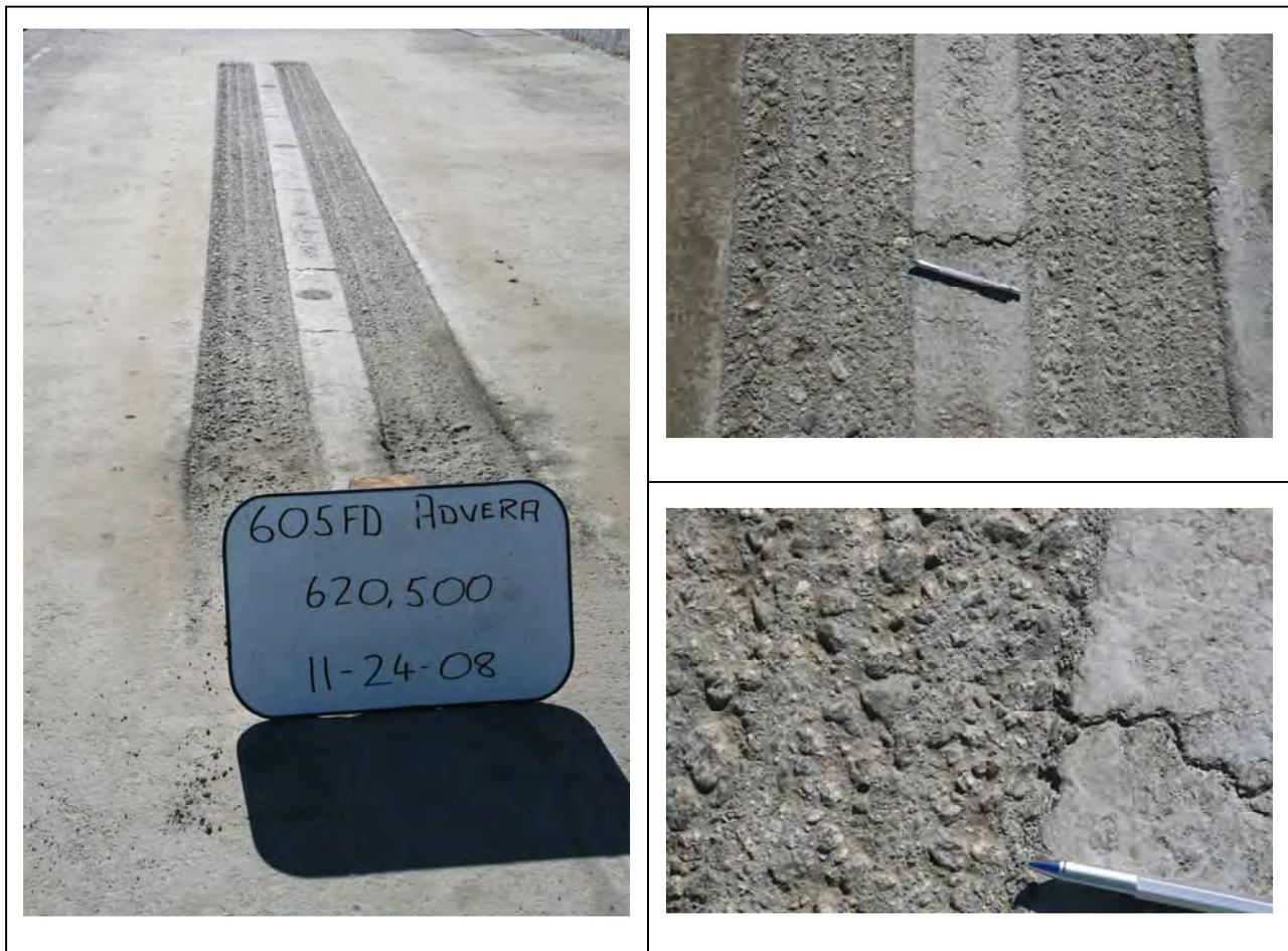
**Figure 4.32: 605FD: Section photographs at test completion.**
