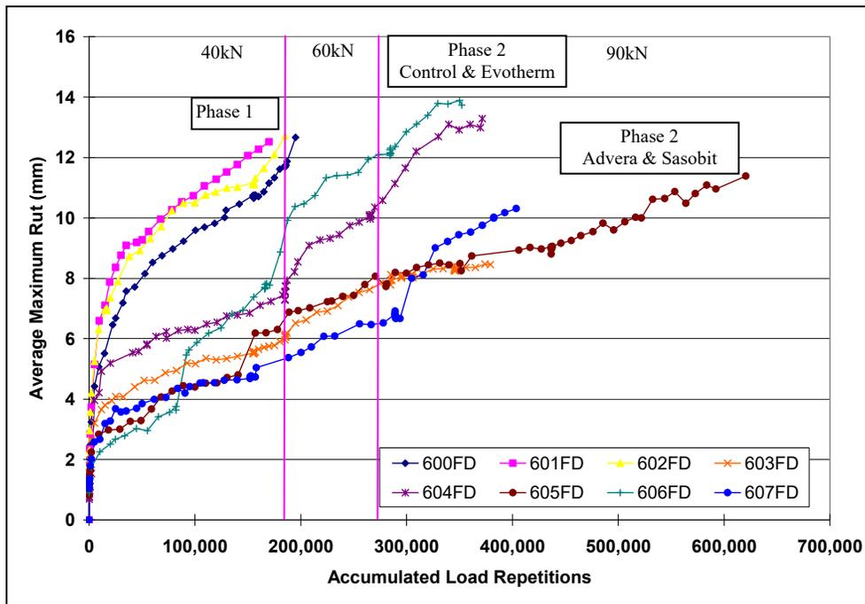
Figure 4.58: Comparison of Phase 1 and Phase 2 rutting performance.
