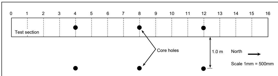
**Figure 4.12: Location of cores for moisture content determination.**
