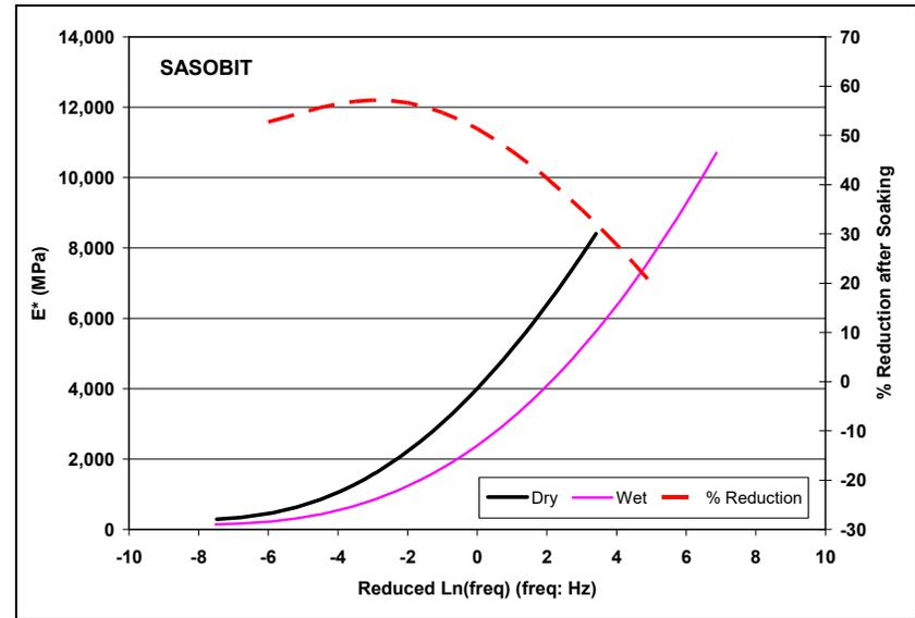
**Figure 6.16: Comparison of dry and wet complex modulus master curves.**
