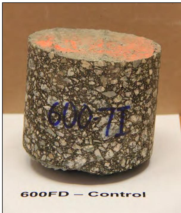
Figure 5.2: 600FD: Core from Trafficked Area.
