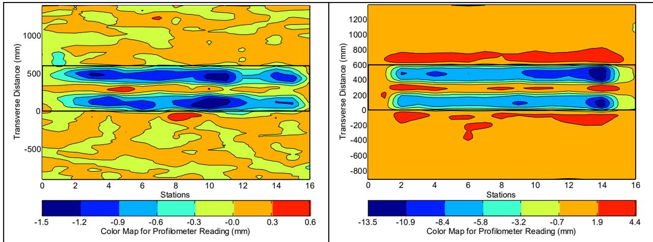
**Figure 4.26: 605FD: Contour plot of permanent surface deformation at start and end of test.**
