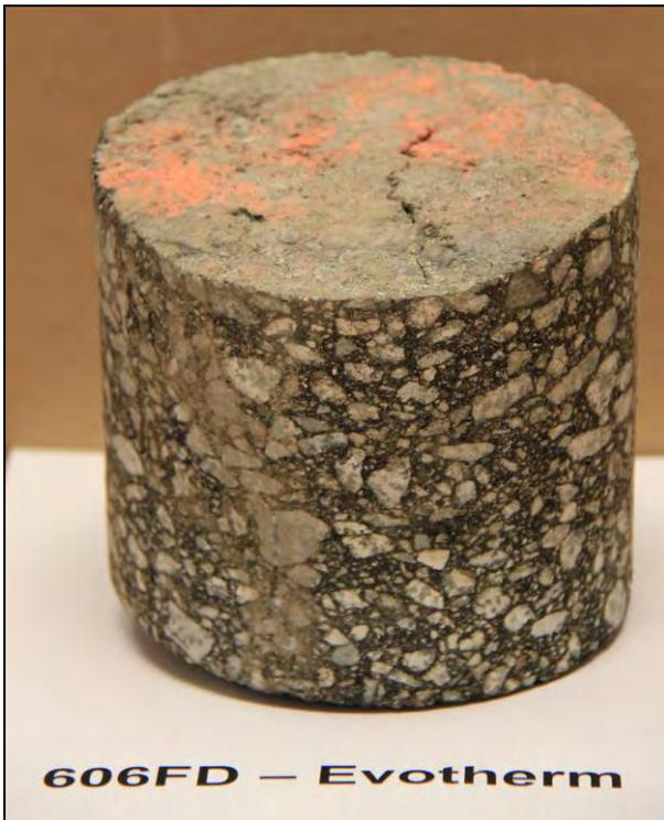
Figure 5.8: 606FD: Core from Trafficked Area.
