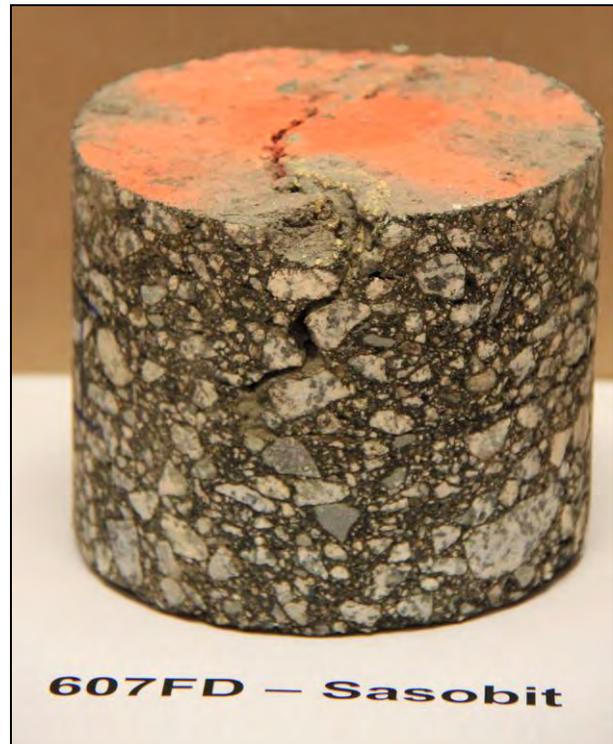
Figure 5.9: 607FD: Core from Trafficked Area.
