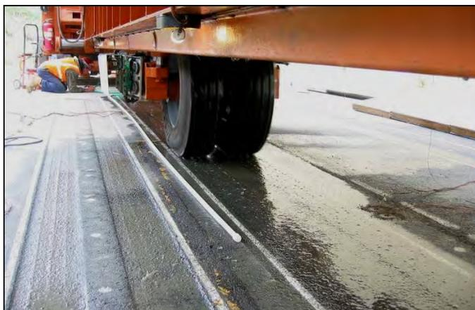
**Figure 3.6: Water flow across test section during trafficking.**
