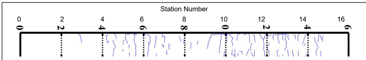
**Figure 4.30: 605FD: Final crack pattern.**
