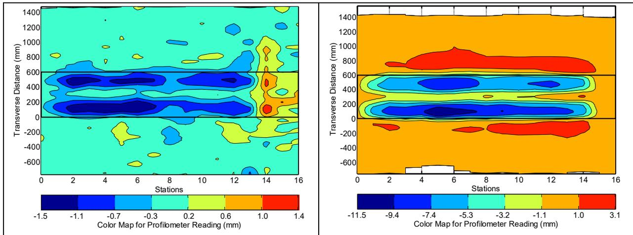
**Figure 4.51: 607FD: Contour plot of permanent surface deformation at start and end of test.**
