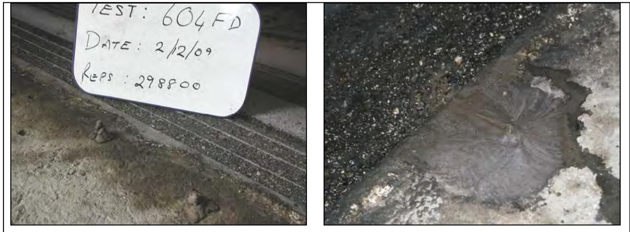
**Figure 4.17: 604FD: Fines pumped from holes drilled for presoaking.**
