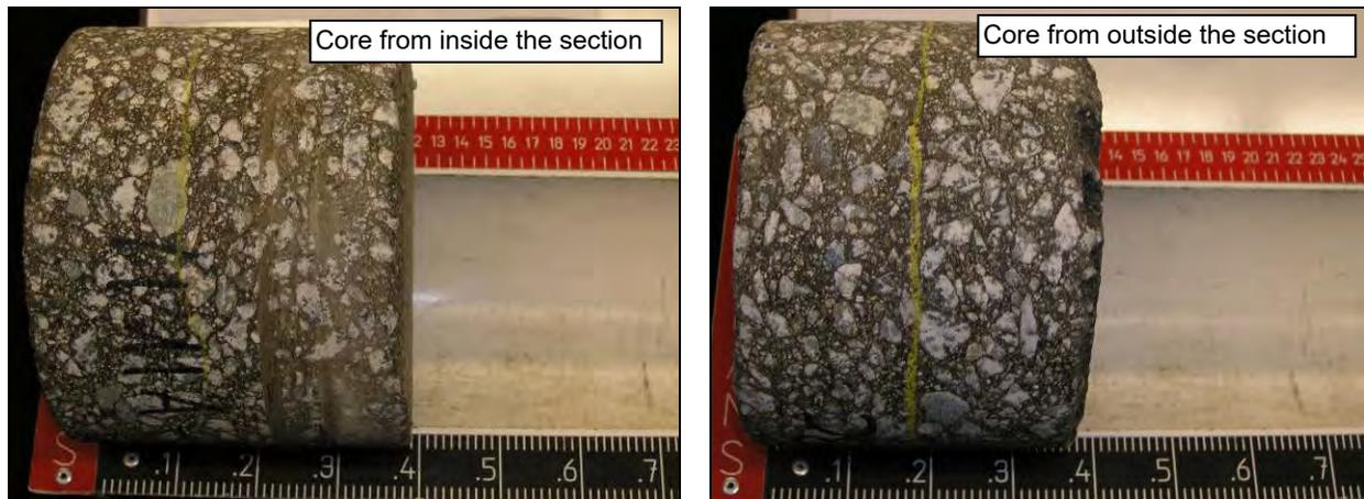
**Figure 4.52: 607FD: Cores for moisture content determination.**
