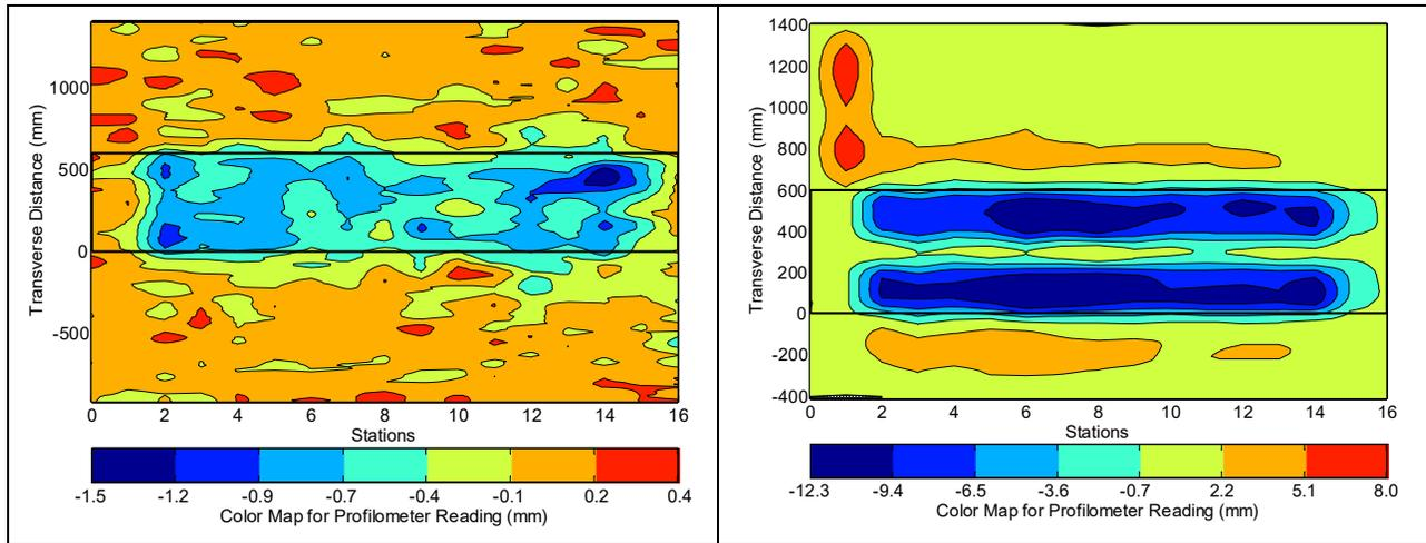
**Figure 4.11: 604FD: Contour plot of permanent surface deformation at start and end of test.**
