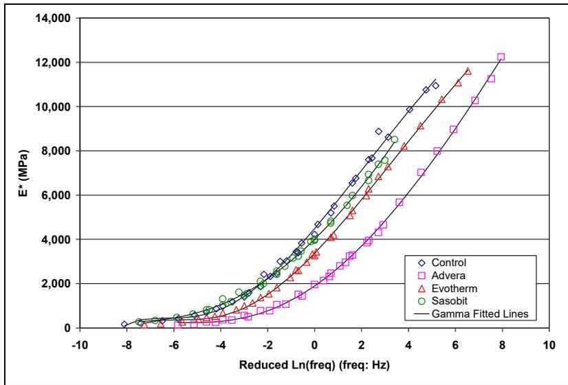
Figure 6.12: Flexural complex modulus ( $E^*$ ) master curves (dry).
