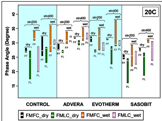
Figure 6.23: Phase angle comparison between FMFC and FMLC fatigue tests.
