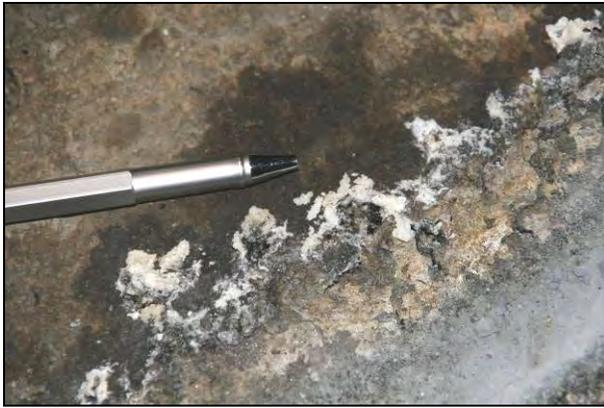
**Figure 4.14: 604FD: Crystallized salt on edges of wheelpaths during testing.**
