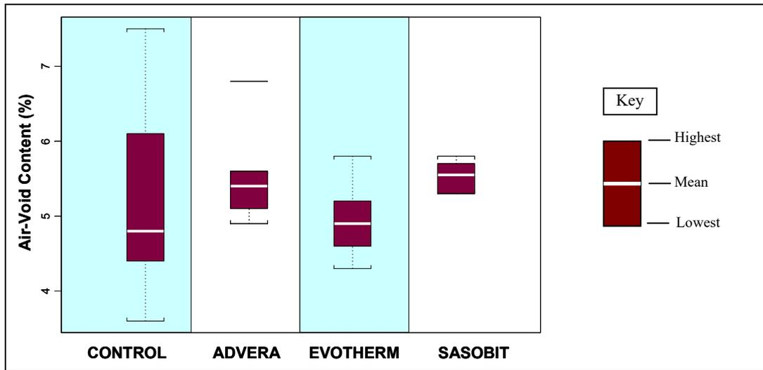
**Figure 6.1: Air-void contents of FMLC shear specimens.**
