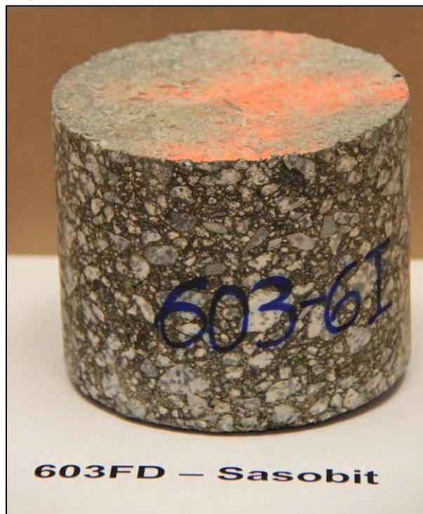
Figure 5.5: 603FD: Core from Trafficked Area.
