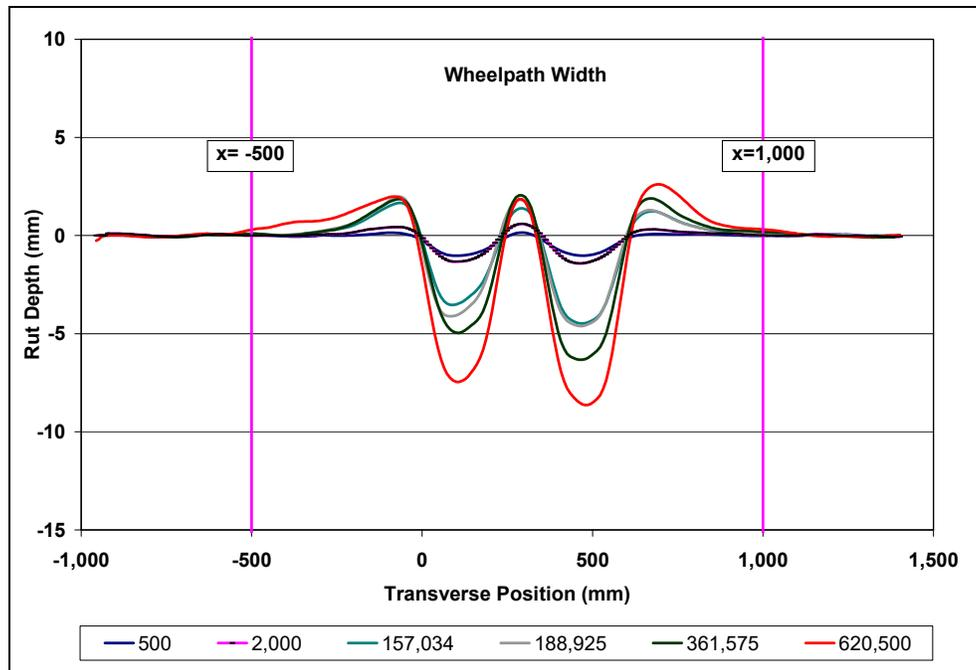
**Figure 4.23: 605FD: Profilometer cross section at various load repetitions.**
