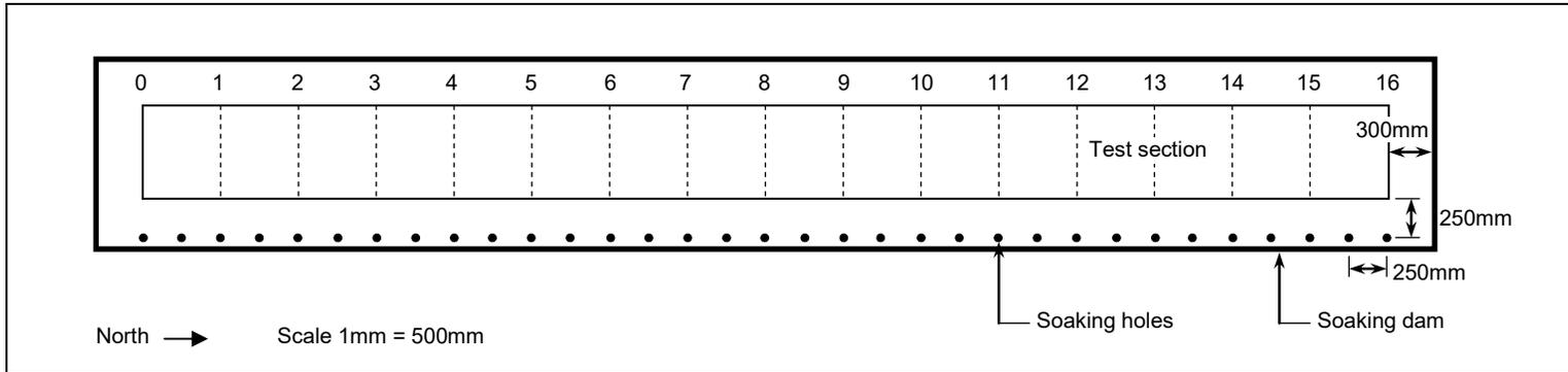
**Figure 3.3: Location of presoaking dam and soak holes.**
