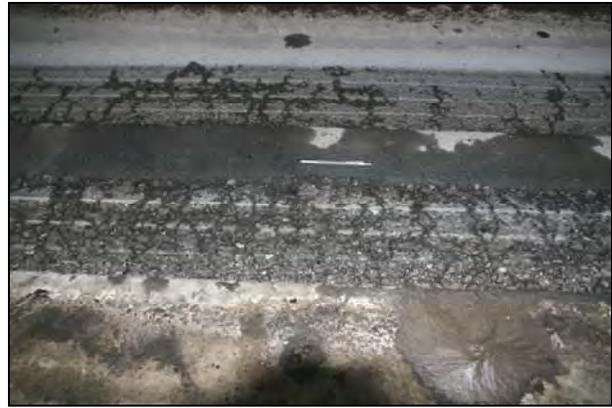
**Figure 4.15: 604FD: Cracks in wheelpaths during testing.**
