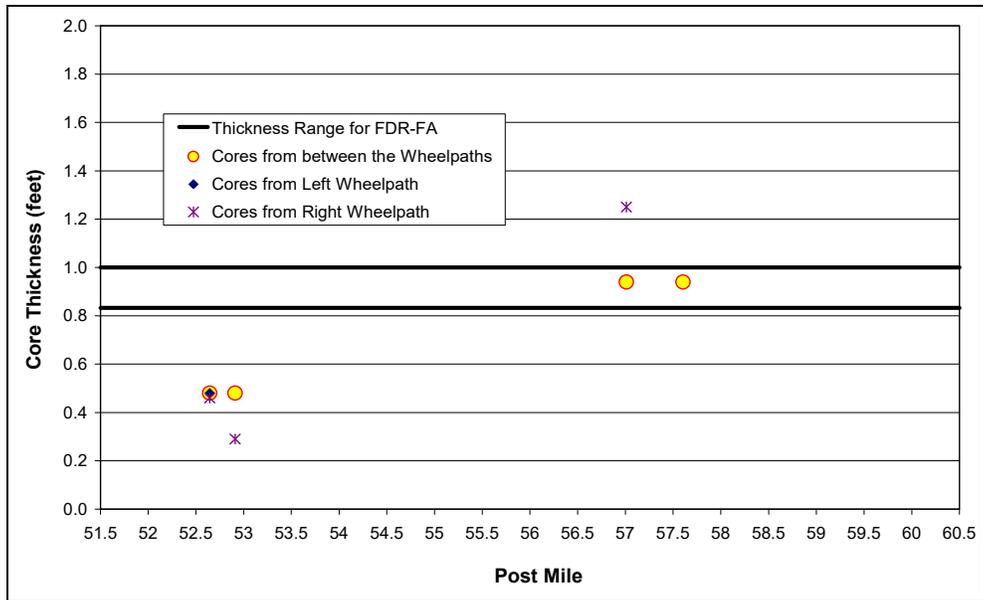
Figure C.2: HMA thickness summary from cores for westbound lane.
