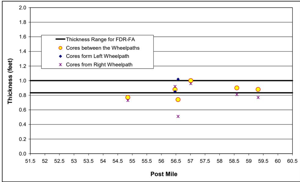
Figure C.1: HMA thickness summary from cores for eastbound lane.
