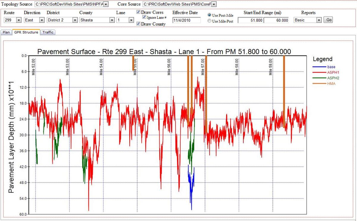
**Figure C.5: Screenshot from PMS GPR/Core viewing tool.**
