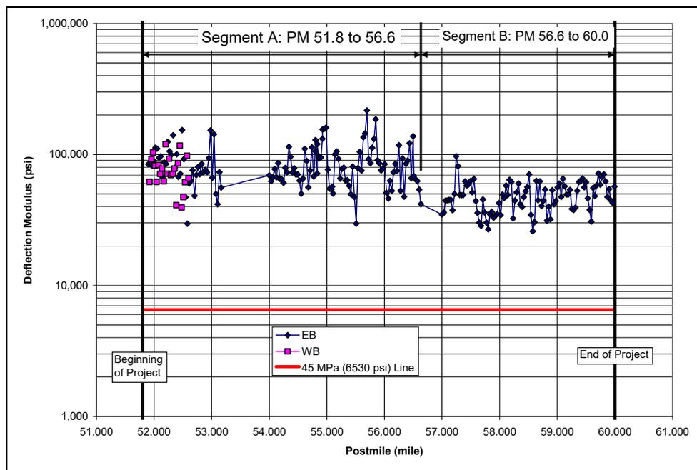
Figure D.1: Subgrade Deflection Modulus.
