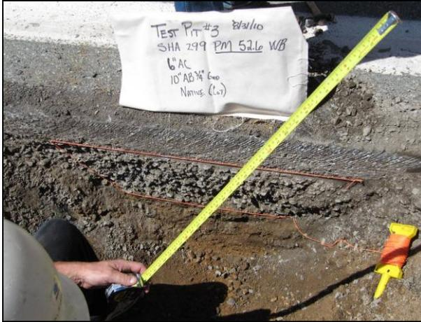
**Figure 2.3: Test Pit 3 cross section at PM 52.51 westbound.**
