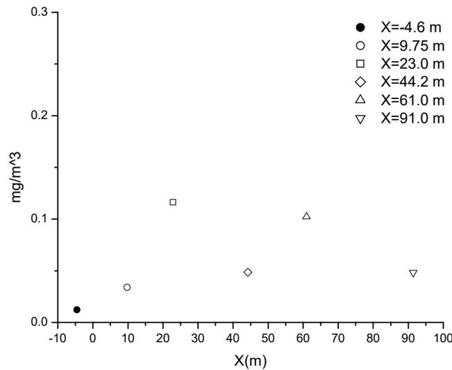
Figure 10. Axial variation of averaged background aerosol concentration.
