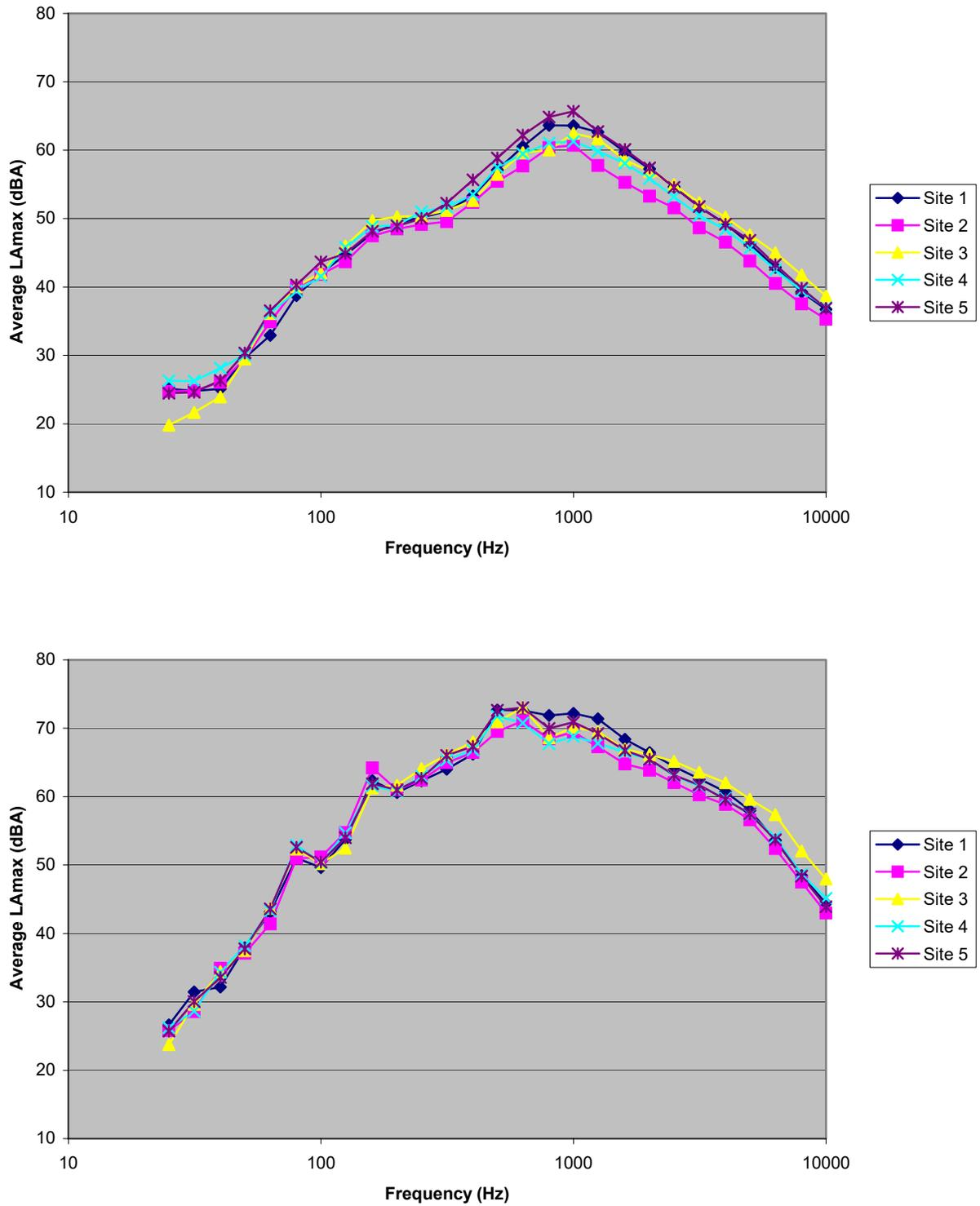
**Figure E-6. Spectral data for automobiles (top) and heavy trucks (bottom) on four different pavement types. Post-overlay results, all pavements aged 4 months. Microphone location: distance 50 ft, height 15 ft.**
