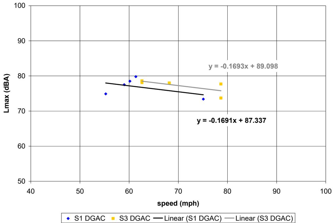
**Figure C-5. (this and previous page) Vehicle pass-by data, pre-overlay; Site 1 (DGAC), Site 3 (DGAC). Automobiles (top), medium trucks (middle), and heavy trucks (bottom). Microphone location: distance 50 ft, height 5 ft.**
