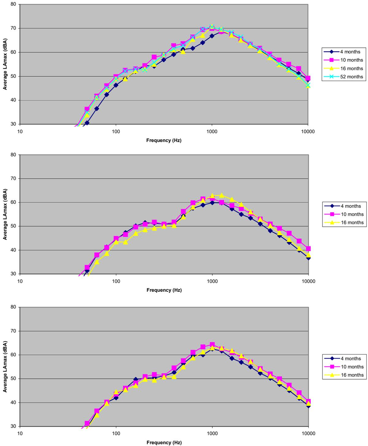
**Figure E-21. Spectral data for automobiles; post-overlay results for Site 3 (OGAC 30 mm); all ages measured. Microphone location: distance 25 ft, height 5 ft (top); microphone location: distance 50 ft, height 5 ft (middle); microphone location: distance 50 ft, height 15 ft (bottom).**
