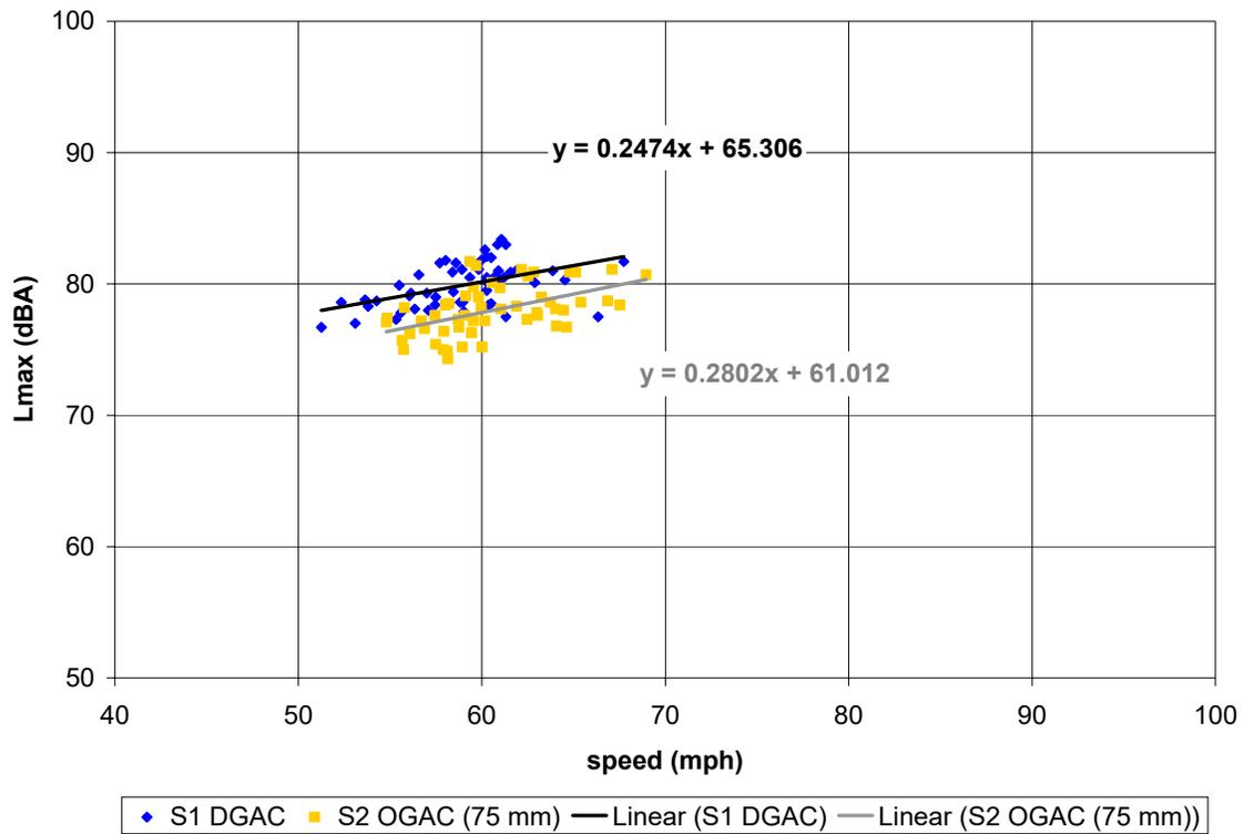
**Figure C-38. (this and previous page) Vehicle pass-by data, post-overlay, 16 months age; Site 1 (DGAC 30mm), Site 2 (OGAC 75mm). Automobiles (top), medium trucks (middle), and heavy trucks (bottom). Microphone location: distance 50 ft, height 5 ft.**
