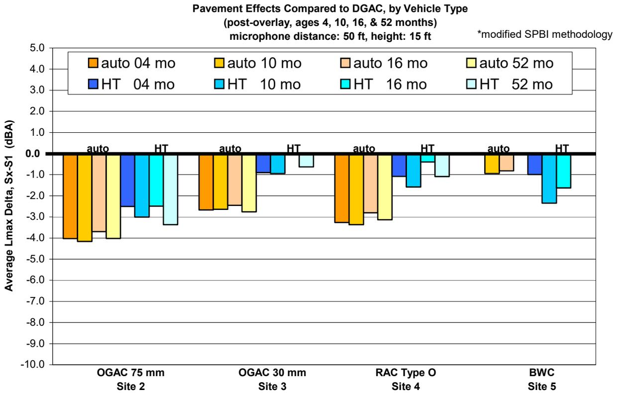
**Figure E-3. Pavement effects compared to DGAC (Site x minus Site 1) for autos and heavy trucks using modified SPBI.\* Post-overlay results, all pavements, including DGAC, aged 4, 10, 16, and 52 months (limited data for BWC). Microphone location: distance 15 m (50 ft), height 4.5 m (15 ft).**
