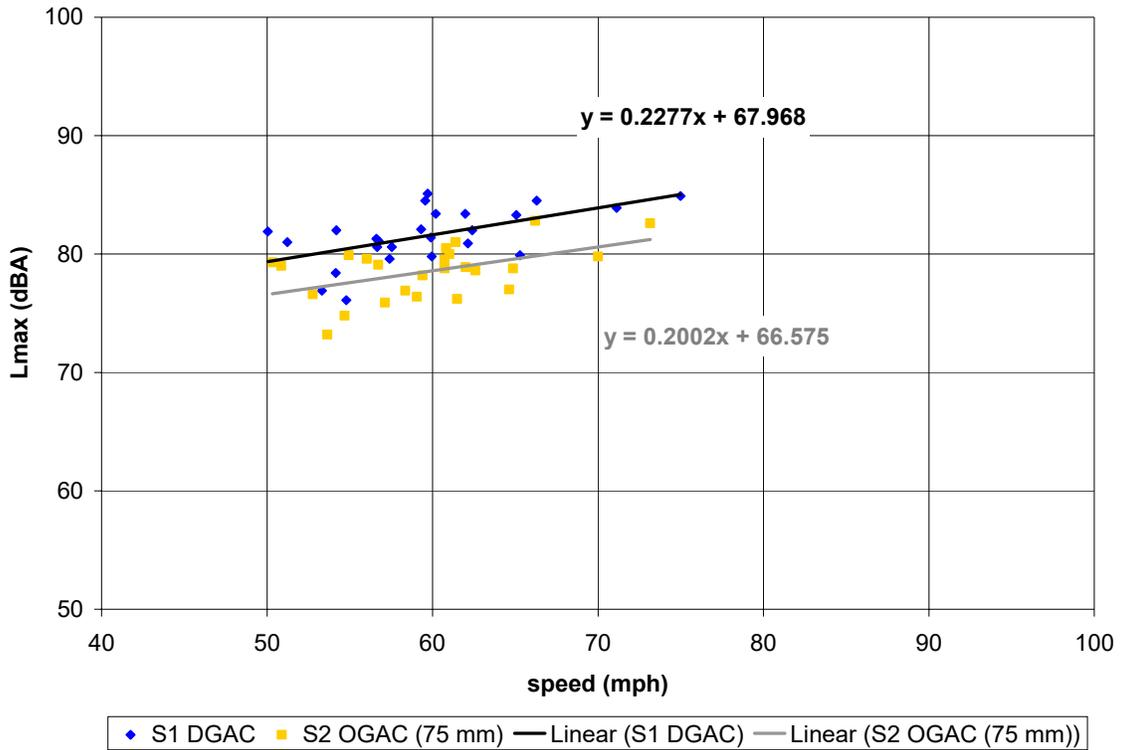
**Figure C-27. (this and previous page) Vehicle pass-by data, post-overlay, 10 months age; Site 1 (DGAC 30mm), Site 2 (OGAC 75mm). Automobiles (top), medium trucks (middle), and heavy trucks (bottom). Microphone location: distance 50 ft, height 15 ft.**
