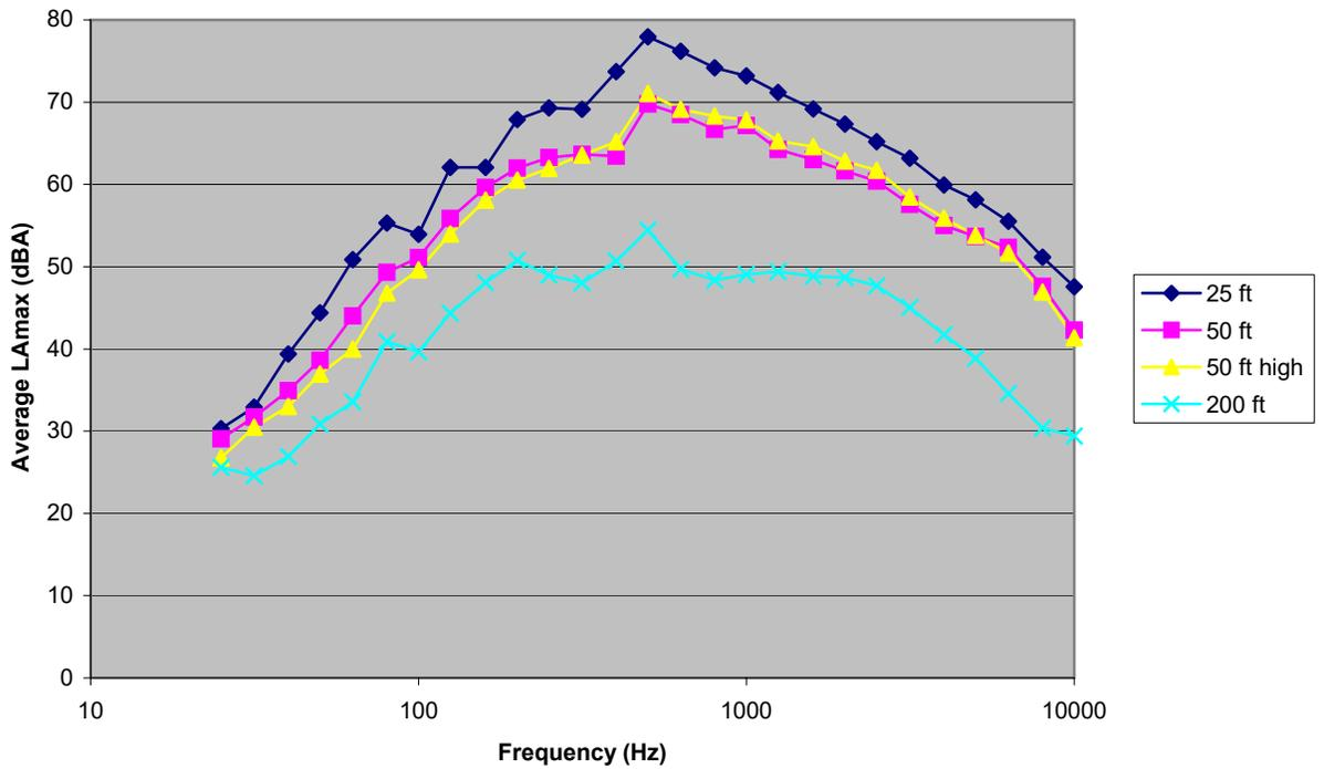
Figure E-25. Spectral data for automobiles (top) and heavy trucks (bottom); post-overlay results for Site 2 (OGAC 75 mm) aged 16 months; all microphone positions.
