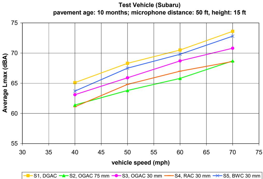
**Figure F-2. Test vehicle average L<sub>AFmx</sub> values for pavement aged 10 months, multiple speeds. Microphone position: (top) distance 15 m (50 ft), height 1.5 m (5 ft); (bottom) distance 15 m (50 ft), height 4.5 m (15 ft). Site bias removed.**
