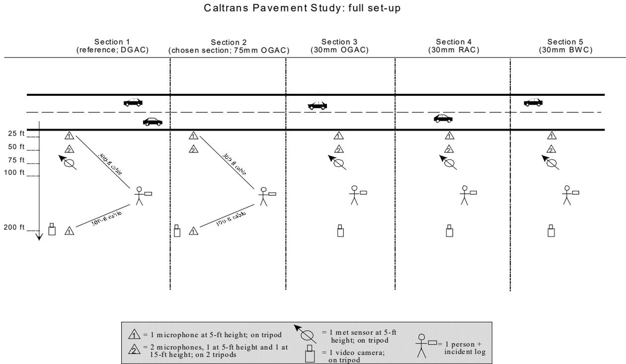
**Figure 3. Illustration of basic instrumentation set-up. (Not proportional or to scale)**
