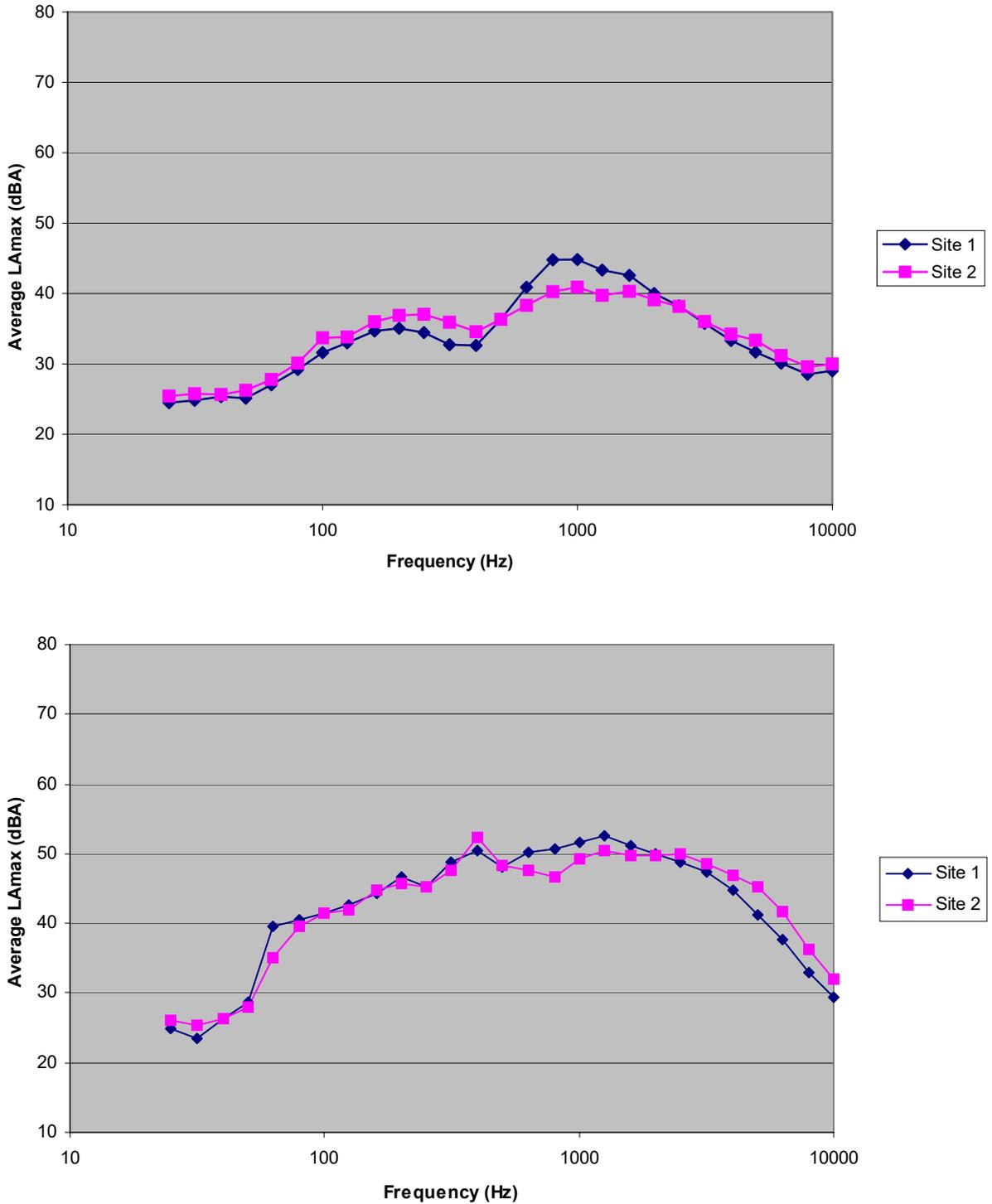
**Figure E-11. Spectral data for automobiles (top) and heavy trucks (bottom) on four different pavement types. Post-overlay results, all pavements aged 10 months. Microphone location: distance 200 ft, height 5 ft.**
