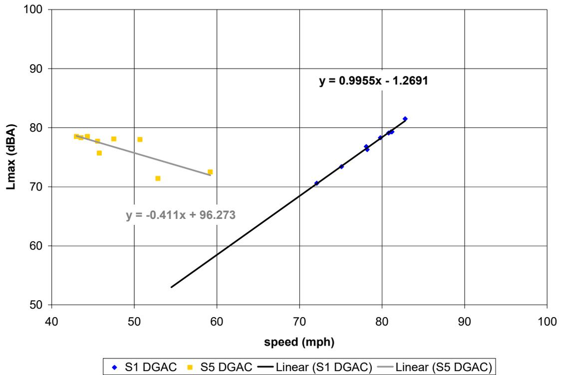
**Figure C-11. (this and previous page) Vehicle pass-by data, pre-overlay; Site 1 (DGAC), Site 5 (DGAC). Automobiles (top), medium trucks (middle), and heavy trucks (bottom). Microphone location: distance 50 ft, height 5 ft.**
