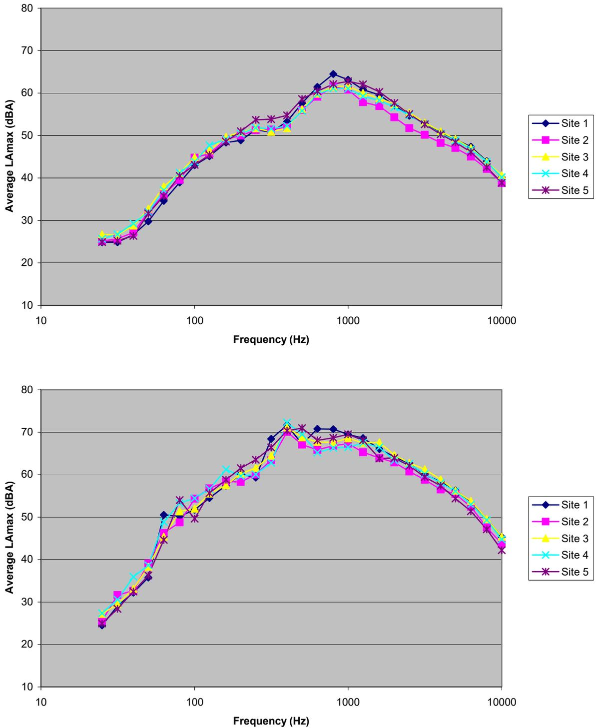
**Figure E-9. Spectral data for automobiles (top) and heavy trucks (bottom) on four different pavement types. Post-overlay results, all pavements aged 10 months. Microphone location: distance 50 ft, height 5 ft.**
