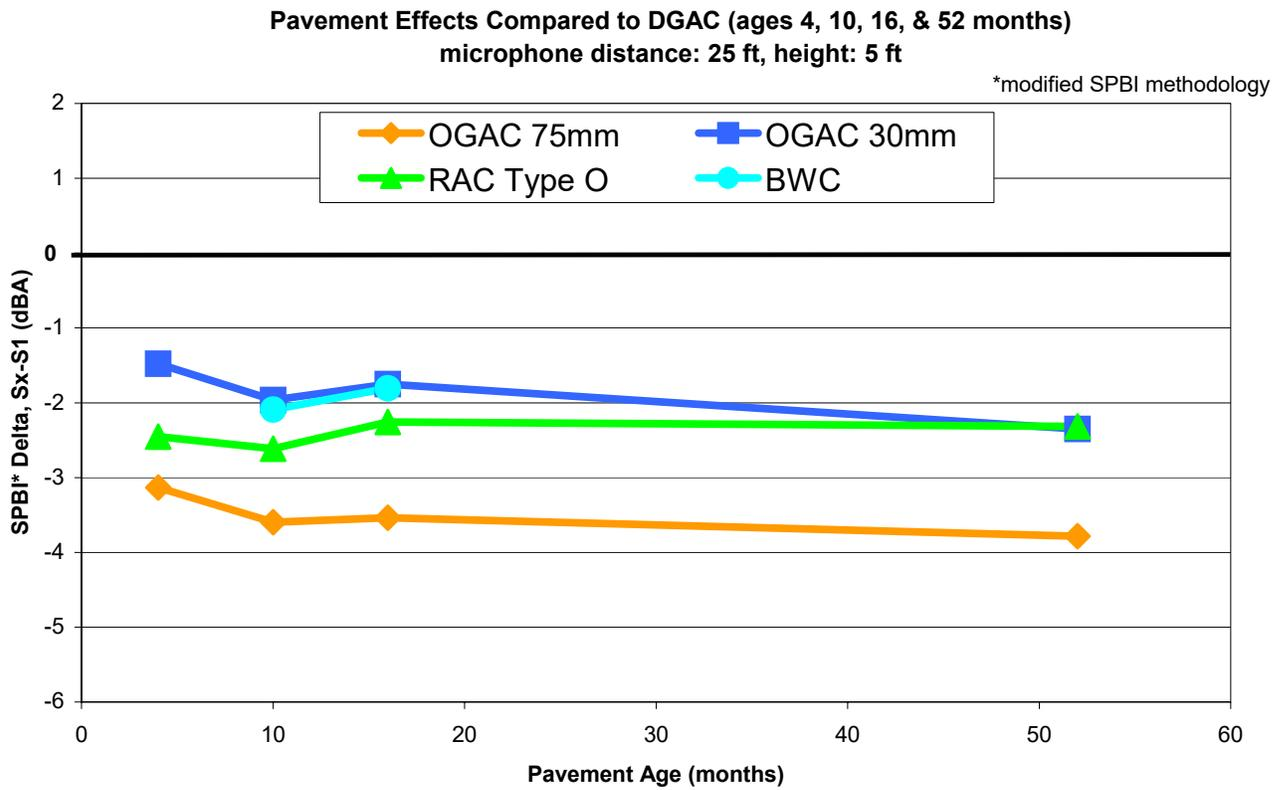
**Figure D-12. Pavement effects compared to DGAC (Site x minus Site 1) using modified SPBI. Post-overlay results, all pavements, including DGAC, aged 4, 10, 16, and 52 months (limited data for BWC). Microphone location: distance 7.5 m (25 ft), height 1.5 m (5 ft).**
