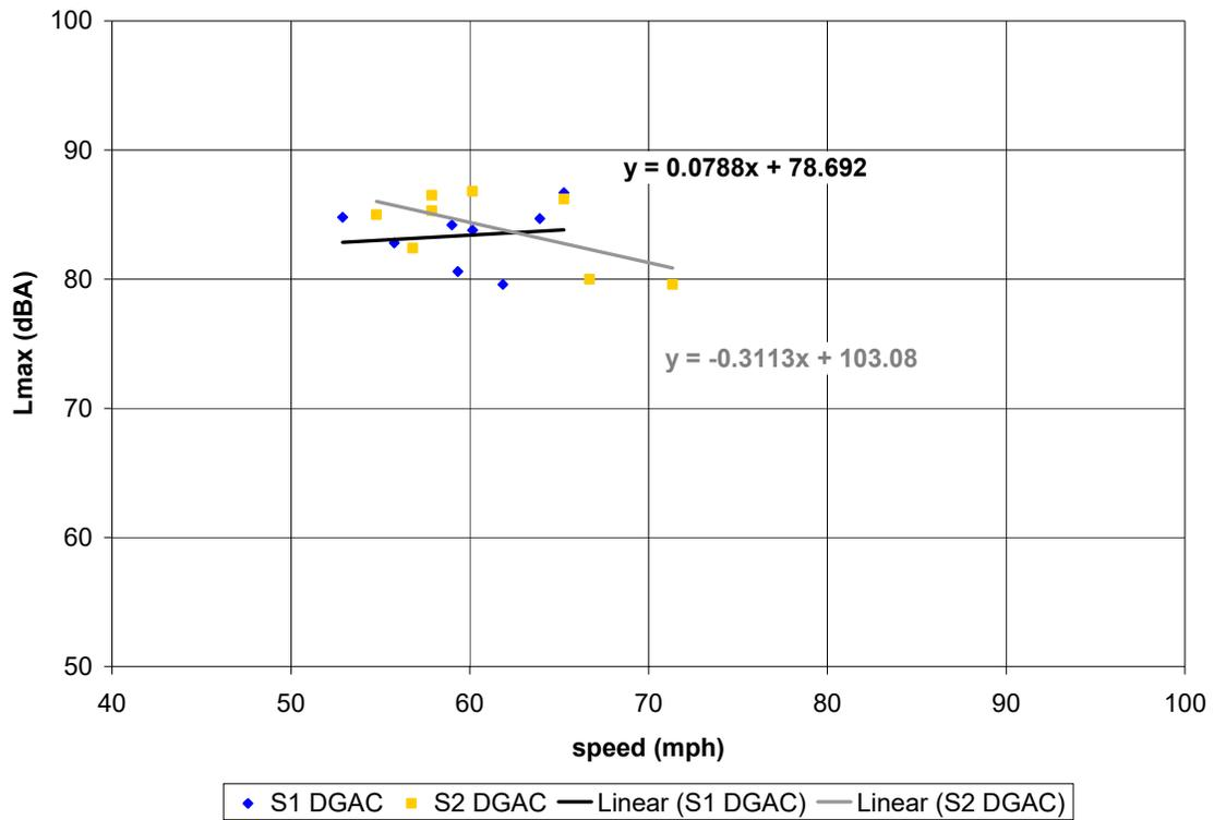
**Figure C-1. (this and previous page) Vehicle pass-by data, pre-overlay; Site 1 (DGAC), Site 2 (DGAC). Automobiles (top), medium trucks (middle), and heavy trucks (bottom). Microphone location: distance 25 ft, height 5 ft.**
