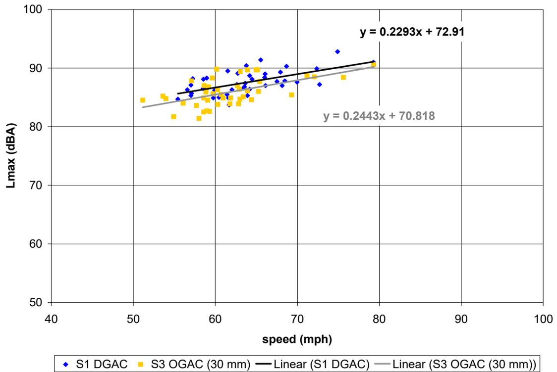
**Figure C-52. (this and previous page) Vehicle pass-by data, post-overlay, 52 months age; Site 1 (DGAC 30mm), Site 3 (OGAC 30mm). Automobiles (top), medium trucks (middle), and heavy trucks (bottom). Microphone location: distance 25 ft, height 5 ft.**
