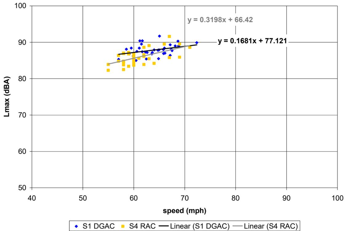
**Figure C-55. (this and previous page) Vehicle pass-by data, post-overlay, 52 months age; Site 1 (DGAC 30mm), Site 4 (RAC Type O 30mm). Automobiles (top), medium trucks (middle), and heavy trucks (bottom). Microphone location: distance 25 ft, height 5 ft.**
