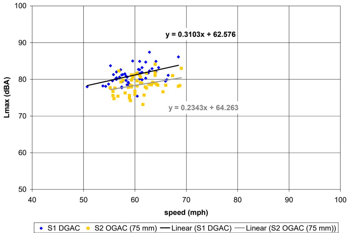
**Figure C-15. Vehicle pass-by data, post-overlay, 4 months age; Site 1 (DGAC 30mm), Site 2 (OGAC 75mm). Automobiles (top), medium trucks (middle), and heavy trucks (bottom). Microphone location: distance 50 ft, height 15 ft.**
