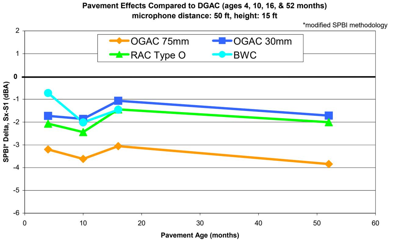
**Figure D-14. Pavement effects compared to DGAC (Site x minus Site 1) using modified SPBI. Post-overlay results, all pavements, including DGAC, aged 4, 10, 16, and 52 months (limited data for BWC). Microphone location: distance 15 m (50 ft), height 4.5 m (15 ft).**
