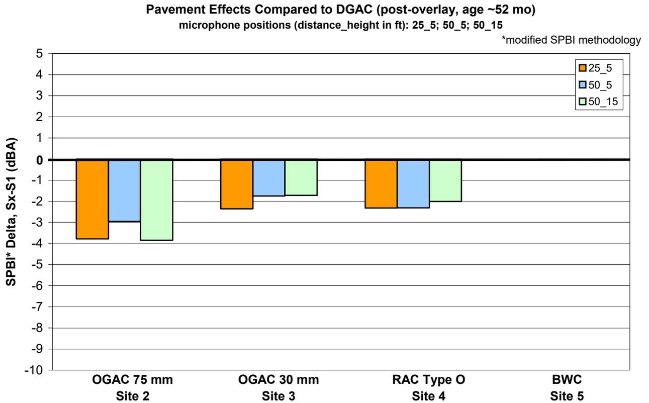
**Figure D-11. Pavement effects compared to DGAC (Site x minus Site 1) using modified SPBI. Post-overlay results, all pavements, including DGAC, aged 52 months. Microphone locations: distance 7.5 m (25 ft), height 1.5 m (5 ft); distance 15 m (50 ft), height 1.5 m (5 ft); distance 15 m (50 ft), height 4.5 m (15 ft).**
