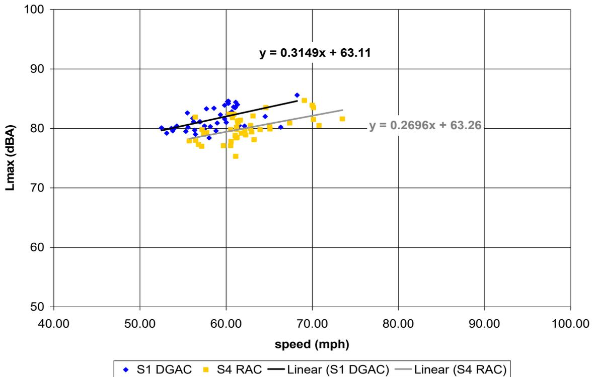
**Figure C-45. (this and previous page) Vehicle pass-by data, post-overlay, 16 months age; Site 1 (DGAC 30mm), Site 4 (RAC Type O 30mm). Automobiles (top), medium trucks (middle), and heavy trucks (bottom). Microphone location: distance 50 ft, height 15 ft.**
