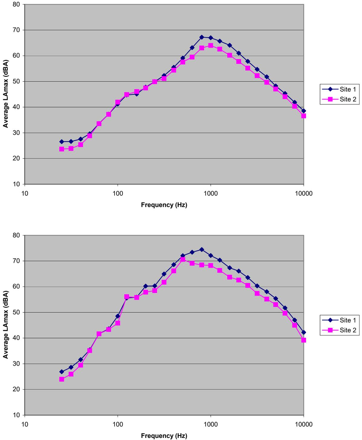
**Figure E-18. Spectral data for automobiles (top) and heavy trucks (bottom) on four different pavement types. Post-overlay results, all pavements aged 52 months. Microphone location: distance 50 ft, height 15 ft.**
