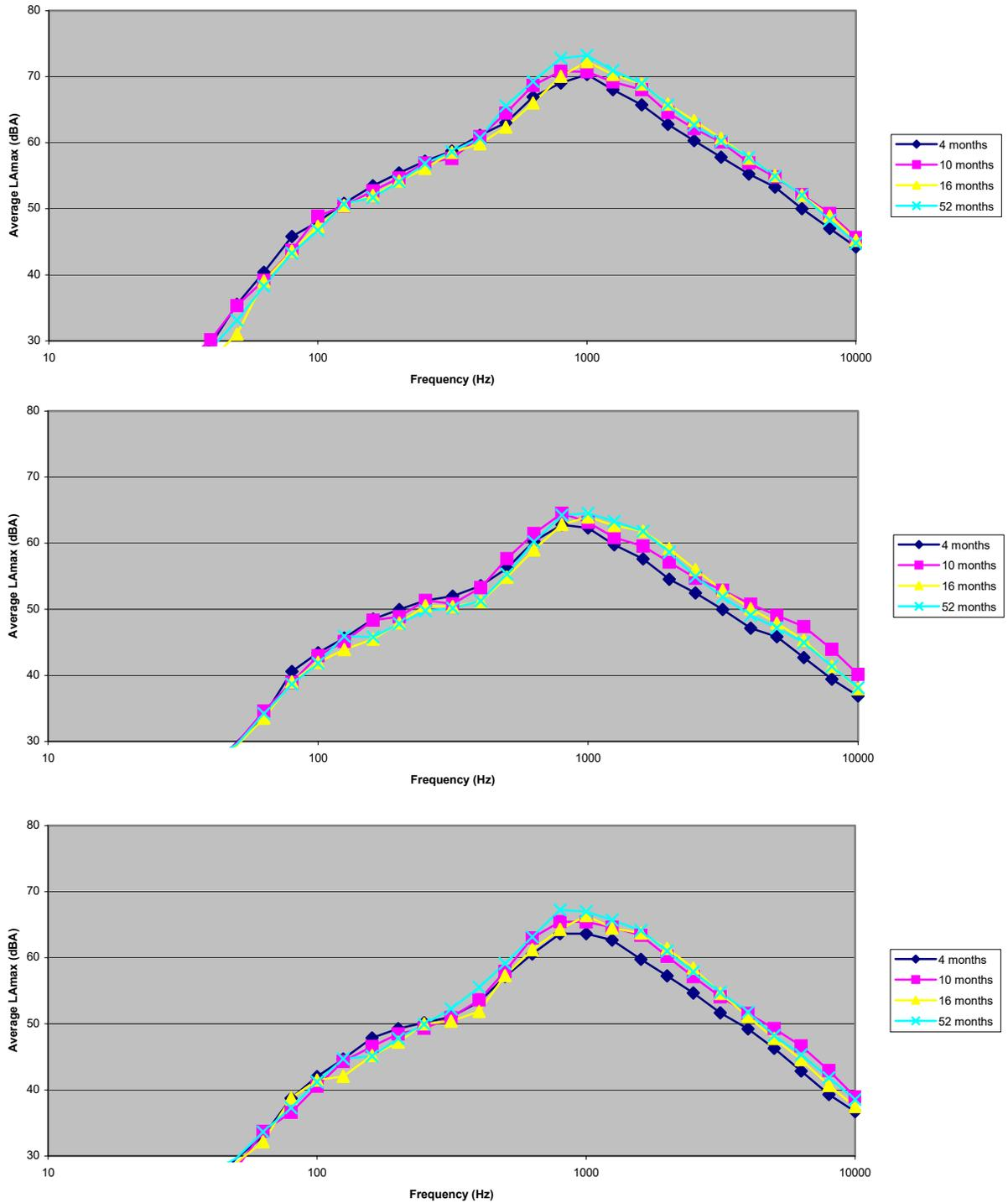
**Figure E-19. Spectral data for automobiles; post-overlay results for Site 1 (DGAC 30 mm); all ages measured. Microphone location: distance 25 ft, height 5 ft (top); microphone location: distance 50 ft, height 5 ft (middle); microphone location: distance 50 ft, height 15 ft (bottom).**
