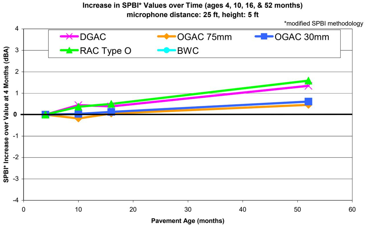
**Figure D-5. Increase in SPBI\* values over time, as compared to values at 4 months. Post-overlay results, all pavements (except BWC – no data available), including DGAC, aged 4, 10, 16, and 52 months. Microphone location: distance 7.5 m (25 ft), height 1.5 m (5 ft).**
