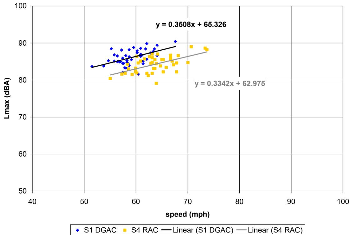
**Figure C-19. (this and previous page) Vehicle pass-by data, post-overlay, 4 months age; Site 1 (DGAC 30mm), Site 4 (RAC Type O 30mm). Automobiles (top), medium trucks (middle), and heavy trucks (bottom). Microphone location: distance 25 ft, height 5 ft.**
