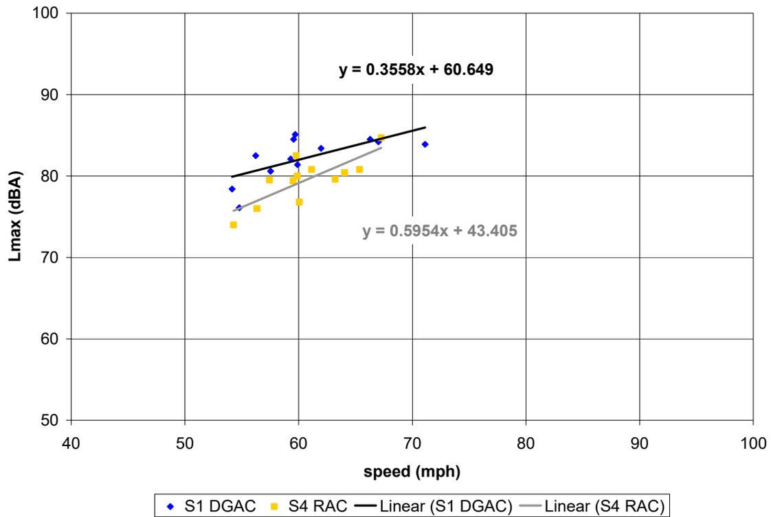
**Figure C-33. (this and previous page) Vehicle pass-by data, post-overlay, 10 months age; Site 1 (DGAC 30mm), Site 4 (RAC Type O 30mm). Automobiles (top), medium trucks (middle), and heavy trucks (bottom). Microphone location: distance 50 ft, height 15 ft.**
