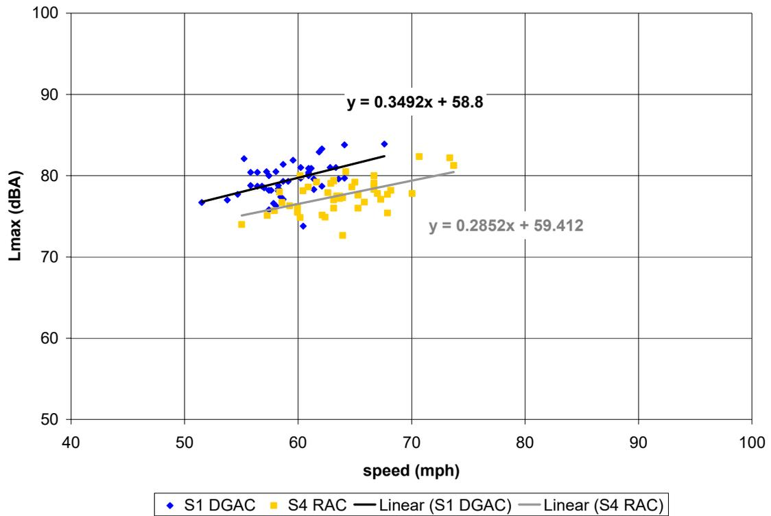
**Figure C-20. (this and previous page) Vehicle pass-by data, post-overlay, 4 months age; Site 1 (DGAC 30mm), Site 4 (RAC Type O 30mm). Automobiles (top), medium trucks (middle), and heavy trucks (bottom). Microphone location: distance 50 ft, height 5 ft.**
