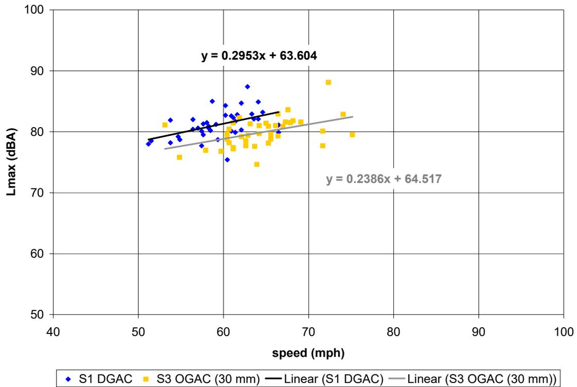
**Figure C-18. (this and previous page) Vehicle pass-by data, post-overlay, 4 months age; Site 1 (DGAC 30mm), Site 3 (OGAC 30mm). Automobiles (top), medium trucks (middle), and heavy trucks (bottom). Microphone location: distance 50 ft, height 15 ft.**
