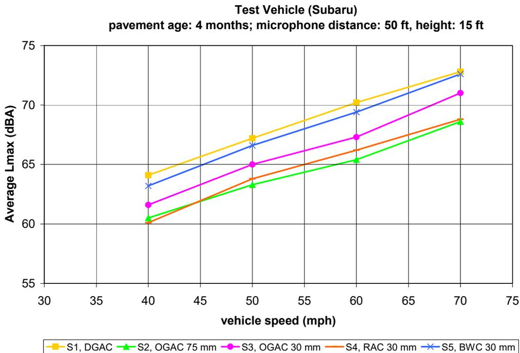
**Figure F-1. Test vehicle average  $L_{AFmx}$  values for pavement aged 4 months, multiple speeds. Microphone position: (top) distance 15 m (50 ft), height 1.5 m (5 ft); (bottom) distance 15 m (50 ft), height 4.5 m (15 ft). Site bias removed.**
