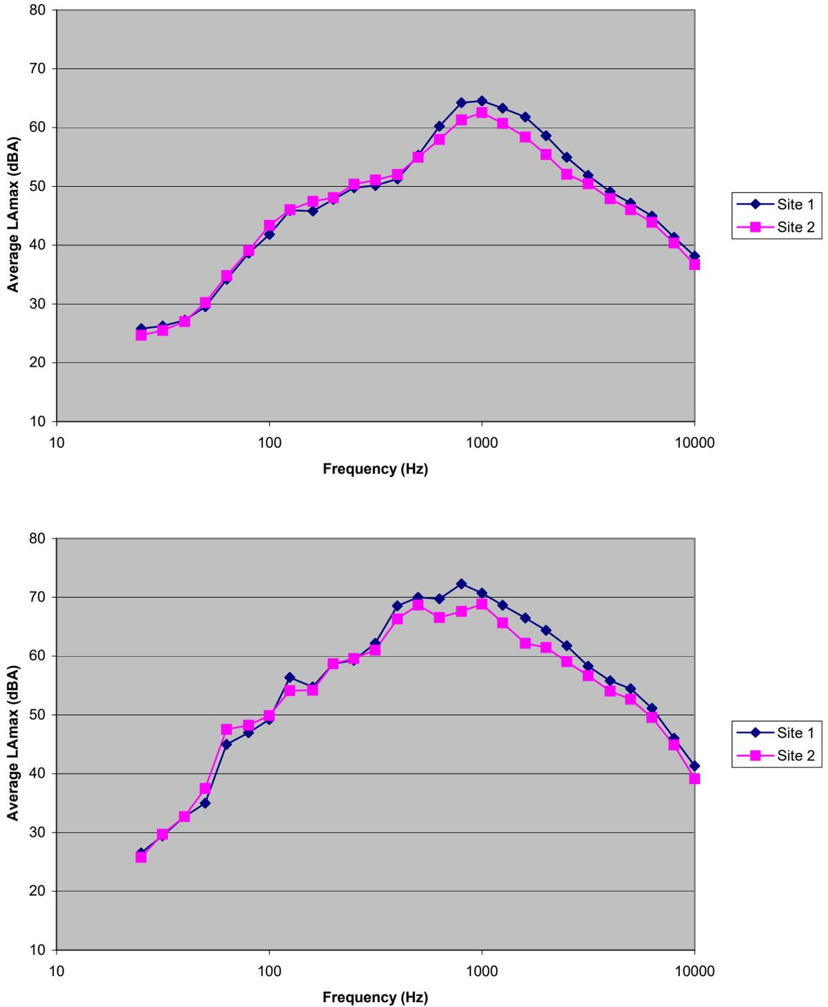
**Figure E-17. Spectral data for automobiles (top) and heavy trucks (bottom) on four different pavement types. Post-overlay results, all pavements aged 52 months. Microphone location: distance 50 ft, height 5 ft.**
