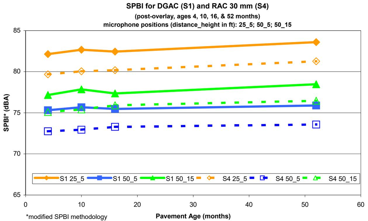
**Figure D-3. SPBI\* values over time for pavement pair DGAC 30mm (S1) and RAC Type O 30mm (S4). Overlay pavements aged 4, 10, 16, and 52 months. Microphone locations: distance 7.5 m (25 ft), height 1.5 m (5 ft); distance 15 m (50 ft), height 1.5 m (5 ft); distance 15 m (50 ft), height 4.5 m (15 ft).**
