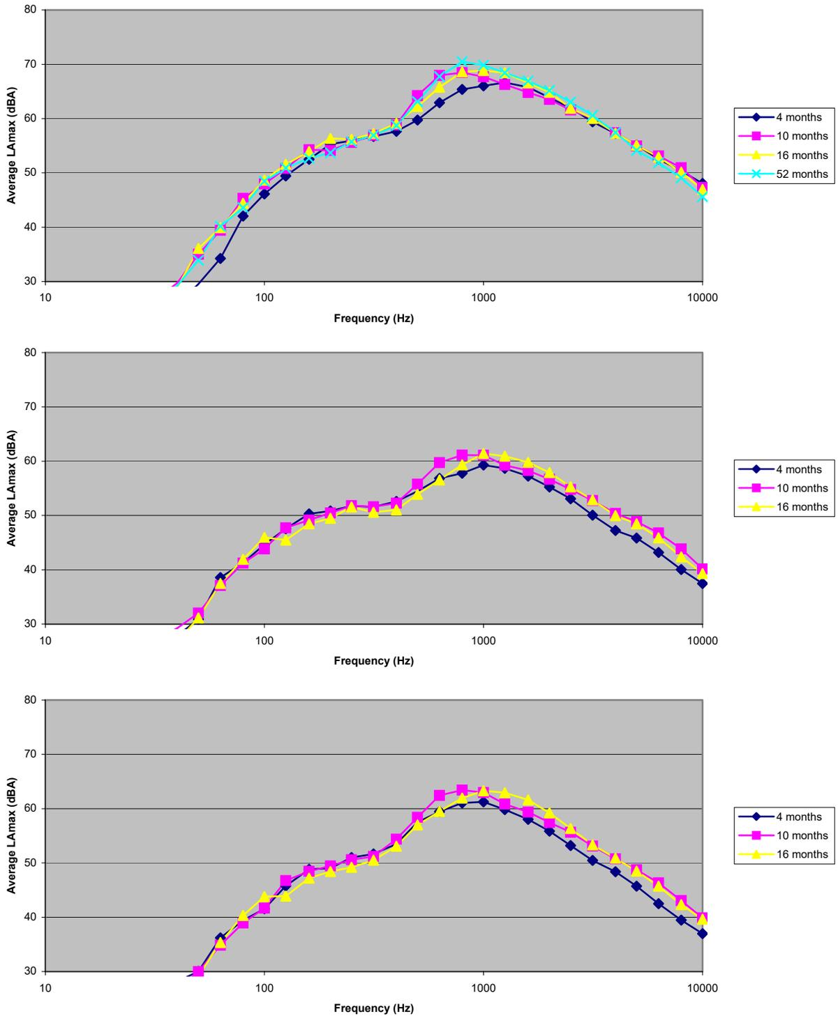
**Figure E-22. Spectral data for automobiles; post-overlay results for Site 4 (RAC Type O 30 mm); all ages measured. Microphone location: distance 25 ft, height 5 ft (top); microphone location: distance 50 ft, height 5 ft (middle); microphone location: distance 50 ft, height 15 ft (bottom).**
