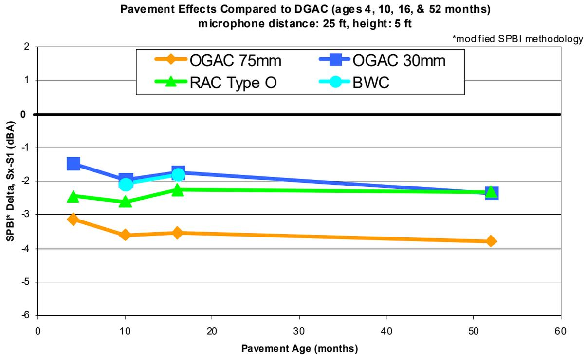
**Figure 5. Pavement effects compared to DGAC (Site x minus Site 1) using modified SPBI (limited data for BWC). Microphone location: distance 7.5 m (25 ft), height 1.5 m (5 ft).**
