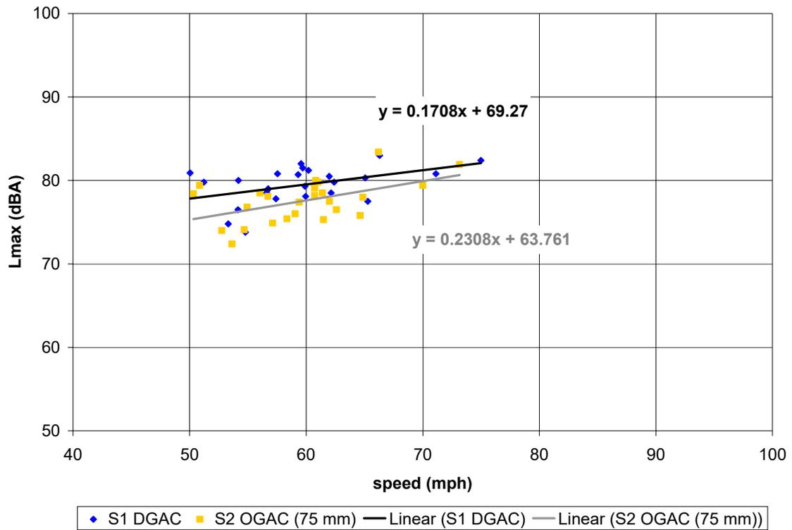
**Figure C-26. (this and previous page) Vehicle pass-by data, post-overlay, 10 months age; Site 1 (DGAC 30mm), Site 2 (OGAC 75mm). Automobiles (top), medium trucks (middle), and heavy trucks (bottom). Microphone location: distance 50 ft, height 5 ft.**
