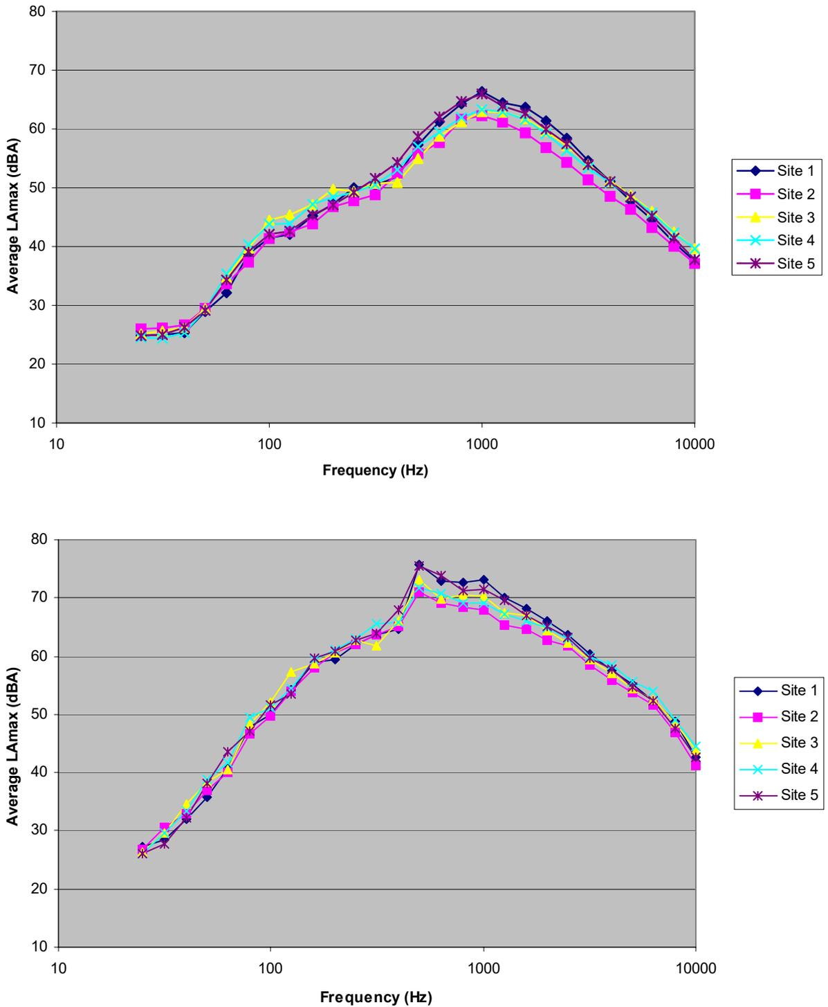
**Figure E-14. Spectral data for automobiles (top) and heavy trucks (bottom) on four different pavement types. Post-overlay results, all pavements aged 16 months. Microphone location: distance 50 ft, height 15 ft.**
