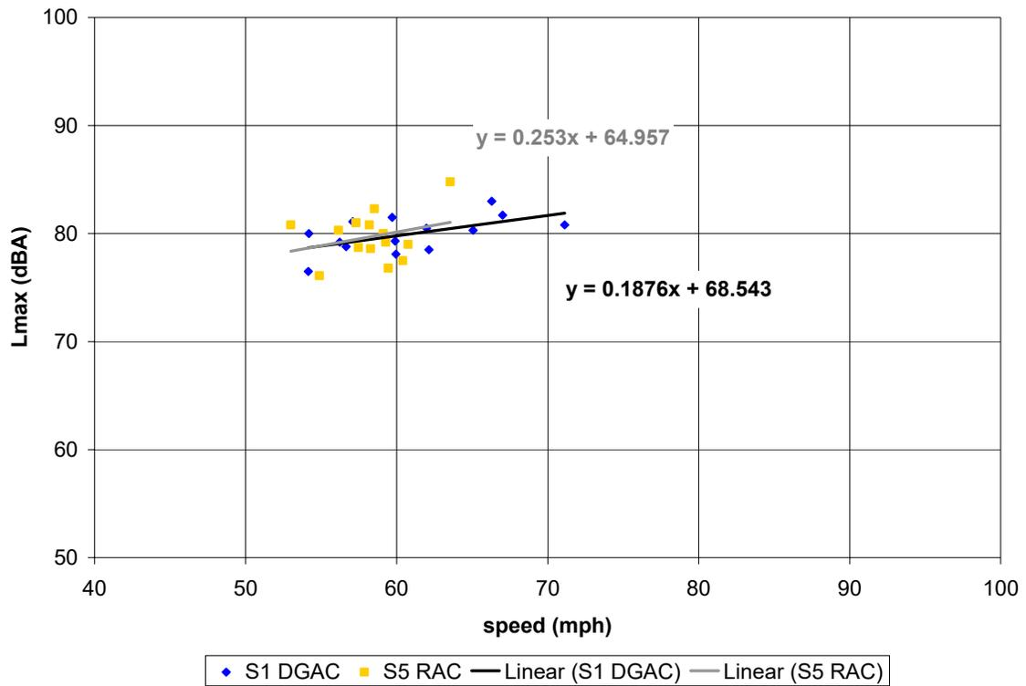
**Figure C-35. (this and previous page) Vehicle pass-by data, post-overlay, 10 months age; Site 1 (DGAC 30mm), Site 5 (BWC 30mm). Automobiles (top), medium trucks (middle), and heavy trucks (bottom). Microphone location: distance 50 ft, height 5 ft.**
