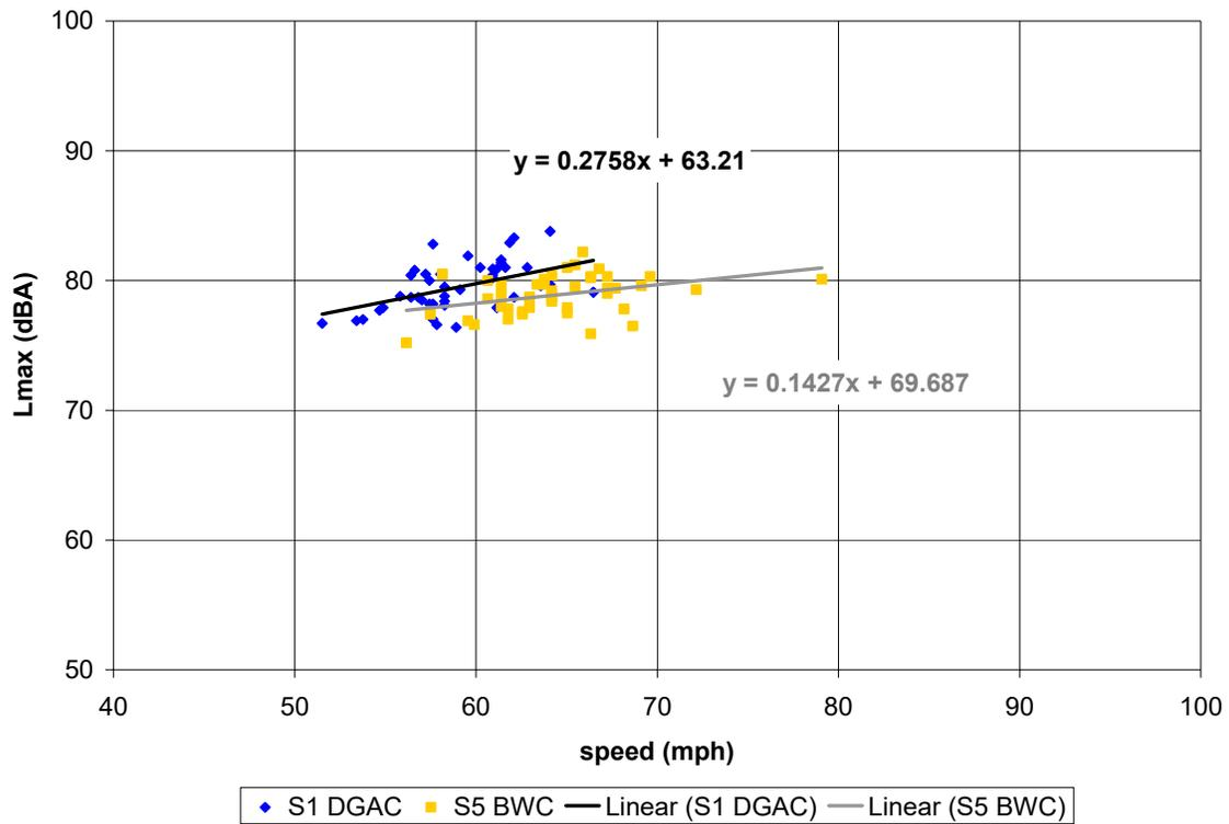
**Figure C-23. (this and previous page) Vehicle pass-by data, post-overlay, 4 months age; Site 1 (DGAC 30mm), Site 5 (BWC 30mm). Automobiles (top), medium trucks (middle), and heavy trucks (bottom). Microphone location: distance 50 ft, height 5 ft.**
