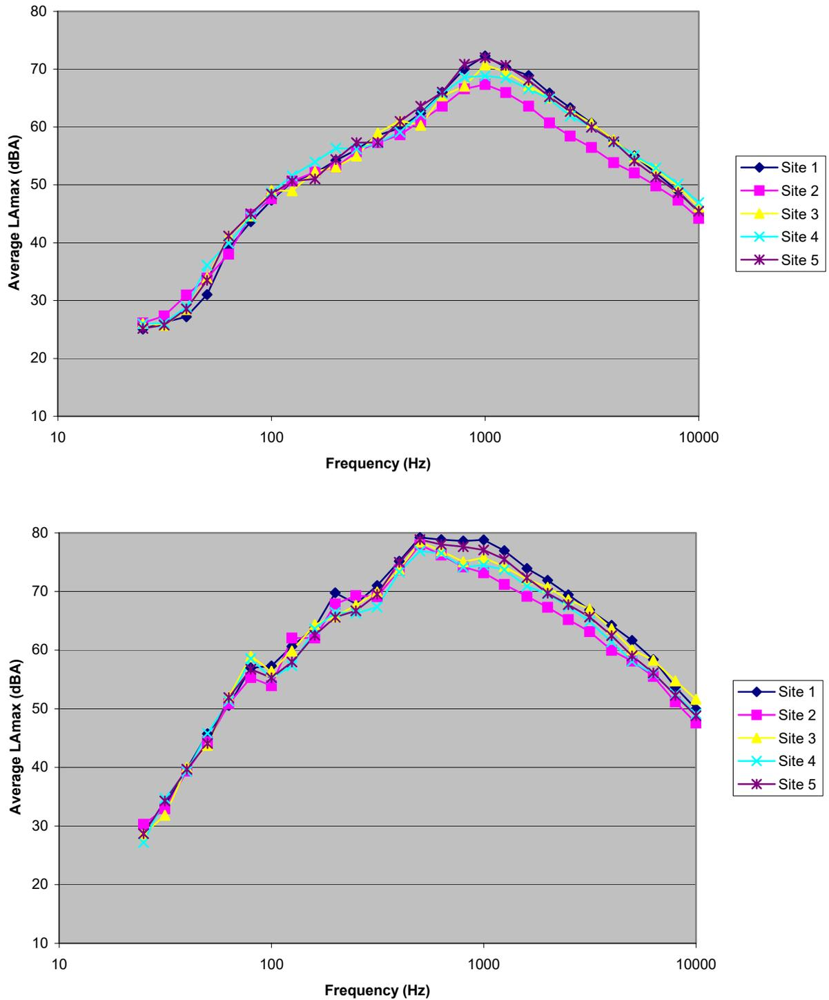
**Figure 8. Spectral data for automobiles (top) and heavy trucks (bottom) on four different pavement types. Post-overlay results, all pavements aged 16 months. Microphone location: distance 25 ft, height 5 ft.**
