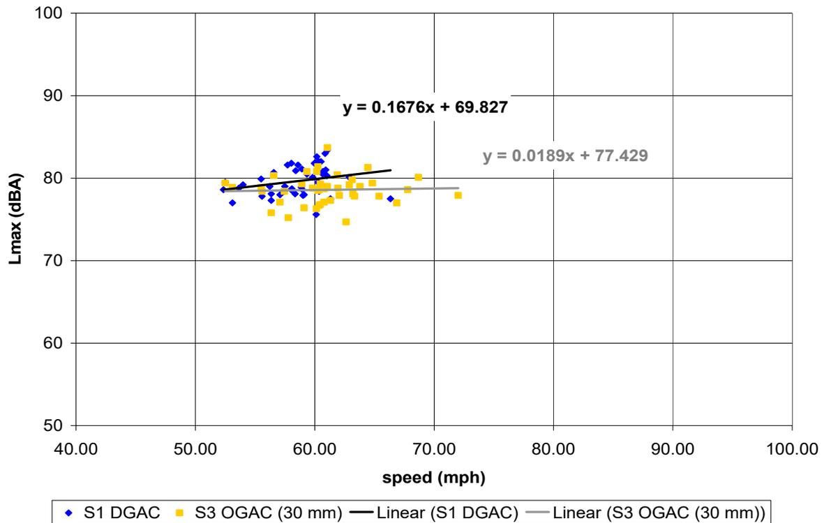
**Figure C-41. (this and previous page) Vehicle pass-by data, post-overlay, 16 months age; Site 1 (DGAC 30mm), Site 3 (OGAC 30mm). Automobiles (top), medium trucks (middle), and heavy trucks (bottom). Microphone location: distance 50 ft, height 5 ft.**
