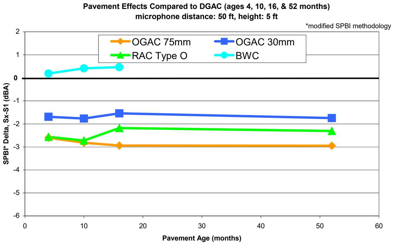
**Figure D-13. Pavement effects compared to DGAC (Site x minus Site 1) using modified SPBI. Post-overlay results, all pavements, including DGAC, aged 4, 10, 16, and 52 months (limited data for BWC). Microphone location: distance 15 m (50 ft), height 1.5 m (5 ft).**
