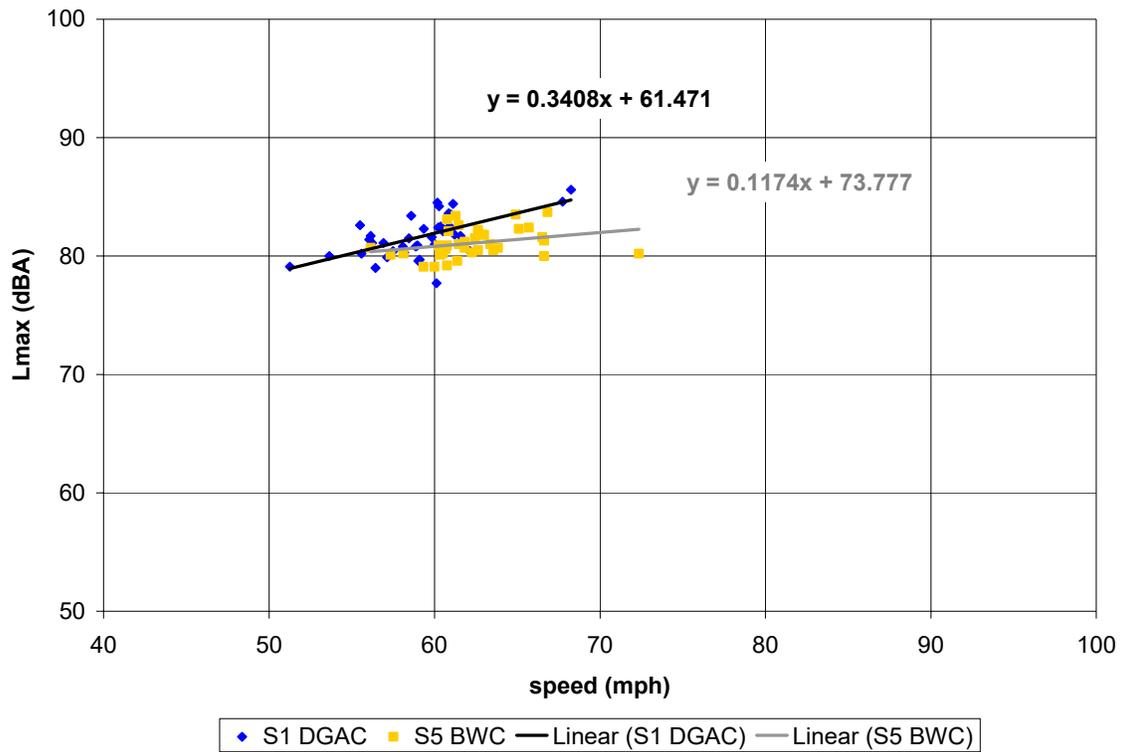
**Figure C-48. (this and previous page) Vehicle pass-by data, post-overlay, 16 months age; Site 1 (DGAC 30mm), Site 5 (BWC 30mm). Automobiles (top), medium trucks (middle), and heavy trucks (bottom). Microphone location: distance 50 ft, height 15 ft.**
