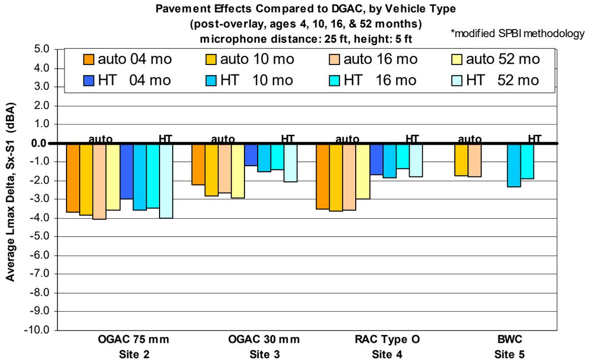
**Figure 7. Pavement effects compared to DGAC (Site x minus Site 1) for autos and heavy trucks using modified SPBI.\* Microphone location: distance 7.5 m (25 ft), height 1.5 m (5 ft).**
