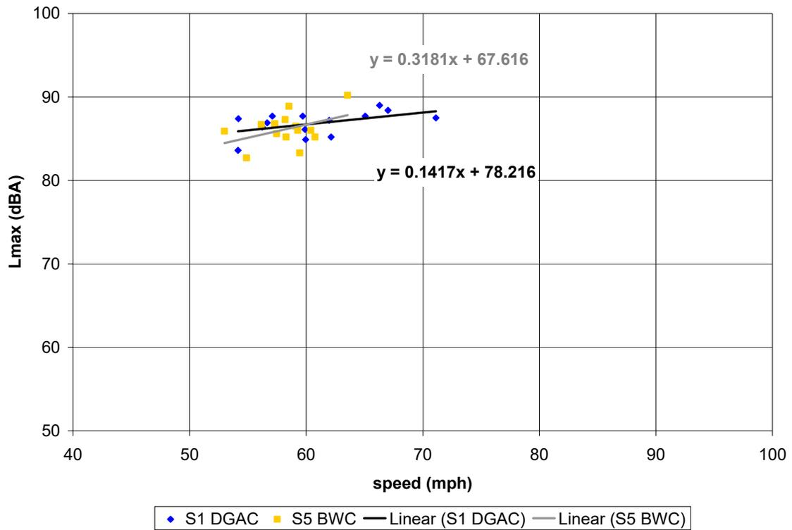
**Figure C-34. (this and previous page) Vehicle pass-by data, post-overlay, 10 months age; Site 1 (DGAC 30mm), Site 5 (BWC 30mm). Automobiles (top), medium trucks (middle), and heavy trucks (bottom). Microphone location: distance 25 ft, height 5 ft.**
