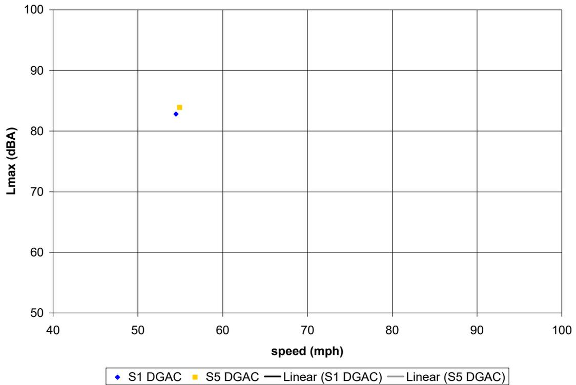
**Figure C-12. (this and previous page) Vehicle pass-by data, pre-overlay; Site 1 (DGAC), Site 5 (DGAC). Automobiles (top), medium trucks (middle), and heavy trucks (bottom). Microphone location: distance 50 ft, height 15 ft.**
