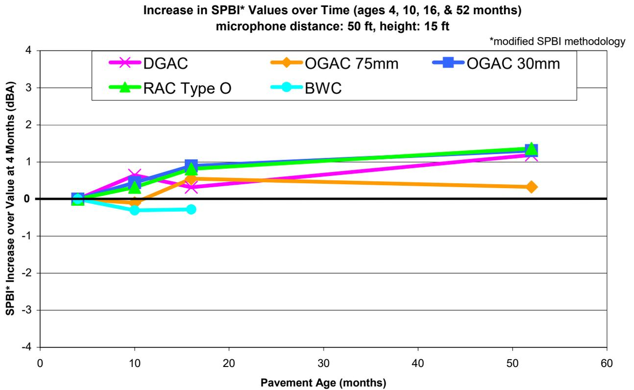
**Figure D-7. Increase in SPBI\* values over time, as compared to values at 4 months. Post-overlay results, all pavements, including DGAC, aged 4, 10, 16, and 52 months (limited data for BWC). Microphone location: distance 15 m (50 ft), height 4.5 m (15 ft).**
