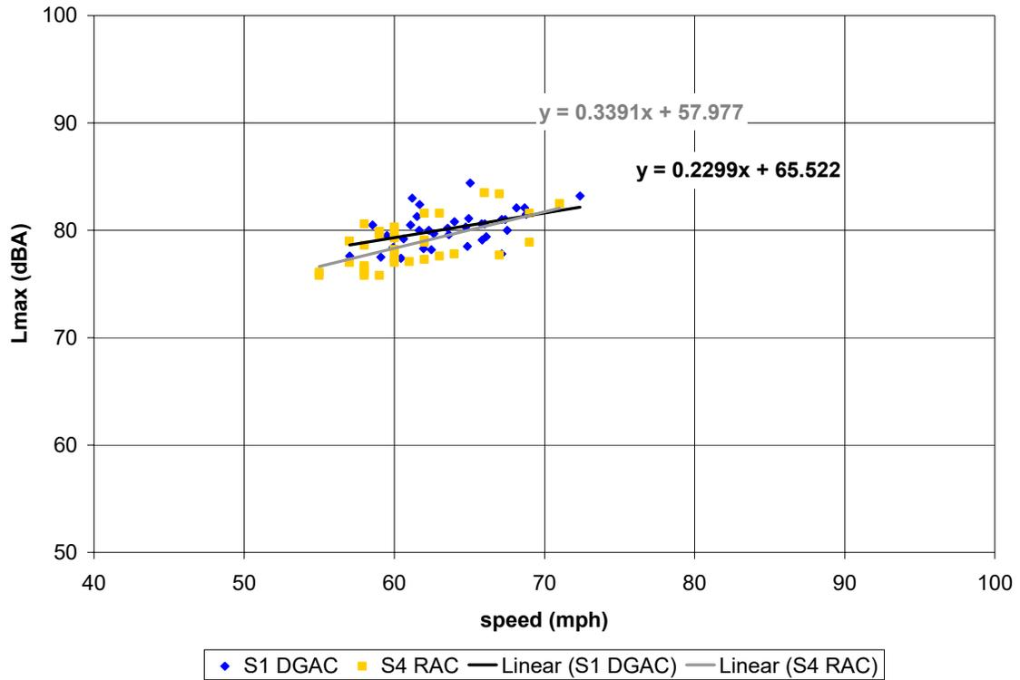
**Figure C-56. (this and previous page) Vehicle pass-by data, post-overlay, 52 months age; Site 1 (DGAC 30mm), Site 4 (RAC Type O 30mm). Automobiles (top), medium trucks (middle), and heavy trucks (bottom). Microphone location: distance 50 ft, height 5 ft.**
