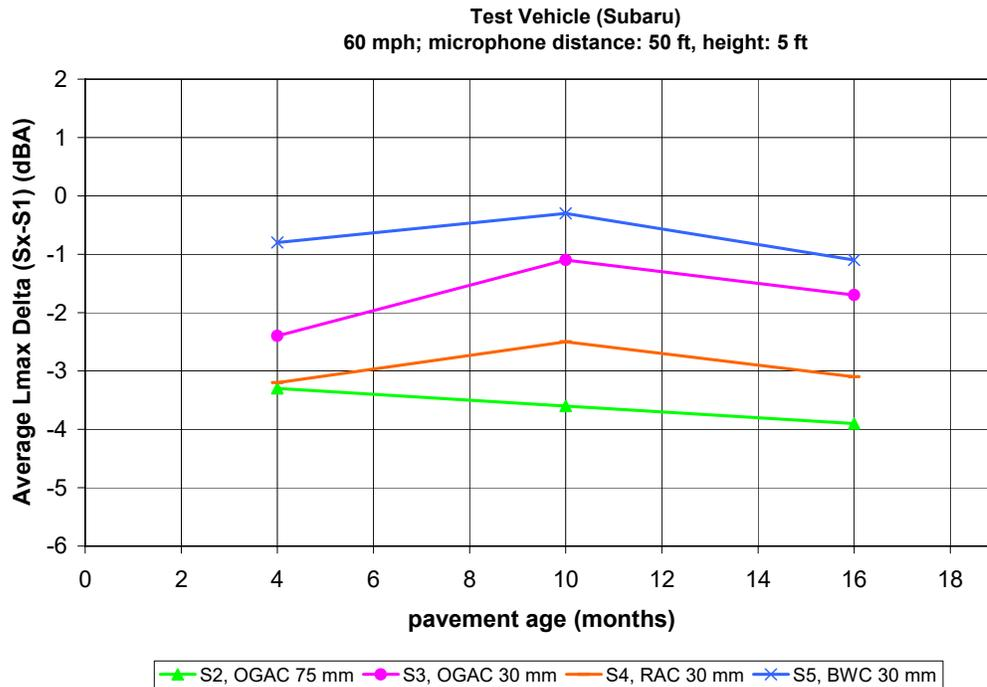
**Figure 10.** Test vehicle average  $L_{AFmx}$  deltas (Site x minus Site 1) for pavement ages 4 months, 10 months, and 16 months, 100 km/h (60 mph). Microphone position: distance 15 m (50 ft), height 1.5 m (5 ft). Site bias removed.
