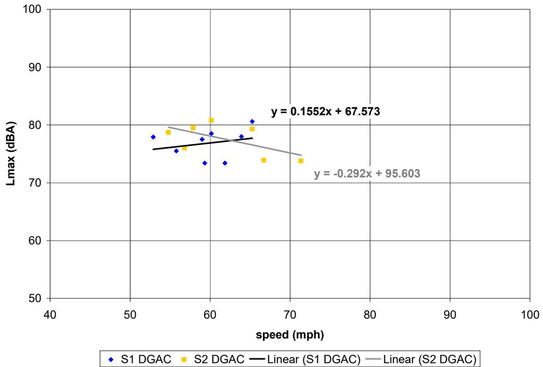
**Figure C-2. (this and previous page) Vehicle pass-by data, pre-overlay; Site 1 (DGAC), Site 2 (DGAC). Automobiles (top), medium trucks (middle), and heavy trucks (bottom). Microphone location: distance 50 ft, height 5 ft.**
