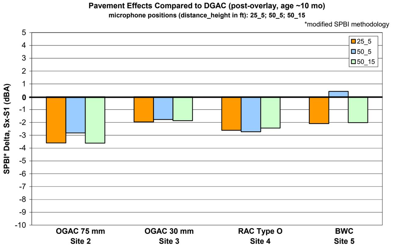
**Figure D-9. Pavement effects compared to DGAC (Site x minus Site 1) using modified SPBI. Post-overlay results, all pavements, including DGAC, aged 10 months. Microphone locations: distance 7.5 m (25 ft), height 1.5 m (5 ft); distance 15 m (50 ft), height 1.5 m (5 ft); distance 15 m (50 ft), height 4.5 m (15 ft).**
