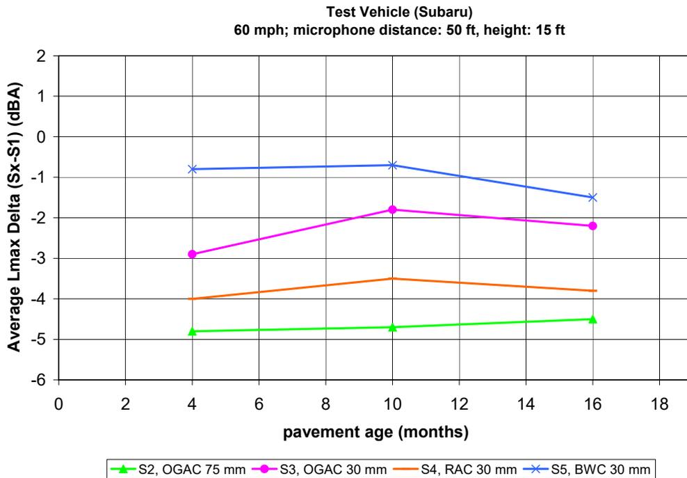
**Figure F-4. Test vehicle average  $L_{AFmx}$  deltas (Site x minus Site 1) for pavement ages 4 months, 10 months, and 16 months, 100 km/h (60 mph). Microphone position: (top) distance 15 m (50 ft), height 1.5 m (5 ft); (bottom) distance 15 m (50 ft), height 4.5 m (15 ft). Site bias removed.**
