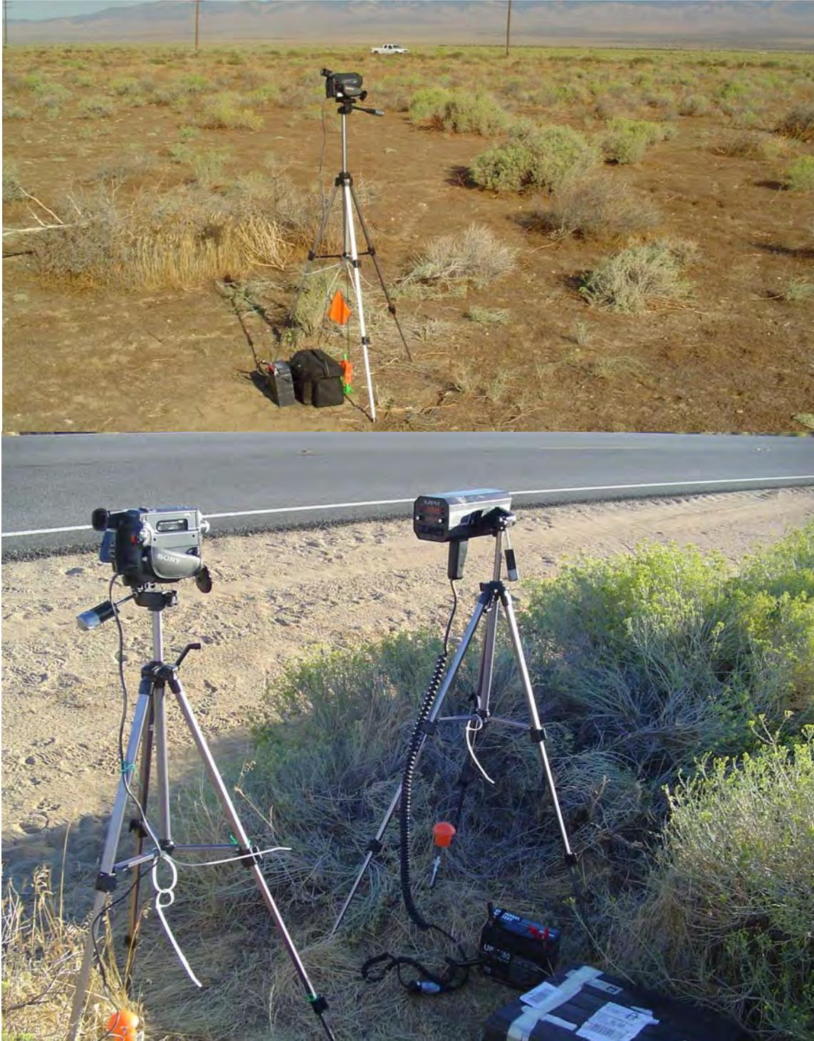
**Figure B-4. Video cameras and radar gun.**
