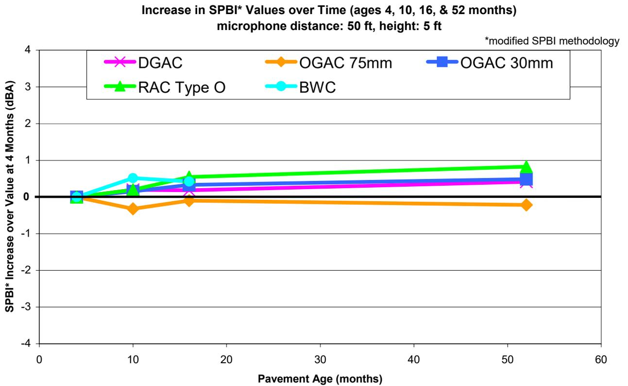
**Figure D-6. Increase in SPBI\* values over time, as compared to values at 4 months. Post-overlay results, all pavements, including DGAC, aged 4, 10, 16, and 52 months (limited data for BWC). Microphone location: distance 15 m (50 ft), height 1.5 m (5 ft).**
