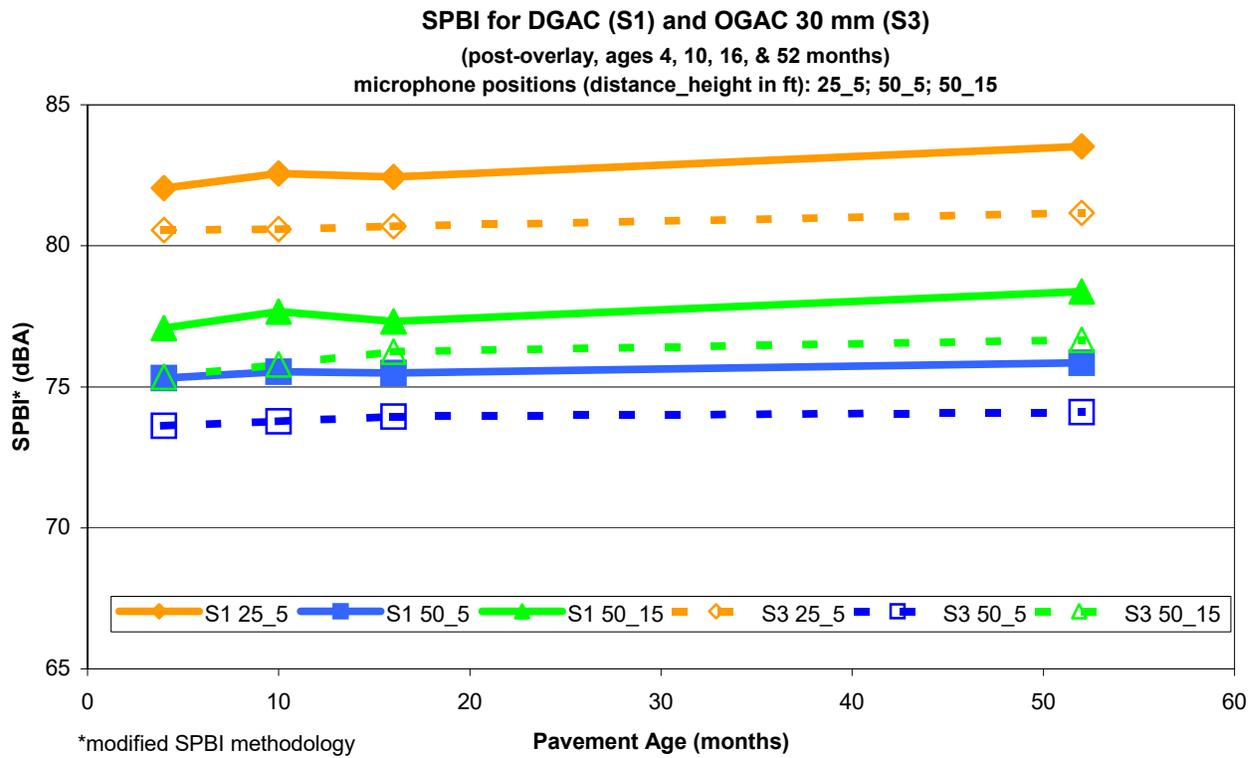
**Figure D-2. SPBI\* values over time for pavement pair DGAC 30mm (S1) and OGAC 30mm (S3). Overlay pavements aged 4, 10, 16, and 52 months. Microphone locations: distance 7.5 m (25 ft), height 1.5 m (5 ft); distance 15 m (50 ft), height 1.5 m (5 ft); distance 15 m (50 ft), height 4.5 m (15 ft).**
