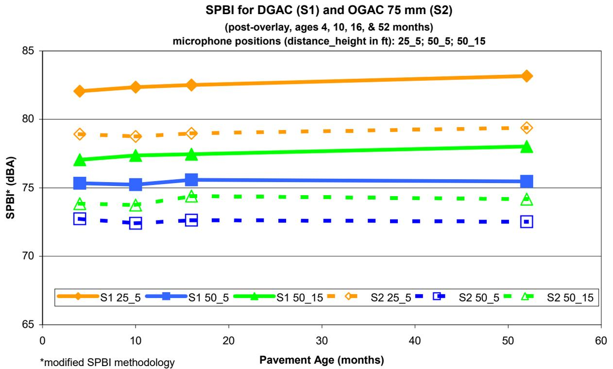
**Figure D-1. SPBI\* values over time for pavement pair DGAC 30mm (S1) and OGAC 75mm (S2). Overlay pavements aged 4, 10, 16, and 52 months. Microphone locations: distance 7.5 m (25 ft), height 1.5 m (5 ft); distance 15 m (50 ft), height 1.5 m (5 ft); distance 15 m (50 ft), height 4.5 m (15 ft).**
