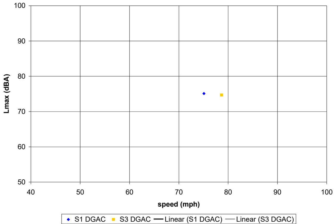
**Figure C-6. (this and previous page) Vehicle pass-by data, pre-overlay; Site 1 (DGAC), Site 3 (DGAC). Automobiles (top), medium trucks (middle), and heavy trucks (bottom). Microphone location: distance 50 ft, height 15 ft.**
