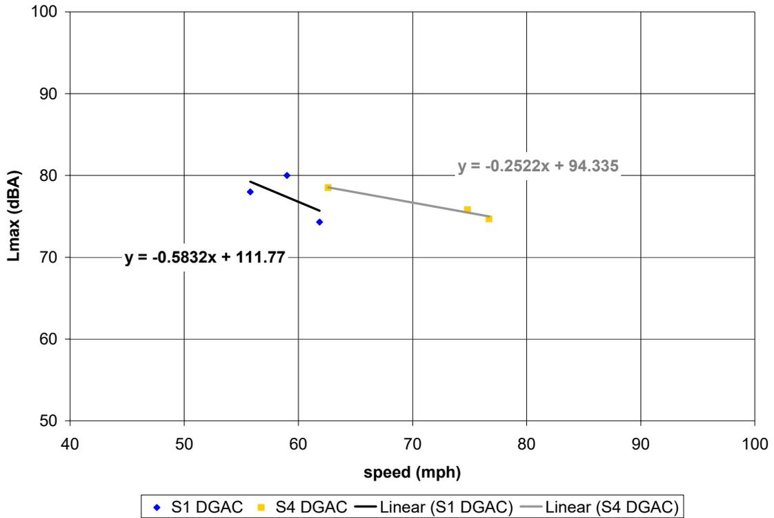
**Figure C-9. (this and previous page) Vehicle pass-by data, pre-overlay; Site 1 (DGAC), Site 4 (DGAC). Automobiles (top), medium trucks (middle), and heavy trucks (bottom). Microphone location: distance 50 ft, height 15 ft.**
