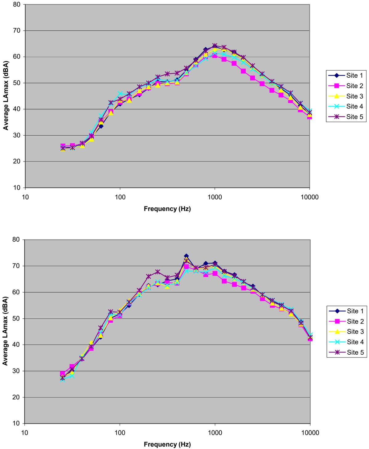
**Figure E-13. Spectral data for automobiles (top) and heavy trucks (bottom) on four different pavement types. Post-overlay results, all pavements aged 16 months. Microphone location: distance 50 ft, height 5 ft.**
