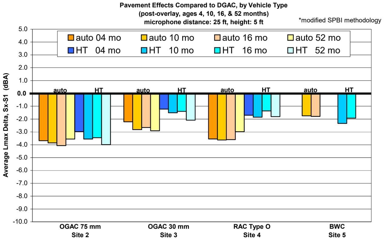
**Figure E-1. Pavement effects compared to DGAC (Site x minus Site 1) for autos and heavy trucks using modified SPBI.\* Post-overlay results, all pavements, including DGAC, aged 4, 10, 16, and 52 months (limited data for BWC). Microphone location: distance 7.5 m (25 ft), height 1.5 m (5 ft).**
