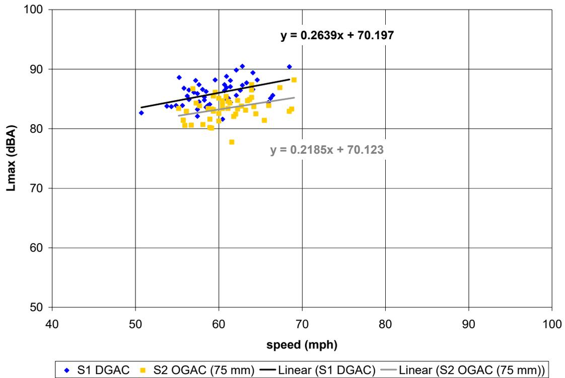
**Figure C-13. (this and previous page) Vehicle pass-by data, post-overlay, 4 months ago; Site 1 (DGAC 30mm), Site 2 (OGAC 75mm). Automobiles (top), medium trucks (middle), and heavy trucks (bottom). Microphone location: distance 25 ft, height 5 ft.**
