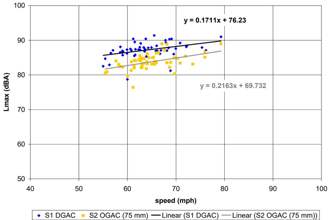
**Figure C-49. (this and previous page) Vehicle pass-by data, post-overlay, 52 months age; Site 1 (DGAC 30mm), Site 2 (OGAC 75mm). Automobiles (top), medium trucks (middle), and heavy trucks (bottom). Microphone location: distance 25 ft, height 5 ft.**
