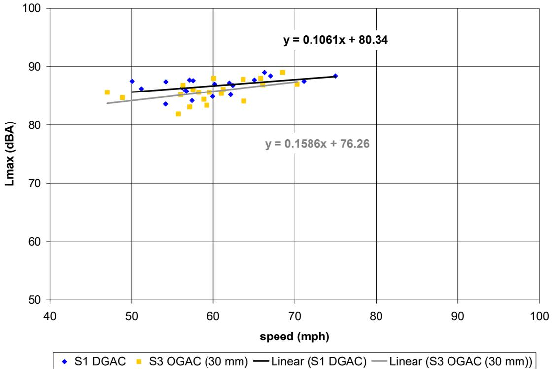
**Figure C-28. (this and previous page) Vehicle pass-by data, post-overlay, 10 months age; Site 1 (DGAC 30mm), Site 3 (OGAC 30mm). Automobiles (top), medium trucks (middle), and heavy trucks (bottom). Microphone location: distance 25 ft, height 5 ft.**
