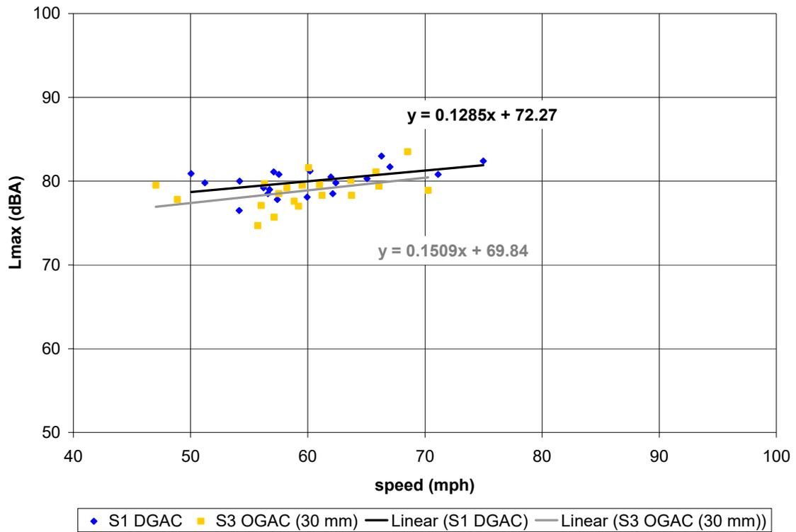
**Figure C-29. (this and previous page) Vehicle pass-by data, post-overlay, 10 months age; Site 1 (DGAC 30mm), Site 3 (OGAC 30mm). Automobiles (top), medium trucks (middle), and heavy trucks (bottom). Microphone location: distance 50 ft, height 5 ft.**
