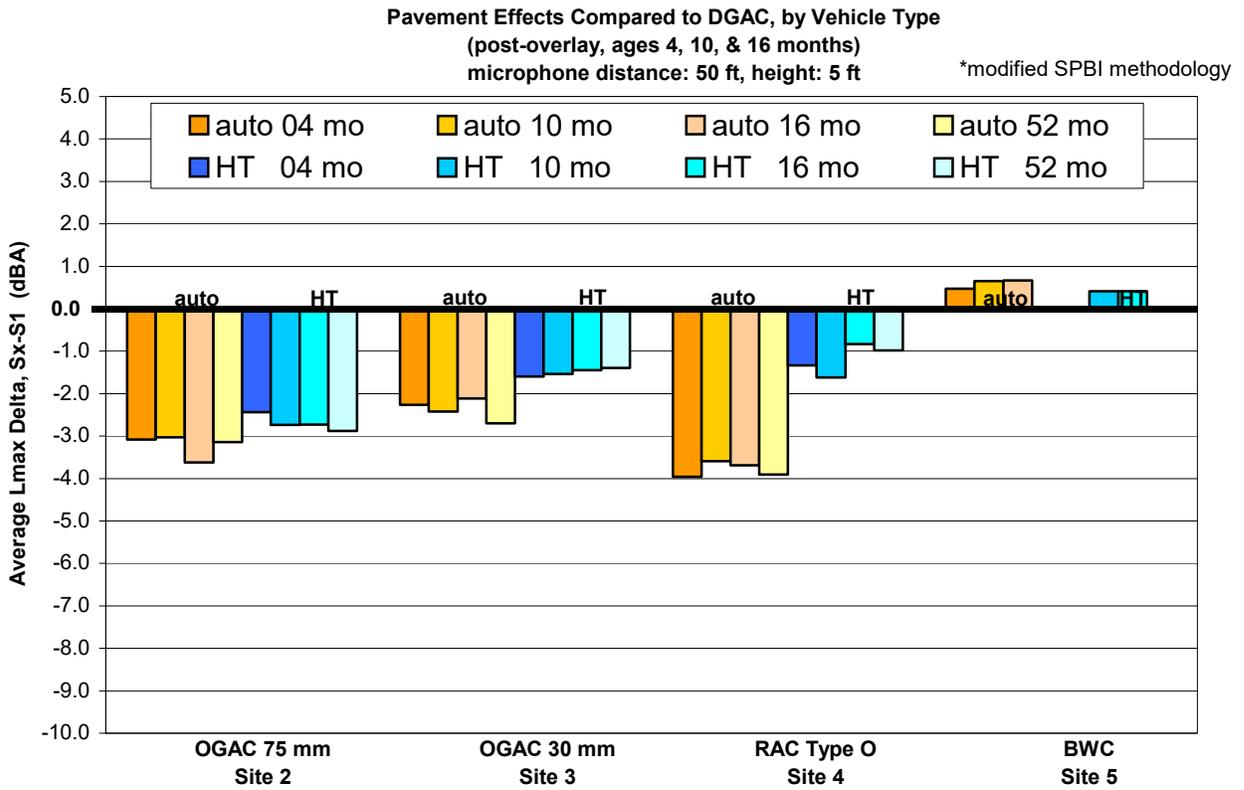
**Figure E-2. Pavement effects compared to DGAC (Site x minus Site 1) for autos and heavy trucks using modified SPBI.\* Post-overlay results, all pavements, including DGAC, aged 4, 10, 16, and 52 months (limited data for BWC). Microphone location: distance 15 m (50 ft), height 1.5 m (5 ft).**
