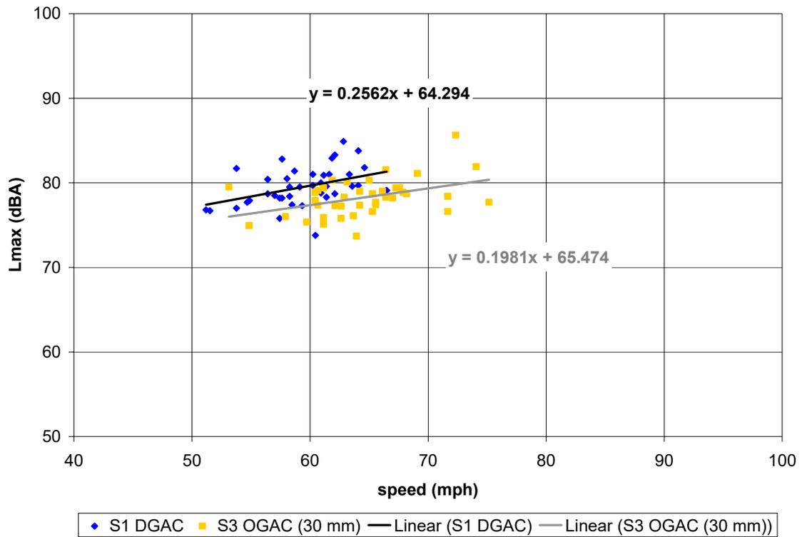
**Figure C-17. (this and previous page) Vehicle pass-by data, post-overlay, 4 months age; Site 1 (DGAC 30mm), Site 3 (OGAC 30mm). Automobiles (top), medium trucks (middle), and heavy trucks (bottom). Microphone location: distance 50 ft, height 5 ft.**
