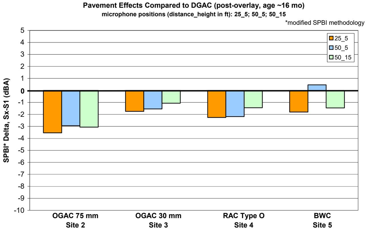
**Figure D-10. Pavement effects compared to DGAC (Site x minus Site 1) using modified SPBI. Post-overlay results, all pavements, including DGAC, aged 16 months. Microphone locations: distance 7.5 m (25 ft), height 1.5 m (5 ft); distance 15 m (50 ft), height 1.5 m (5 ft); distance 15 m (50 ft), height 4.5 m (15 ft).**
