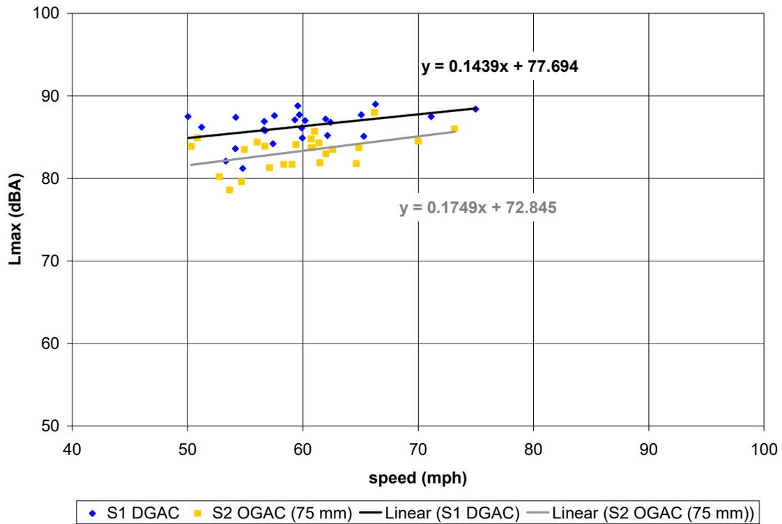
**Figure C-25. (this and previous page) Vehicle pass-by data, post-overlay, 10 months age; Site 1 (DGAC 30mm), Site 2 (OGAC 75mm). Automobiles (top), medium trucks (middle), and heavy trucks (bottom). Microphone location: distance 25 ft, height 5 ft.**
