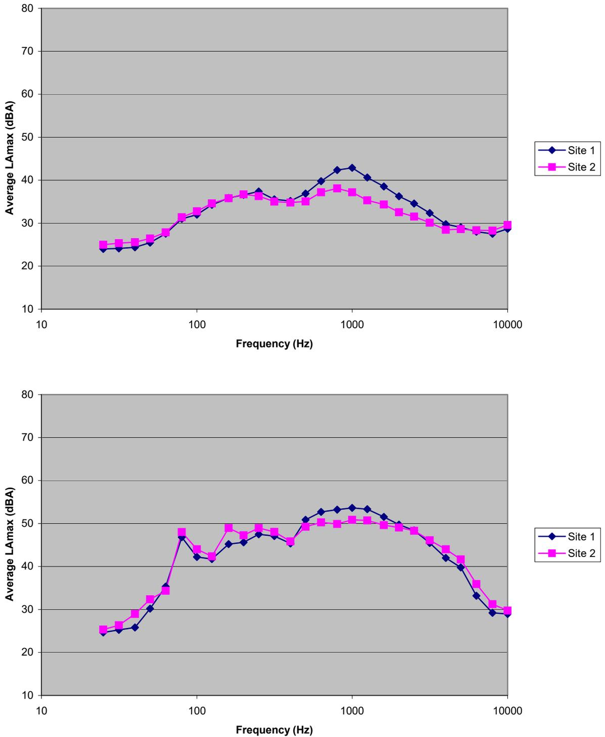
**Figure E-7. Spectral data for automobiles (top) and heavy trucks (bottom) on four different pavement types. Post-overlay results, all pavements aged 4 months. Microphone location: distance 200 ft, height 5 ft.**
