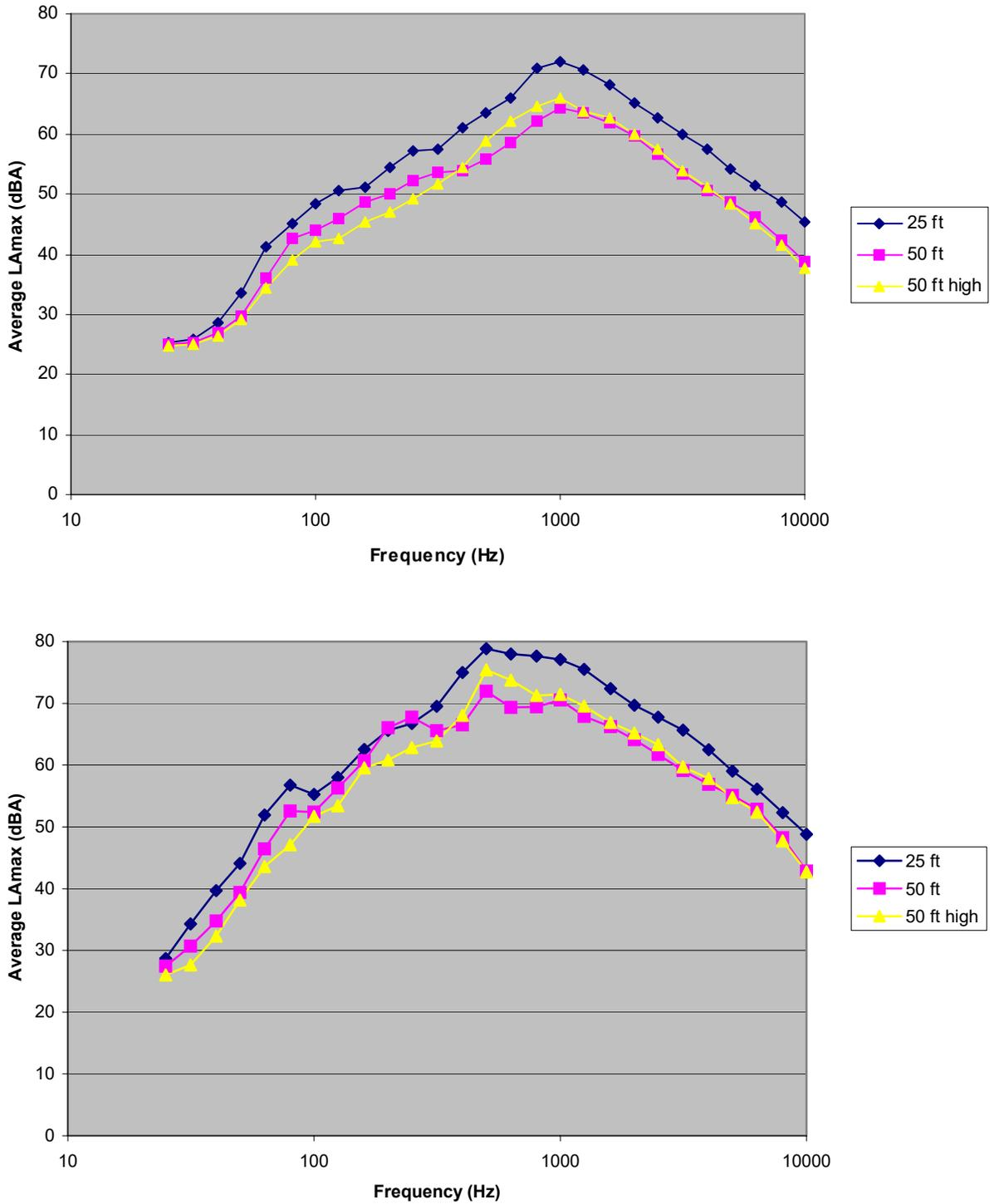
Figure E-28. Spectral data for automobiles (top) and heavy trucks (bottom); post-overlay results for Site 5 (BWC 30 mm) aged 16 months; all microphone positions.
