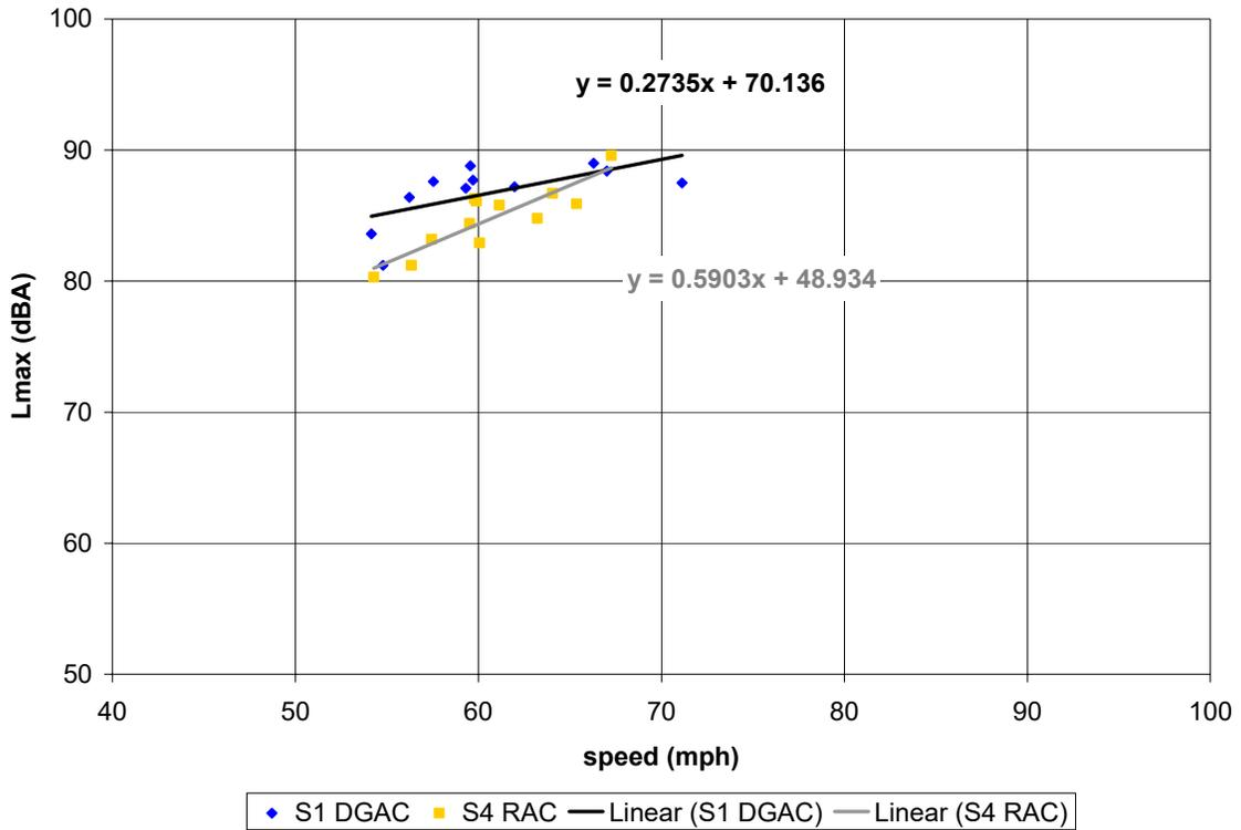
**Figure C-31. (this and previous page) Vehicle pass-by data, post-overlay, 10 months age; Site 1 (DGAC 30mm), Site 4 (RAC Type O 30mm). Automobiles (top), medium trucks (middle), and heavy trucks (bottom). Microphone location: distance 25 ft, height 5 ft.**
