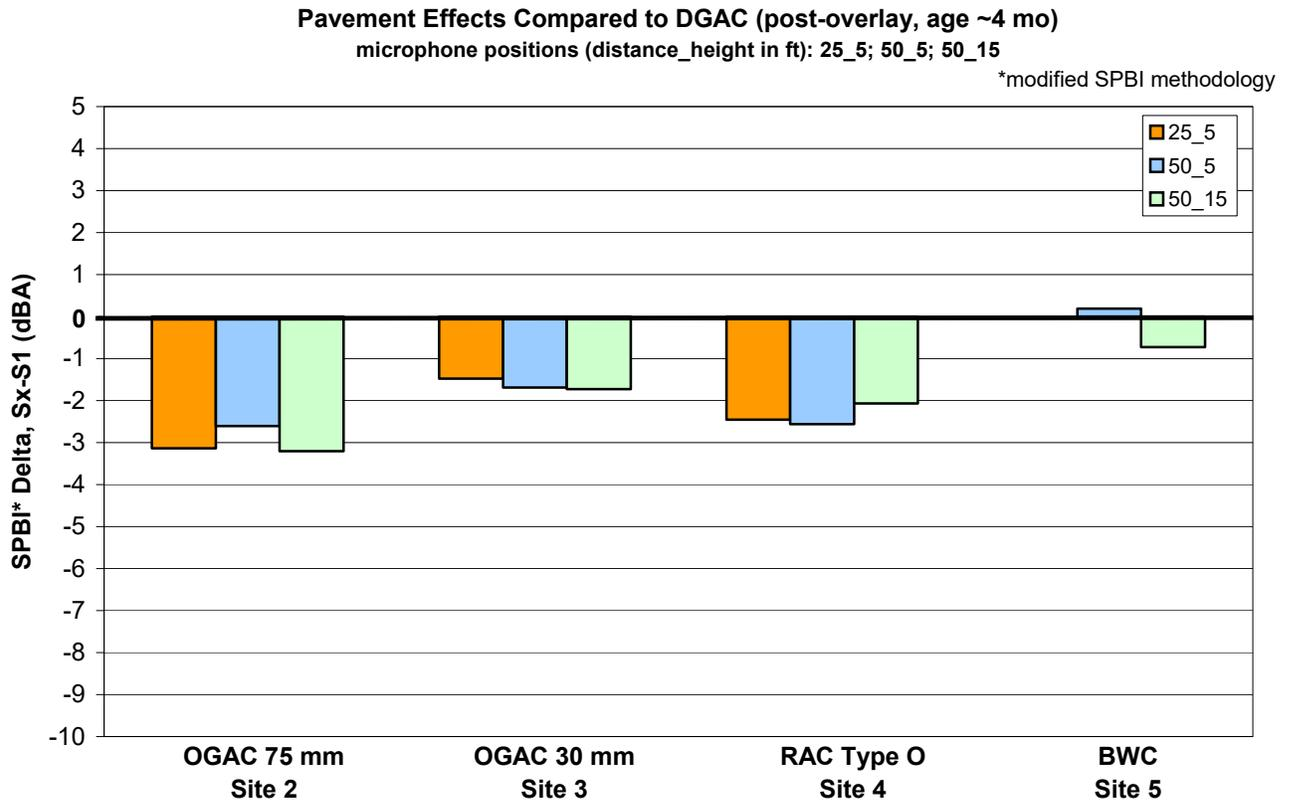
**Figure D-8. Pavement effects compared to DGAC (Site x minus Site 1) using modified SPBI. Post-overlay results, all pavements, including DGAC, aged 4 months. Microphone locations: distance 7.5 m (25 ft), height 1.5 m (5 ft); distance 15 m (50 ft), height 1.5 m (5 ft); distance 15 m (50 ft), height 4.5 m (15 ft).**
