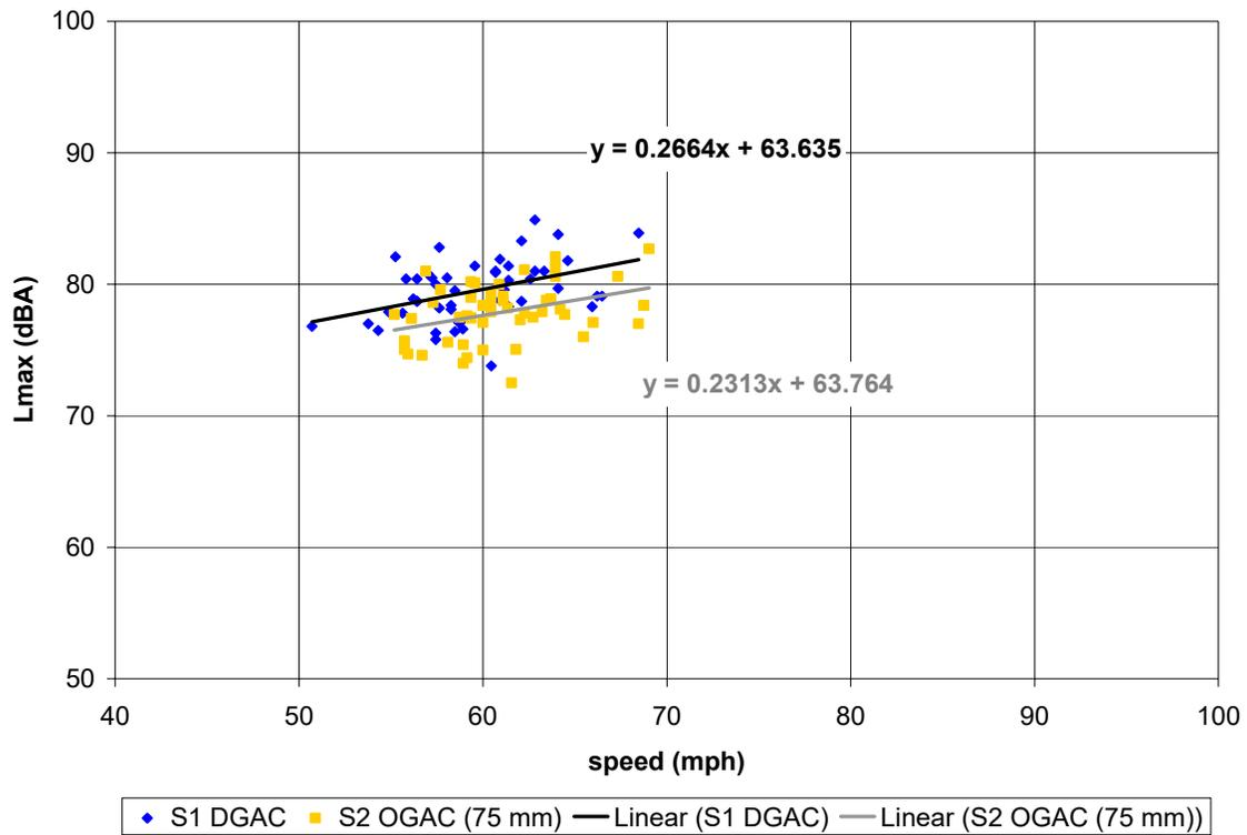
**Figure C-14. (this and previous page) Vehicle pass-by data, post-overlay, 4 months ago; Site 1 (DGAC 30mm), Site 2 (OGAC 75mm). Automobiles (top), medium trucks (middle), and heavy trucks (bottom). Microphone location: distance 50 ft, height 5 ft.**
