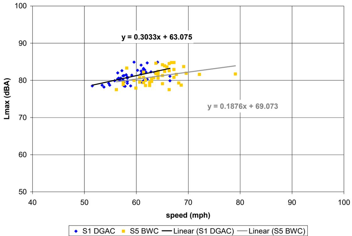
**Figure C-24. (this and previous page) Vehicle pass-by data, post-overlay, 4 months ago; Site 1 (DGAC 30mm), Site 5 (BWC 30mm). Automobiles (top), medium trucks (middle), and heavy trucks (bottom). Microphone location: distance 50 ft, height 15 ft.**
