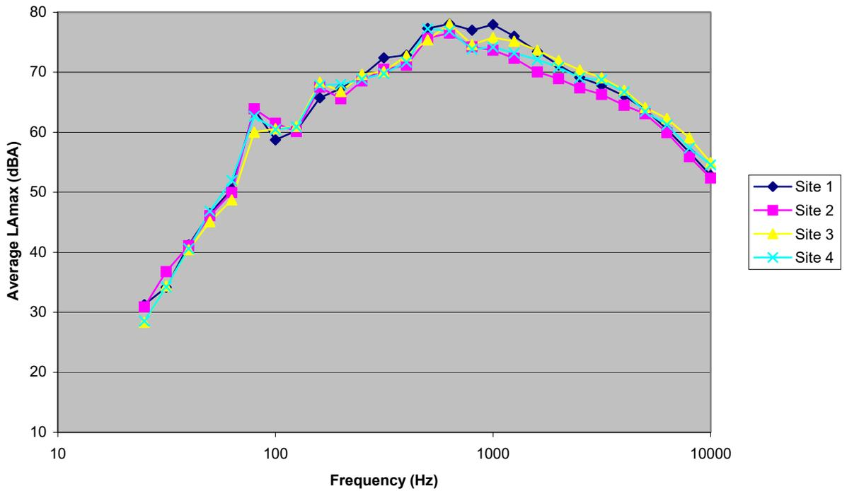
**Figure E-4. Spectral data for automobiles (top) and heavy trucks (bottom) on four different pavement types. Post-overlay results, all pavements aged 4 months. Microphone location: distance 25 ft, height 5 ft.**
