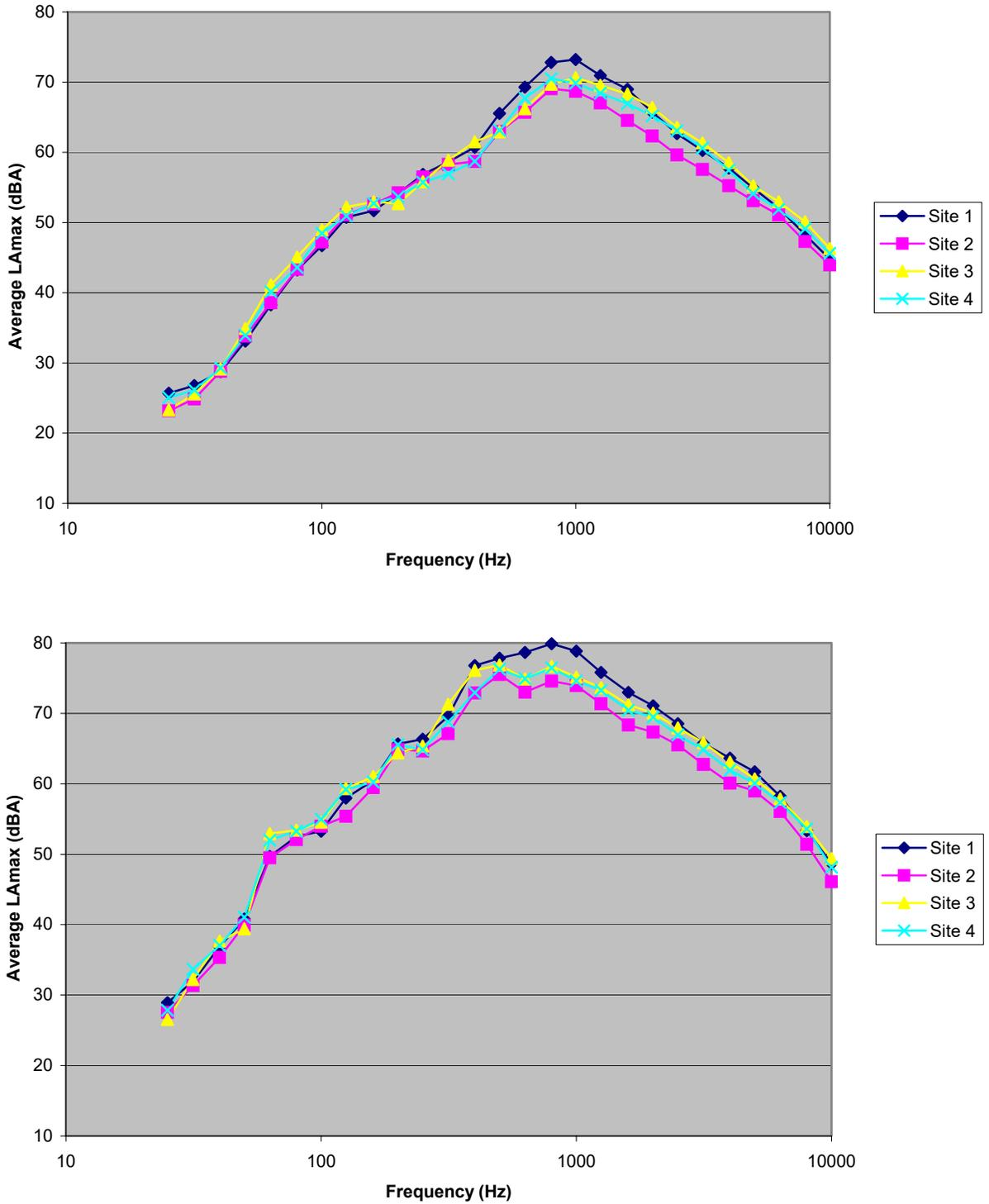
**Figure E-16. Spectral data for automobiles (top) and heavy trucks (bottom) on four different pavement types. Post-overlay results, all pavements aged 52 months. Microphone location: distance 25 ft, height 5 ft.**
