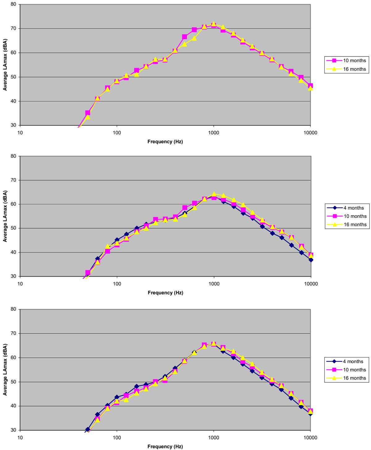
**Figure E-23. Spectral data for automobiles; post-overlay results for Site 5 (BWC 30 mm); all ages measured. Microphone location: distance 25 ft, height 5 ft (top); microphone location: distance 50 ft, height 5 ft (middle); microphone location: distance 50 ft, height 15 ft (bottom).**
