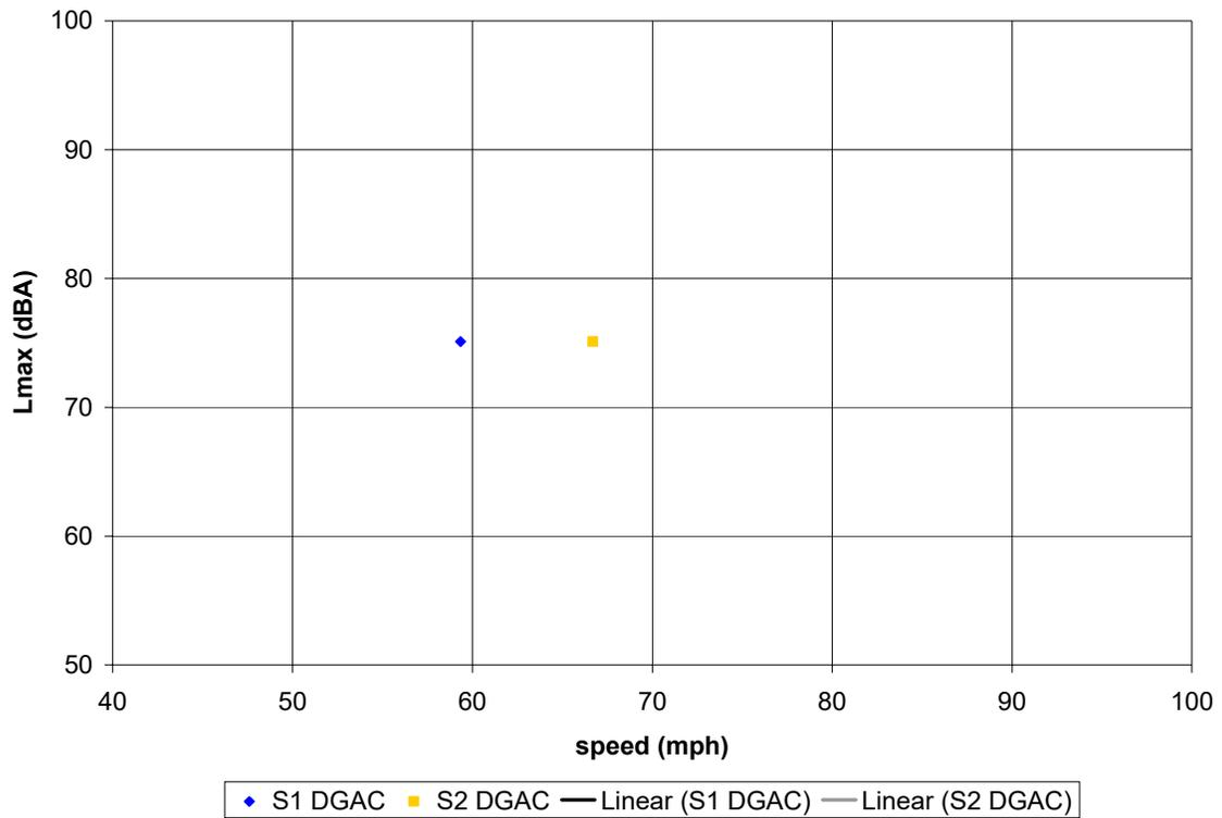
**Figure C-3. (this and previous page) Vehicle pass-by data, pre-overlay; Site 1 (DGAC), Site 2 (DGAC). Automobiles (top), medium trucks (middle), and heavy trucks (bottom). Microphone location: distance 50 ft, height 15 ft.**
