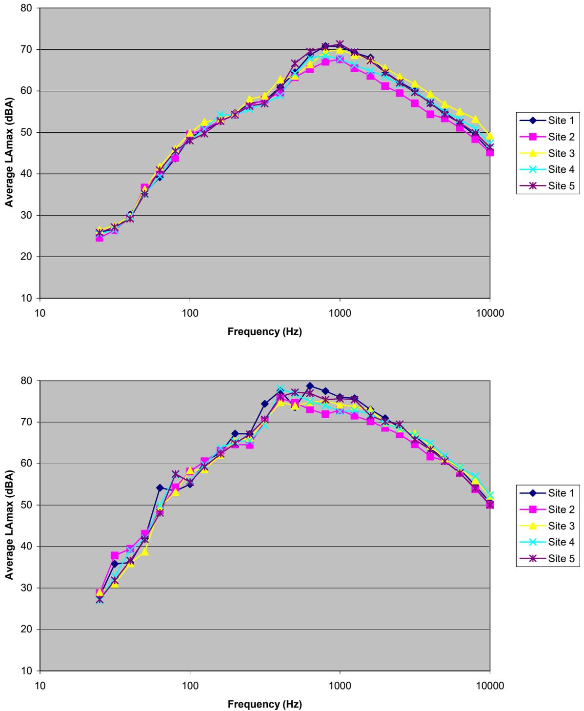
**Figure E-8. Spectral data for automobiles (top) and heavy trucks (bottom) on four different pavement types. Post-overlay results, all pavements aged 10 months. Microphone location: distance 25 ft, height 5 ft.**
