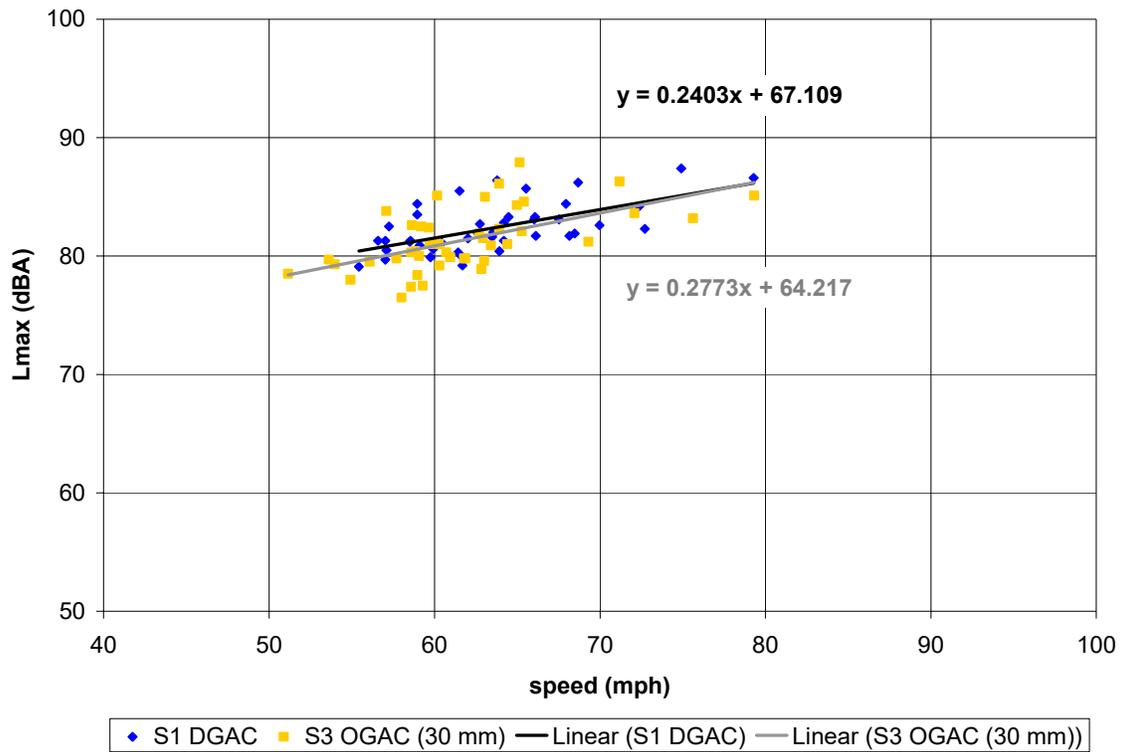
**Figure C-54. (this and previous page) Vehicle pass-by data, post-overlay, 52 months age; Site 1 (DGAC 30mm), Site 3 (OGAC 30mm). Automobiles (top), medium trucks (middle), and heavy trucks (bottom). Microphone location: distance 50 ft, height 15 ft.**
