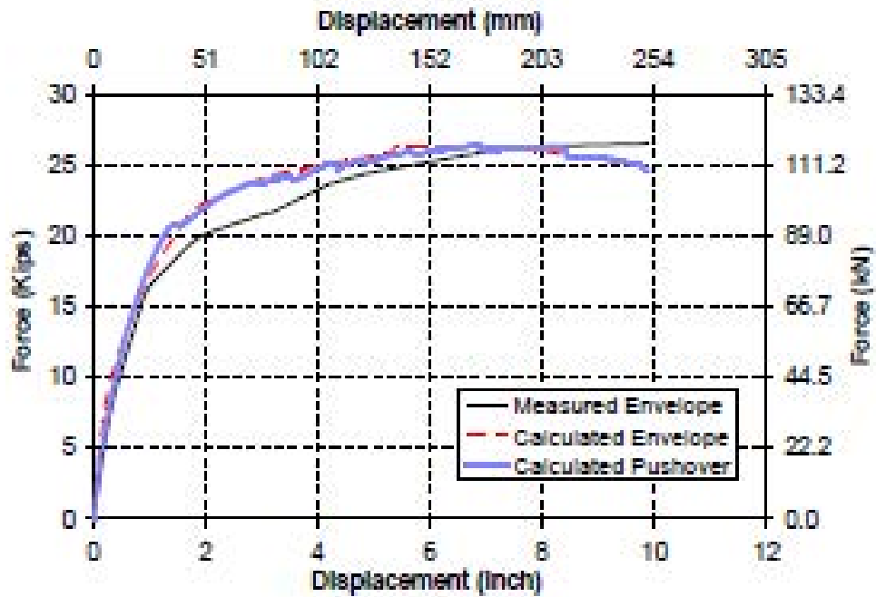
Fig. 6-10. Pushover and Average Backbone Curves of SBR-1
