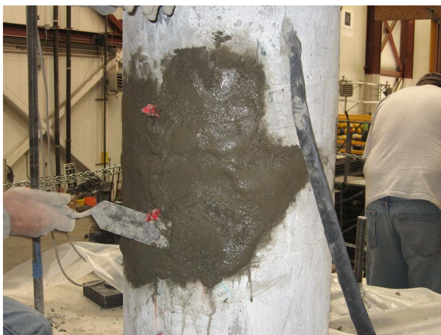
Fig. 2-53. Patching SC-2R with High Strength Grout
