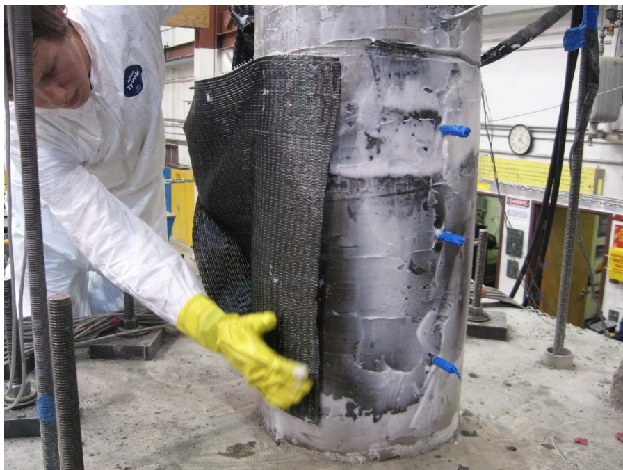
Fig. 2-54. FRP Wrapping for Column SC-2R
