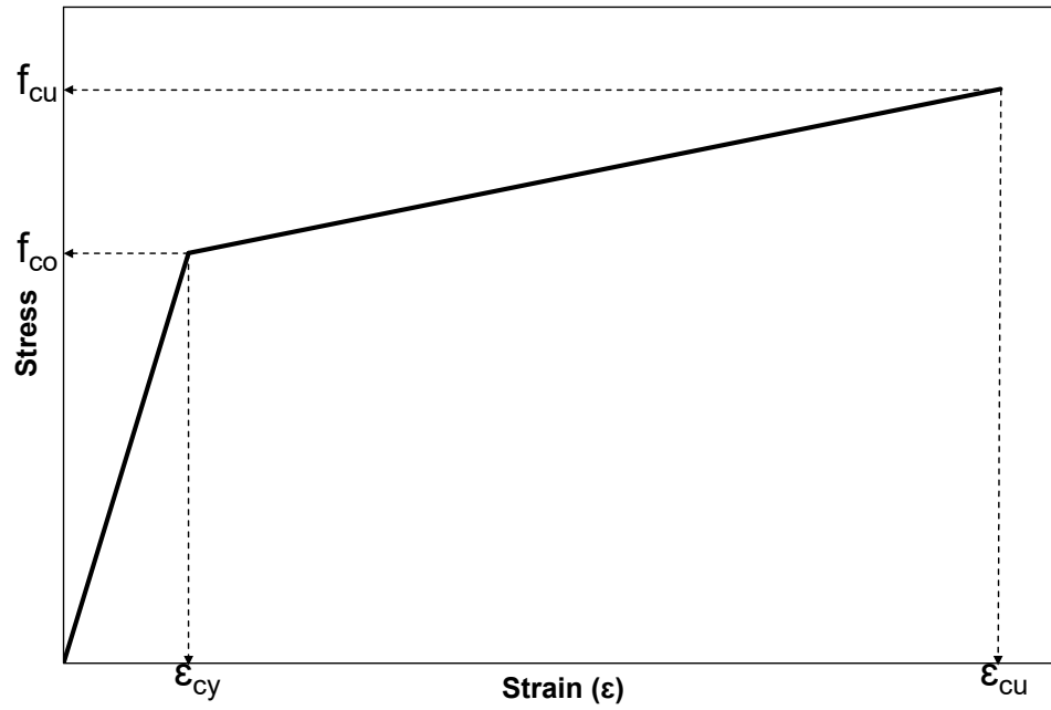
Fig. 2-34. Stress-Strain Bilinear Model for Concrete Confined with FRP
