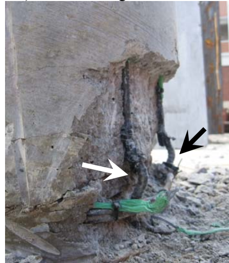
d) Two Buuckled bars, South, Run 6
