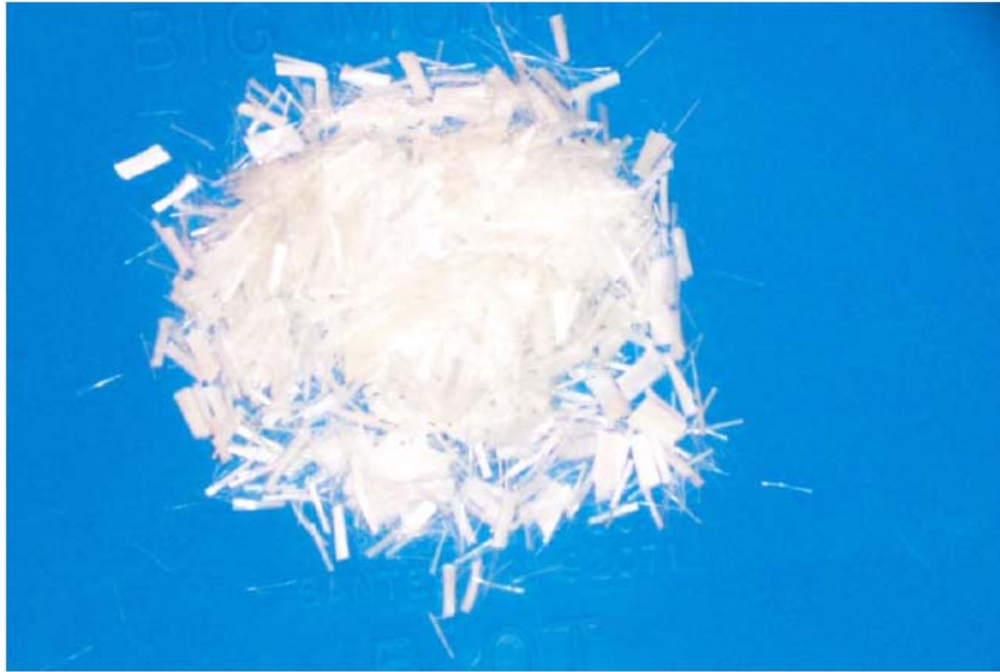
Fig. 1-10. PVA Fibers in ECC Material [Wang and Saiidi, 2005]
