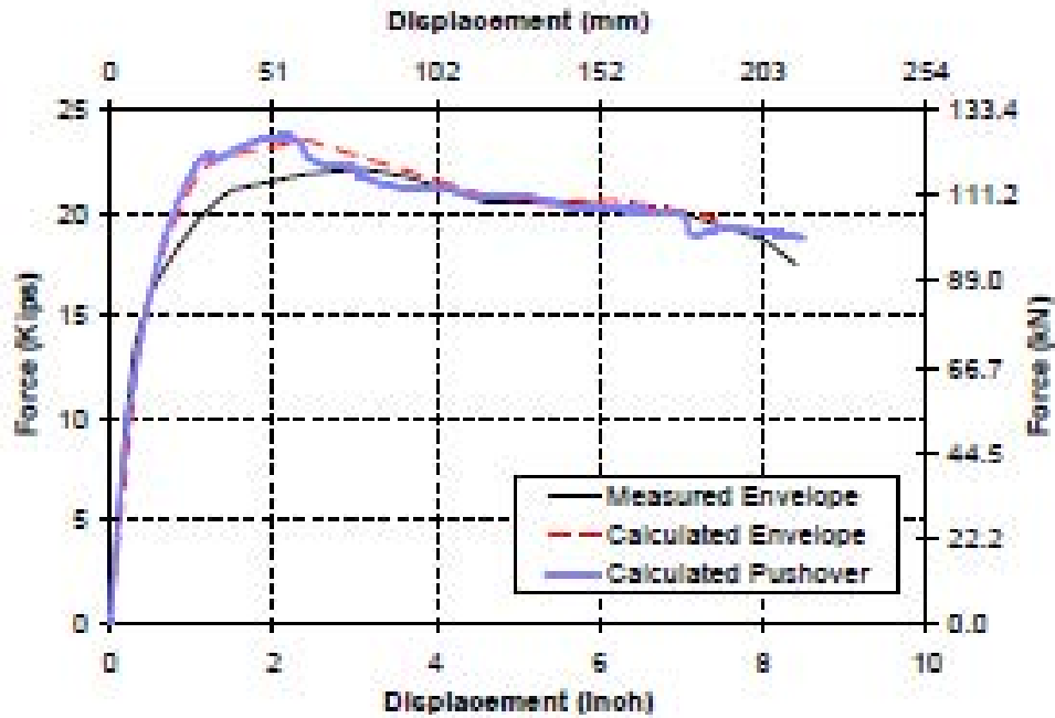
Fig. 6-9. Pushover and Average Backbone Curves of SC-2
