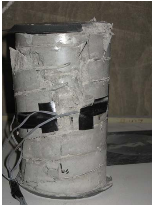
Fig. 5-9. ECC Cylinders after Test
