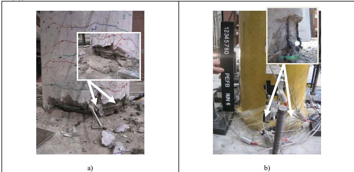
Fig. 9- Apparent Damage at Failure Point in a) RC-ECC Column, b) FRP Column
