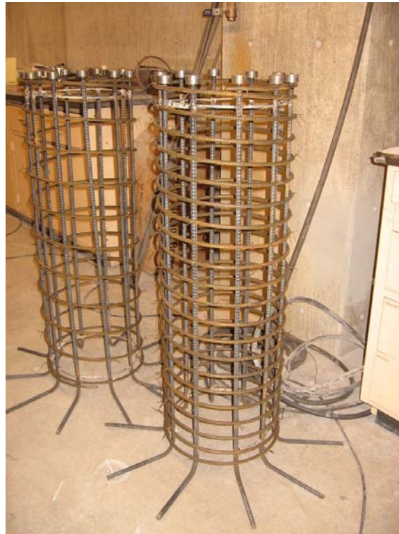
Fig. 2-16. Base Segment Steel Cage
