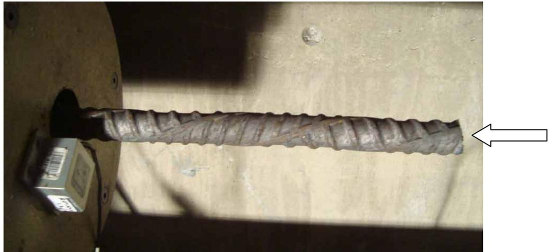
Figure 3.42: Fracture of #6 Bar under Torsional Loading
