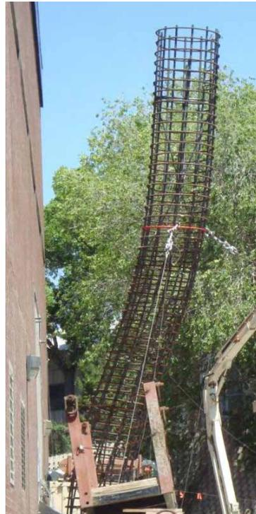
**Figure 3.70: Specimen I deformed shape, view from South**
