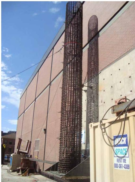
**Figure 3.51: Specimen II standing without any Temporary Support**
