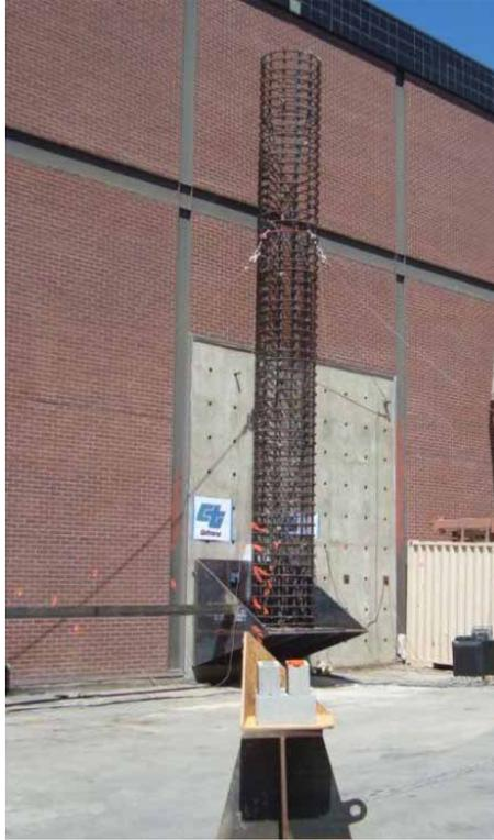
**Figure 3.50: Specimen I standing without any Temporary Support**
