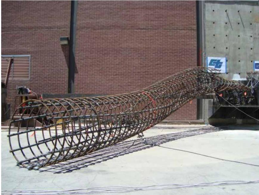
**Figure 3.67: Collapse of Specimen I**
