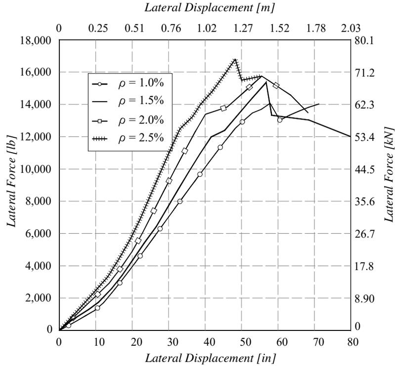
Figure AII.24: Response of Rebar Cage Models with #11 Braces, Height = 40-ft and Diameter = 8-ft
