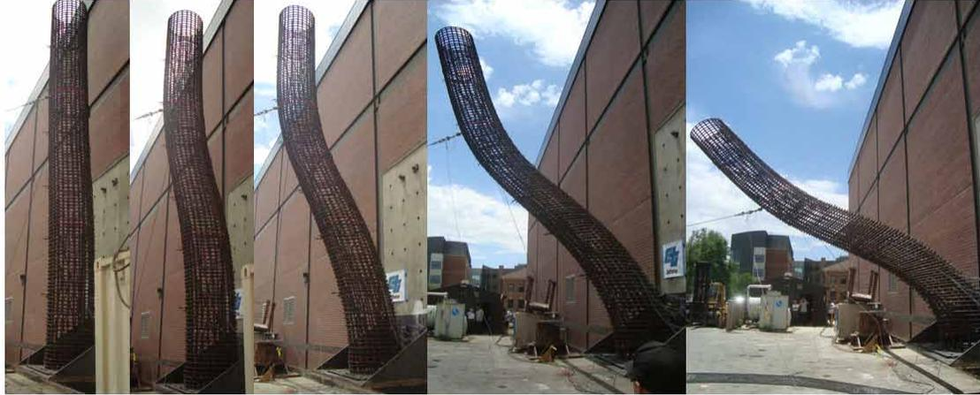
**Figure 3.89: Sequence of deformed shapes for Specimen II, view from North**
