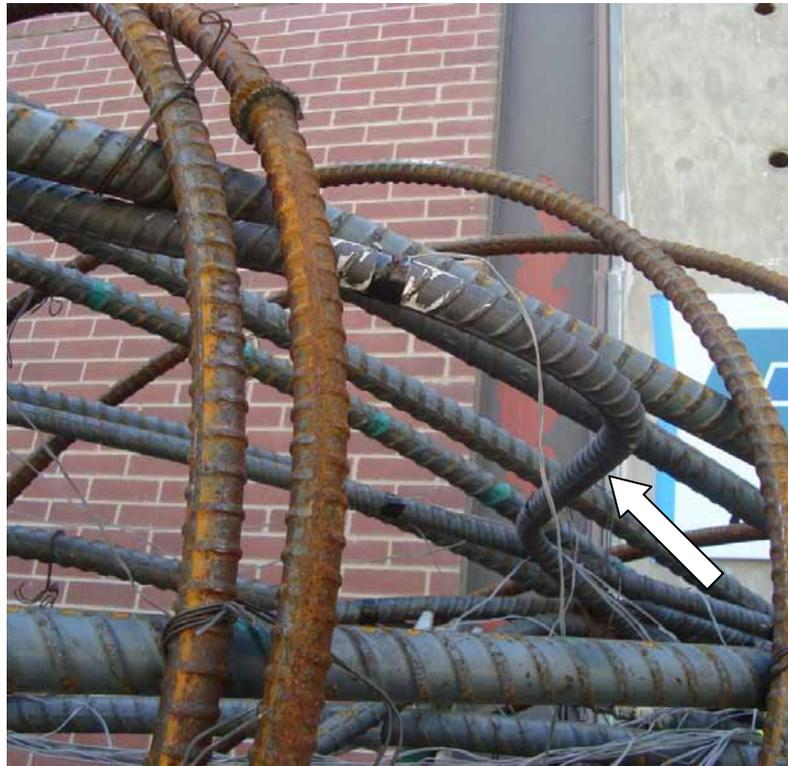
**Figure 3.82: Close up of buckled brace bar after collapse of Specimen I**
