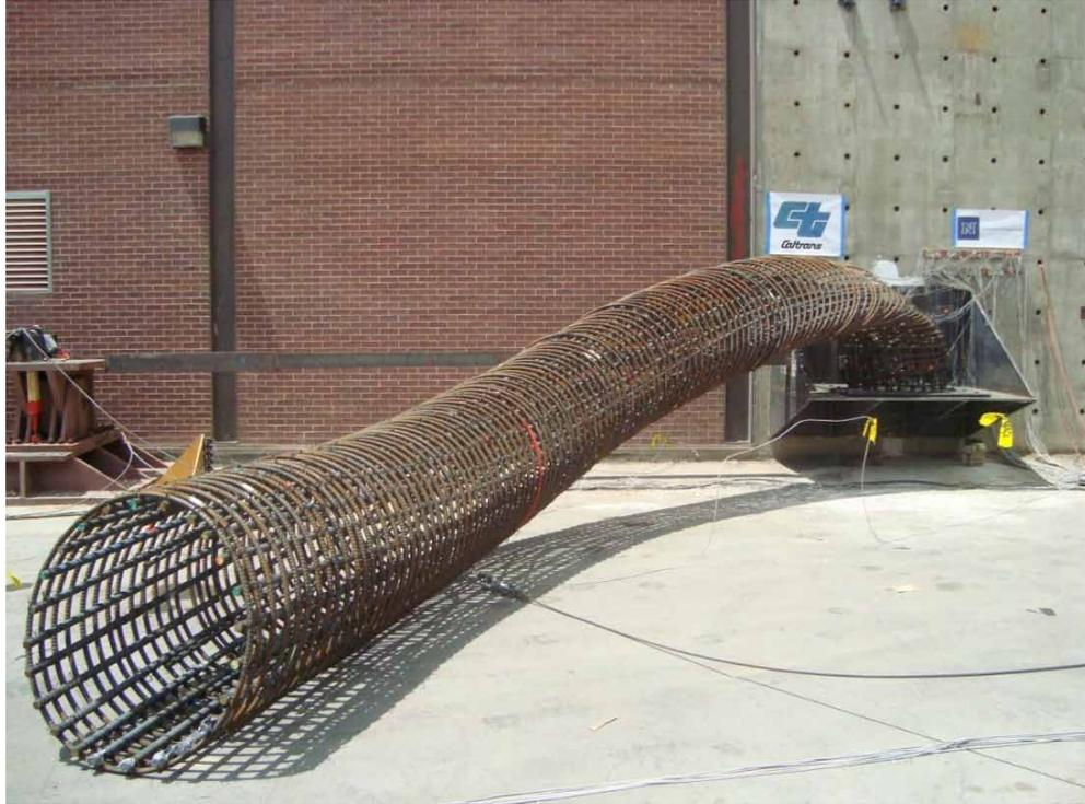
Figure 3.87: Collapse of Specimen II
