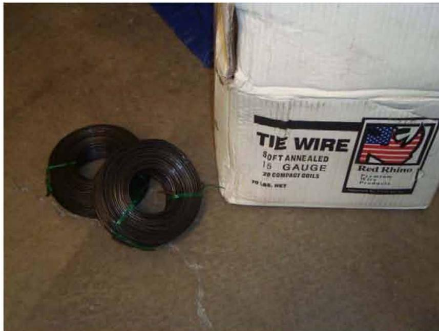
Figure 2.5: No. 15 gauge Tie Wire Coils
