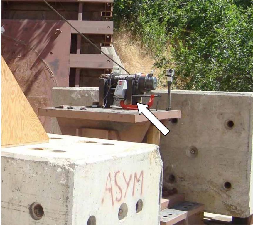
**Figure 3.58: Winch and Displacement Transducer box located to the west of the Rebar Cage**
