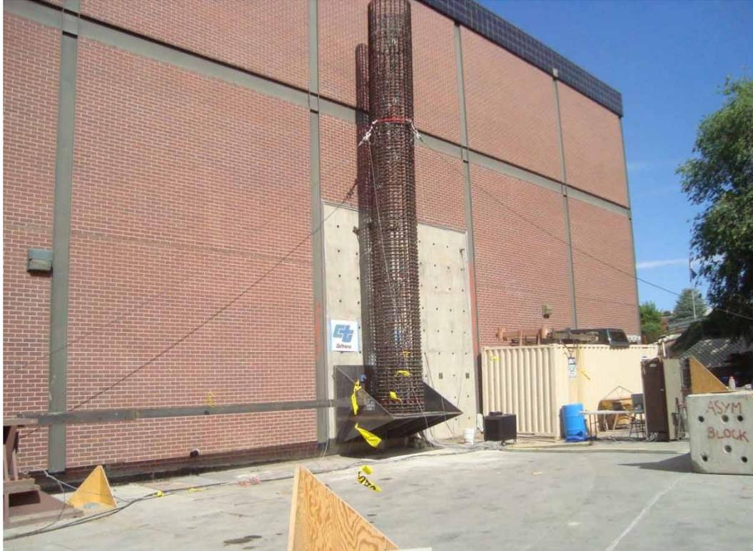
**Figure 3.60: Specimen II Test Set-Up**
