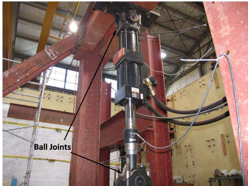
*Figure 2.4: MTS 55-kip Hydraulic Actuator*
