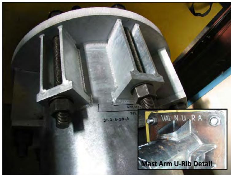
Figure 1.2: U Rib Stiffener and Stool Base Details
