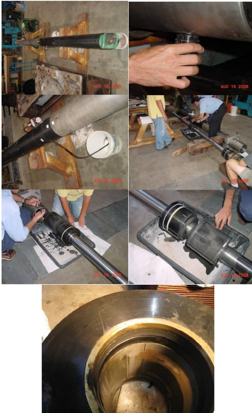
Figure 1.5 Photos of VTB Damper Disassembly and Internal Damage (Graziotti 2010)
