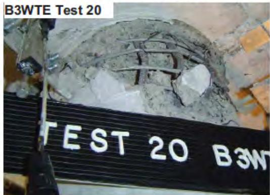
Figure 2-6 Damage progression @ Bent-3 (Top of west column)
