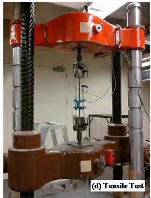
Figure 3-13: Testing longitudinal and transverse reinforcing bars (sample results and setup)
