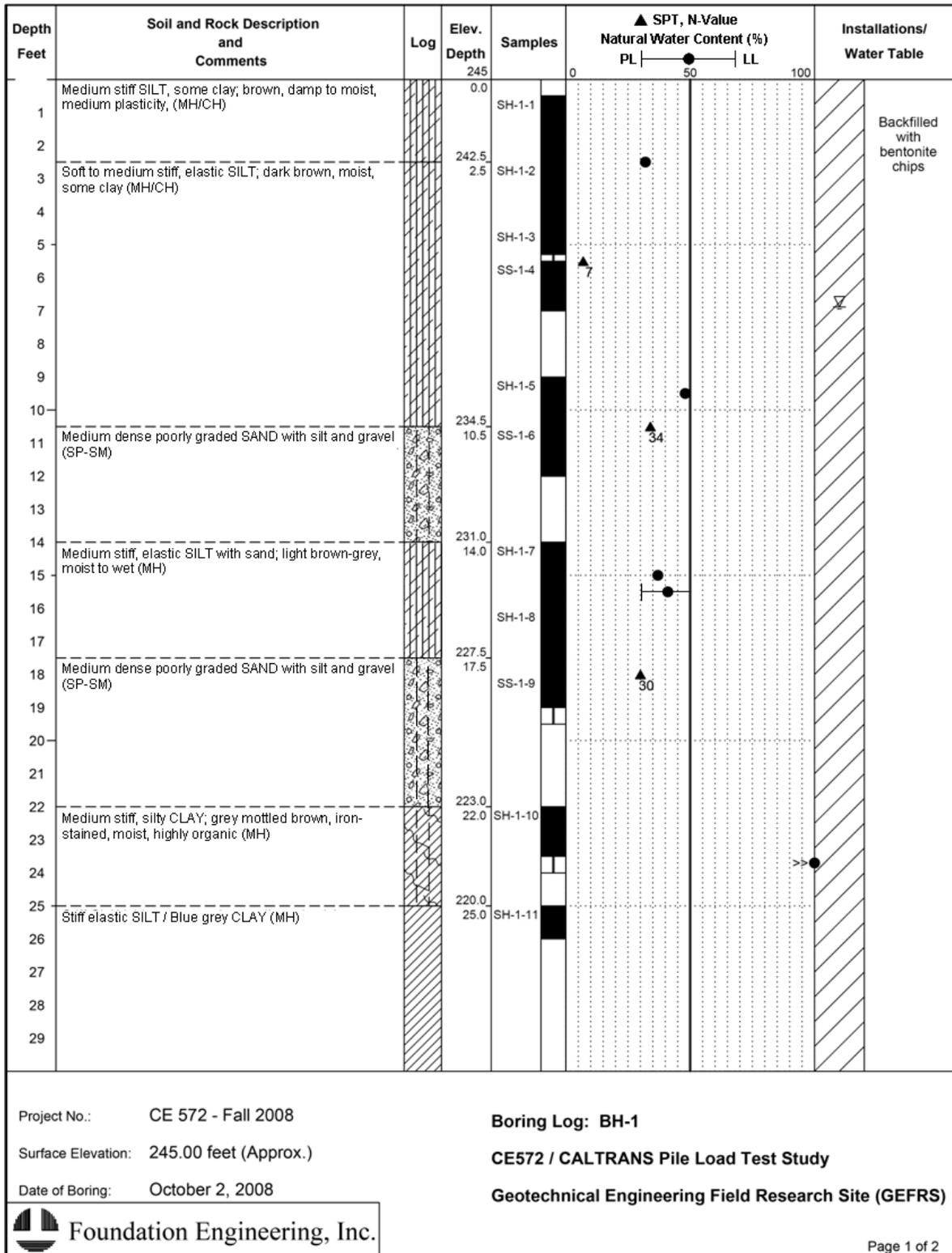
Figure A-3. Soil Boring Log, B-10
