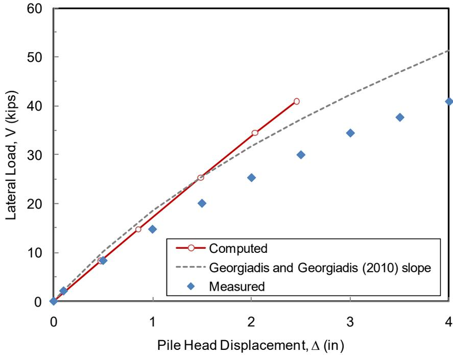
**Figure 9-9** Comparison of Load-Displacement Curve from Test Results and FEM Analysis for the OD Pile
