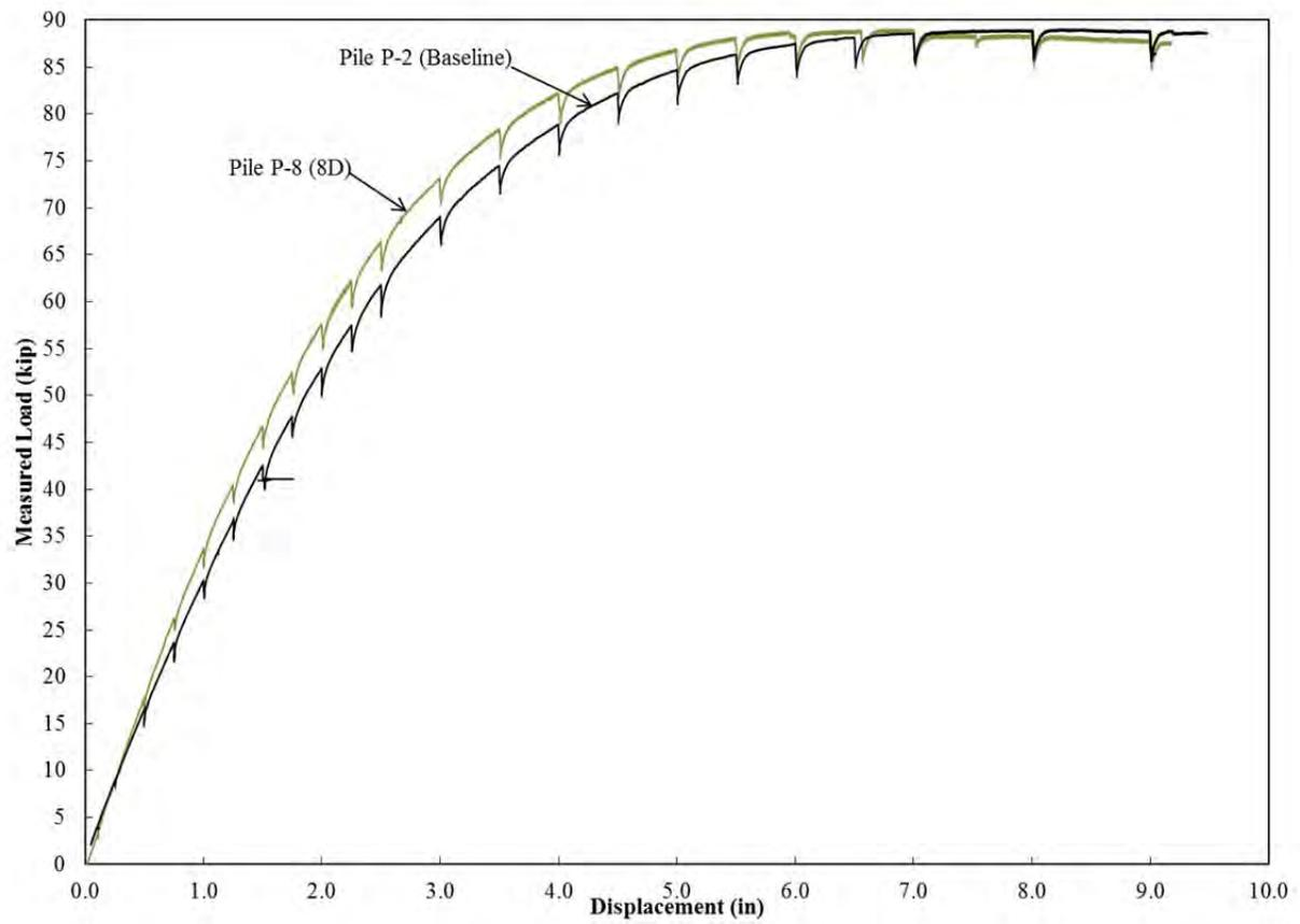
**Figure 11-1** Comparison of Load-Displacement Curves between the Baseline Pile (P-2) and the 8D Pile (P-6)
