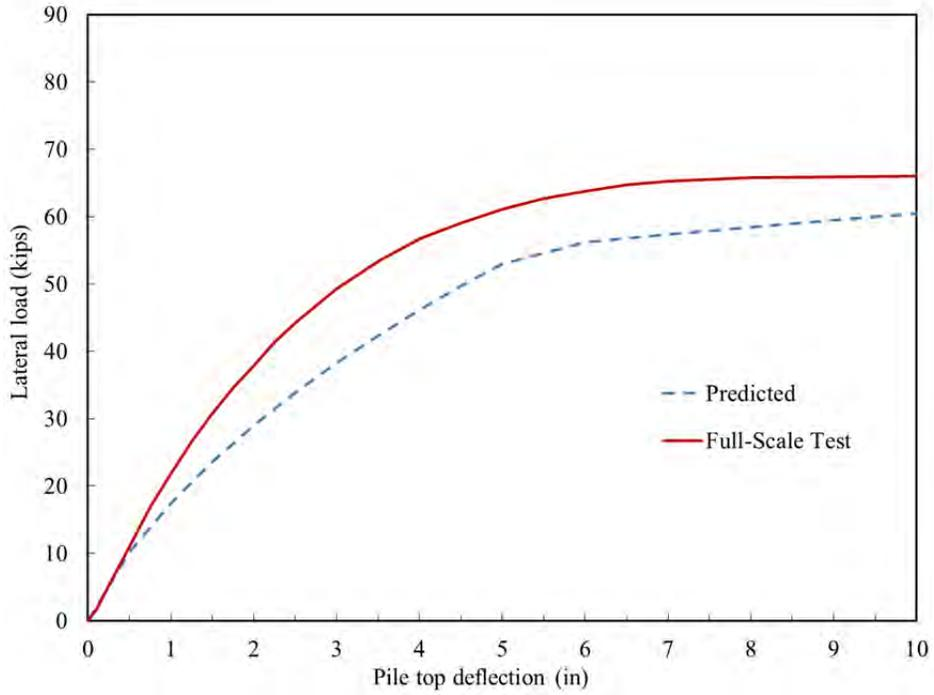
Figure 13-9 LPILE predicted 0D (slope crest) load-displacement curve with the full-scale test results
