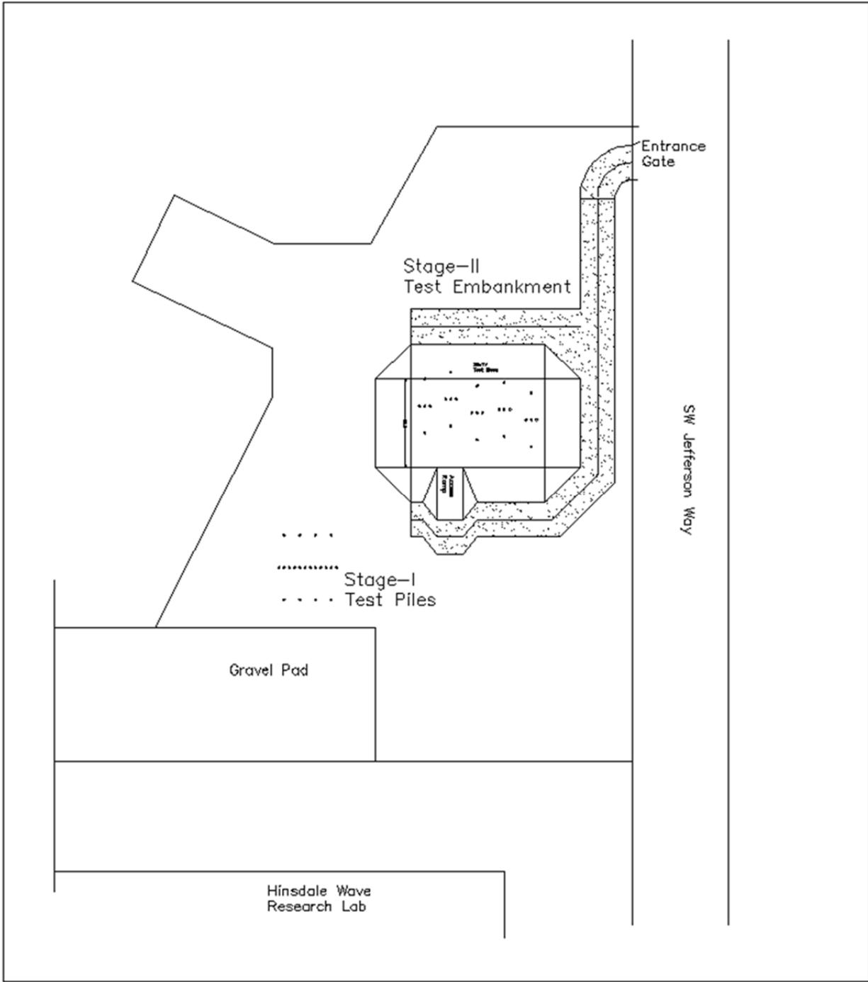
**Figure 3-5.** Series-II Lateral Load Testing Layout on the Caltrans Test Site
