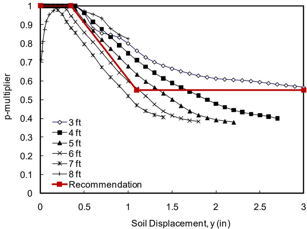
Figure 7-21. Direct Comparison of p-Multiplier at Different Depths for 2D Pile (I-4)
