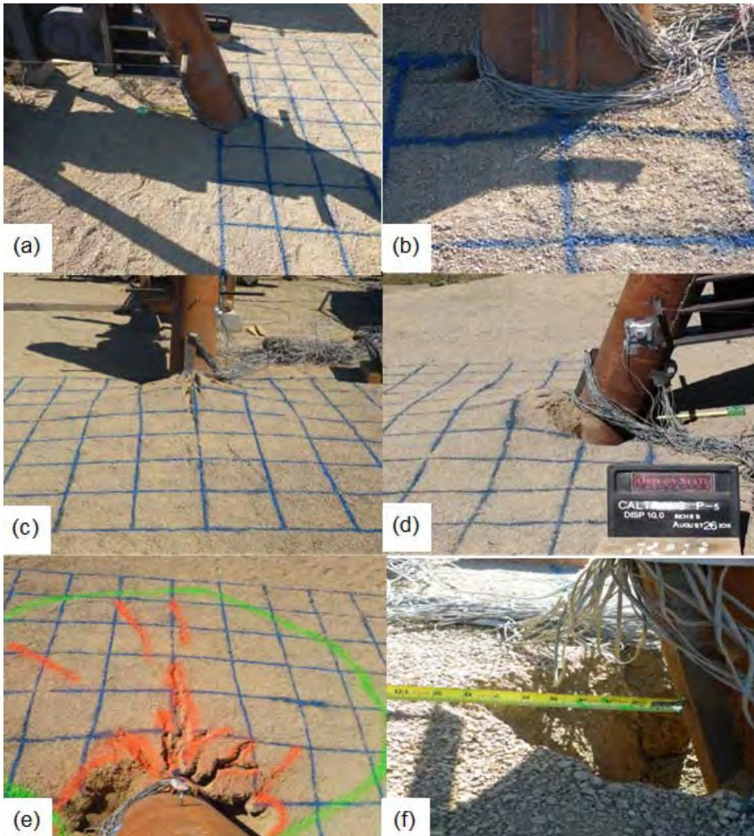
**Figure 10-9** Observations during Lateral Loading Testing of Pile P-5 (+26 Batter) a) Pile before loading b) Front of pile before testing c) Soil heave and cracking at end of testing d) Soil heave at end of testing e) Extensive cracking f) Gap formation behind pile
