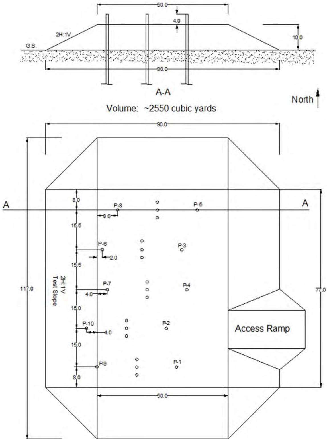
Figure 4-17. Plan and Cross-Sectional Views of the Series-II Cohesionless Embankment
