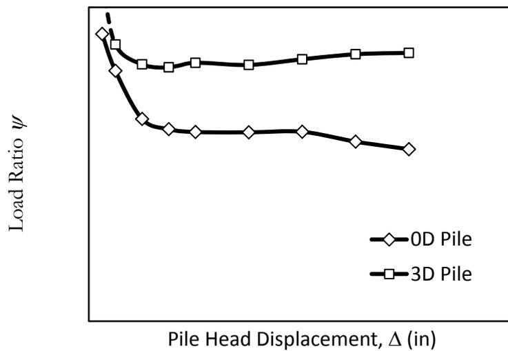
**Figure 2-24** Load Ratio for Piles Near Sand Slope (after Mirzoyan 2004)
