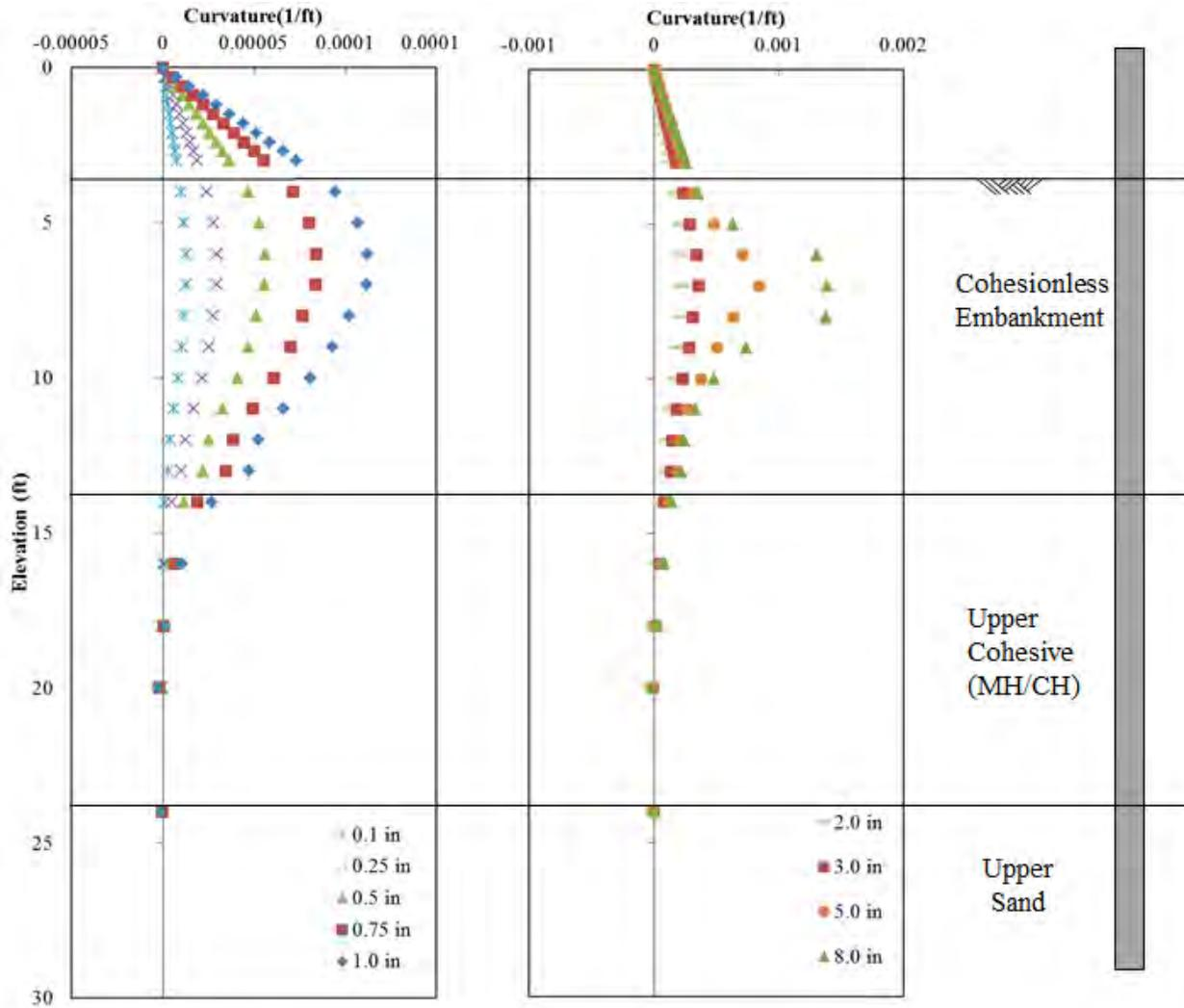
**Figure 11-9** Curvature Results for the 2D Pile (P-6) at varying Displacements
