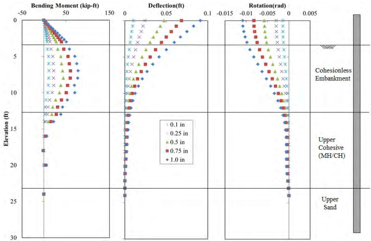
**Figure 12-19** Comparison of Test Results and Analysis Using Back-Calculated  $p$ - $y$  Curves for the -4D (P-10) for Pile Head Displacement of 0.1, 0.25, 0.5 and 1.0 in.
