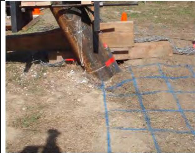
a) Initial condition before 1<sup>st</sup> battered pile test
