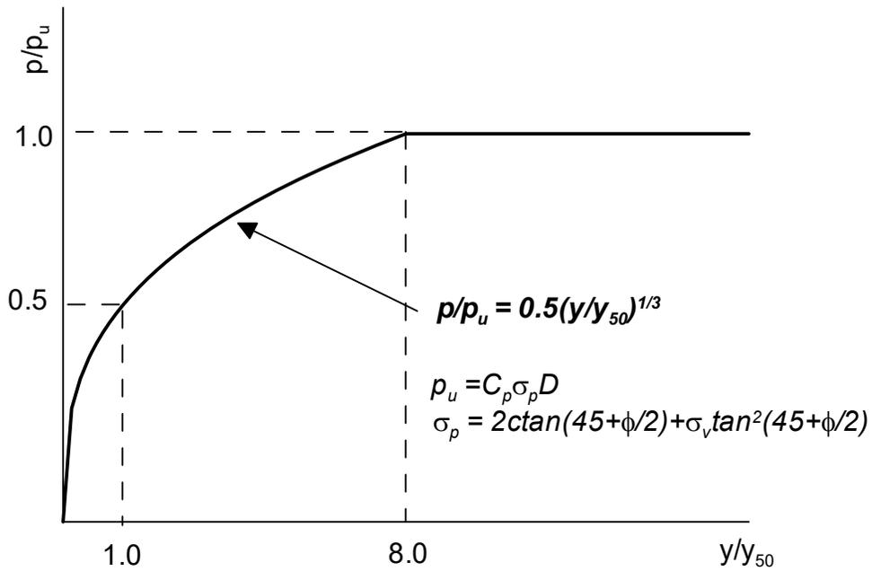
**Figure 2-17** Characteristic Shape of  $p$ - $y$  Curve for Cemented Sand (after Ismael 1990)
