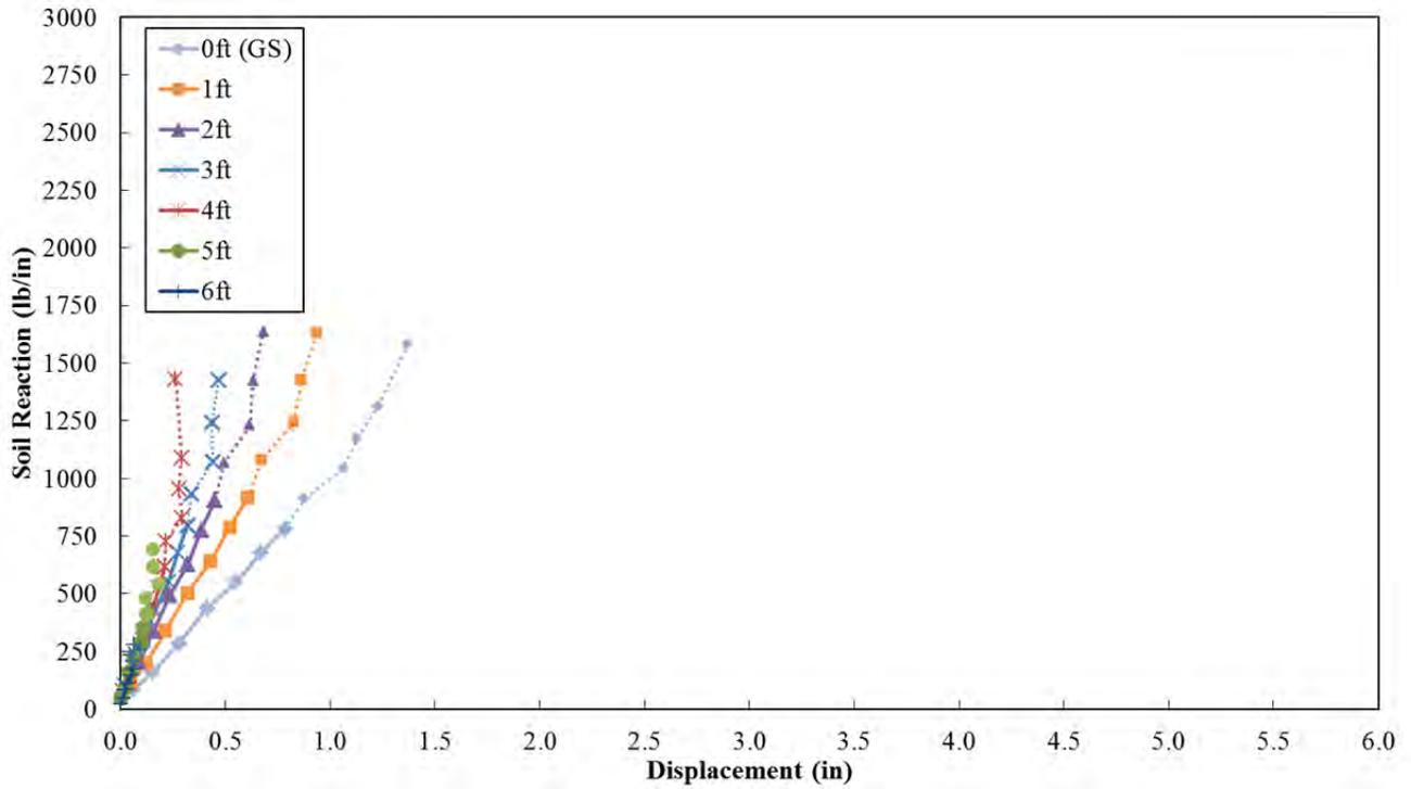
**Figure 12-5** Back-Calculated  $p$ - $y$  Curves for the 4D Pile (P-7)
