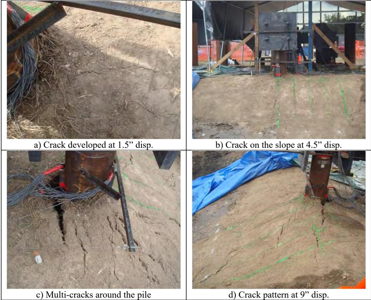
**Figure 5-5.** Observations from Lateral Load Test for 0D Pile (I-7)
