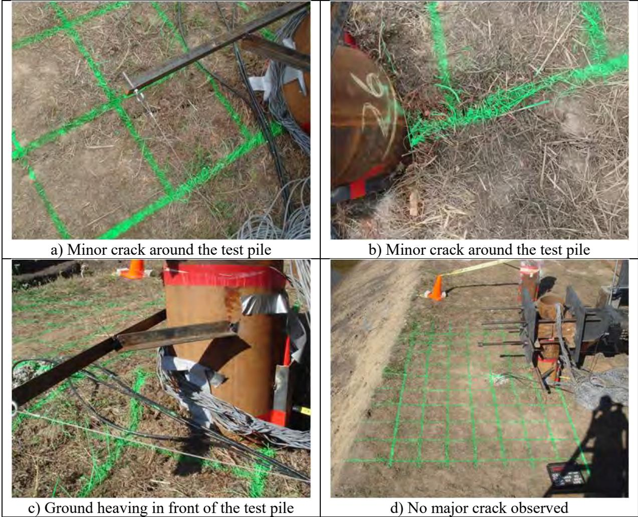
**Figure 5-4.** Observations from Lateral Load Test for 8D Pile (I-6)
