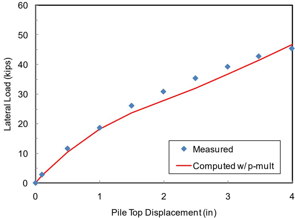
**Figure 7-24.** Comparison of Load-Displacement Curves from Test Results and Analysis Using Proposed Recommendation for 2D Pile (I-4)
