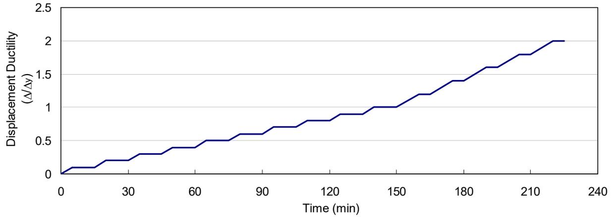
**Figure 4-15.** Load Protocol for Pseudo Static Lateral Load Tests
