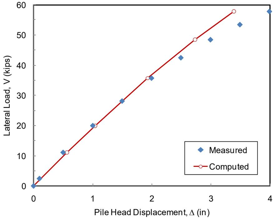
**Figure 9-7** Comparison of Load-Displacement Curve from Test Results and FEM Analysis for the Baseline Pile
