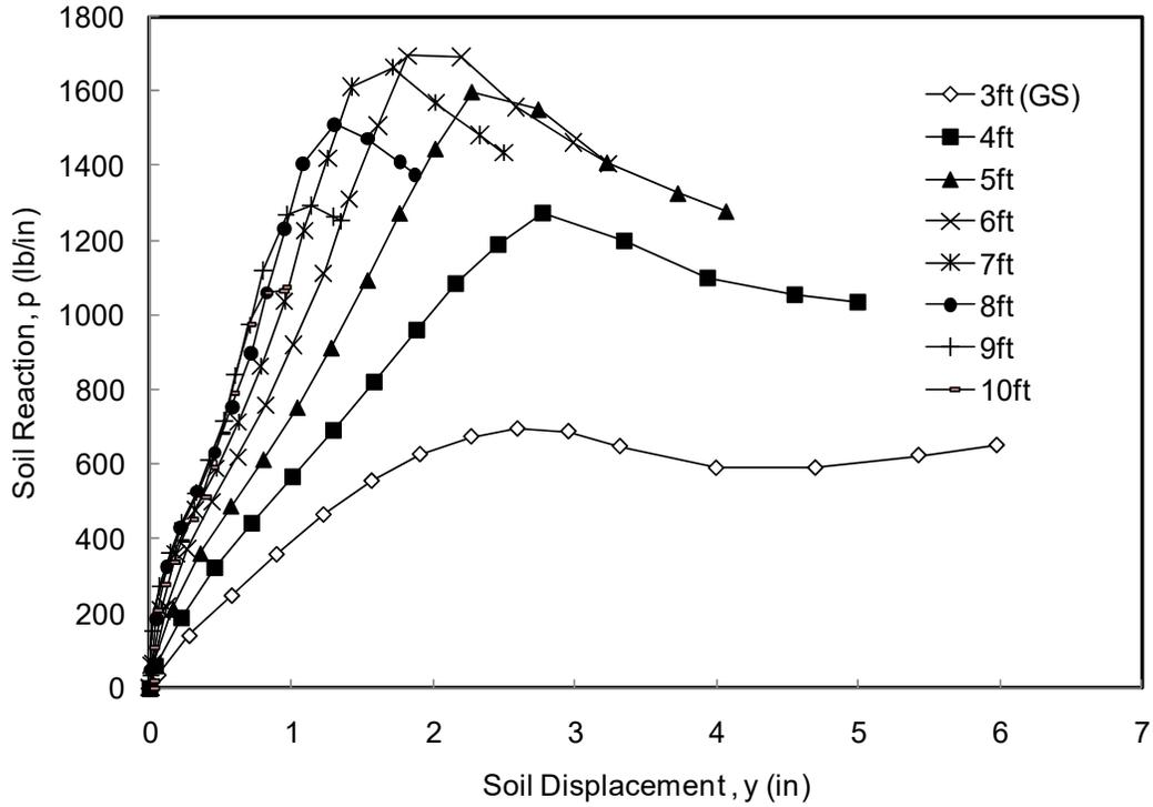
**Figure 7-2.** Back-Calculated  $p$ - $y$  Curves for 8D Pile (I-6) (8D from crest)
