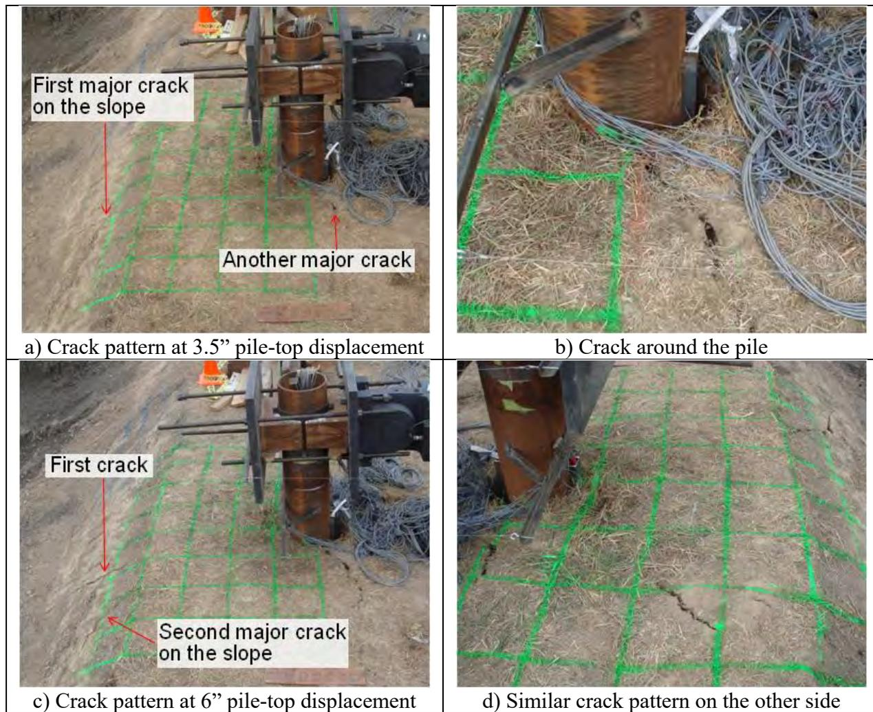
**Figure 5-3.** Observations from Lateral Load Test for 4D Pile (I-5)
