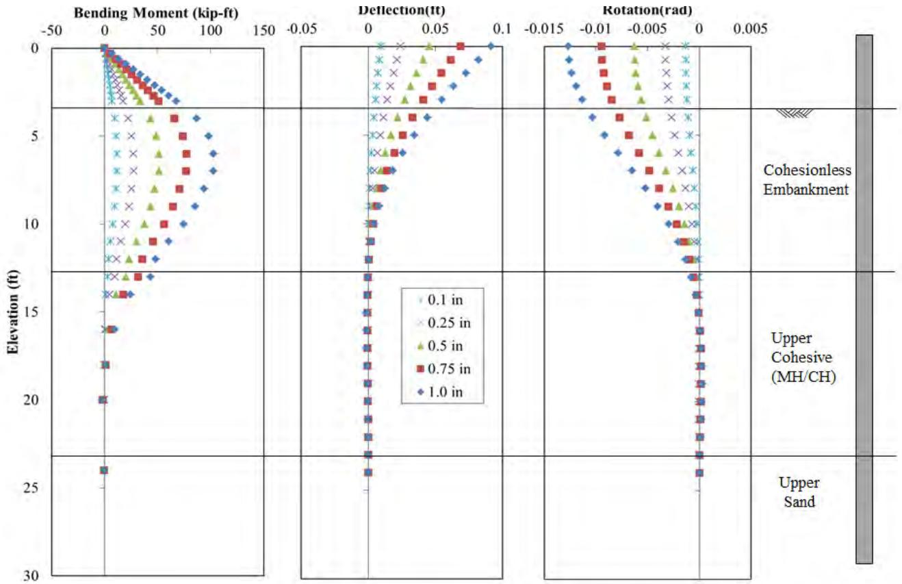
**Figure 12-11** Comparison of Test Results and Analysis Using Back-Calculated  $p$ - $y$  Curves for the 2D (P-6) for Pile Head Displacement of 0.1, 0.25, 0.5 and 1.0 in.
