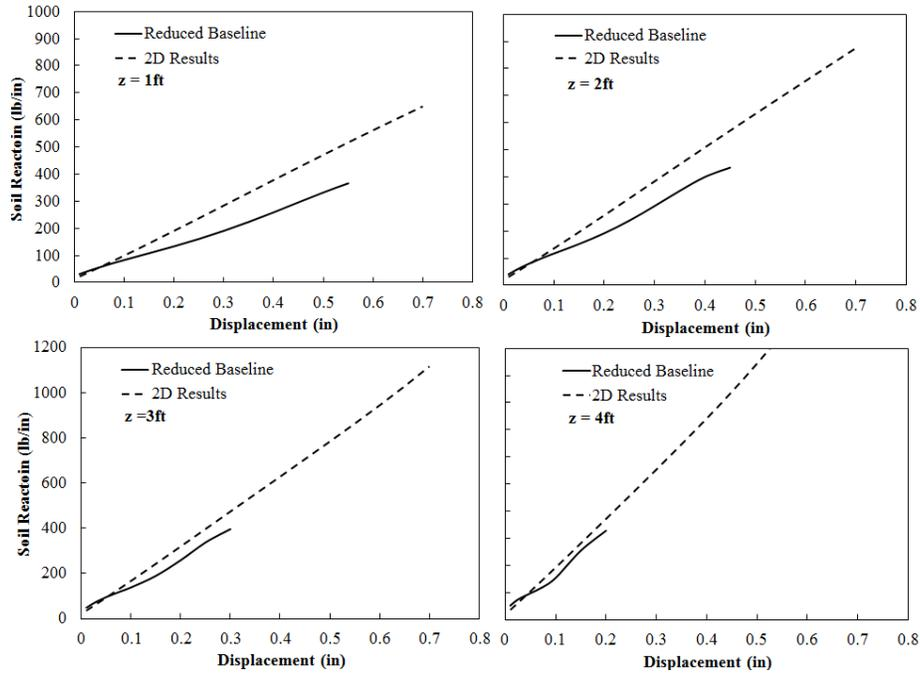
**Figure 13-11** Reduced baseline (with Mezazigh and Levacher (1998) reduction coefficients) and 2D p-y curve comparison
