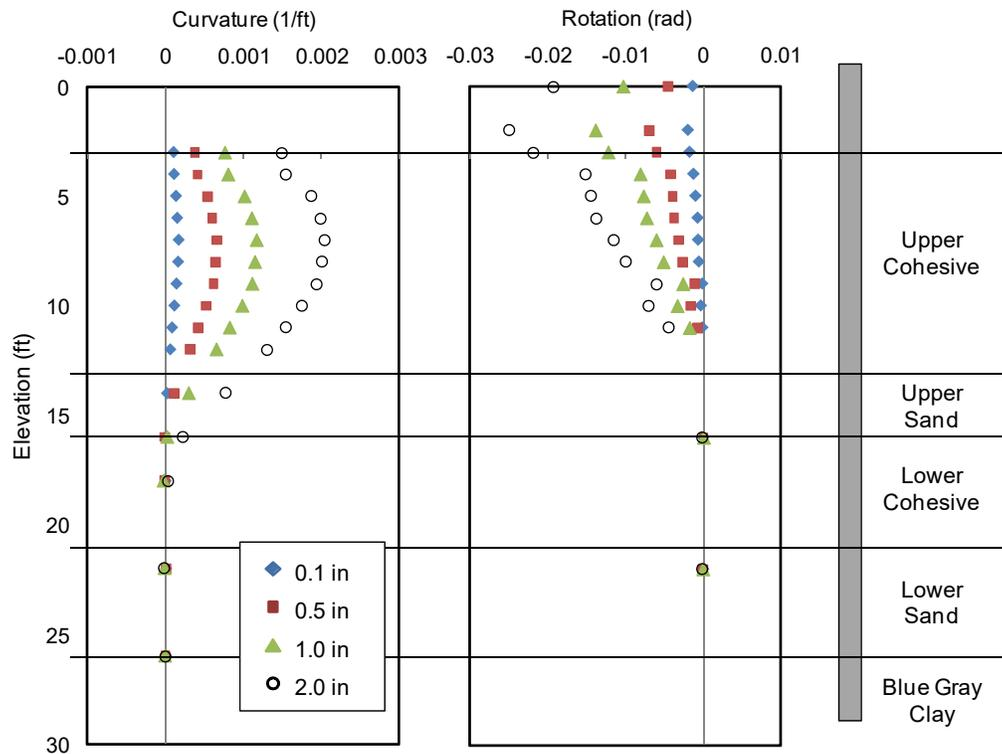
**Figure 6-3.** Test Results of 8D pile (I-6) for Pile Head Displacement of 0.1, 0.5, 1.0 and 2.0 in
