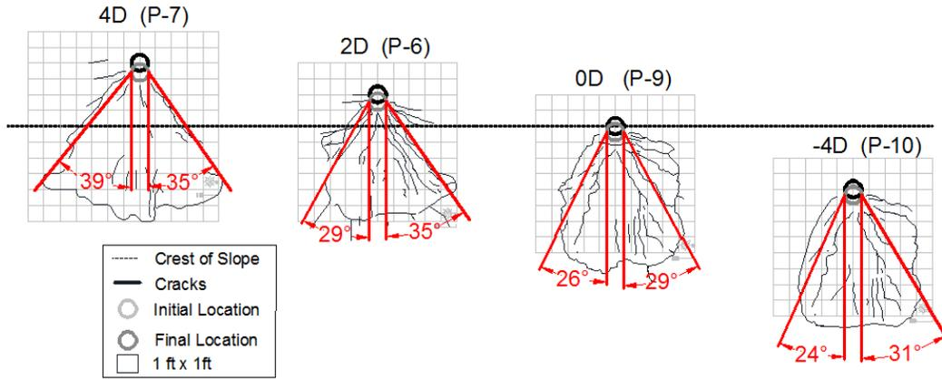
**Figure 10-10** The Shear Failure Angle,  $\Omega$ , for the Near Slope Tests
