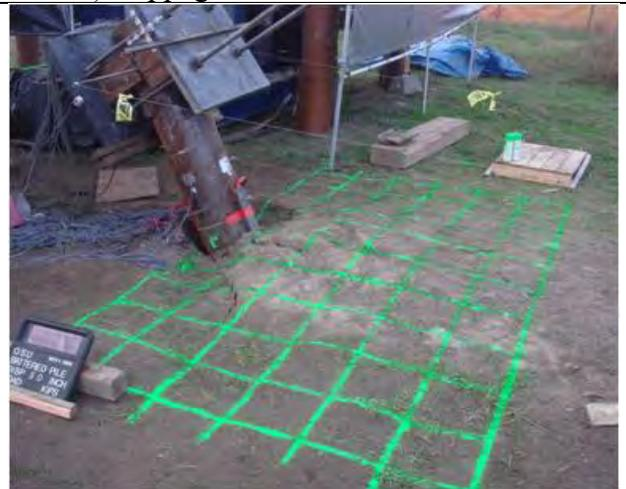
d) Crack pattern at 5" displacement
