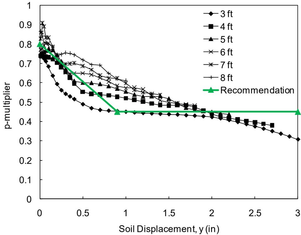
**Figure 7-22.** Direct Comparison of p-Multiplier at Different Depths for 0D Pile (I-7)
