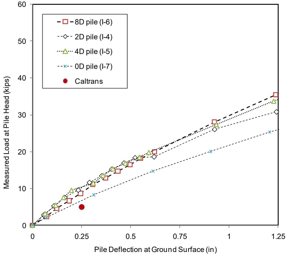
**Figure 6-17.** Comparison of Caltrans Method and Measured Results for 0D Pile, 2D Pile, 4D Pile and 8D Pile
