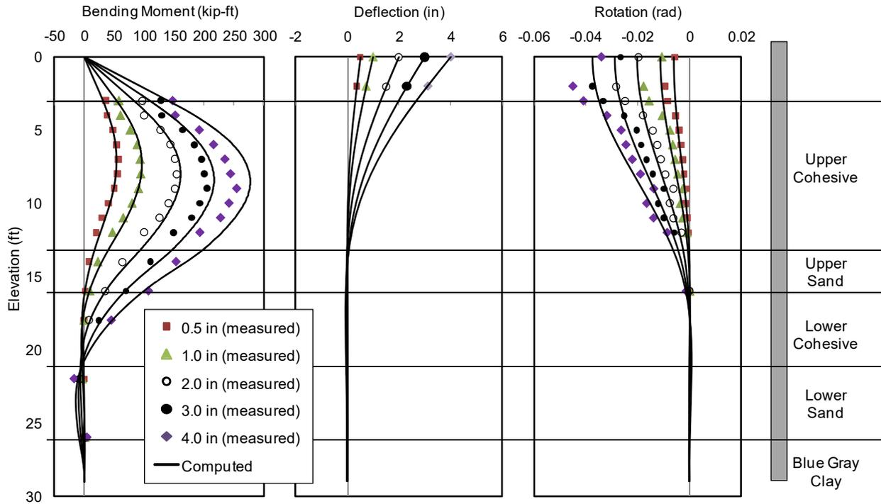
**Figure 7-25.** Comparison of Test Results and Analysis Using Proposed Recommendation for 2D Pile (I-4)
