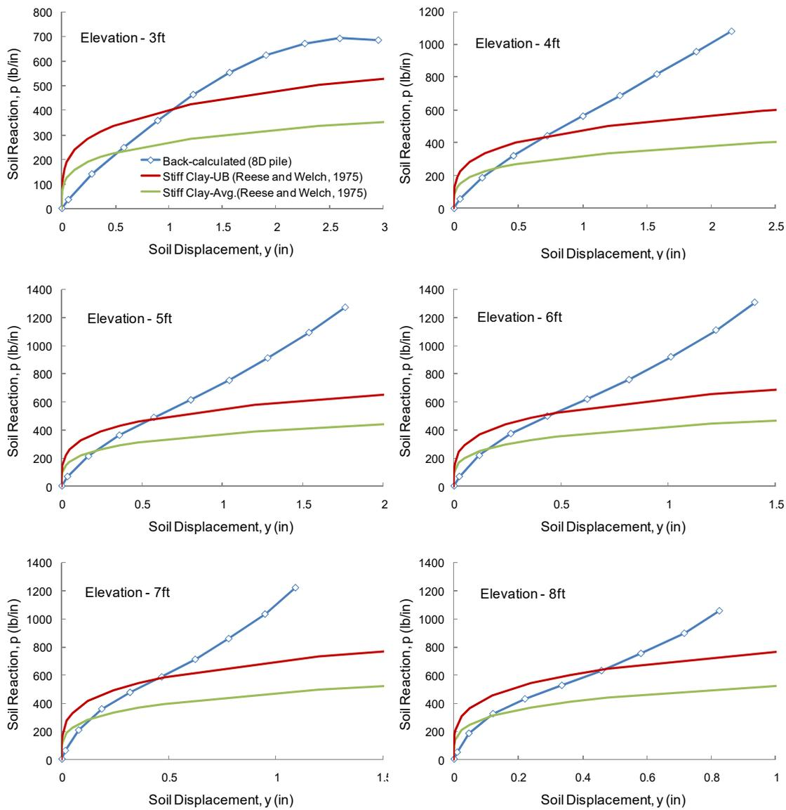
**Figure 8-1.** Comparison of Back-Calculated  $p$ - $y$  Curves for 8D Pile (I-6) to Stiff Clay  $p$ - $y$  Curves (Reese and Welch, 1975) for Elevation 3ft (GS) to 8ft
