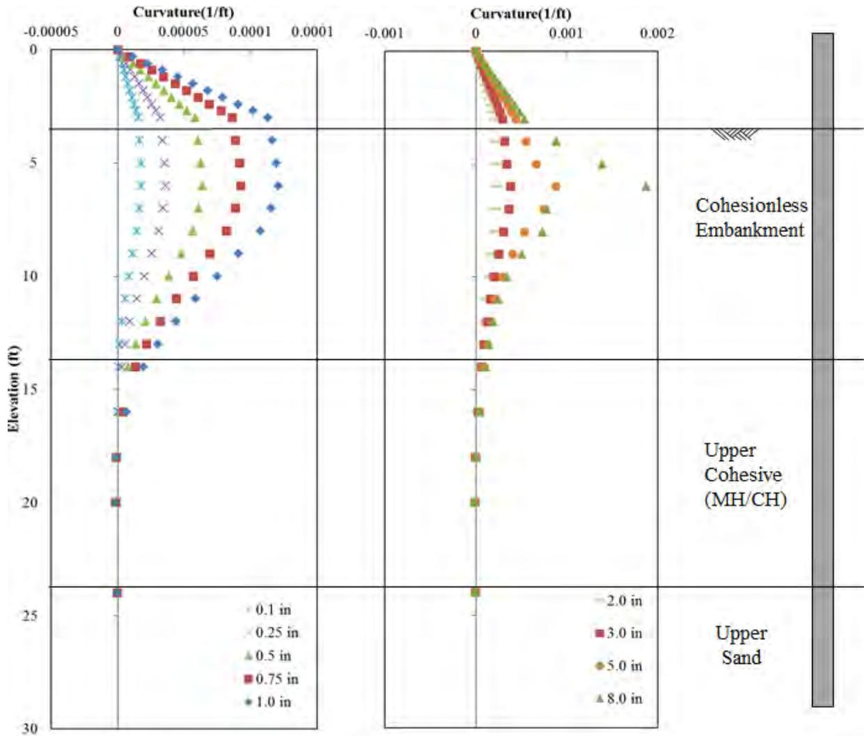
Figure 11-6 Curvature Results for the 4D Pile (P-7) at varying Displacements
