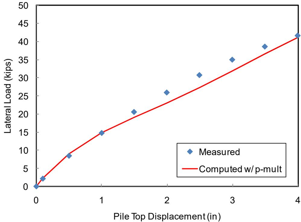
**Figure 7-28.** Comparison of Load-Displacement Curves from Test Results and Analysis Using Proposed Recommendation for 0D Pile (I-7)
