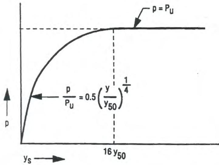
**Figure 2-11** Characteristic Shape of  $p$ - $y$  Curve for Stiff Clay above Water Table for Static Loading (after Welch and Reese 1972; Reese and Welch 1975)
