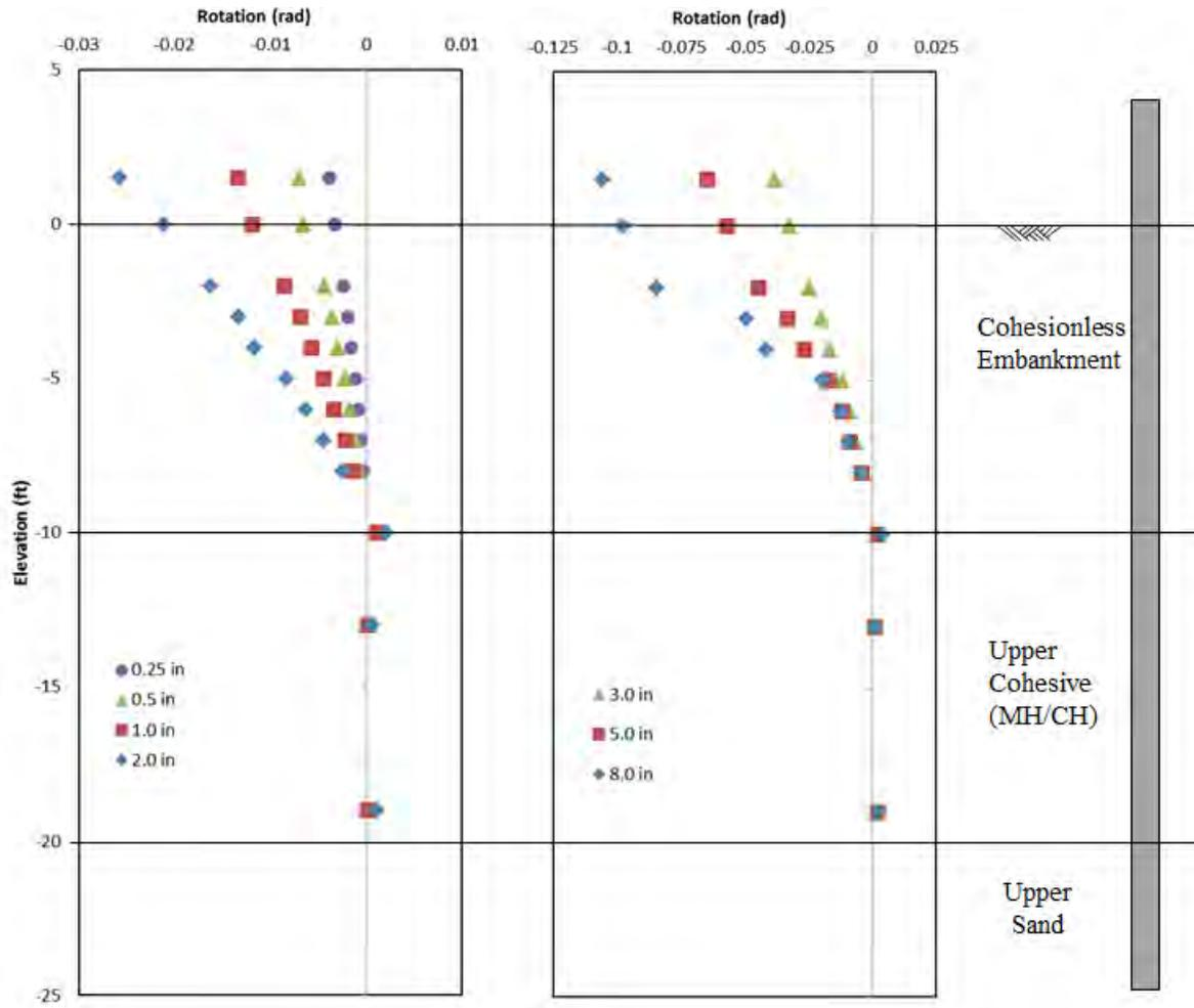
Figure 11-7 Rotation Results for the 4D Pile (P-7) at varying Displacements
