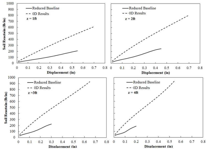
Figure 13-10 Reduced baseline (with Mezazigh and Levacher (1998) reduction coefficients) and 0D p-y curve comparison
