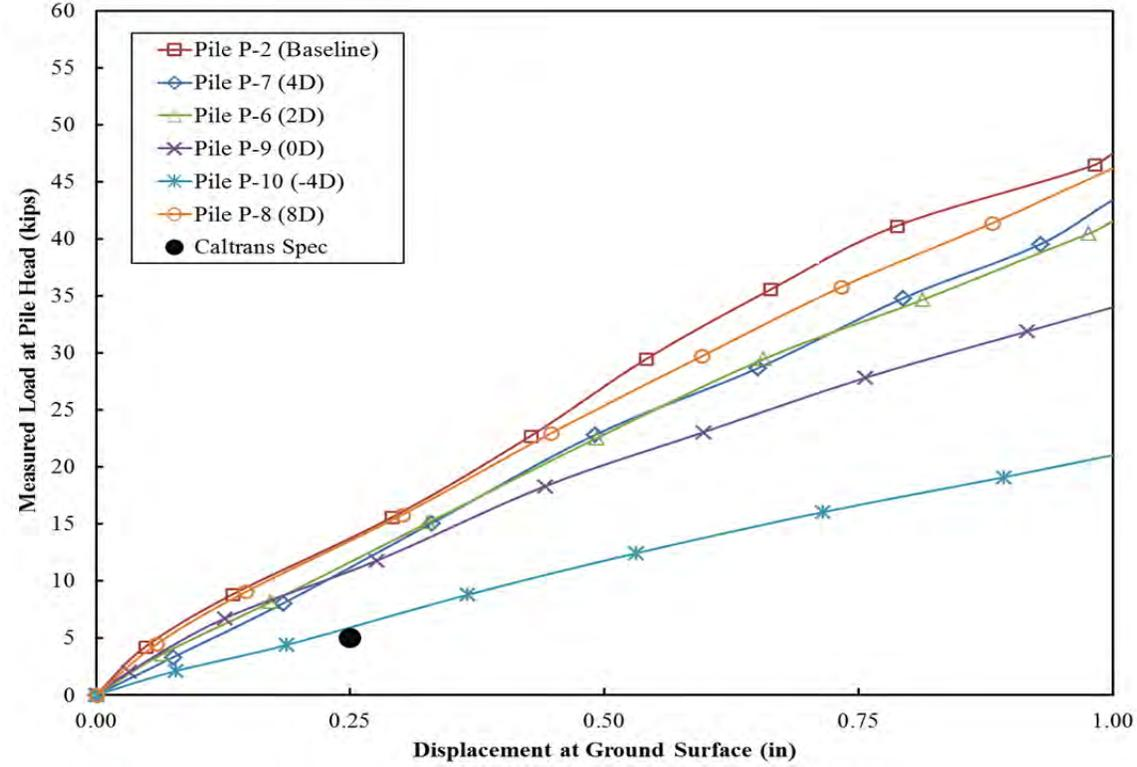
**Figure 11-17** Top: Load Displacement Curve at Ground Surface with Caltrans Spec
