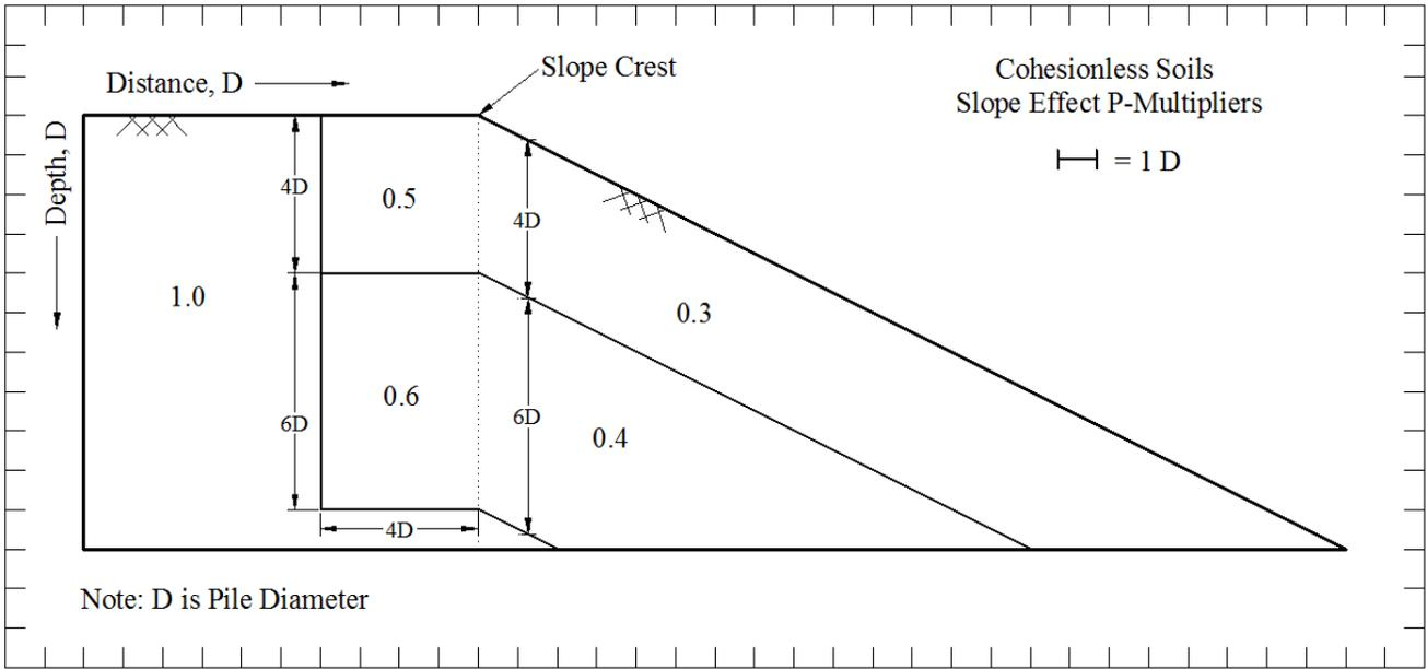
**Figure 14-2** Recommended p-Multipliers for a Generalized Cohesionless Slope
