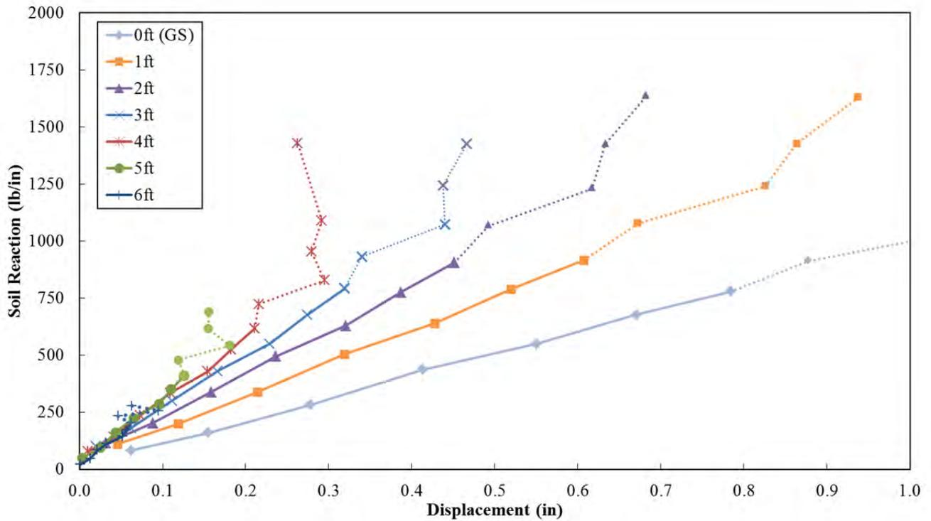
**Figure 12-6** Back-Calculated  $p$ - $y$  Curves for the 4D Pile (P-7) Showing Lower Displacements
