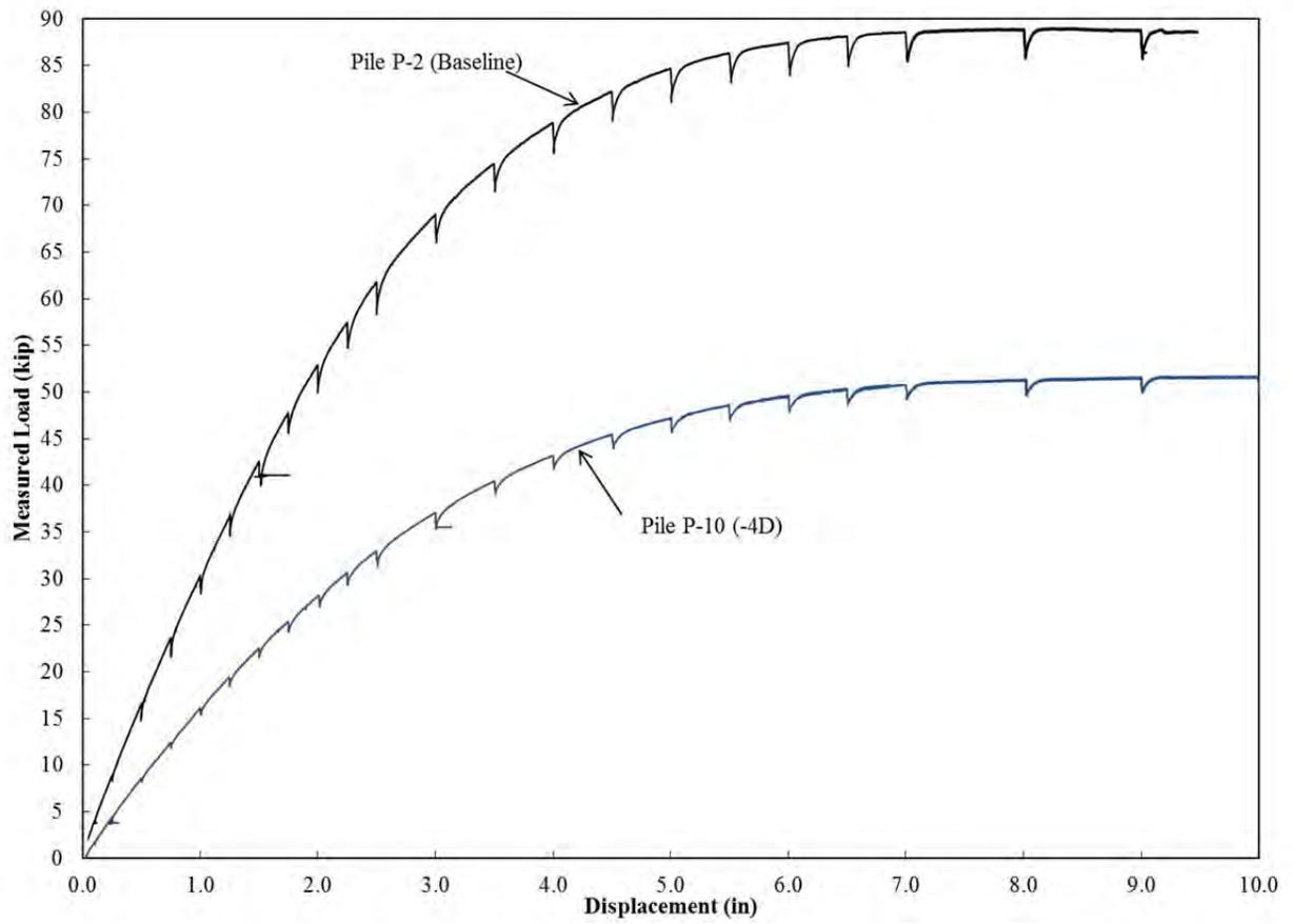
**Figure 11-14** Comparison of Load-Displacement Curves between the Baseline Pile (P-2) and the -4D Pile (P-10)
