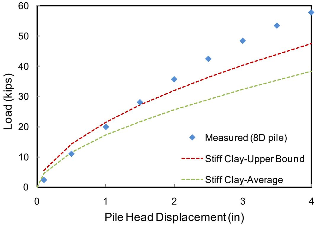
**Figure 8-2.** Comparison of Load-Displacement Curve Using Stiff Clay p-y Curves and Measured Results from 8D pile
