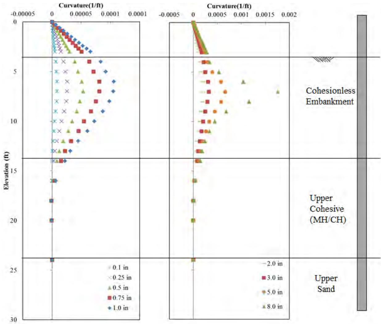
**Figure 11-12** Curvature Results for the OD Pile (P-9) at varying Displacements
