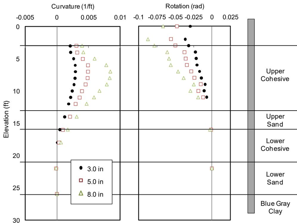
**Figure 6-4.** Test Results of 8D pile (I-6) for Pile Head Displacement of 3.0, 5.0 and 8.0 in
