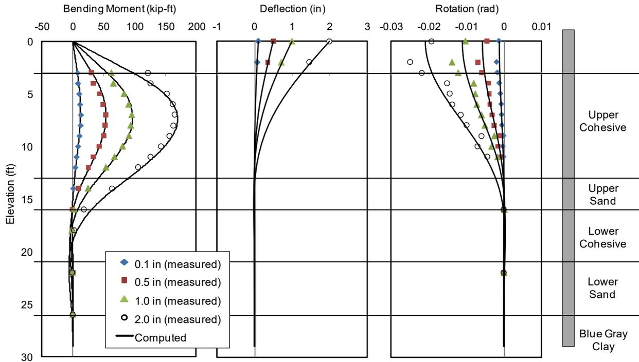
**Figure 7-4.** Comparison of Test Results and Analysis Using Back-Calculated  $p$ - $y$  Curves for 8D Pile (I-6) for Pile Head Displacement of 0.1, 0.5, 1.0 and 2.0 in.
