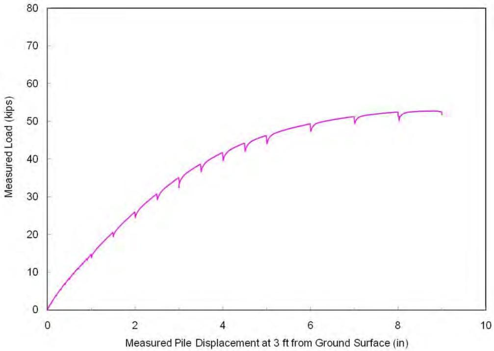
**Figure 6-11.** Load Displacement Curves for 0D pile (I-7)
