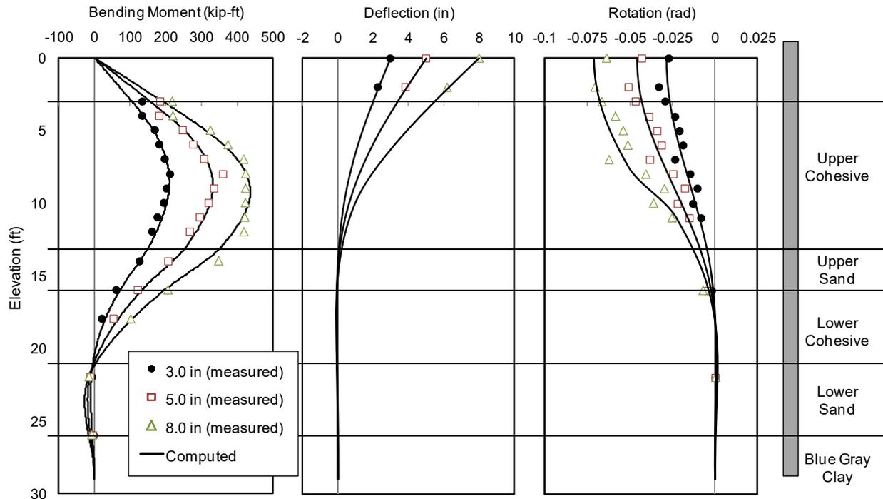
**Figure 7-17.** Comparison of Test Results and Analysis Using Back-Calculated  $p$ - $y$  Curves for OD Pile (I-7) for Pile Head Displacement of 3.0, 5.0 and 8.0 in.
