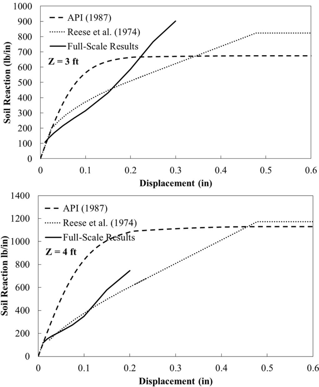
**Figure 13-8** Comparison of the API (1987), Reese et al. (1974) predicted baseline p-y curves with full-scale results at depths of 3 ft (top) and 4 ft (bottom)
