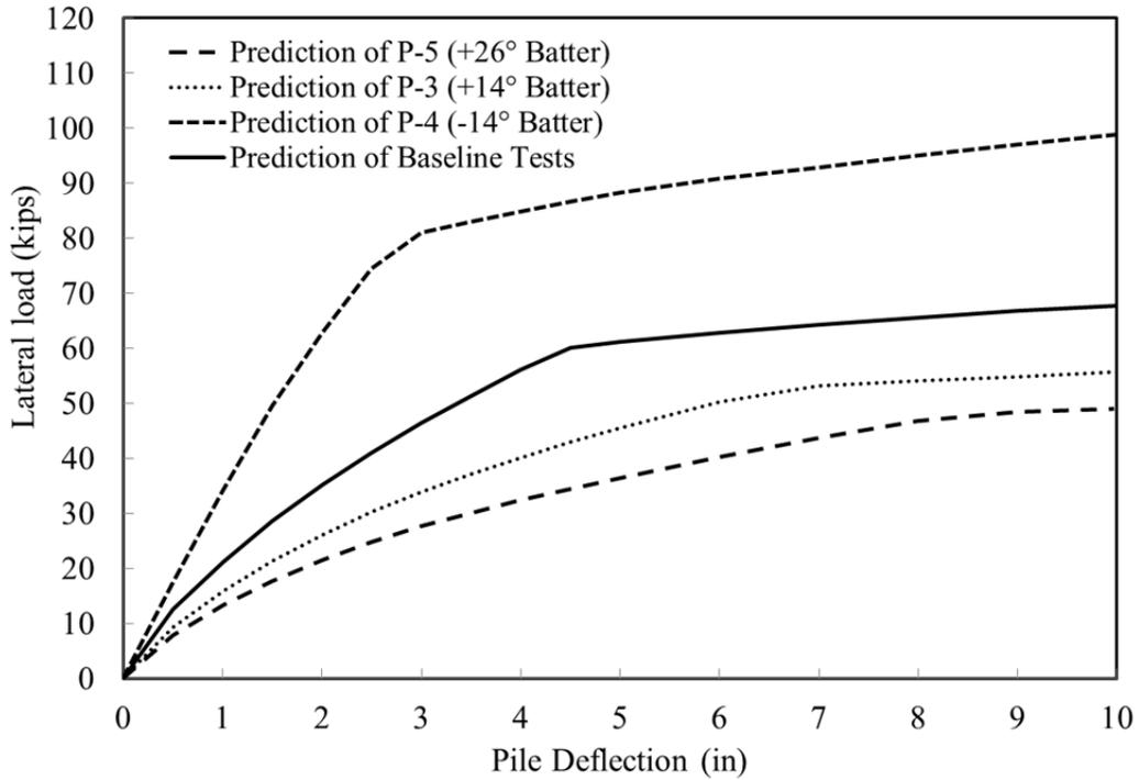
**Figure 11-19** Predicted Load-Displacement Curves for the Battered Pile and Baseline Piles from LPILE
