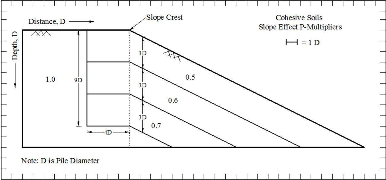
**Figure 14-1** Recommended p-Multipliers for a Generalized Cohesive Slope
