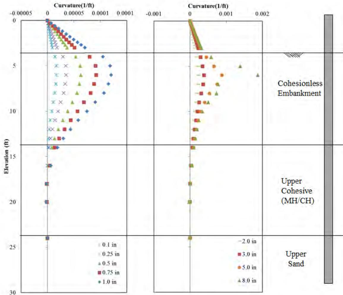
Figure 11-3 Curvature Results for Baseline Pile (P-2) at varying Displacements
