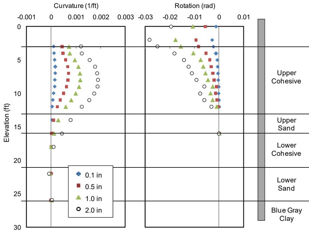
**Figure 6-6.** Test Results of 2D pile (I-4) for Pile Head Displacement of 0.1, 0.5, 1.0 and 2.0 in
