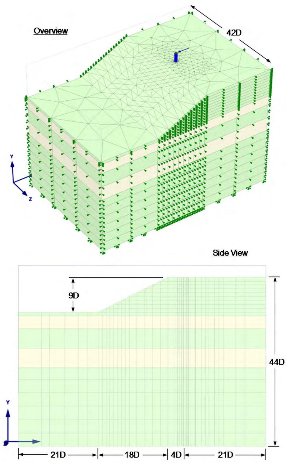
**Figure 9-6** Finite Element Mesh for the 4D Pile
