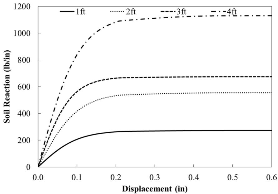
**Figure 13-6** API (1987) predicted baseline p-y curves with input soil properties matching the full-scale tests
