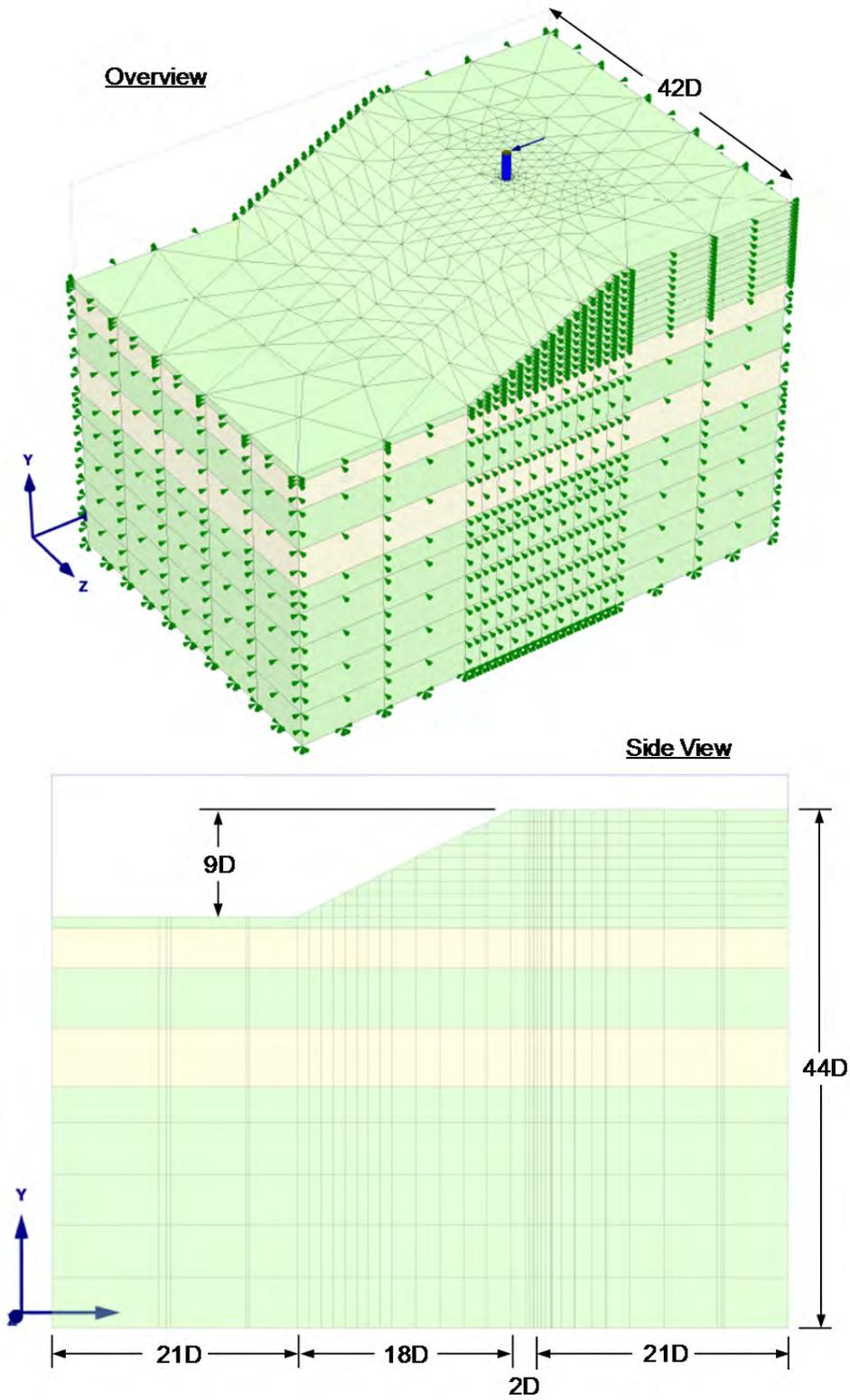
**Figure 9-5** Finite Element Mesh for the 2D Pile
