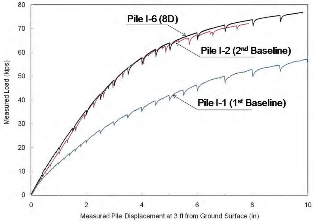
**Figure 6-1.** Comparison of Load-Displacement Curves between Baseline Piles (I-1 and I-2) and Pile at 8D from the Slope Crest (I-6)
