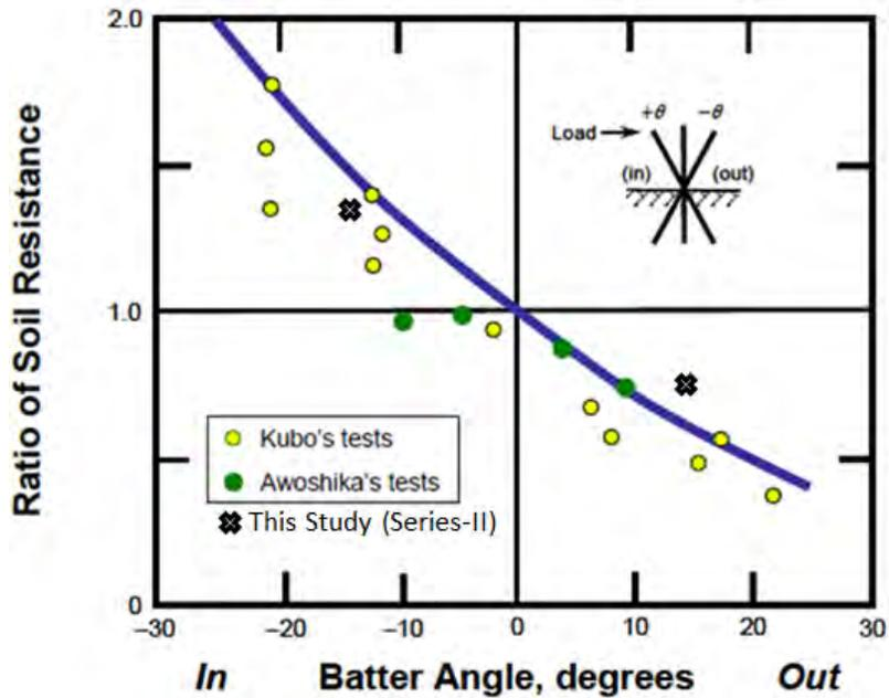
**Figure 11-20** Model used for LPILE Battered Pile Predictions with the +14° and -14° Battered Pile Results from this Study (Series-II) (after Reese et al., 2004)
