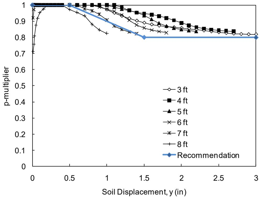
Figure 7-20. Direct Comparison of p-multiplier at Different Depths for 4D Pile (I-5)
