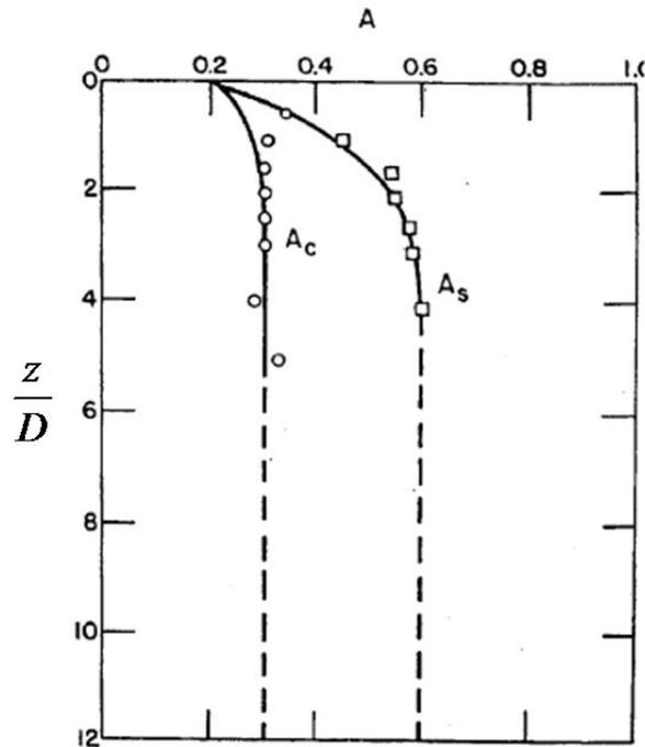
**Figure 2-10** Value of Constant  $A$  for  $p$ - $y$  Curves for Stiff Clay Below Water Table (after Reese *et al.* 1975)
