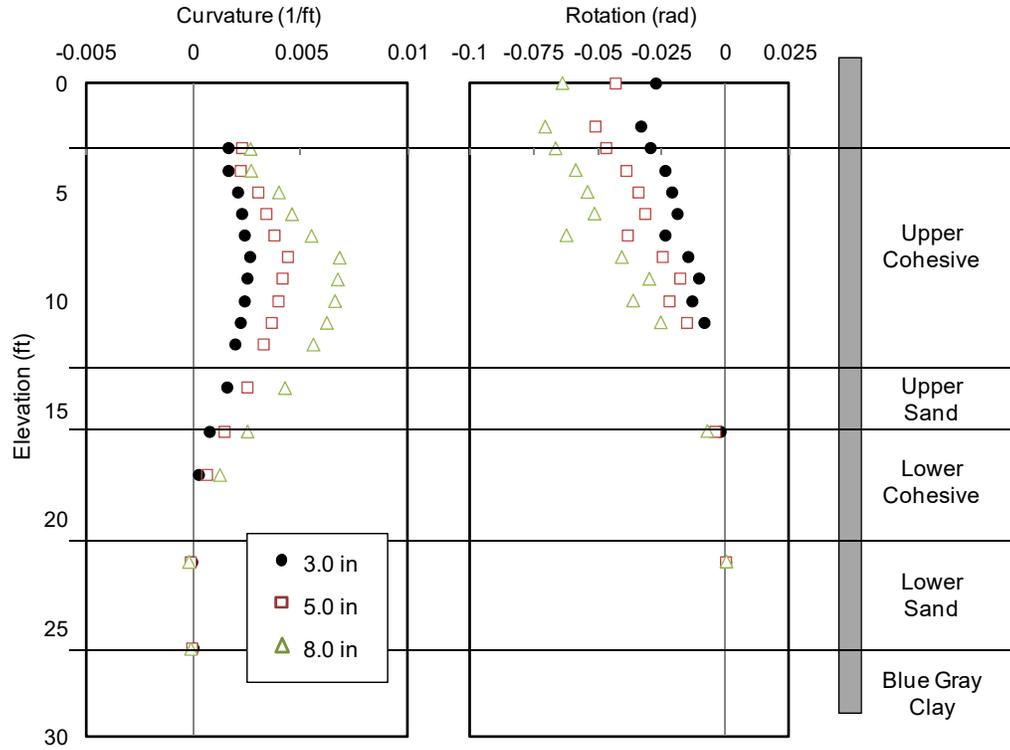
**Figure 6-13.** Test Results of 0D Pile (I-7) for Pile Head Displacement of 3.0, 5.0 and 8.0 in
