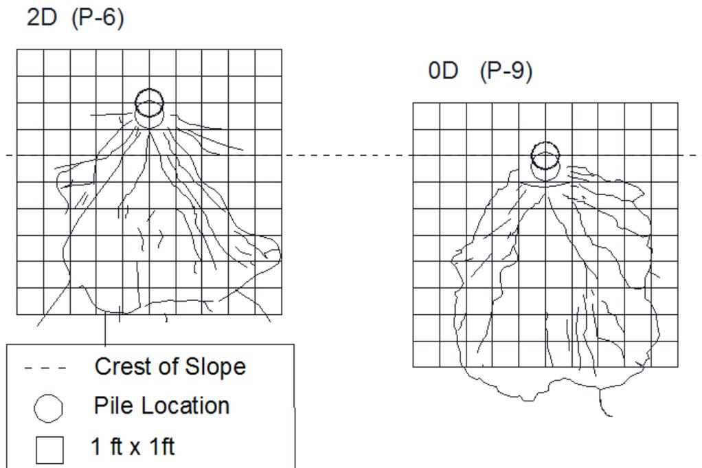
**Figure 10-12** Cracking Patterns for the 2D and 0D Test Piles
