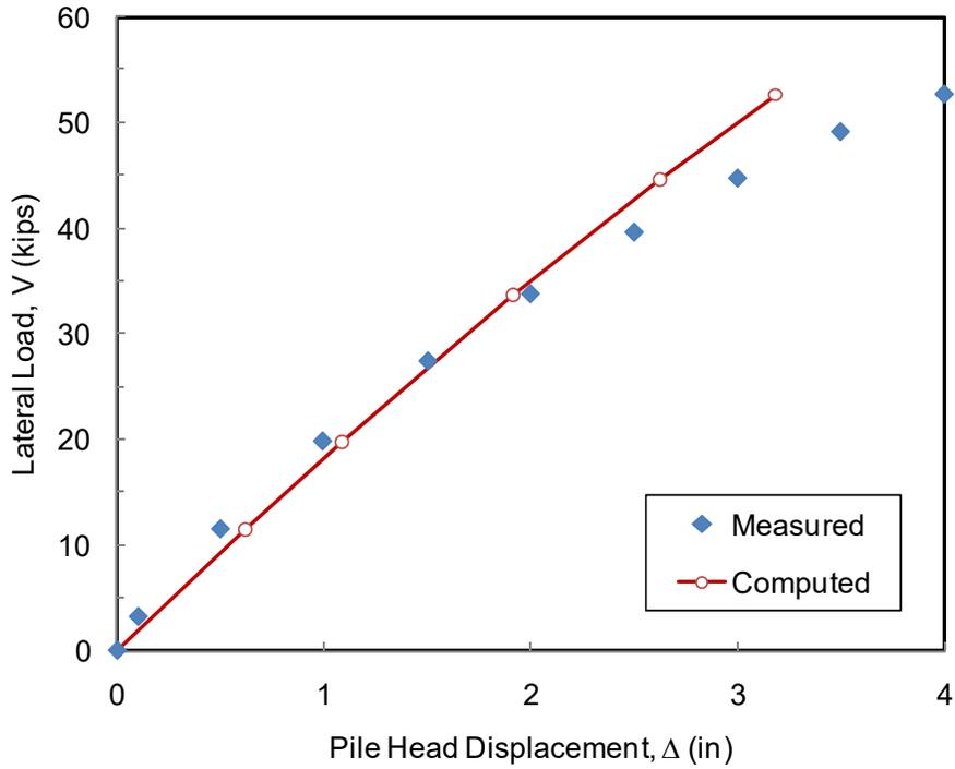
**Figure 9-13** Comparison of Load-Displacement Curve from Test Results and FEM Analysis for the 4D Pile
