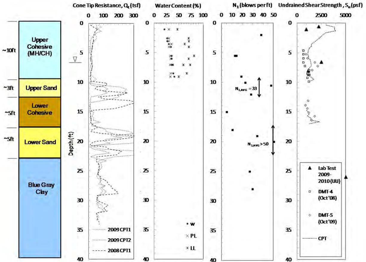
Figure 3-4. Summary of Site Specific Explorations for Caltrans Pile Load Study (as of March 31, 2010)
