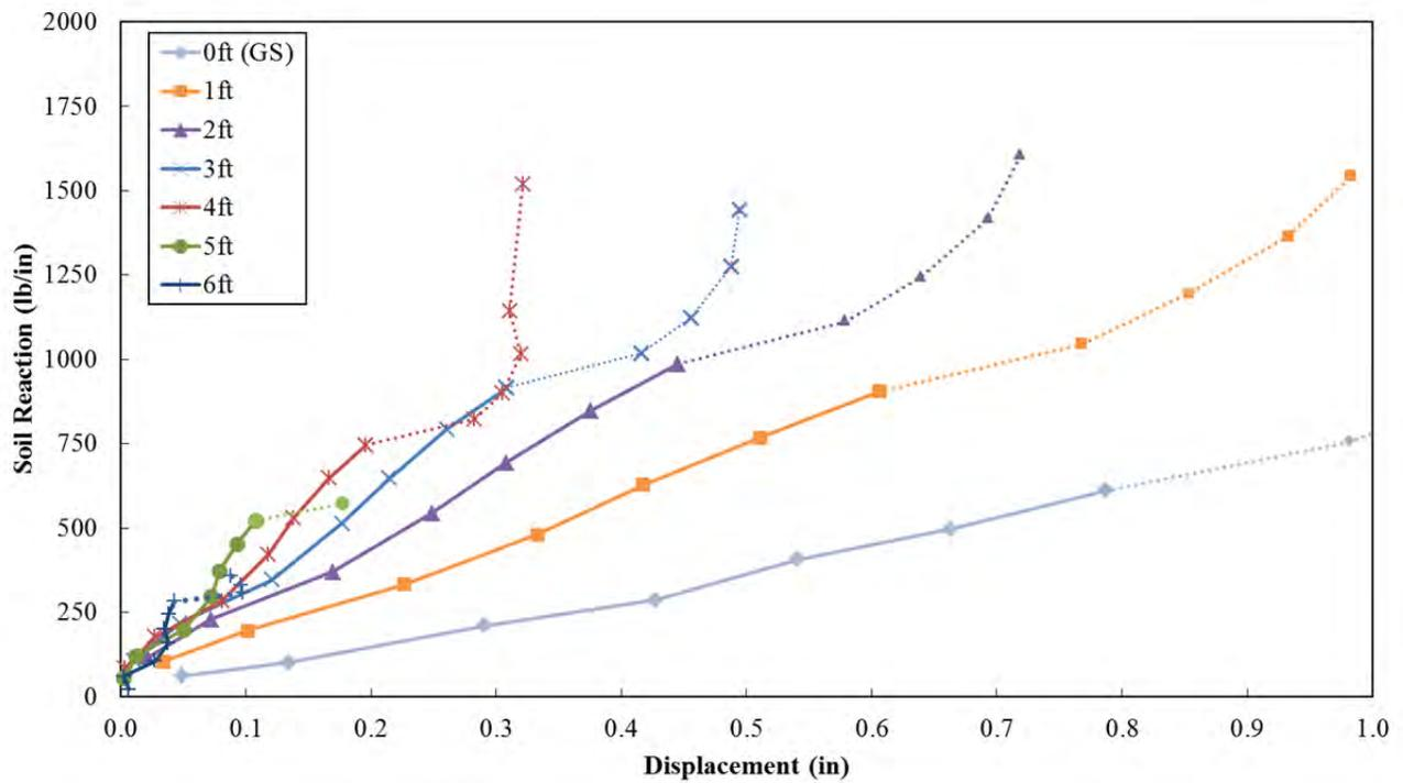
**Figure 12-2** Back-Calculated  $p$ - $y$  Curves for the -Baseline Pile (P-2) with Lower Displacements
