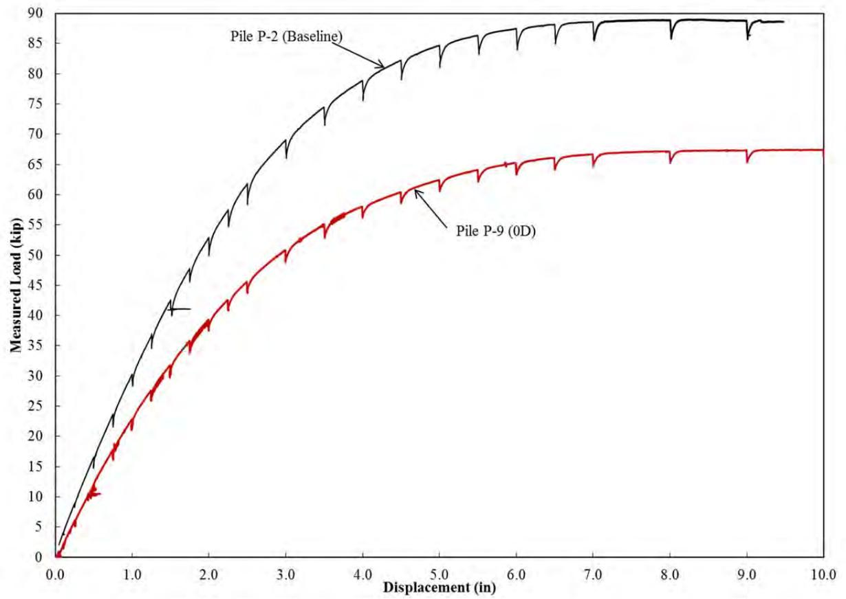
**Figure 11-11** Comparison of Load-Displacement Curves between the Baseline Pile (P-2) and the 0D Pile (P-9)
