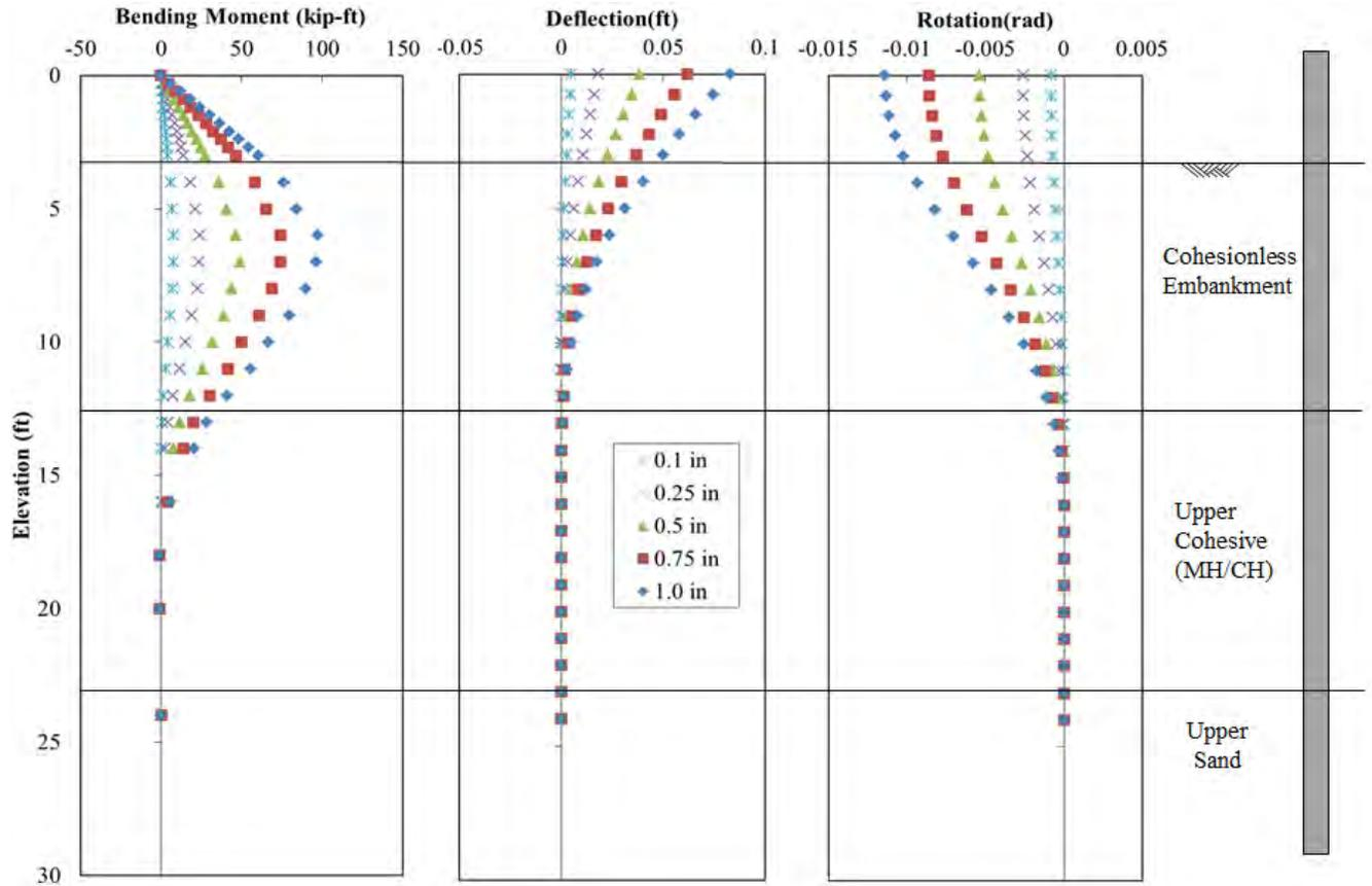
**Figure 12-15** Comparison of Test Results and Analysis Using Back-Calculated  $p$ - $y$  Curves for the 0 (P-9) for Pile Head Displacement of 0.1, 0.25, 0.5 and 1.0 in.
