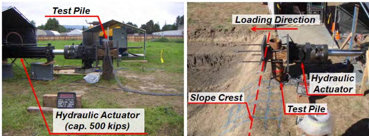
Figure 4-6. Actual test setup – Baseline Pile Test (left) and Pile Located at 2D from the Slope Crest (right)
