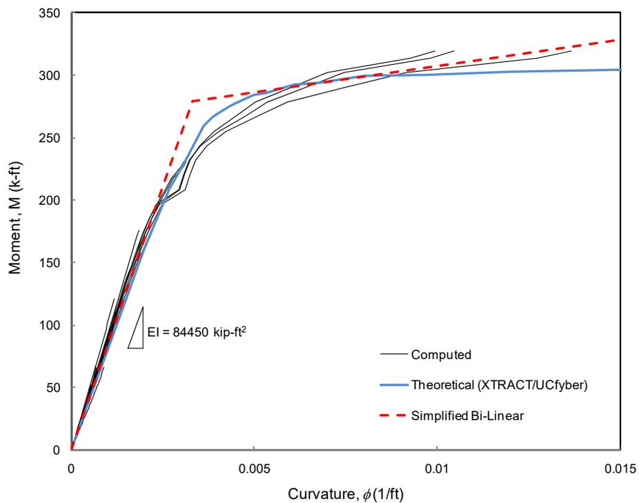
**Figure 4-4.** Comparison of Computed and Theoretical Moment-Curvature Relationship
