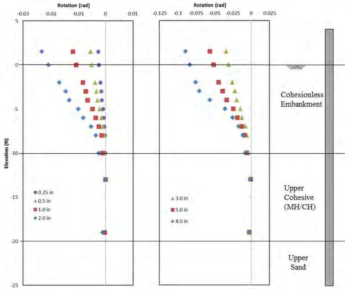
Figure 11-13 Rotation Results for the OD Pile (P-9) at varying Displacements
