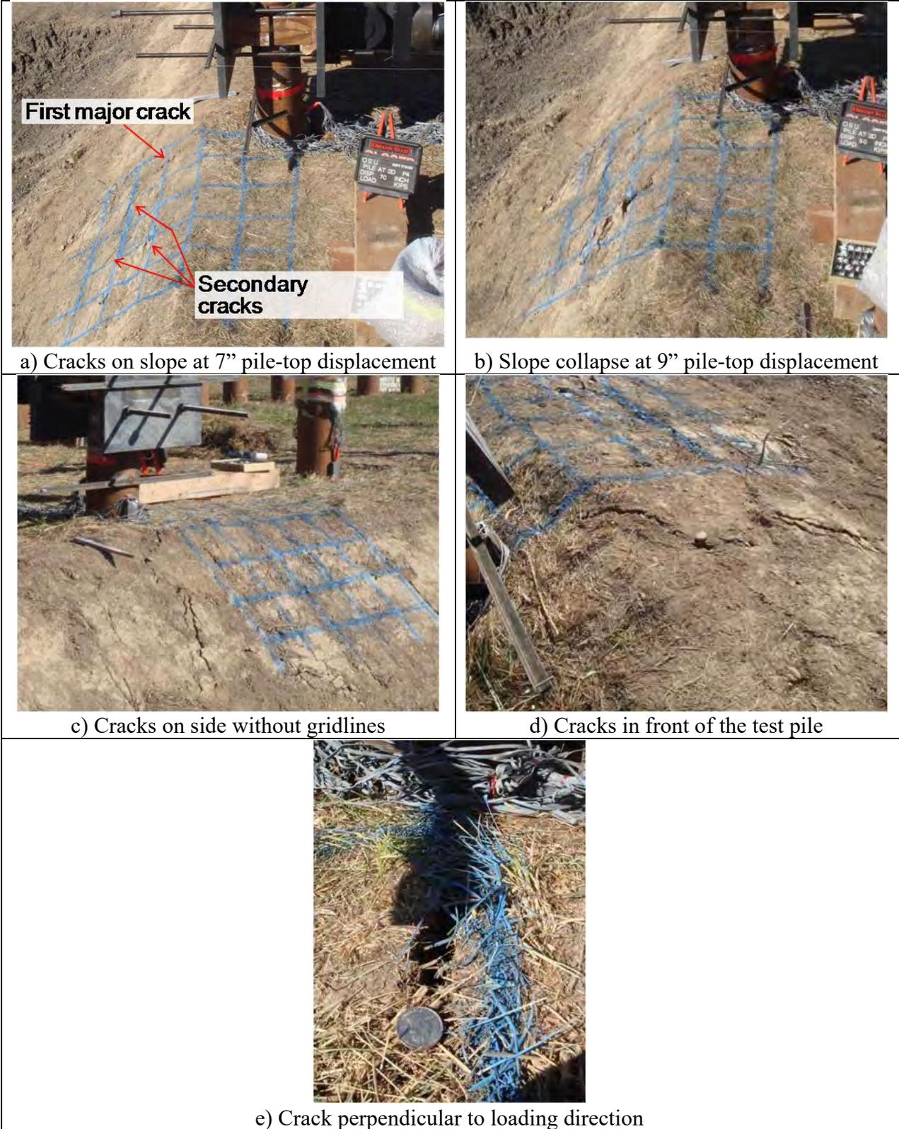
**Figure 5-2.** Observations from Lateral Load Test for 2D Pile (I-4)
