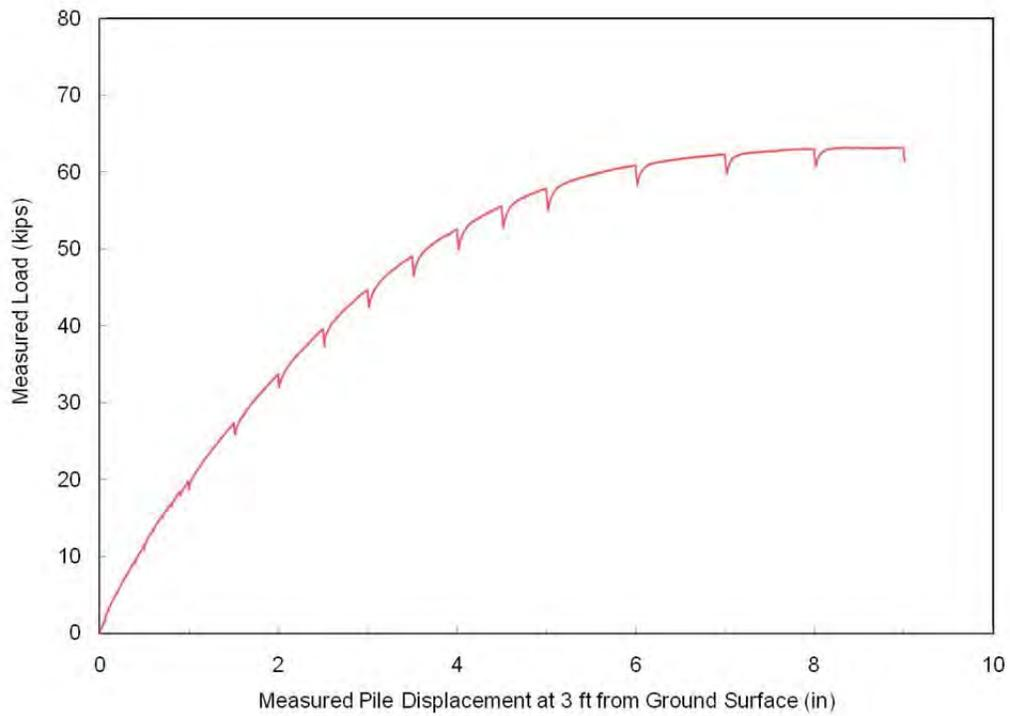
**Figure 6-8.** Load Displacement Curve for 4D pile (I-5)
