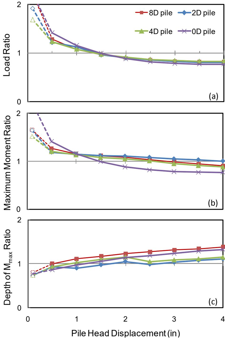
**Figure 8-4.** Predicted Pile Head Load, Maximum Moment and Depth to Maximum Moment using Stiff Clay curve (Reese and Welch, 1975) and Proposed Design Recommendation Compared to Measured Response for (a) Pile Head Load, (b) Maximum Moment, and (c) Depth to Maximum Moment
