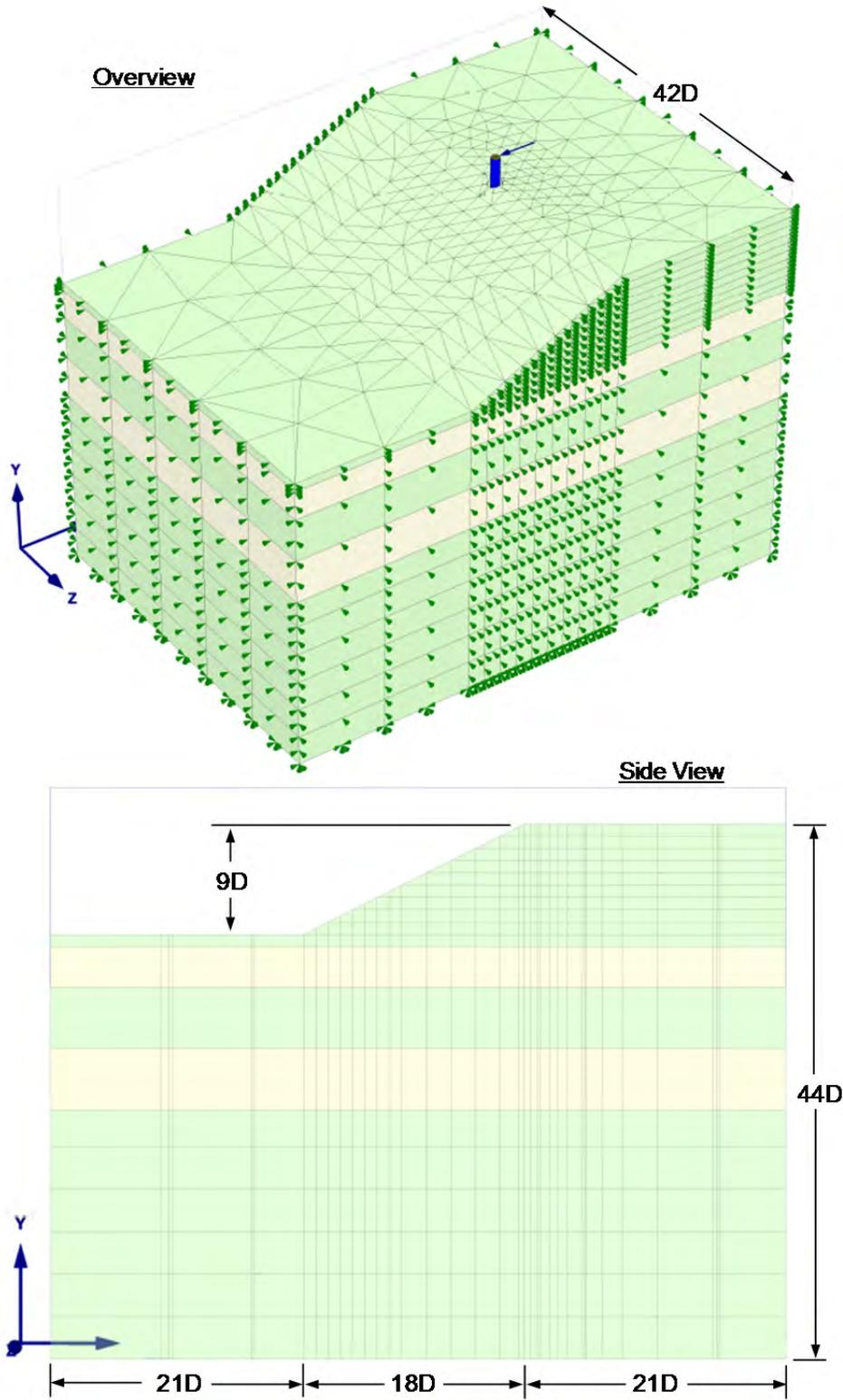
Figure 9-4 Finite Element Mesh for the OD Pile
