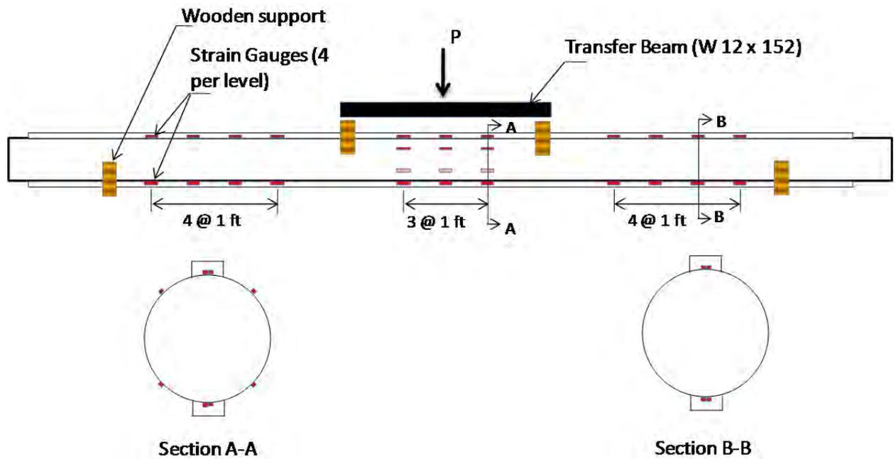
**Figure 4-3.** Test Set-Up for Calibration Pile
