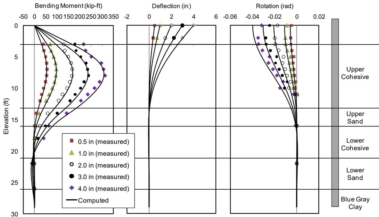
**Figure 7-27.** Comparison of Test Results and Analysis Using Recommendation for 4D Pile (I-5)
