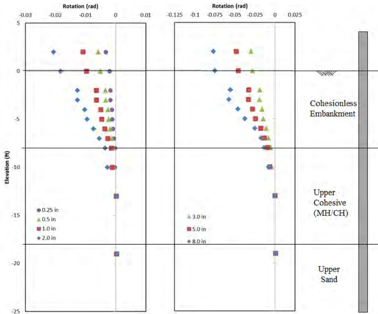
Figure 11-16 Rotation Results for the -4D Pile (P-10) at varying Displacements
