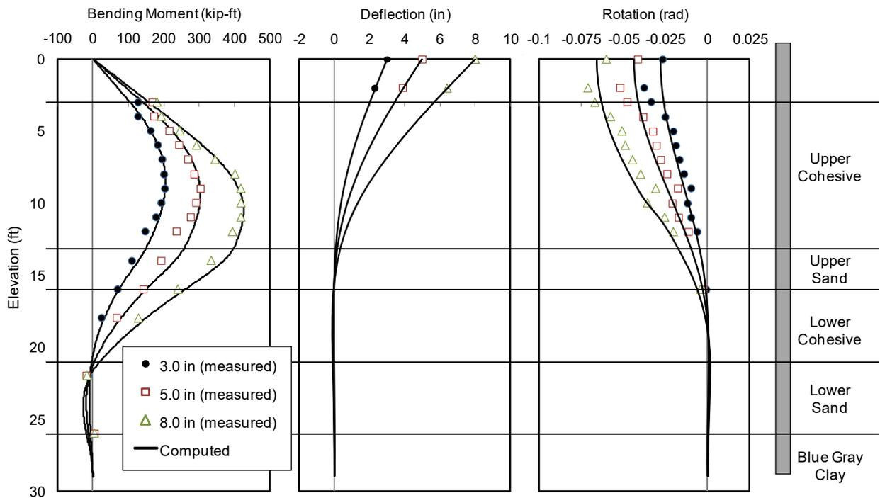
**Figure 7-9.** Comparison of Test Results and Analysis Using Back-Calculated  $p$ - $y$  Curves for 2D Pile (I-4) for Pile Head Displacement of 3.0, 5.0 and 8.0 in.
