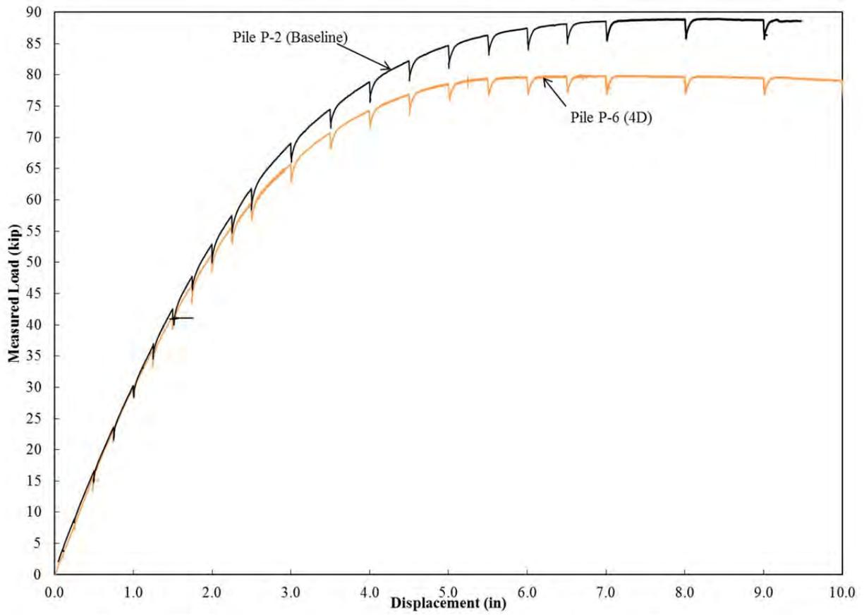
**Figure 11-5** Comparison of Load-Displacement Curves between the Baseline Pile (P-2) and the 4D Pile (P-7)
