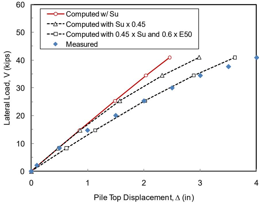
**Figure 9-15** Comparison of Load-Displacement Curves from Sensitivity Analysis and the Measured Results for the OD Pile
