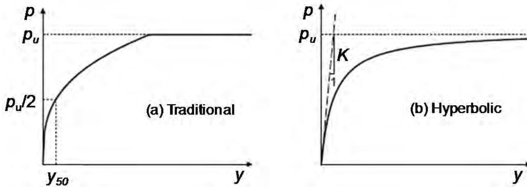
**Figure 2-7** Typical Shapes of  $p$ - $y$  Curves (after Georgiadis and Georgiadis 2010)
