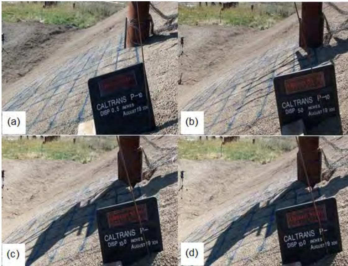
**Figure 10-6** Observations during lateral loading testing of pile P-10 (-4D)
