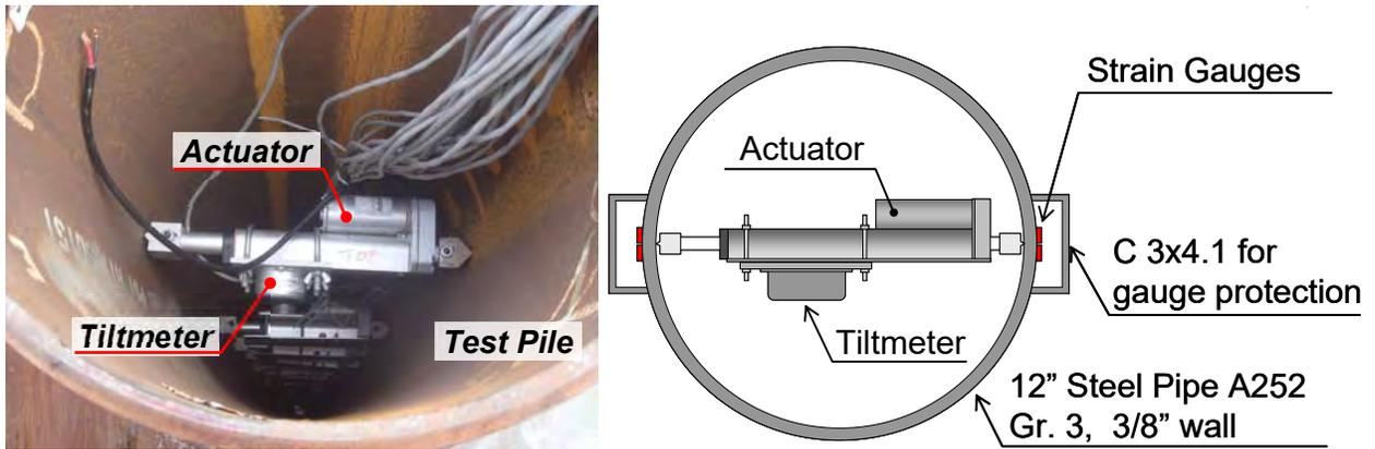
**Figure 4-13.** Cross-section view of test pile showing tiltmeter arrangement
