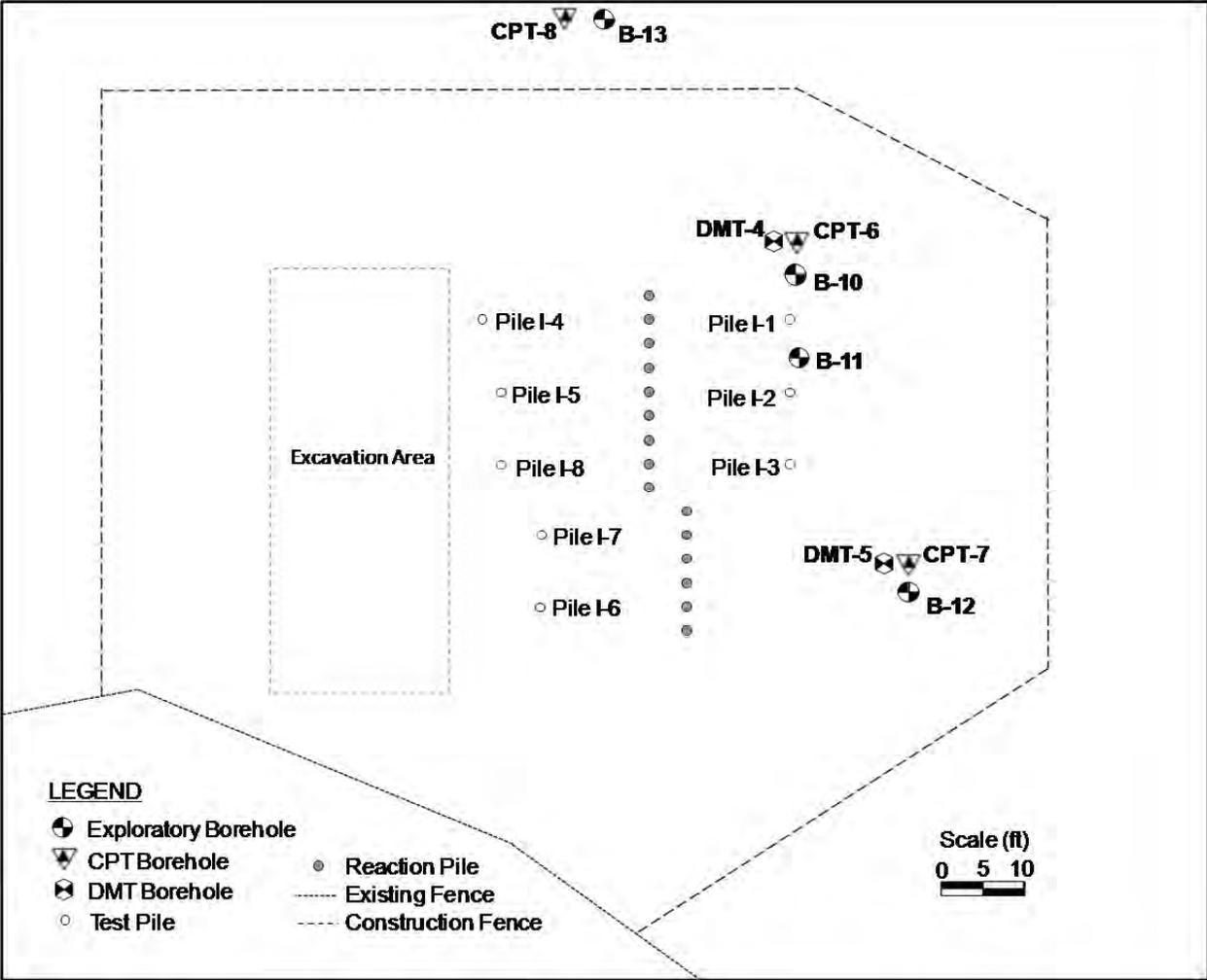
Figure 3-3. Locations of Borings and Test Piles locations at the Caltrans Test Site.
