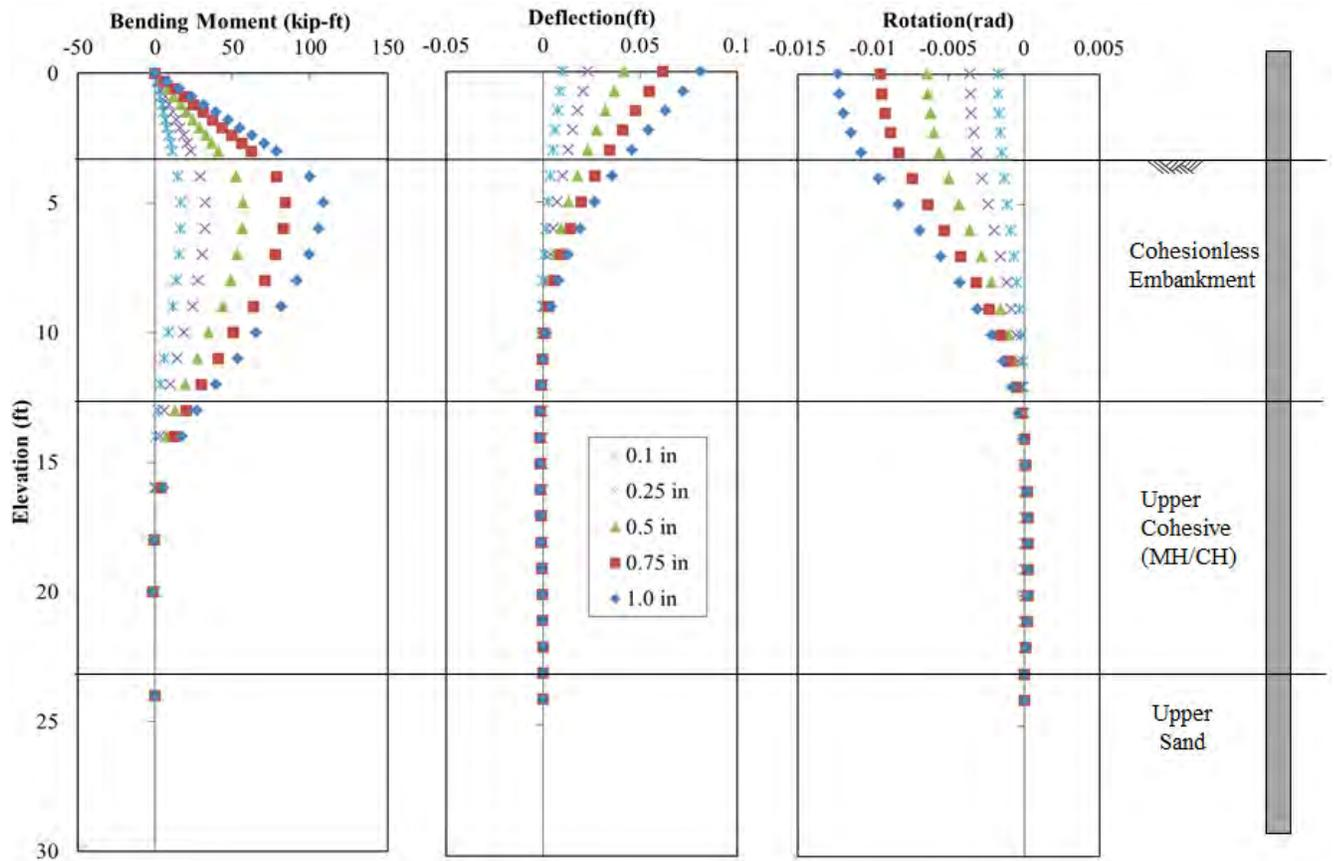
**Figure 12-7** Comparison of Test Results and Analysis Using Back-Calculated  $p$ - $y$  Curves for the 4D Pile (P-7) for Pile Head Displacement of 0.1, 0.25, 0.5 and 1.0 in.
