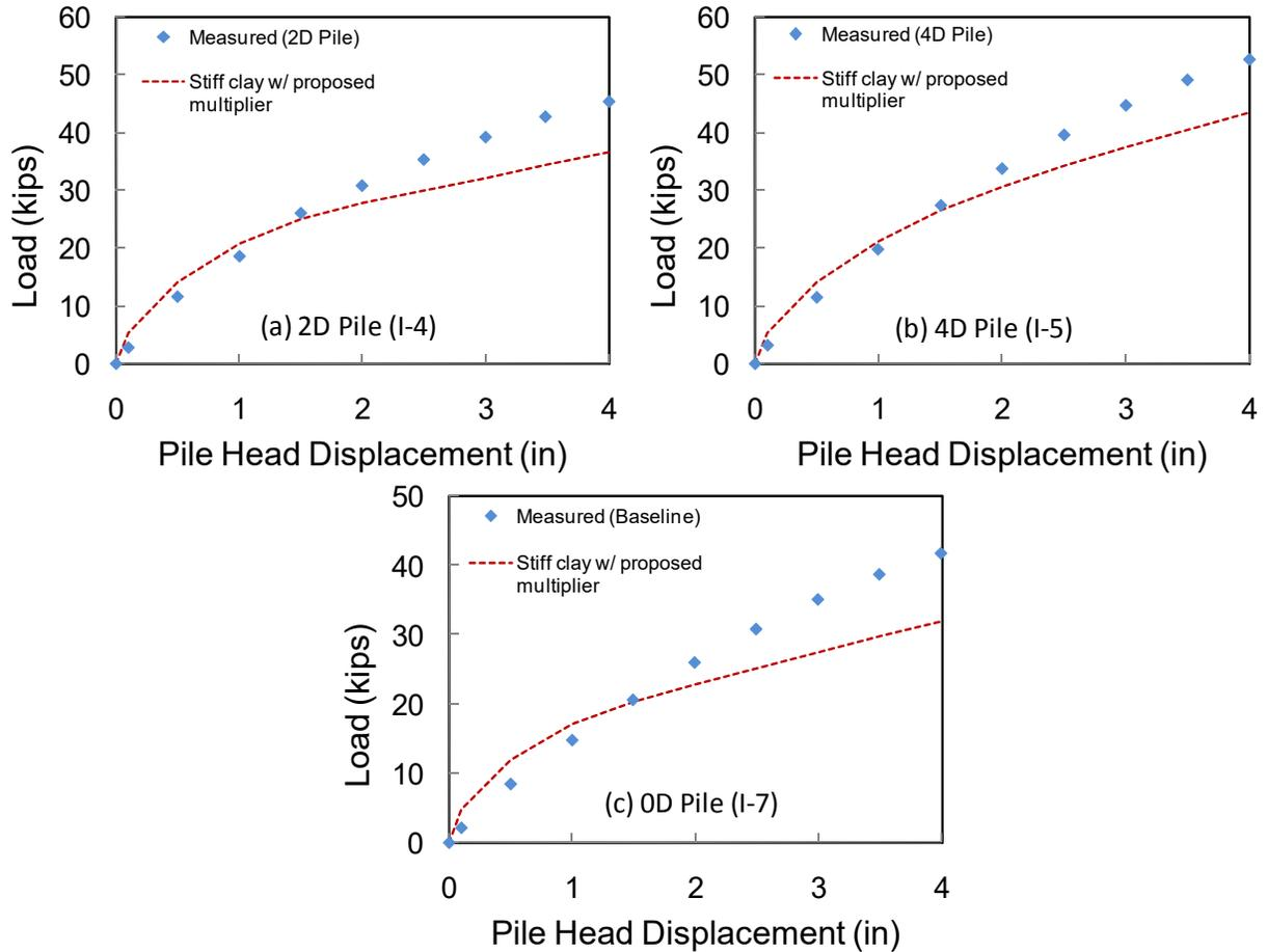
**Figure 8-3.** Computed Load Displacement Curves using Stiff Clay  $p$ - $y$  Curve (Reese and Welch, 1975) and Proposed Recommendation Compared to Measured Response (a) 2D Pile (I-4), (b) 4D Pile (I-5) and OD Pile (I-7)
