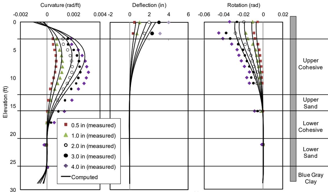
**Figure 9-12** Comparison of Test Results and FEM Analysis for the 2D Pile
