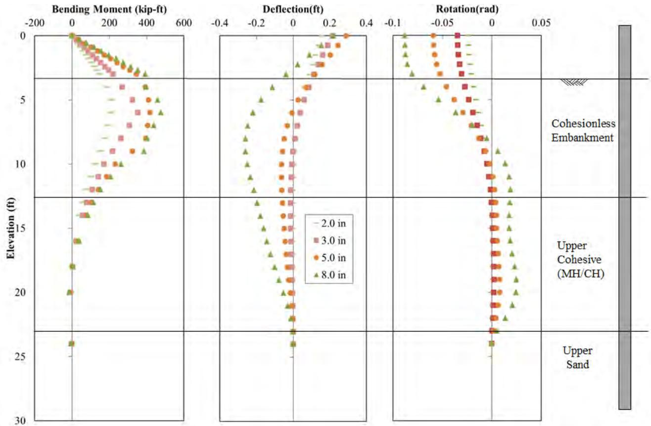
**Figure 12-8** Comparison of Test Results and Analysis Using Back-Calculated  $p$ - $y$  Curves for the 4D Pile (P-7) for Pile Head Displacement of 2.0, 3.0, 5.0 and 8.0 in.
