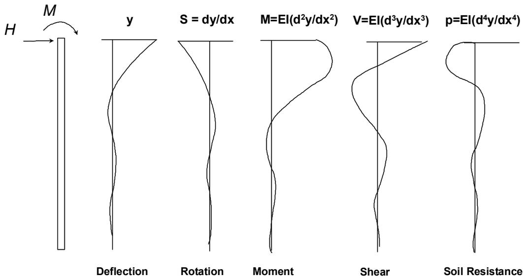
**Figure 2-4** Methodology in Developing  $p$ - $y$  Curves (after Reese and Van Impe 2001)
