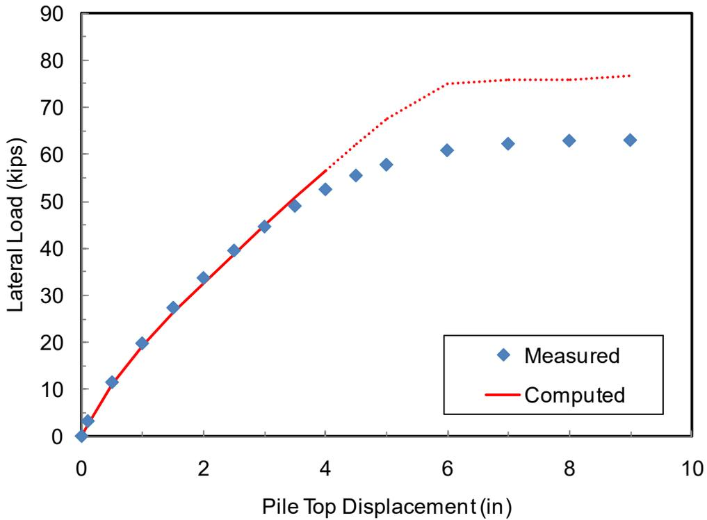
**Figure 7-11.** Comparison of Load-Displacement Curves from Test Results and Analysis Using Back-Calculated  $p$ - $y$  Curves for 4D pile (I-5)
