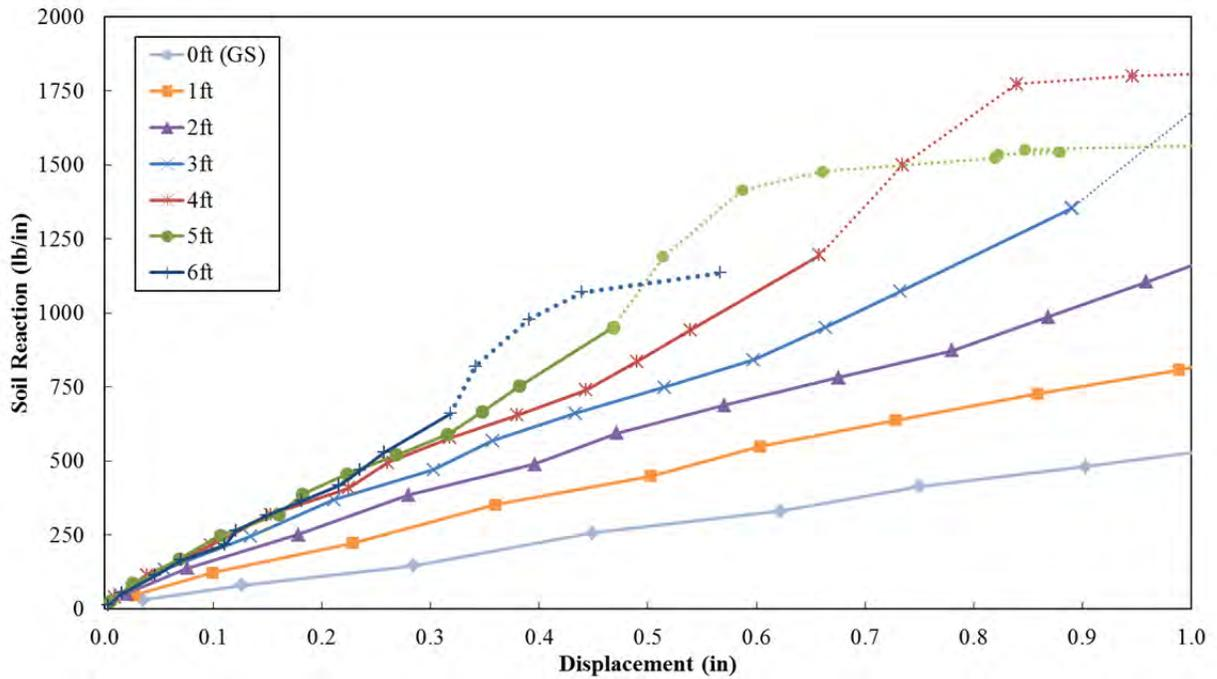
**Figure 12-14** Back-Calculated  $p$ - $y$  Curves for the 0D Pile (P-9) Showing Lower Displacements
