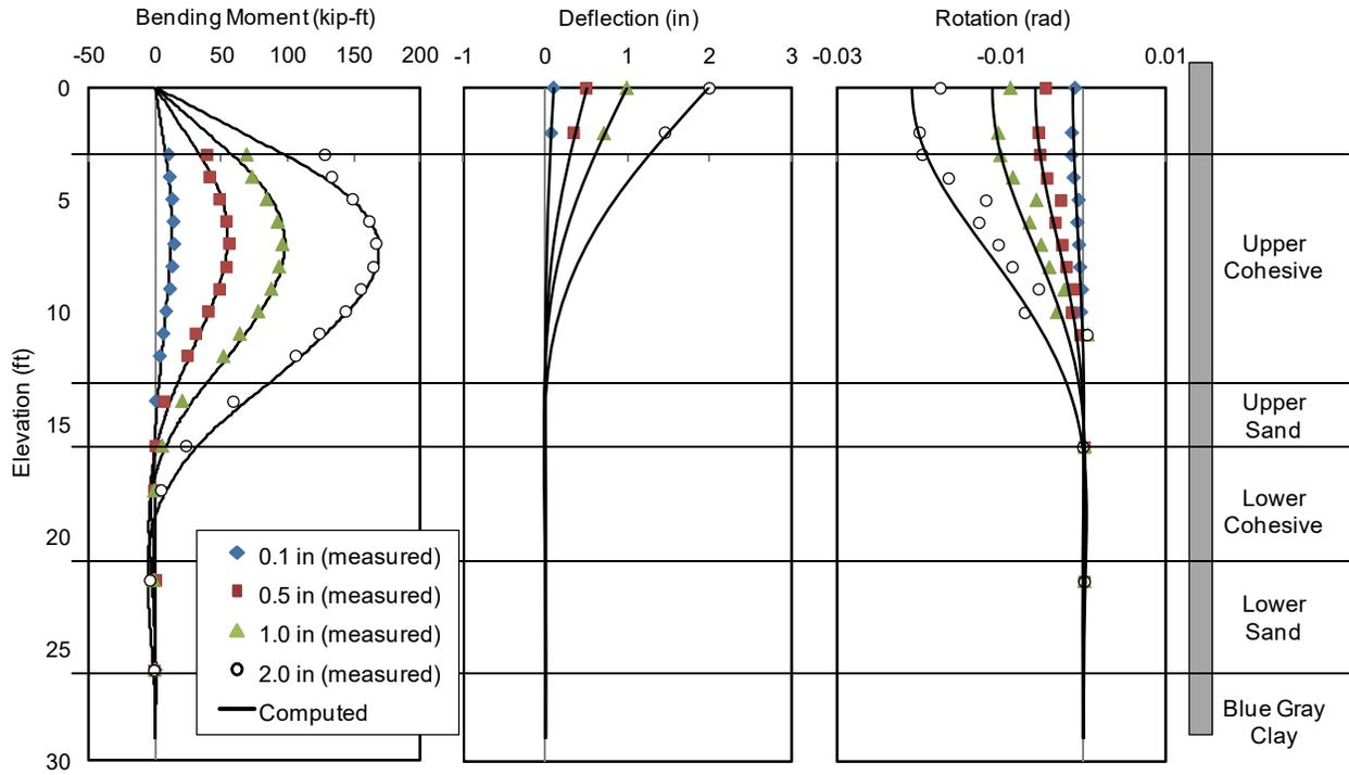
**Figure 7-12.** Comparison of Test Results and Analysis Using Back-Calculated  $p$ - $y$  Curves for 4D Pile (I-5) for Pile Head Displacement of 0.1, 0.5, 1.0 and 2.0 in.
