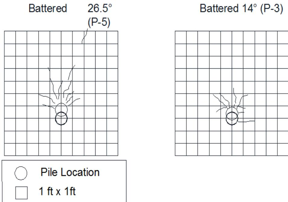
**Figure 10-13** Cracking Patterns for the +26° and +14° battered test piles
