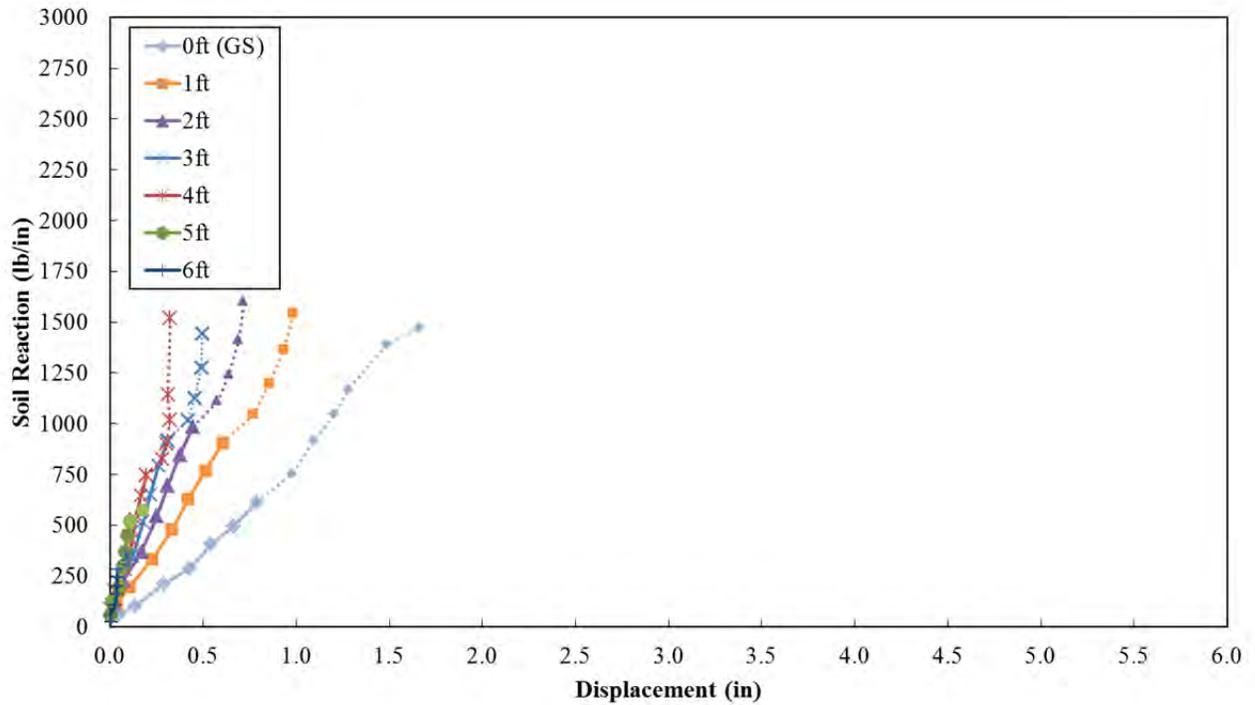
**Figure 12-1** Back-Calculated  $p$ - $y$  Curves for the 2<sup>nd</sup> Baseline Pile (P-2)
