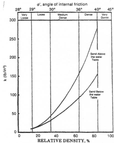
b) Initial Modulus of Subgrade Reaction for API Sand
