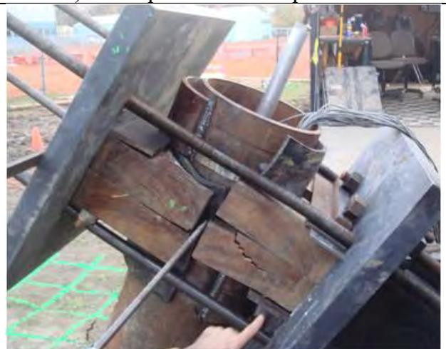
f) Significant cracks on timber spacer blocks
