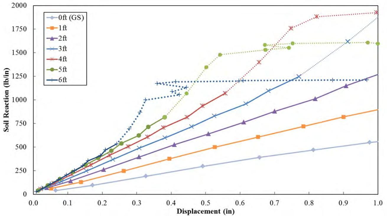
**Figure 12-10** Back-Calculated  $p$ - $y$  Curves for the 2D Pile (P-6) Showing Lower Displacements
