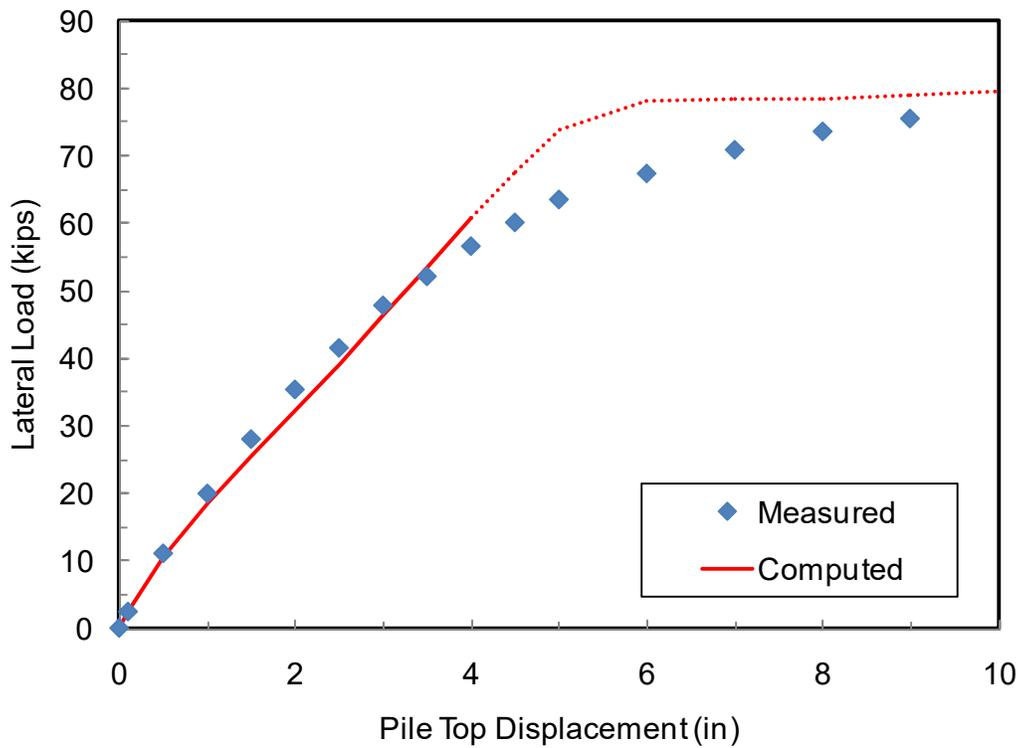
**Figure 7-3.** Comparison of Load-Displacement Curves from Test Results and Analysis Using Back-Calculated  $p$ - $y$  Curves for 8D Pile (I-6)
