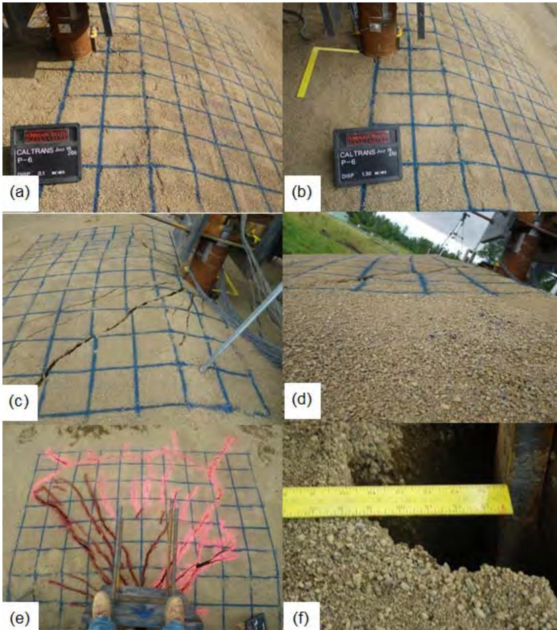
**Figure 10-2** Observations during lateral loading testing of pile P-5 (2D)
