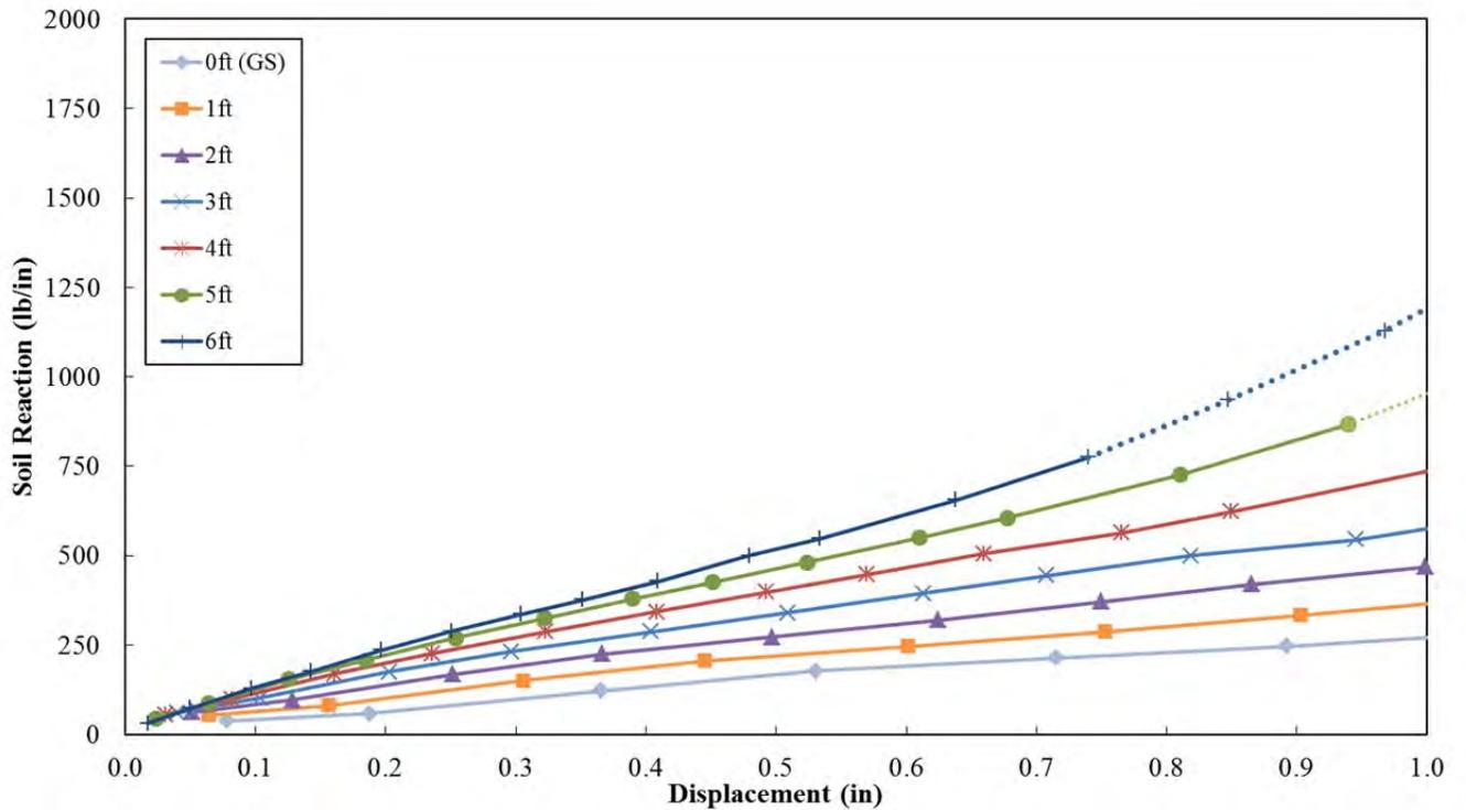
**Figure 12-18** Back-Calculated  $p$ - $y$  Curves for the -4D Pile (P-10) With Lower Displacements
