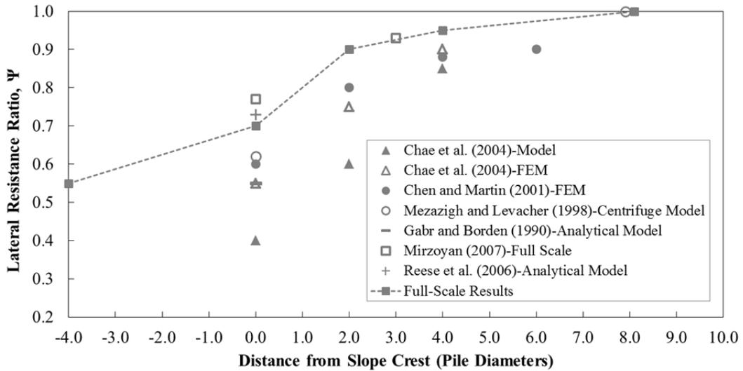
**Figure 13-14** Comparison of resistance ratios presented by researchers as a function of distance from a slope crest with the findings from this study
