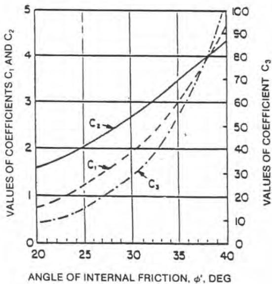
a) Coefficients as Function of  $\phi$  for API Sand
