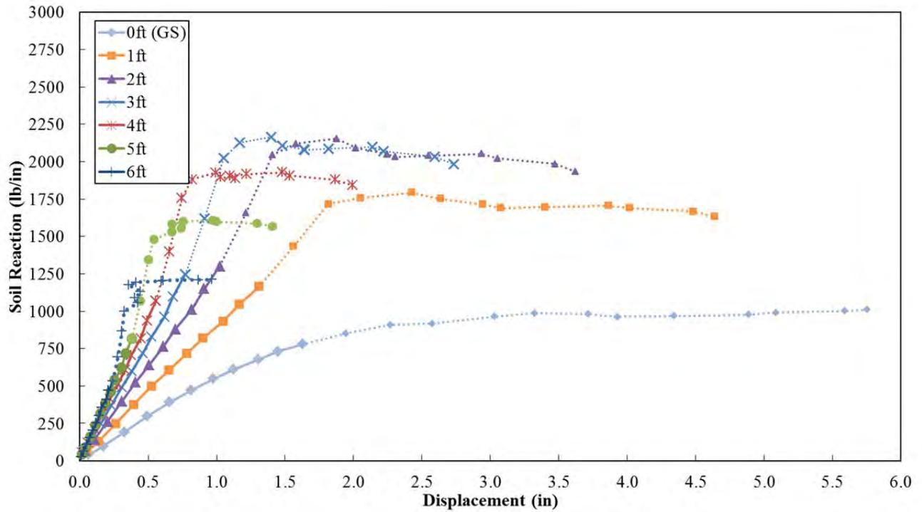
**Figure 12-9** Back-Calculated  $p$ - $y$  Curves for the 2D Pile (P-6)
