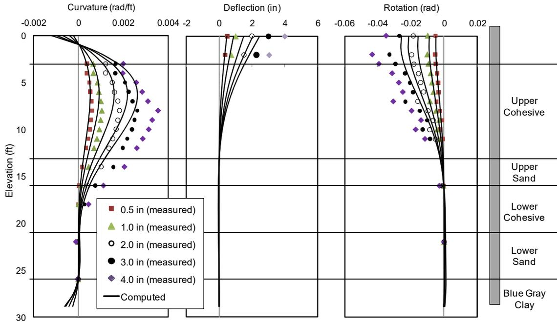
**Figure 9-10** Comparison of Test Results and FEM Analysis for the OD Pile
