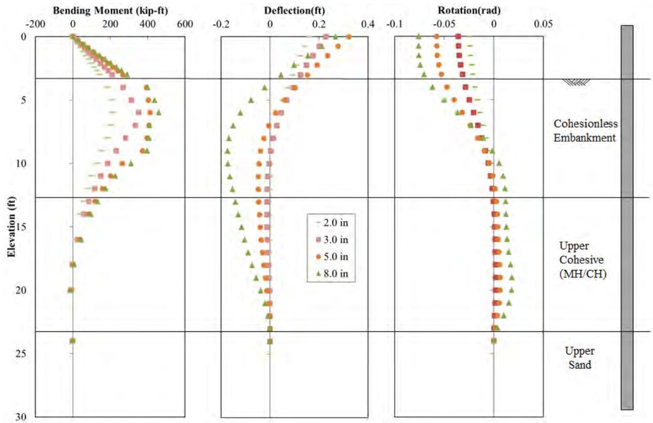
**Figure 12-4** Comparison of Test Results and Analysis Using Back-Calculated  $p$ - $y$  Curves for the 2<sup>nd</sup> Baseline Pile (P-2) for Pile Head Displacement of 2.0, 3.0, 5.0 and 8.0 in.
