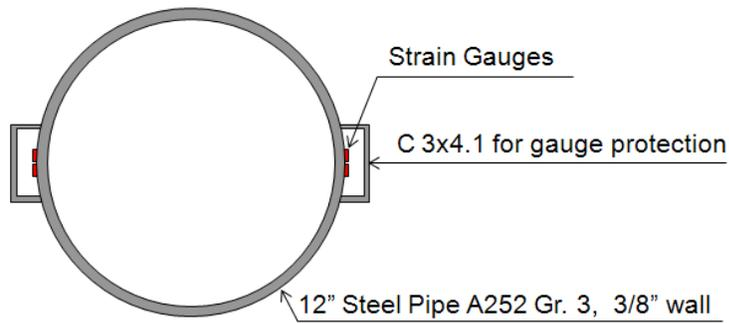
**Figure 4-2.** Geometry of Experimental Test Piles used in all Full-Scale Lateral Load Tests
