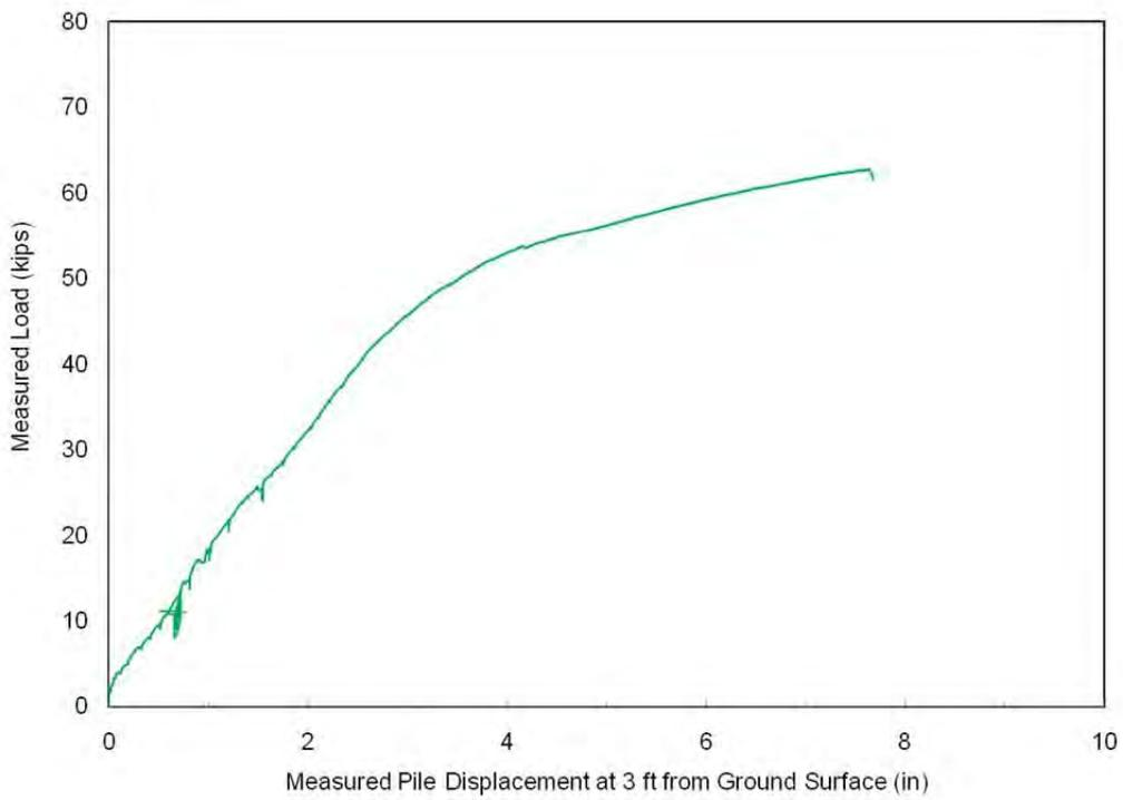
**Figure 6-16.** Load-Displacement Curve for Battered Pile (I-3)
