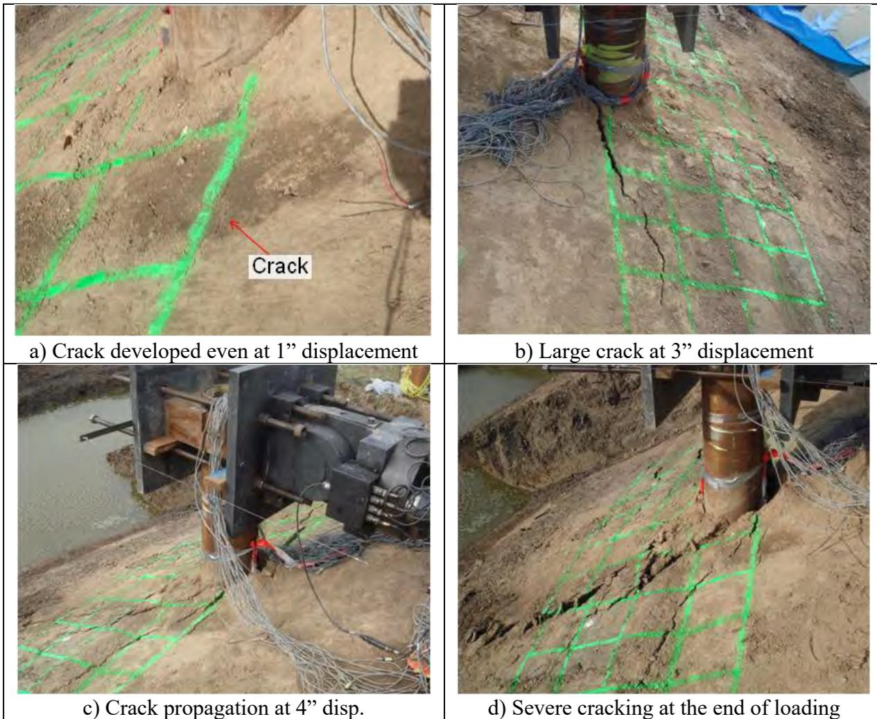
**Figure 5-6.** Observations from Lateral Load Test for -4D Pile (I-8)
