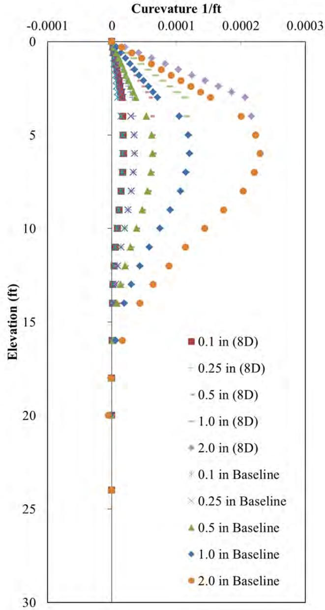
**Figure 11-2** Comparison of Calculated Curvature for 2nd Baseline Pile (P-2) and 8D pile (P-8)
