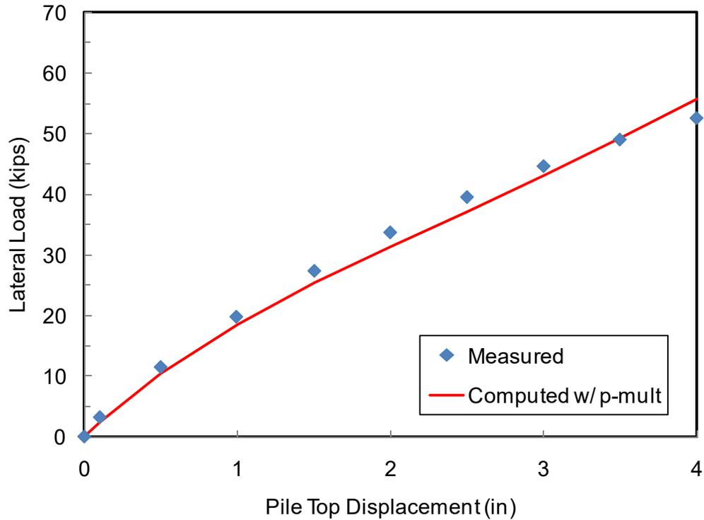
**Figure 7-26.** Comparison of Load-Displacement Curves from Test Results and Analysis Using Proposed Recommendation for 4D Pile (I-5)
