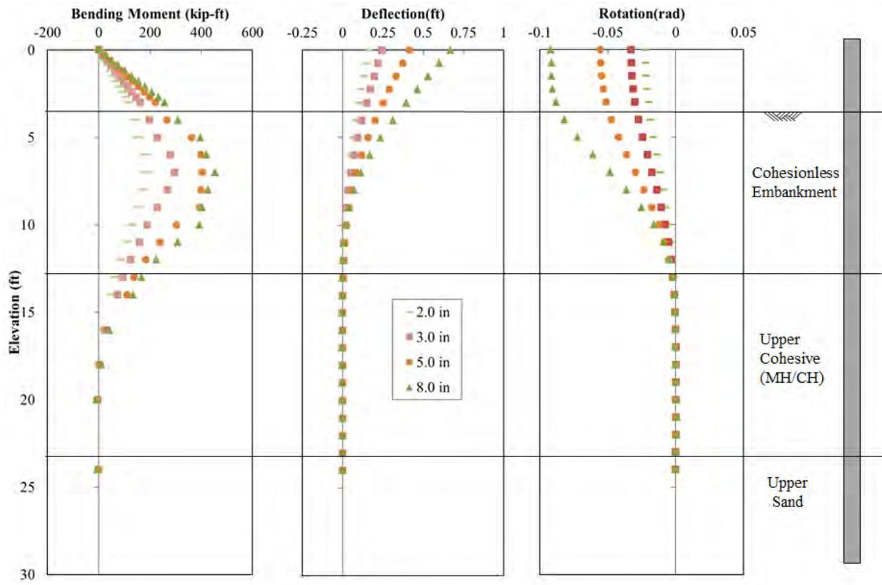
**Figure 12-16** Comparison of Test Results and Analysis Using Back-Calculated  $p$ - $y$  Curves for the OD Pile (P-9) for Pile Head Displacement of 2.0, 3.0, 5.0 and 8.0 in.
