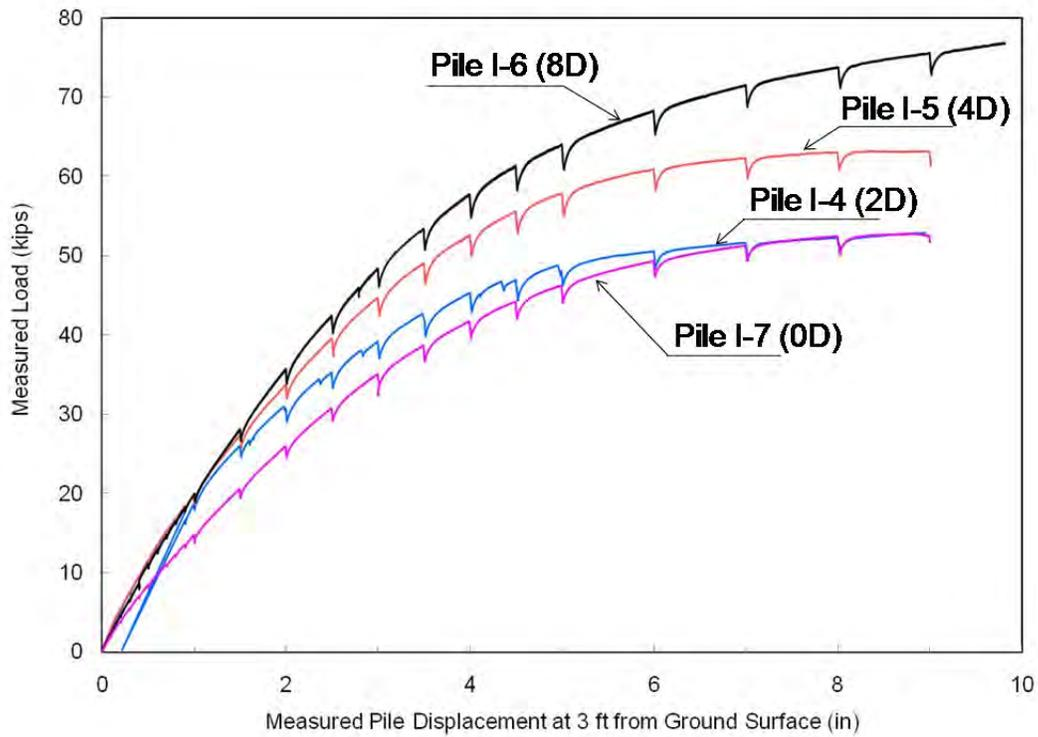
**Figure 6-14.** A Comparison of Load-Displacement Curves for 2D, 4D, 8D and 0D Pile
