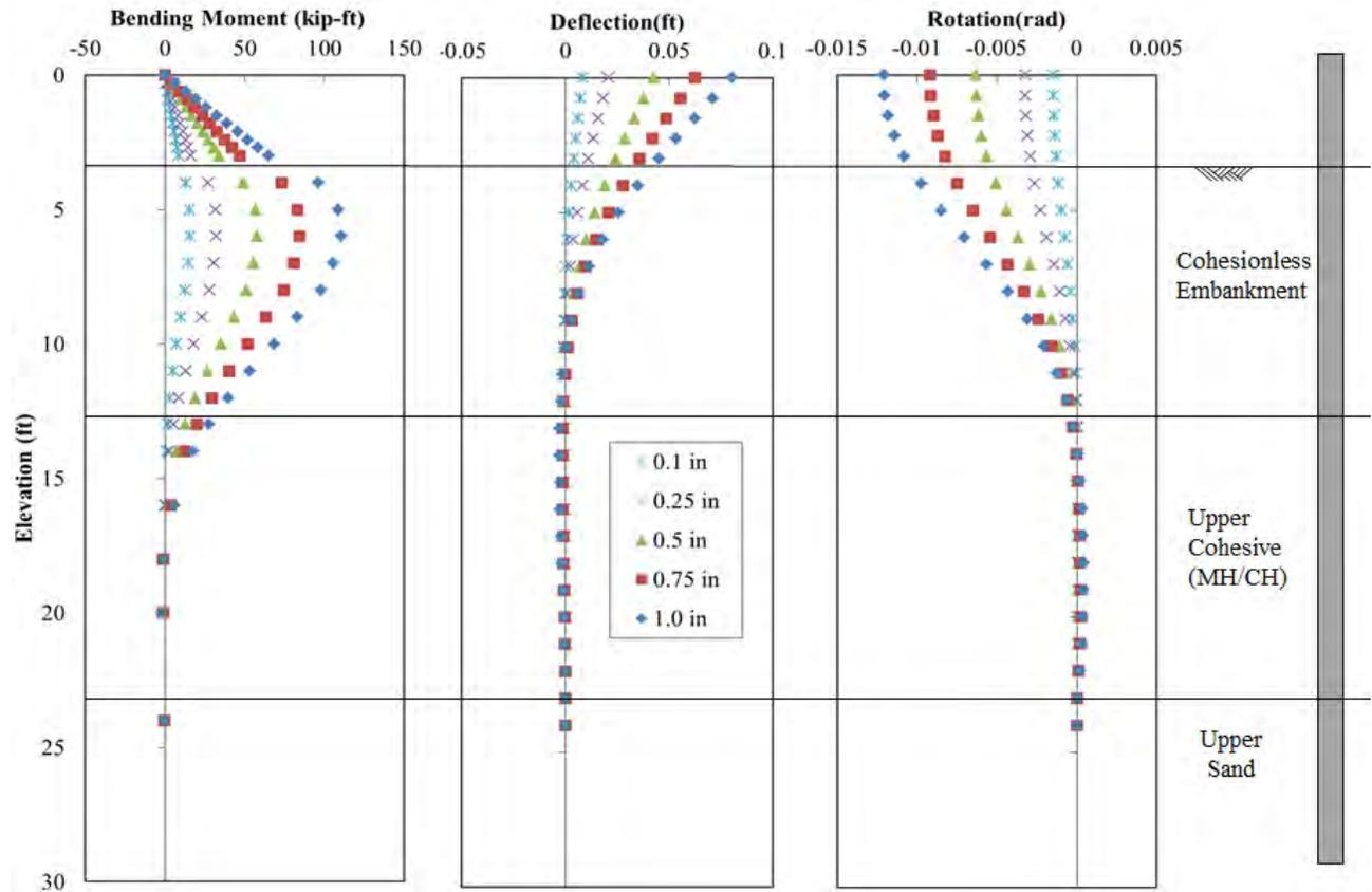
**Figure 12-3** Comparison of Test Results and Analysis Using Back-Calculated  $p$ - $y$  Curves for the 2<sup>nd</sup> Baseline Pile (P-2) for Pile Head Displacement of 0.1, 0.25, 0.5 and 1.0 in.
