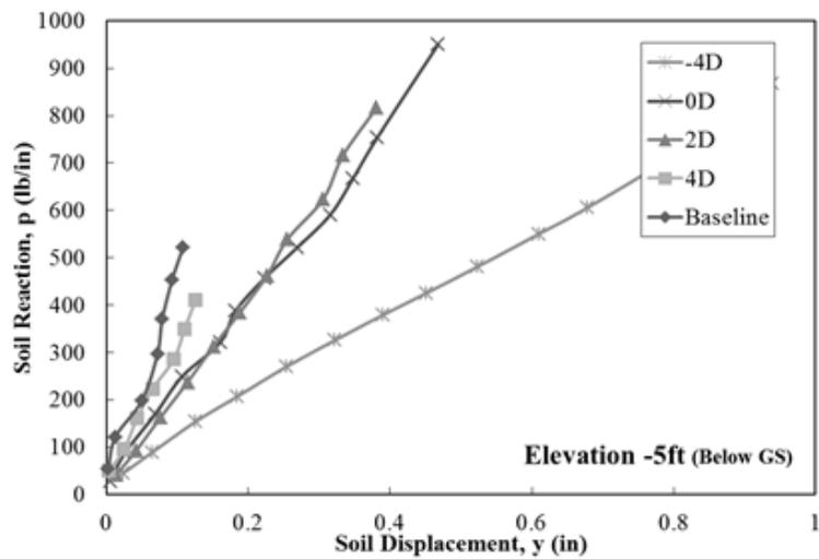
Figure 12-22 Comparison of  $p$ - $y$  Curves for Each Pile at the Same Depth (-2ft to -5ft)
