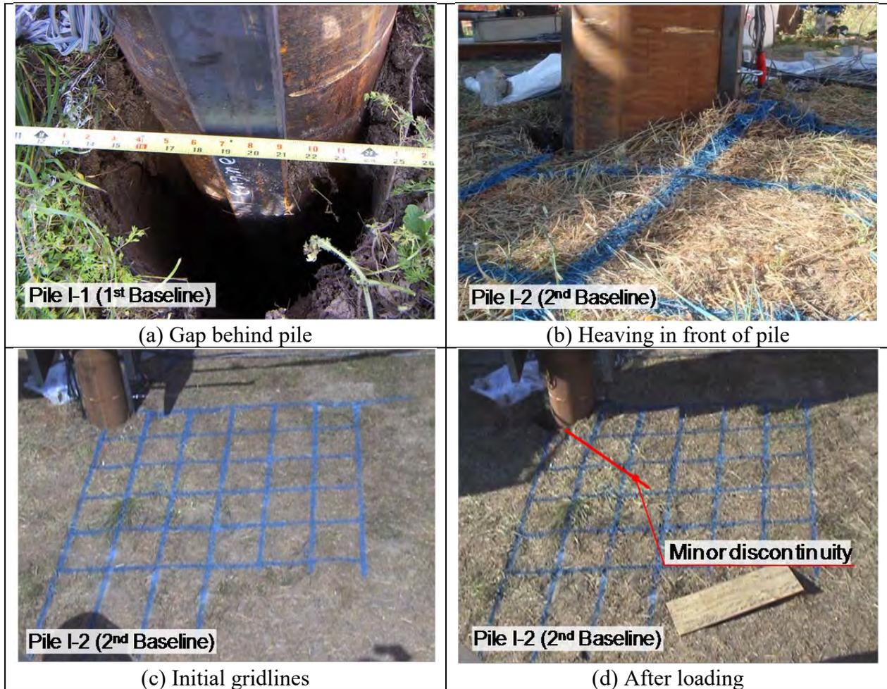
**Figure 5-1.** Observations during Load Test of 1<sup>st</sup> and 2<sup>nd</sup> Baseline Piles (Free Field)
