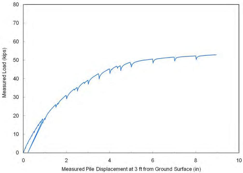
**Figure 6-5.** Load Displacement Curve for 2D pile (I-4)
