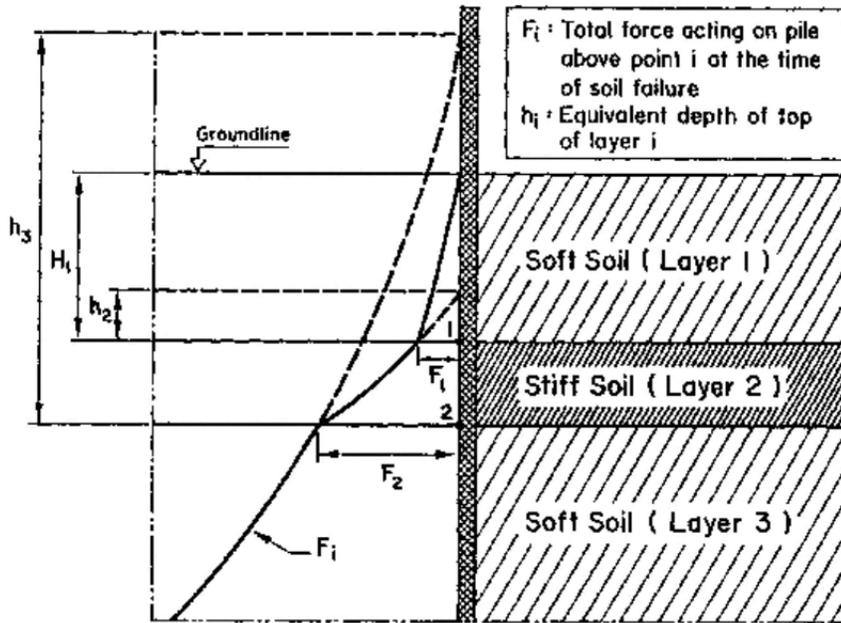
**Figure 2-20** Typical Determination of Equivalent Depths in a Layered Soil Profile (Georgiadis 1983)
