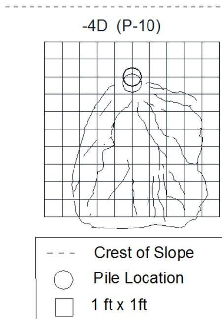
**Figure 10-15** Cracking Patterns for the  $-4D$  (on slope) Pile
