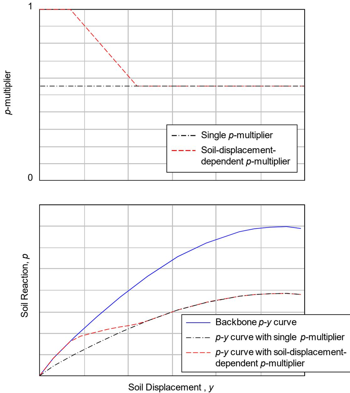
**Figure 7-19.** Concept of Single  $p$ -Multiplier and Soil Displacement Dependent  $p$ -Multiplier
