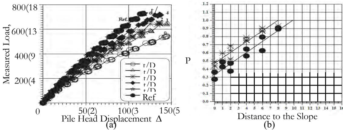
**Figure 2-22** Load Displacement Curves (a) and Recommended  $p_{multi}$  (b) for Centrifuge Tests (after Mezazigh and Levacher 1998)
