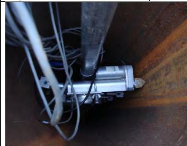
e) Bent actuator rod due to section deformation
