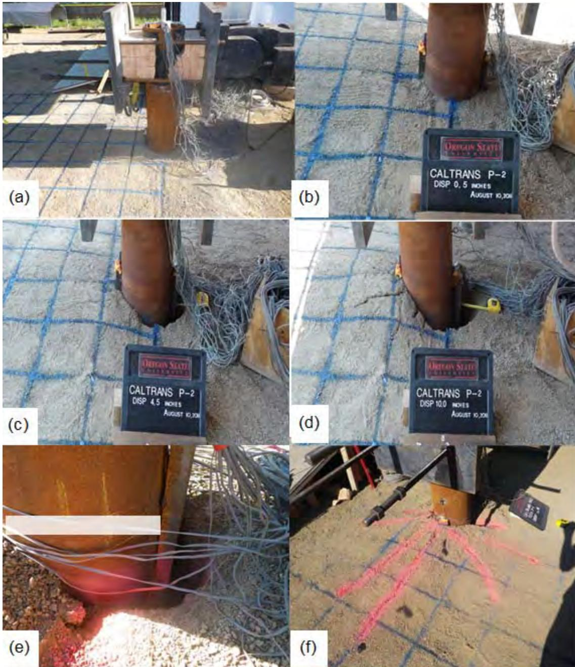
**Figure 10-1** Observations during load test of first and second baseline piles
