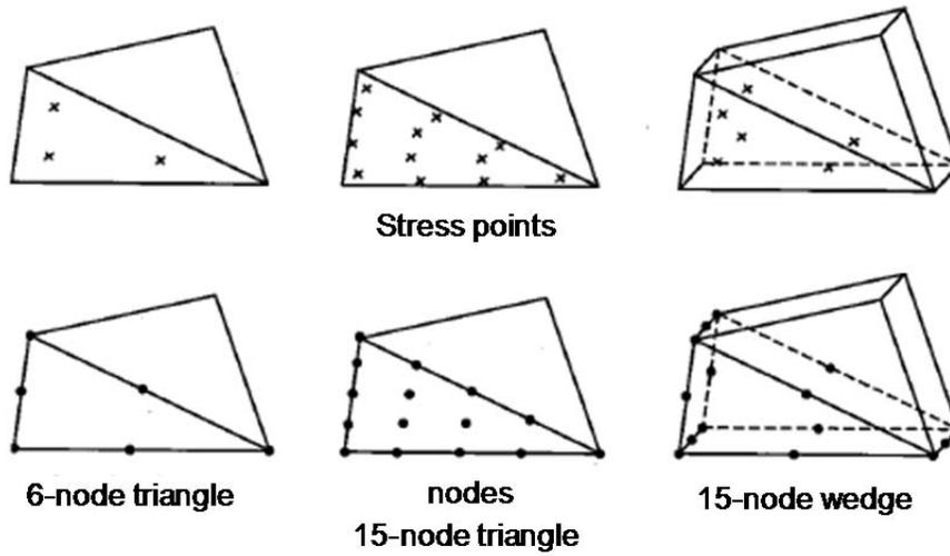
**Figure 9-2** Distribution of Nodes and Stress Points in a 15-Node Wedge Element (after Brinkgreve and Swolfs 2007)
