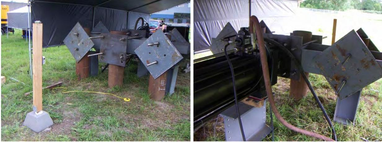
Figure 4-7. Actual test setup – Three-in-a-row Reaction Pile Arrangement
