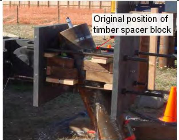
b) Slippage of load stub in the 1<sup>st</sup> test
