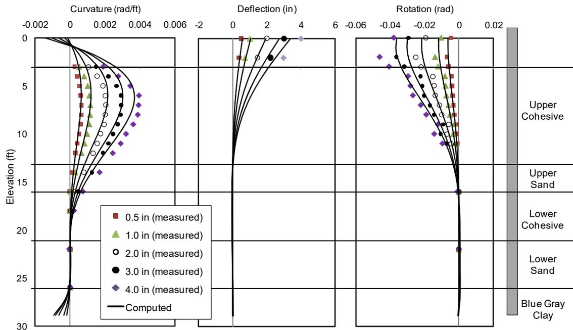
**Figure 9-8** Comparison of Test Results and FEM Analysis for the Baseline Pile
