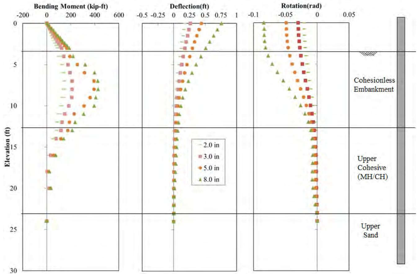
**Figure 12-20** Comparison of Test Results and Analysis Using Back-Calculated  $p$ - $y$  Curves for the -4D Pile (P-10) for Pile Head Displacement of 2.0, 3.0, 5.0 and 8.0 in.
