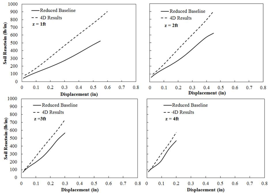
**Figure 13-12** Reduced baseline (with Mezazigh and Levacher (1998) reduction coefficients) and 4D p-y curve comparison
