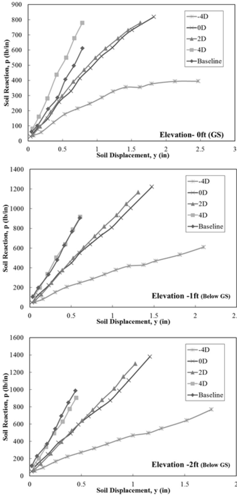
Figure 12-21 Comparison of  $p$ - $y$  Curves for Each Pile at the Same Depth (GS to -2ft)
