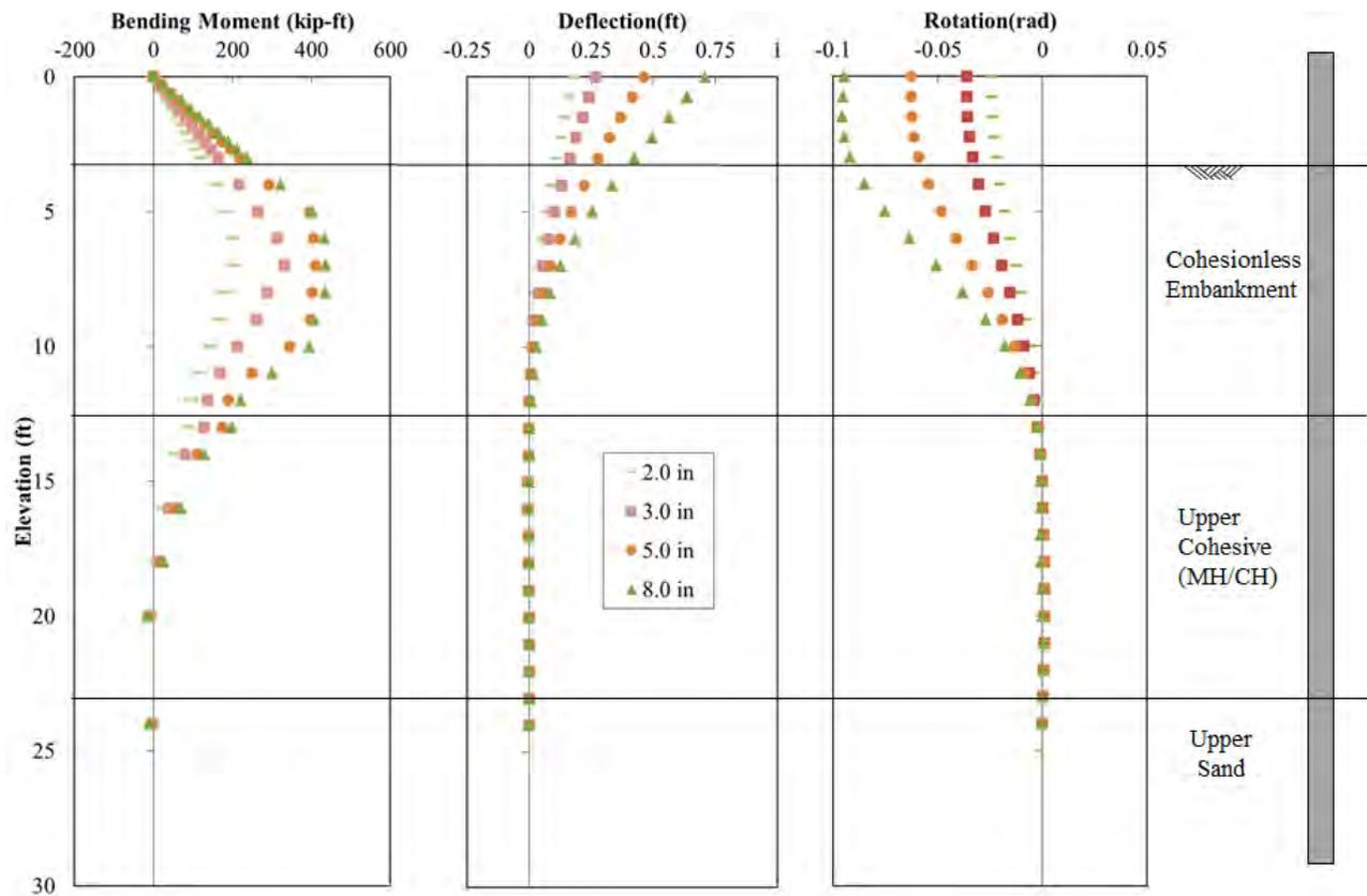
**Figure 12-12** Comparison of Test Results and Analysis Using Back-Calculated  $p$ - $y$  Curves for the 2D Pile (P-6) for Pile Head Displacement of 2.0, 3.0, 5.0 and 8.0 in.
