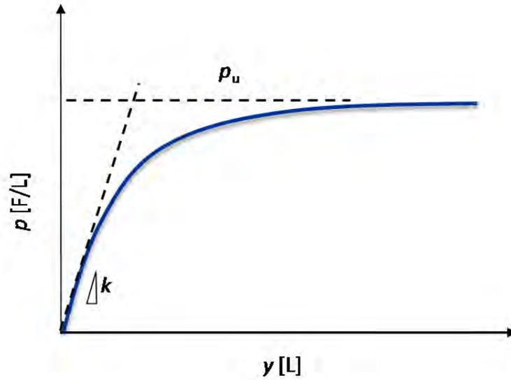
Figure 2-5 Conceptual  $p$ - $y$  Curve for Static Loading
