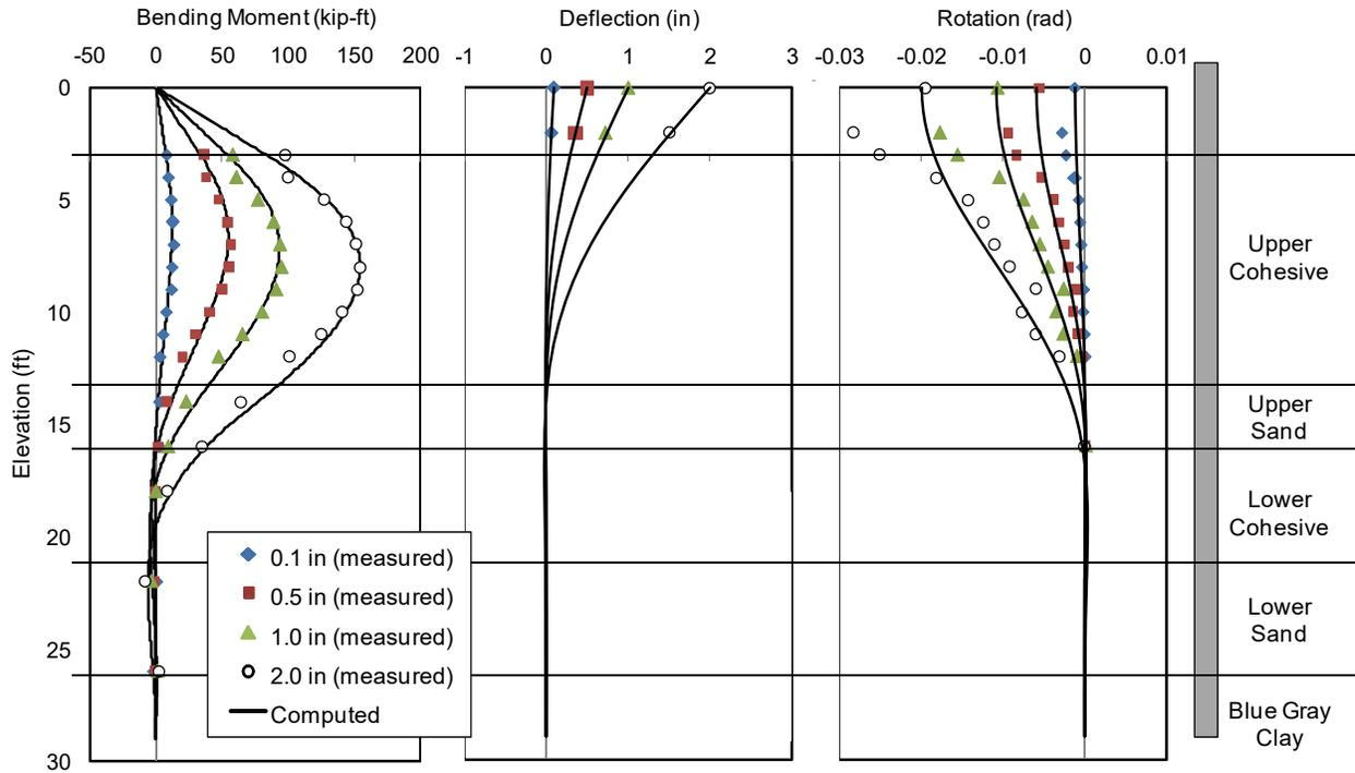
**Figure 7-8.** Comparison of Test Results and Analysis Using Back-Calculated  $p$ - $y$  Curves for 2D Pile (I-4) for Pile Head Displacement of 0.1, 0.5, 1.0 and 2.0 in.
