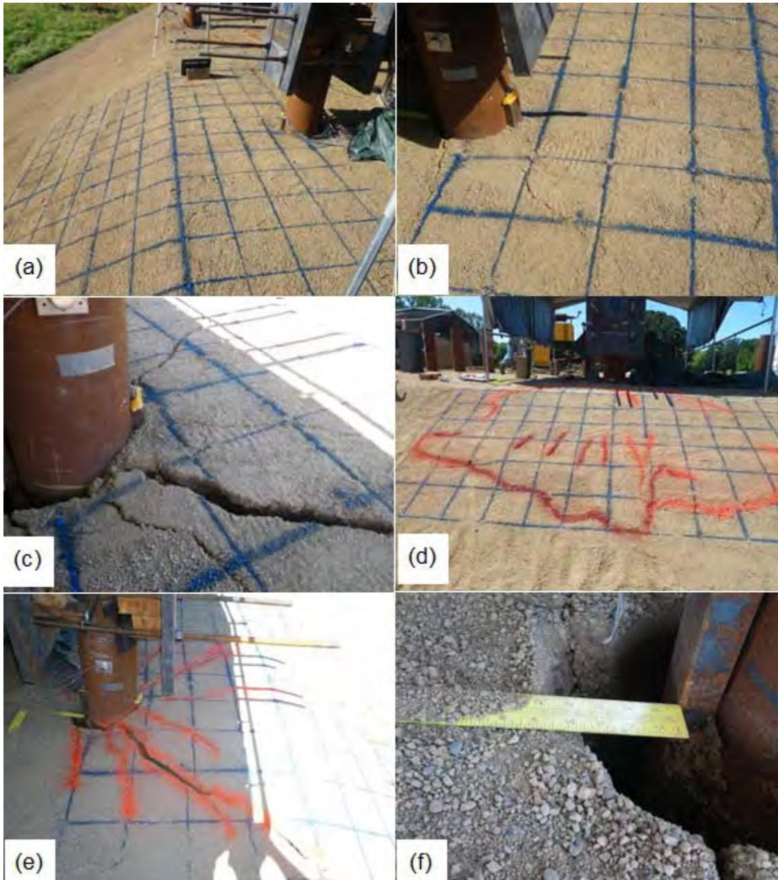
**Figure 10-3** Observations during lateral loading testing of pile P-6 (4D)
