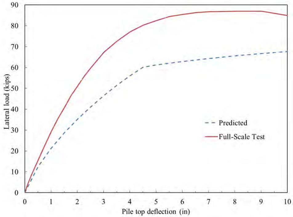
**Figure 13-1** LPILE predicted baseline load-displacement curve with the full-scale test results
