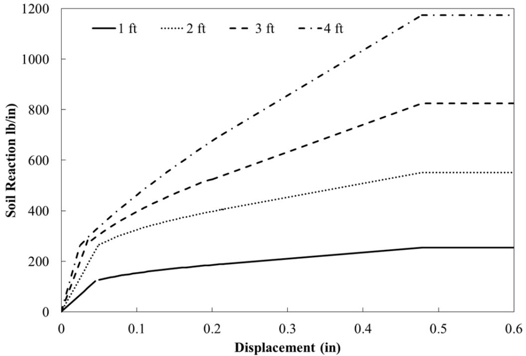
**Figure 13-2** Reese et al. (1974) predicted baseline p-y curves with input soil properties matching the full-scale tests
