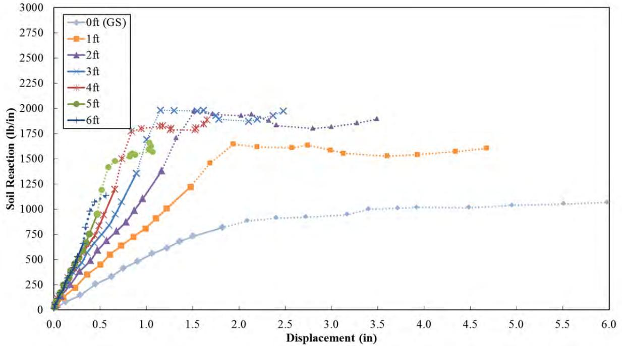
**Figure 12-13** Back-Calculated  $p$ - $y$  Curves for the 0D Pile (P-9) (On Crest)
