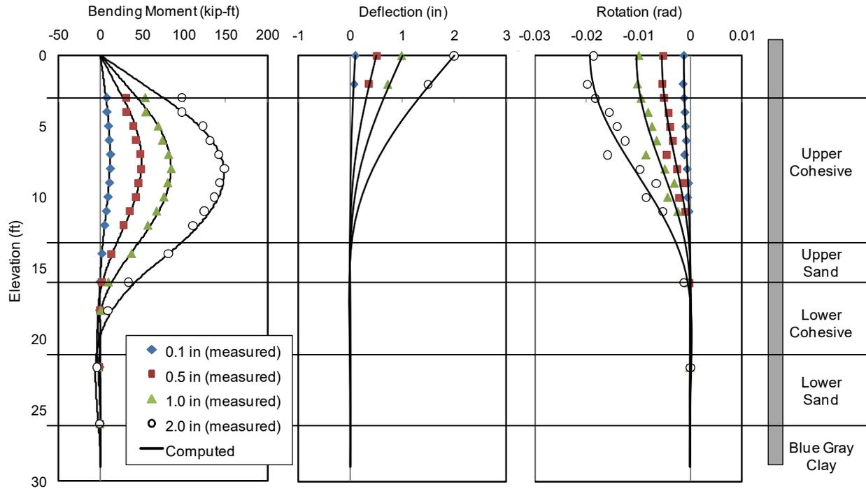
**Figure 7-16.** Comparison of Test Results and Analysis Using Back-Calculated  $p$ - $y$  Curves for OD Pile (I-7) for Pile Head Displacement of 0.1, 0.5, 1.0 and 2.0 in.
