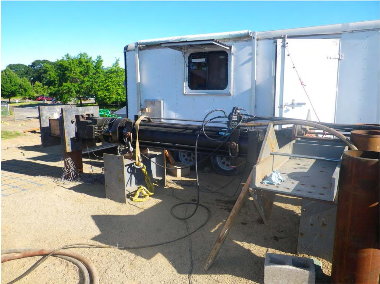
**Figure 4-18.** Top: Constructed Embankment and Test slope Bottom: Test Pile, Reaction Piles, and Hydraulic Actuator Set up
