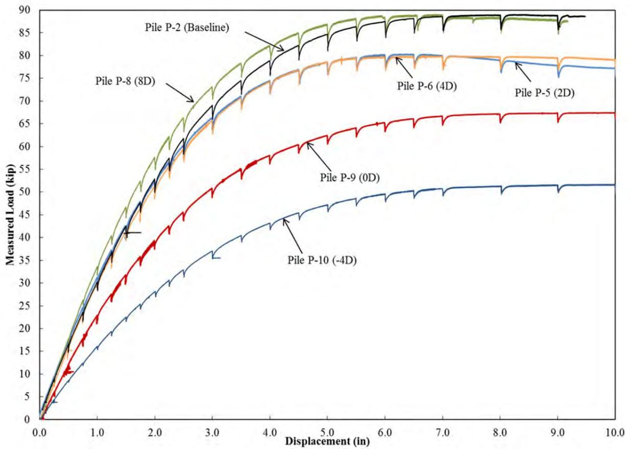
Figure 11-21 Comparison of all Non-Battered Load-Displacement Curves
