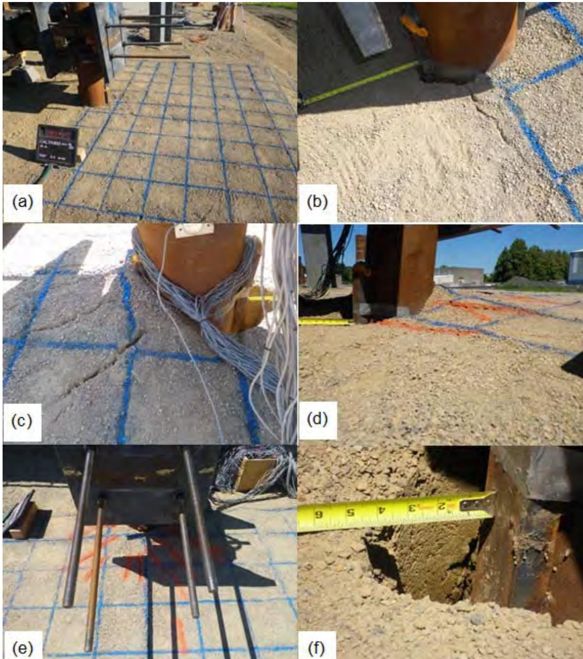
**Figure 10-4** Observations during lateral loading testing of pile P-8 (8D) a) Pile before loading b) Pile at 0.5” of displacement c) Pile at 5.0” of displacement with cracking d) Soil heave at end of testing e) Soil cracking at end of testing f) Gap formation behind pile
