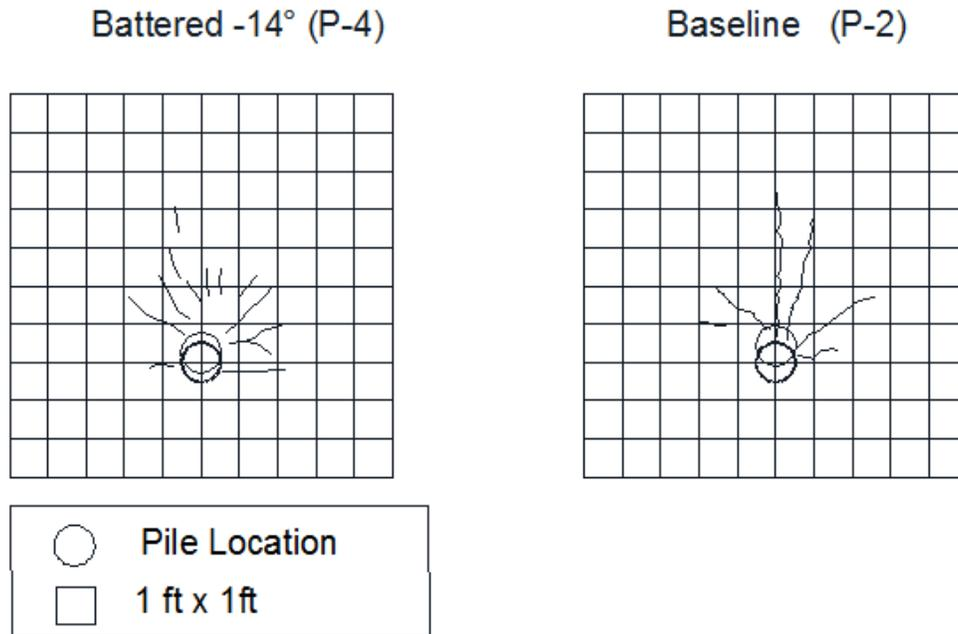
**Figure 10-14** Cracking Patterns for the Baseline and  $-14^\circ$  Battered Piles
