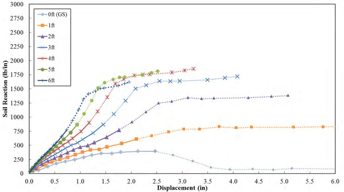
**Figure 12-17** Back-Calculated  $p$ - $y$  Curves for the -4D Pile (P-10) (On Slope)
