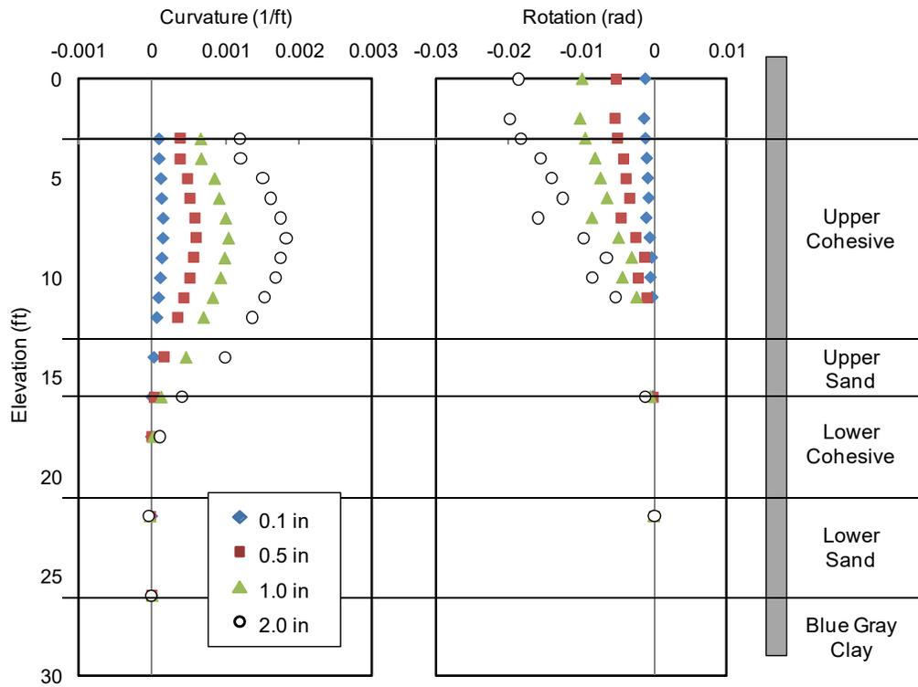
**Figure 6-12.** Test Results of 0D pile (I-7) for Pile Head Displacement of 0.1, 0.5, 1.0 and 2.0 in
