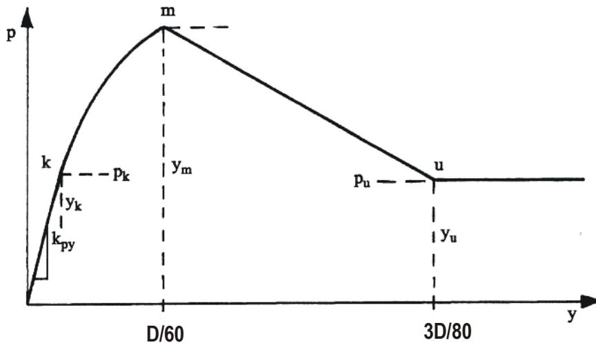
**Figure 2-18** Characteristic Shape of  $p$ - $y$  Curve for  $c$ - $\phi$  Soil (Reese and Van Impe 2001)
