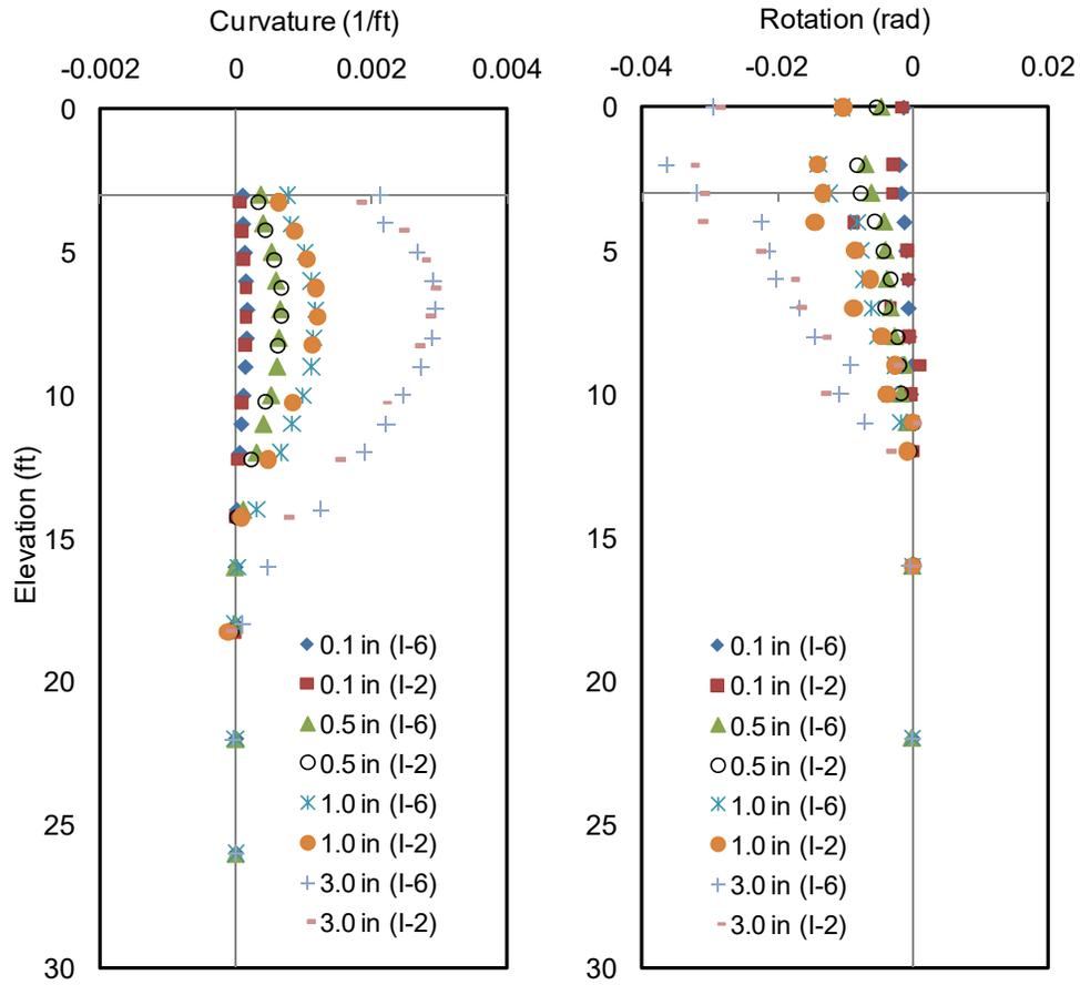
**Figure 6-2.** A Comparison of Calculated Curvature and Measured Rotation for 2<sup>nd</sup> Baseline Pile (I-2) and 8D pile (I-6)
