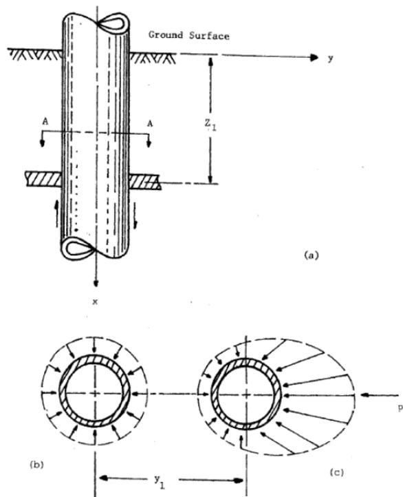
**Figure 2-2** Distribution of Soil Pressure against the Pile before and after Lateral Loading: a) Elevation View of Pile; b) Soil Pressure at Rest; c) Soil Pressure after Lateral Loading (after Reese *et al.* 2006)
