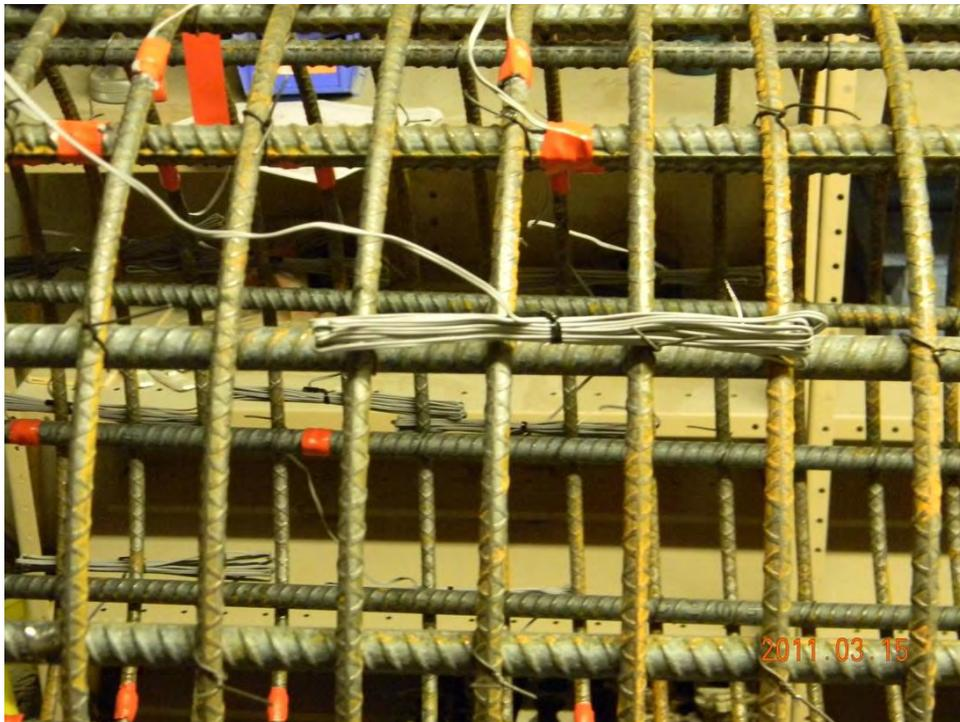
**Figure 4.5.2. Column Reinforcement Instrumented with Strain Gauges**
