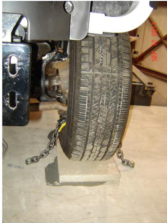
**Figure 4.6.7. Wheel Restraint**
