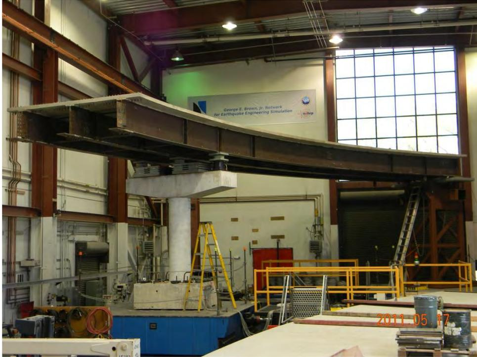
**Figure 4.5.13. North Segment of Superstructure in Place**
