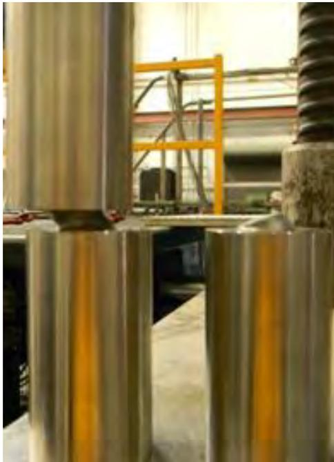
**Figure 4.4.5. Left: Plastic Shear Distortion in Shear Pin
