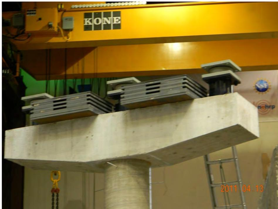
**Figure 4.5.10. Added Weight, Load Cells, and Bearings on a Bent Cap**
