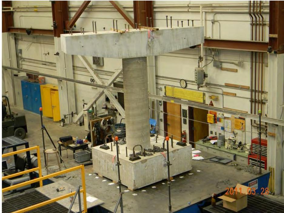
**Figure 4.5.9. Single-Column Bent on Shake Table**
