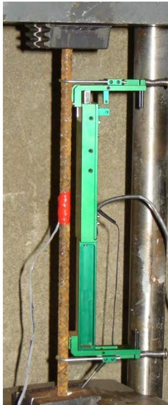
**Figure 5.2.2. Typical Steel Tension Test**
