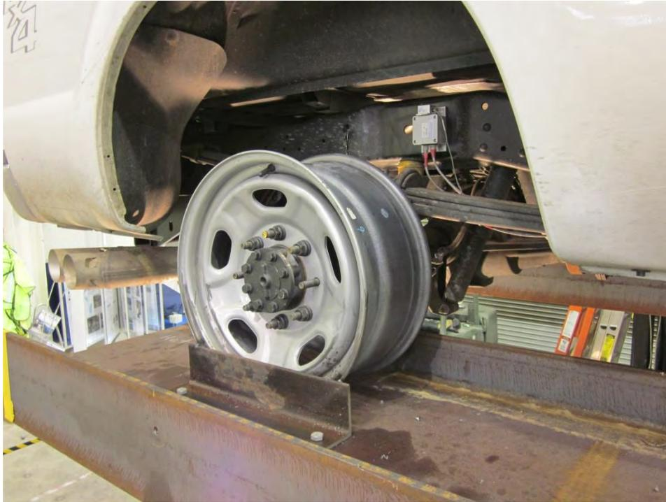
**Figure 3.3.5. Restraint System for Truck without Tires**
