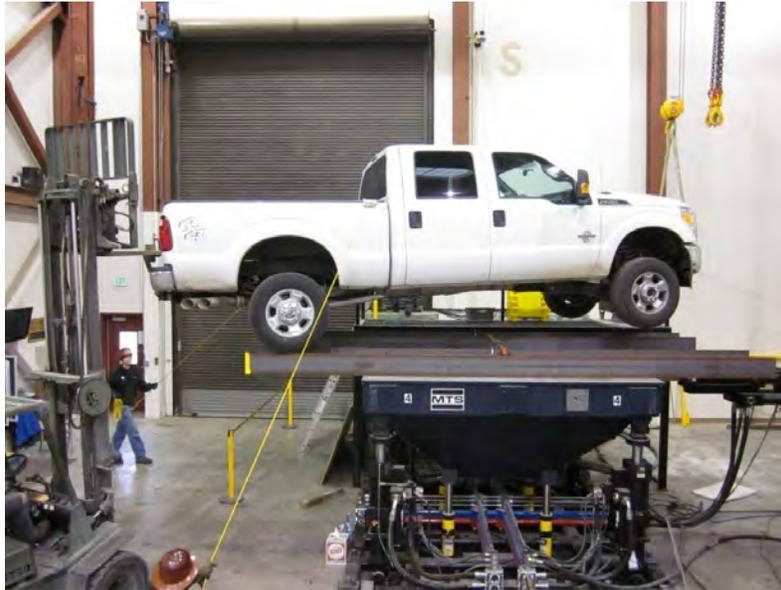
**Figure 3.3.3. Truck Placement on Shake Table**
