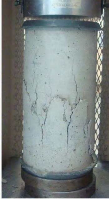
**Figure 5.2.1. Typical Concrete Compression Test**
