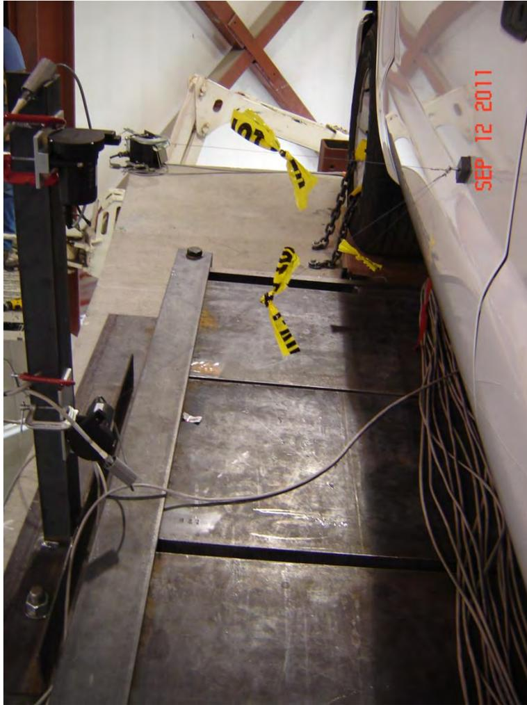
**Figure 4.6.11. Displacement Transducers Attached to Door of TR6**
