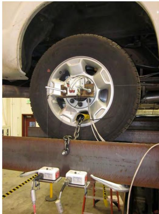
**Figure 3.3.4. Instrumentation of Rear Axle Note Restraint System for Truck with Tires**
