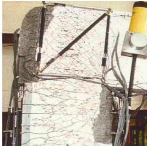
Figure 6-4. Damage state 4
