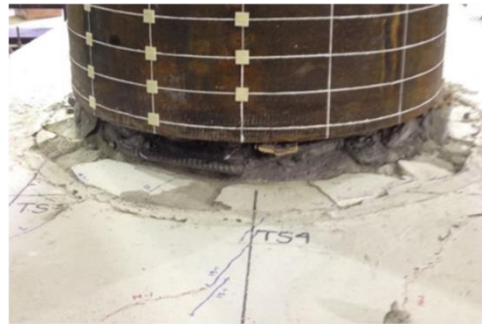
(c) 11.25% Drift (spalled grout removed)
