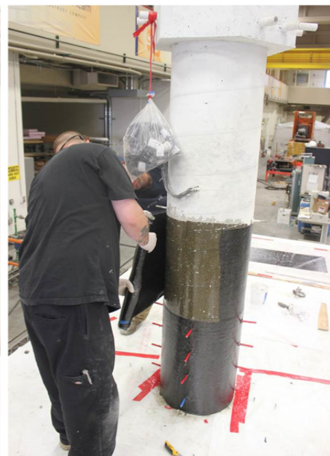
Figure 3.4 Applying the first CFRP layer of (a) the lower part of the jacket and (b) the upper part of the jacket of the column using the ready CFRP wet rolls.
