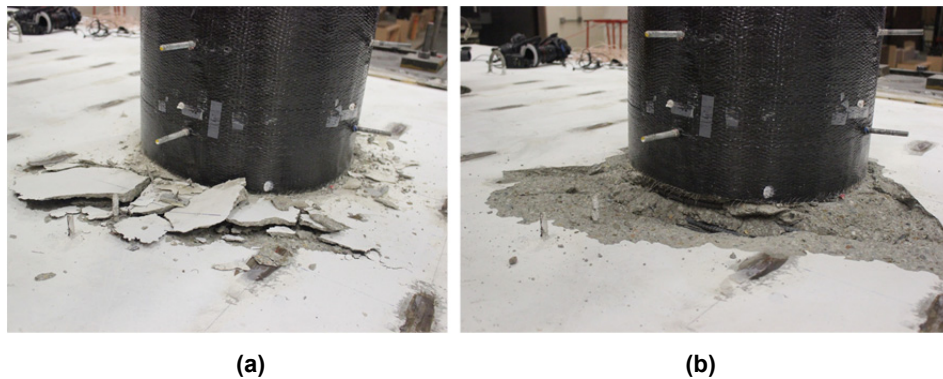
Figure 3.7 Damaged state of Specimen No. 2 (a) after all HS tests and (b) final view of this damage state after all loose concrete were removed.
