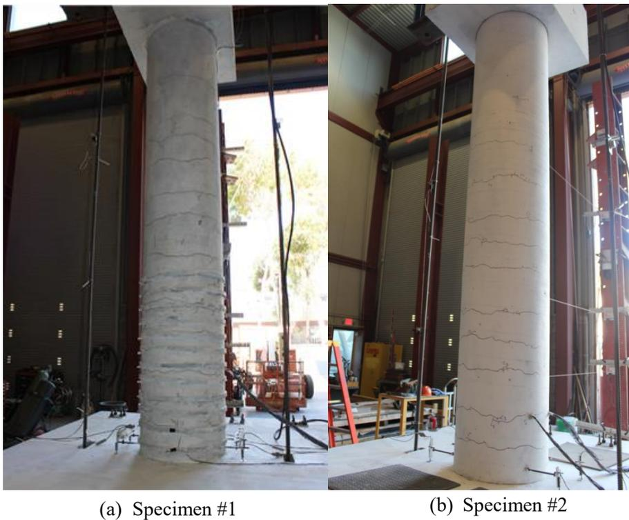
Figure 4.4 – Flexural cracks at the south face of the columns of Specimens #1 and #2 at Cycle 4 (1<sup>st</sup> yield)
