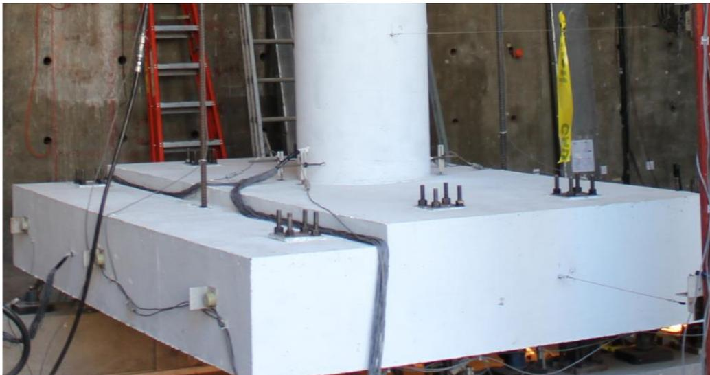
Figure 3.4 – Slab with drop cap in Specimen #3
