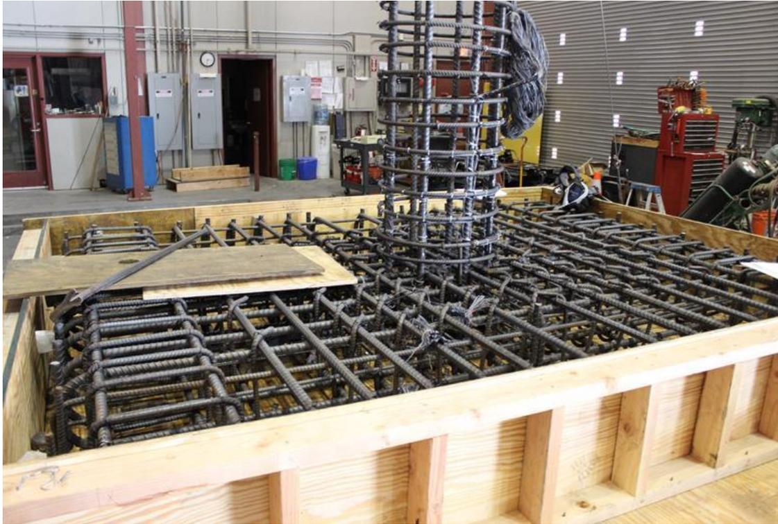
Figure 3.9 – Picture of the slab and column reinforcement of Specimen #1 prior to cast
