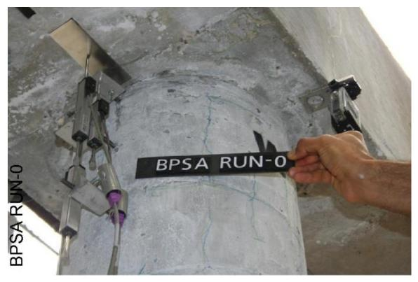
Fig. 3-15. BPSA ECC shrinkage cracks in CIP column before test
