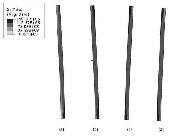
Fig. 18. Von Mises stress (psi) in the rods, South direction: (a) CIP (b) PC, North direction: (c) CIP (d) PC
