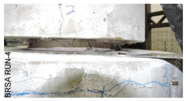
Fig. 3-95. BRSA CIP rebar-pin after Run-4 a) E view b)W view
