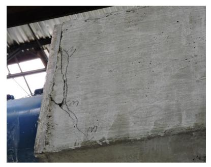
Fig. 3-30. BPSA crack formation at load cell connection after Run-3
