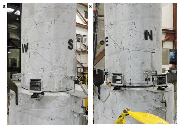
Fig. 3-24. BPSA CIP pipe-pin after Run-8 a) SW view b) NE view
