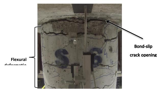
Fig. 4-8. Bond-slip rotation CIP column of BRSA during Run-5
