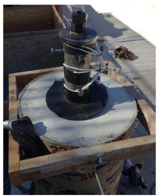
Fig. 2-22. Pipe-pin after placing the bearing pad and top pipe
