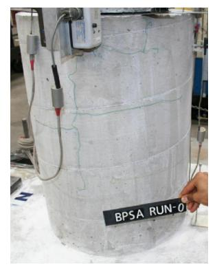
Fig. 3-32. BPSA shrinkage cracks on PC pedestal prior to tests
