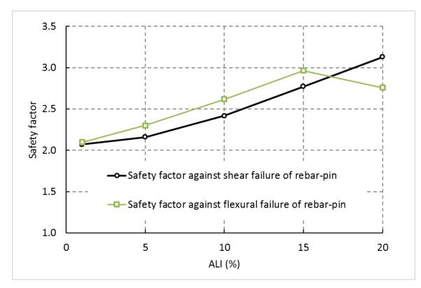
Fig. 5-51. Effect of ALI on the safety factors against shear and flexural failure
