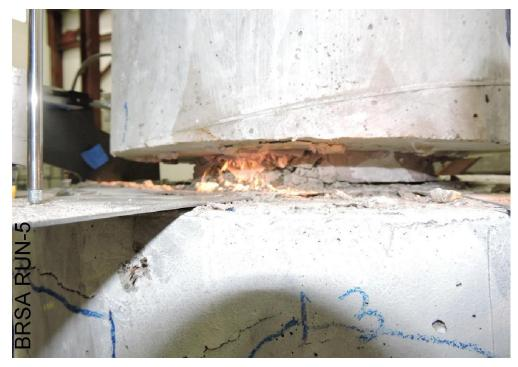
Fig. 3-97. BRSA CIP rebar-pin after Run-5, NW view
