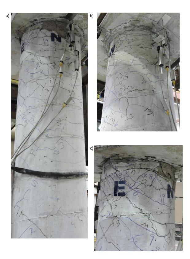
Fig. 3-41. BPSA PC column after Run-9 a) NE view b) SW view c) NE top
