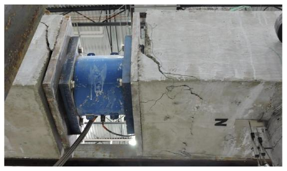
Fig. 3-31. BPSA cap beam condition after load cell failure end of Run-4
