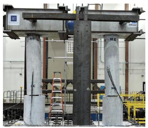
Fig. 11. BRSA final condition after tests
