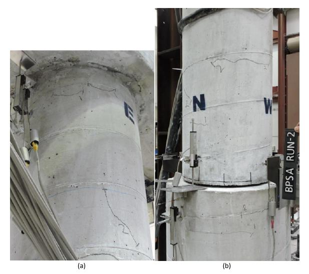
Fig. 3-34. BPSA PC column after Run-2 a) SE view b) NW view
