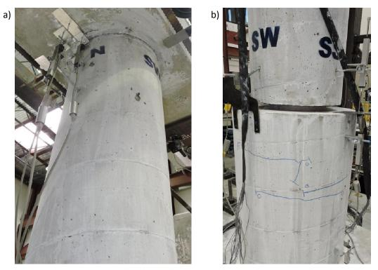
Fig. 3-89. BRSA CIP condition after Run-1 a) column, NW view b) rebar-pin, SW view
