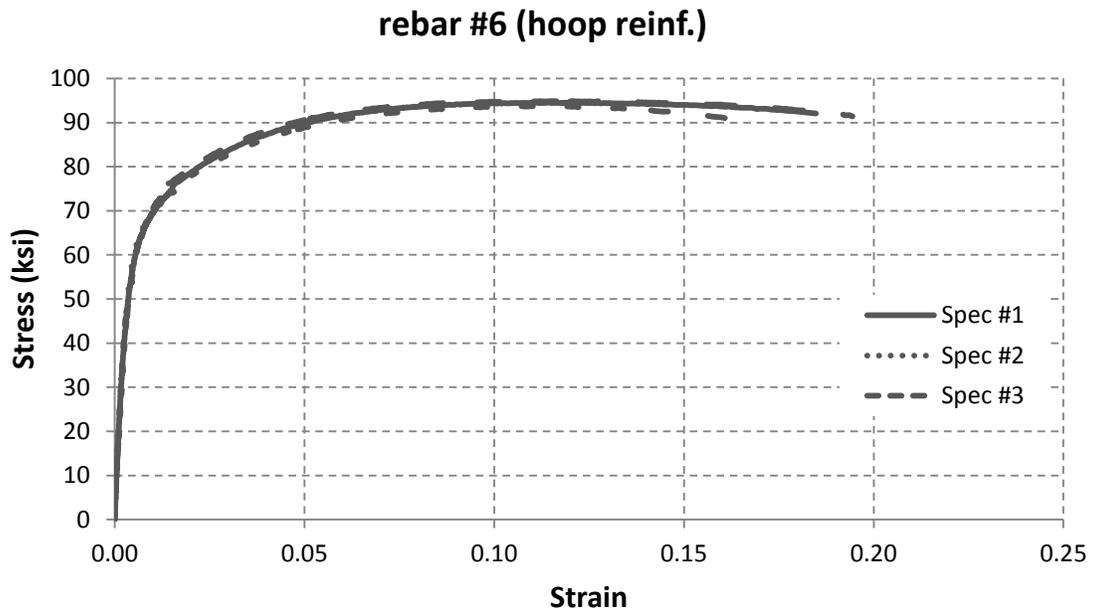
Figure 2.20 – Stress – strain curves for #6 hoop reinforcement
