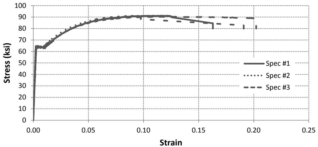
Figure 2.22 – Stress - strain curves for #11 longitudinal reinforcement
