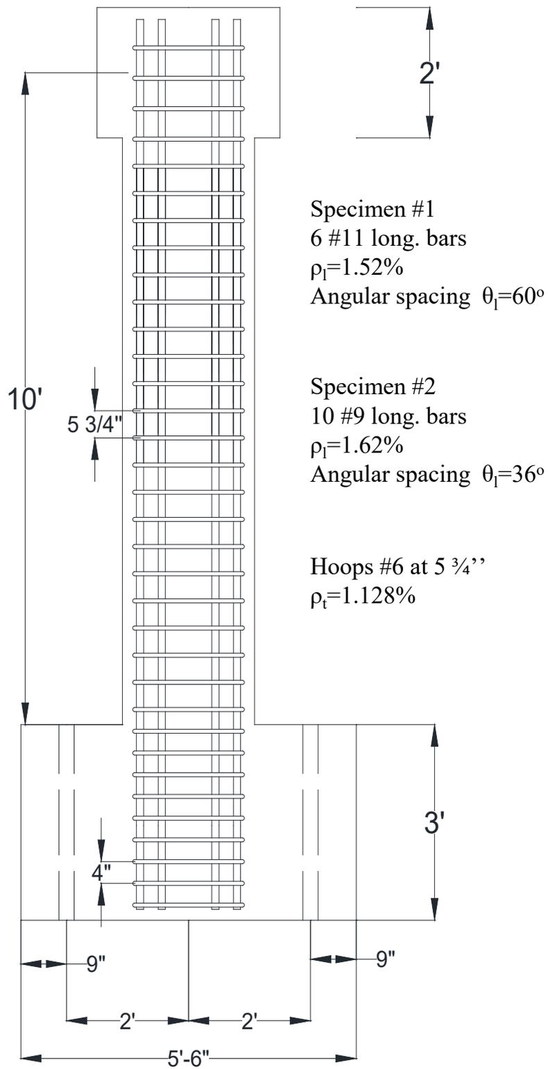
Figure 2.1 - Elevation view of Specimens #1 and #2
