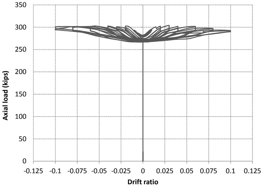
Figure 3.2 – Axial load-vs.-drift ratio plot for Specimen #1
