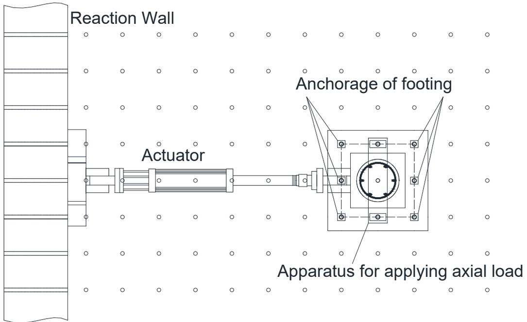
Figure 2.8 - Plan view of test setup
