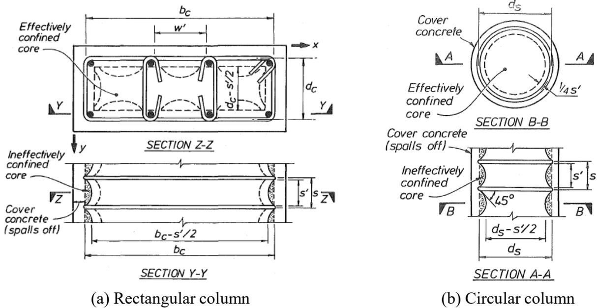
Figure 1.4 – Arching action of confining reinforcement (Mander et al. 1988a)
