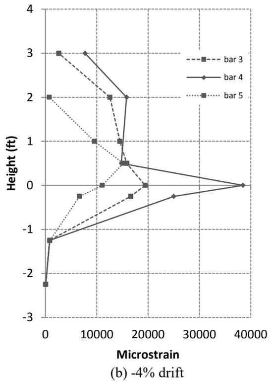
Figure 3.33 - Tensile strains in longitudinal bars of Specimen #2 at 4% drift
