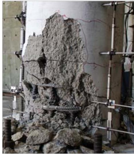
Figure 3.25 – Specimen #2 at the end of testing
