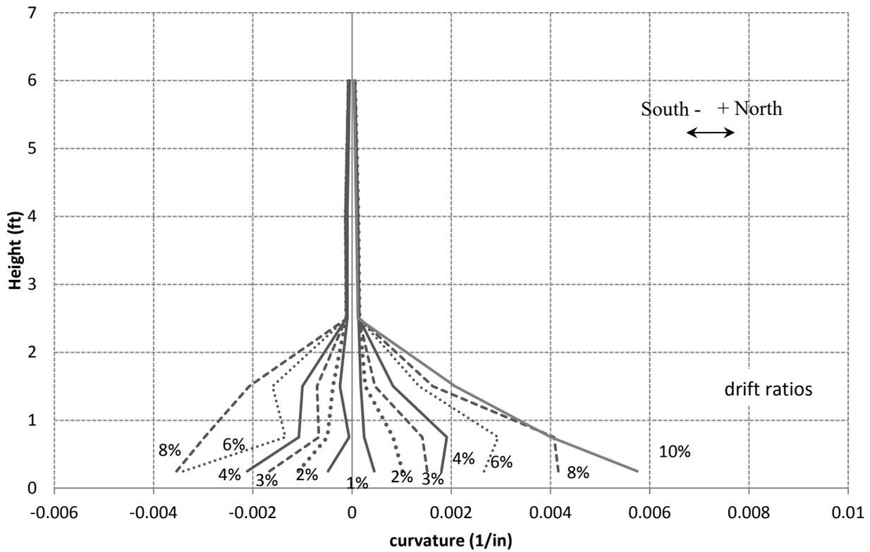
Figure 3.29 – Curvature along the height of Specimen #2
