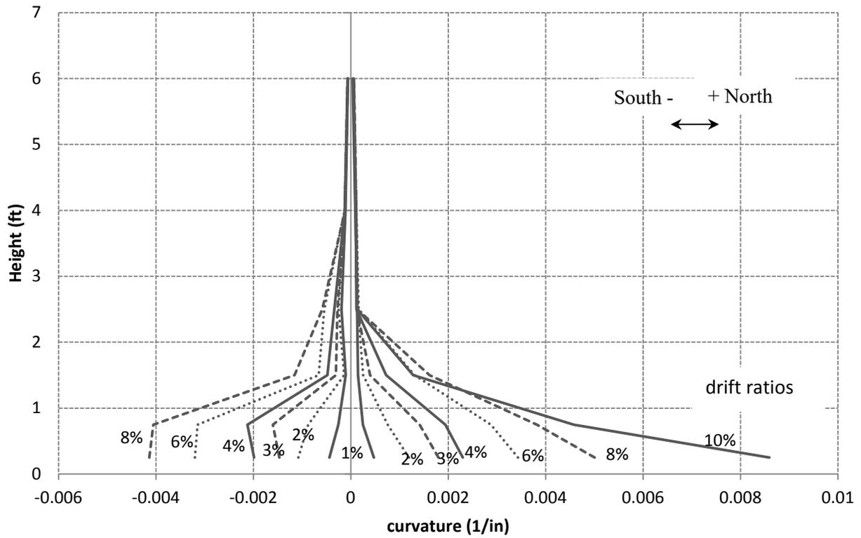
Figure 3.28 – Curvature along the height of Specimen #1
