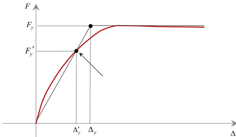
Figure 2.10 – Equivalent elastic-perfectly plastic system
