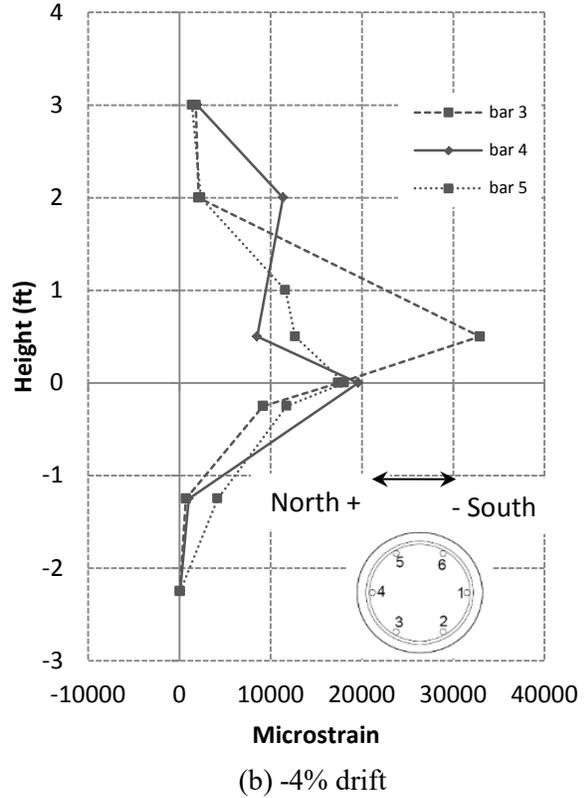
Figure 3.32 - Tensile strains in longitudinal bars of Specimen #1 at 4% drift
