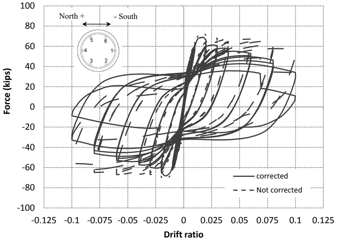
Figure 3.1 – Lateral load-vs.-drift ratio plots for Specimen #1
