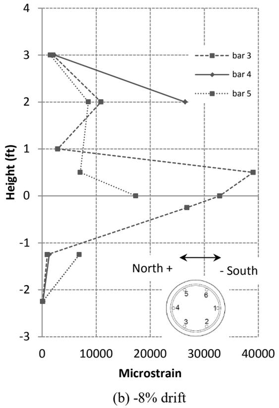
Figure 3.34 - Tensile strains in longitudinal bars of Specimen #1 at 8% drift
