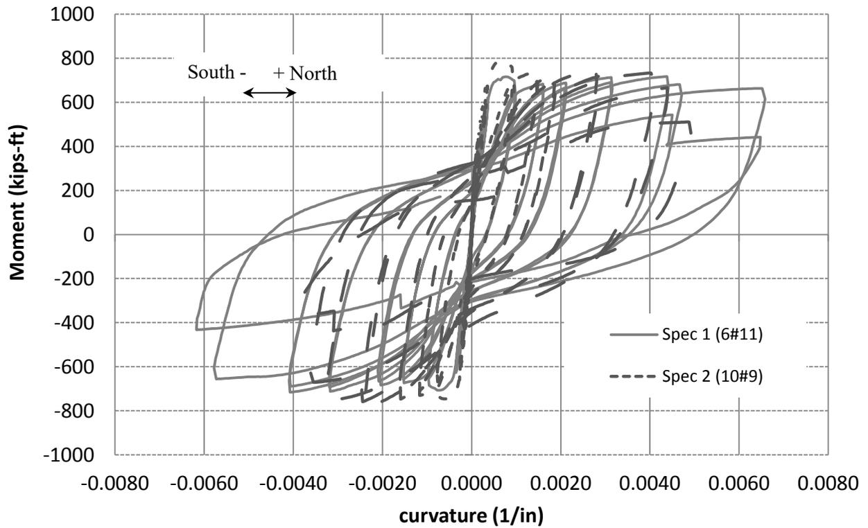
Figure 3.27 – Moment-vs.-curvature curves for Specimens #1 and #2
