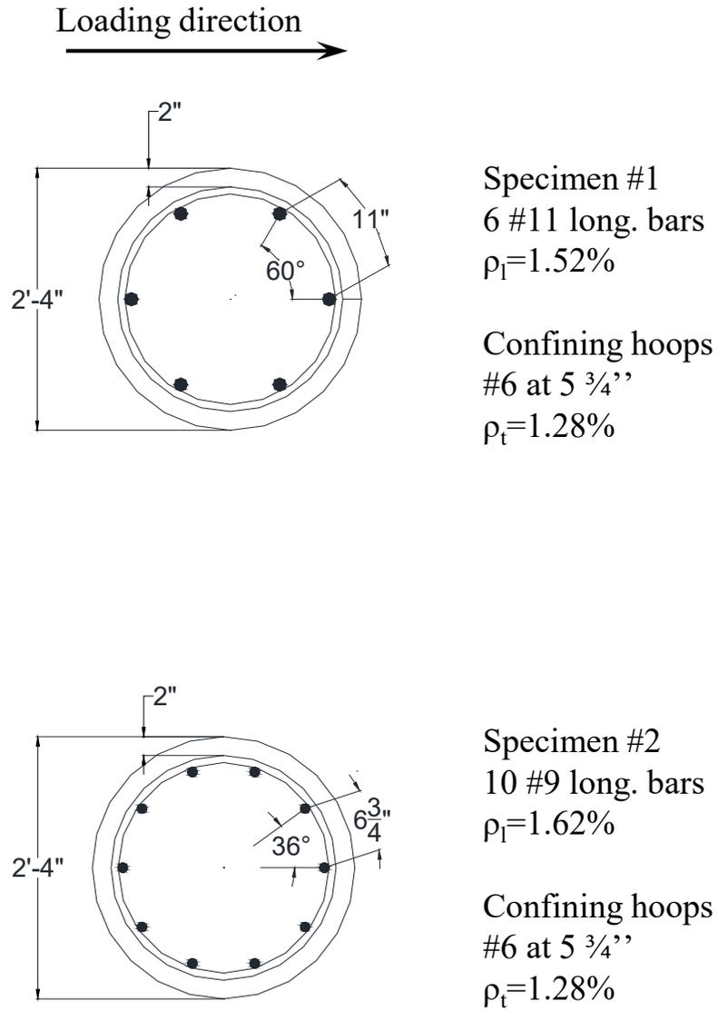
Figure 2.2 – Cross-sections of Specimens #1 and #2
