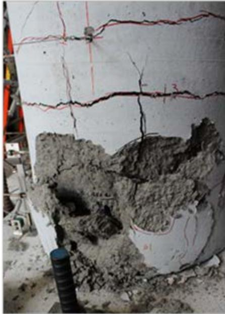
Figure 3.7 – Specimen #1 at 6% drift
