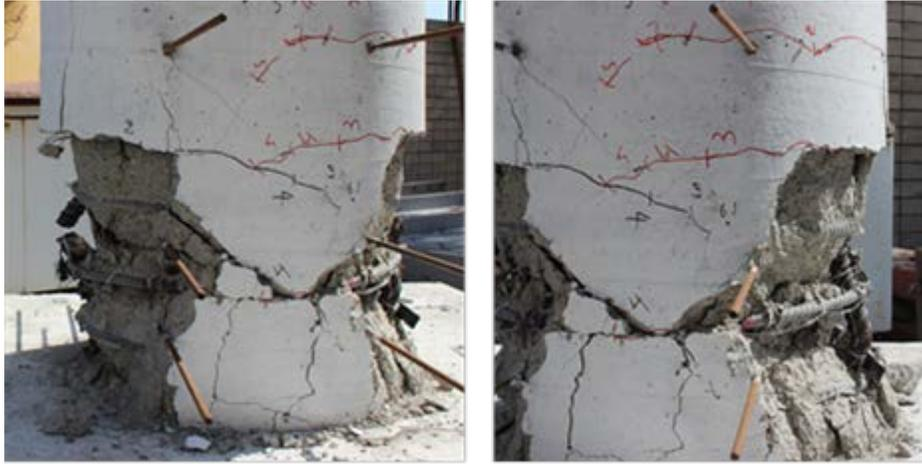
Figure 3.12 – Specimen #1 at the end of testing
