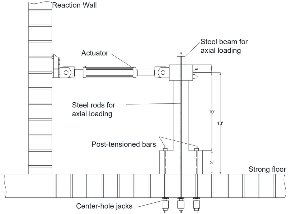
Figure 2.7 - Elevation view of test setup
