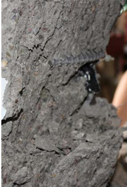
Figure 3.8 – Buckled bar #1 at south face of Specimen #1 during 2<sup>nd</sup> cycle of -8% drift
