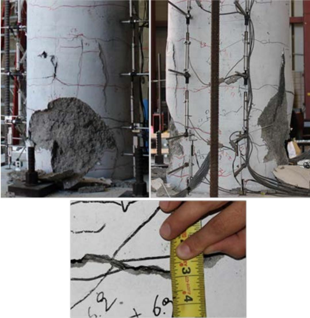
Figure 3.18 - Specimen #2 at 3% drift
