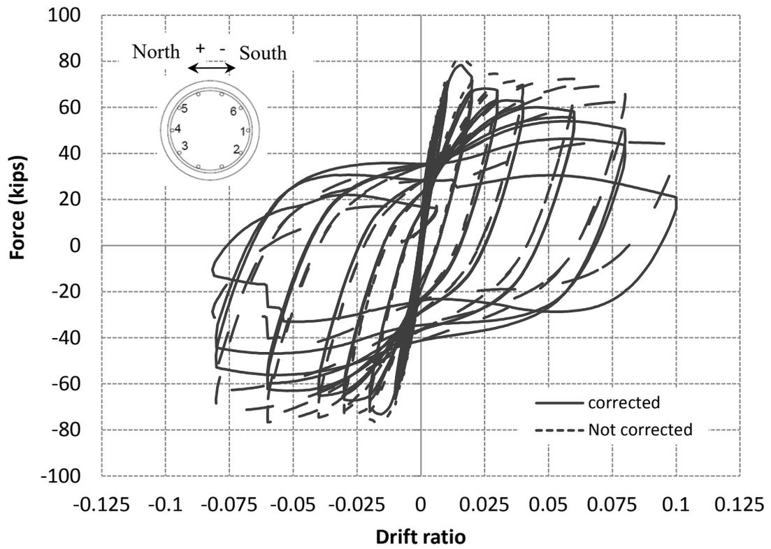
Figure 3.13 - Lateral load-vs.-drift ratio plots for Specimen #2
