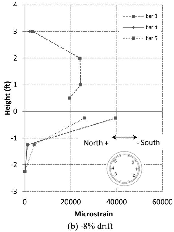
Figure 3.35 - Tensile strains in longitudinal bars of Specimen #2 at 8% drift
