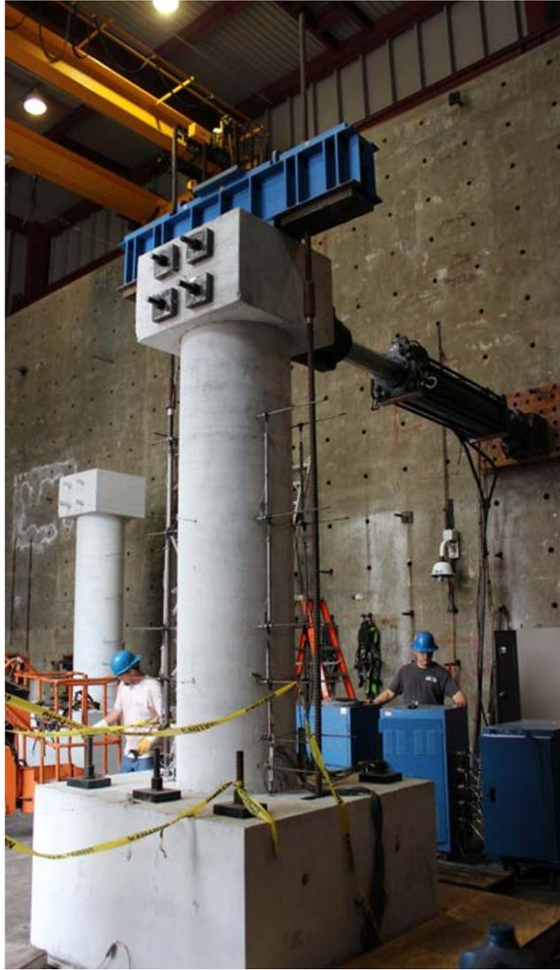
Figure 2.9 Picture of Specimen #1 test setup
