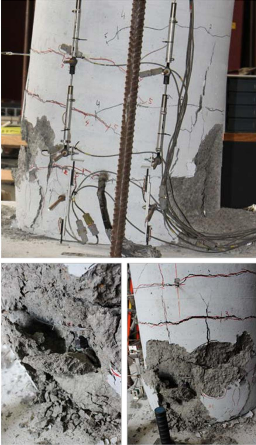
Figure 3.7 – Specimen #1 at 6% drift
