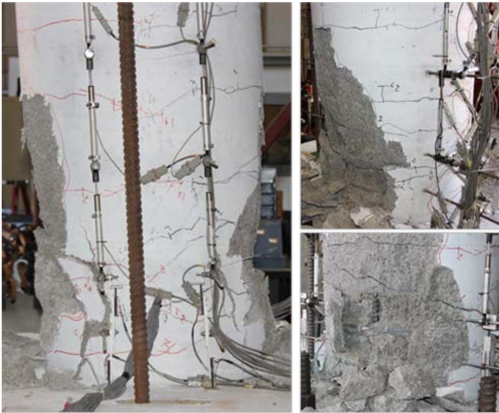
Figure 3.20 - Specimen #2 at 6% drift
