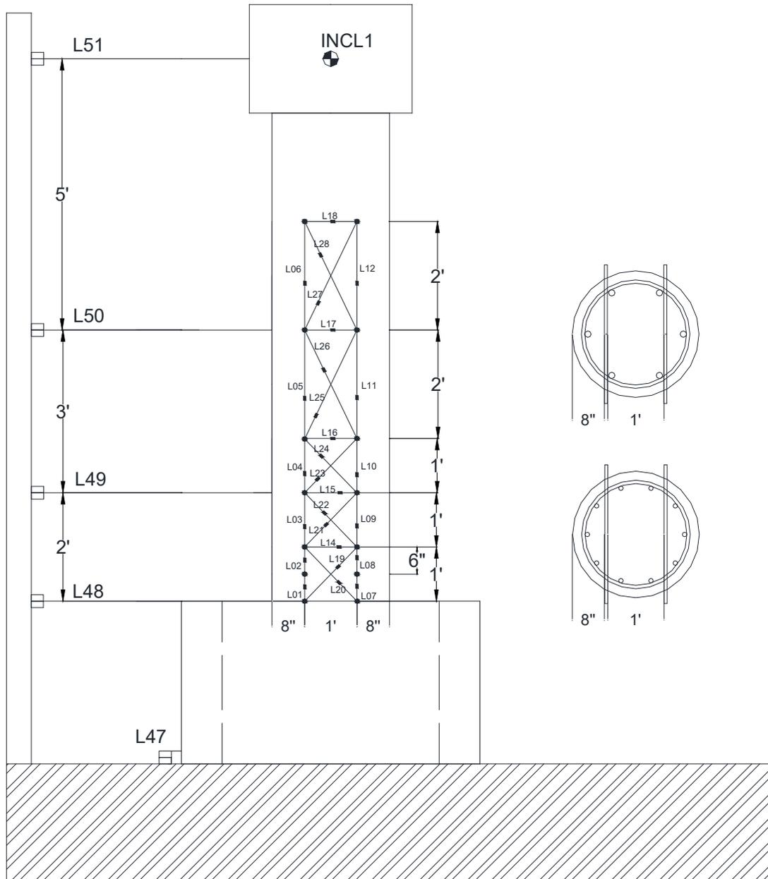
Figure 2.11 - Elevation view of displacement transducers (East face)
