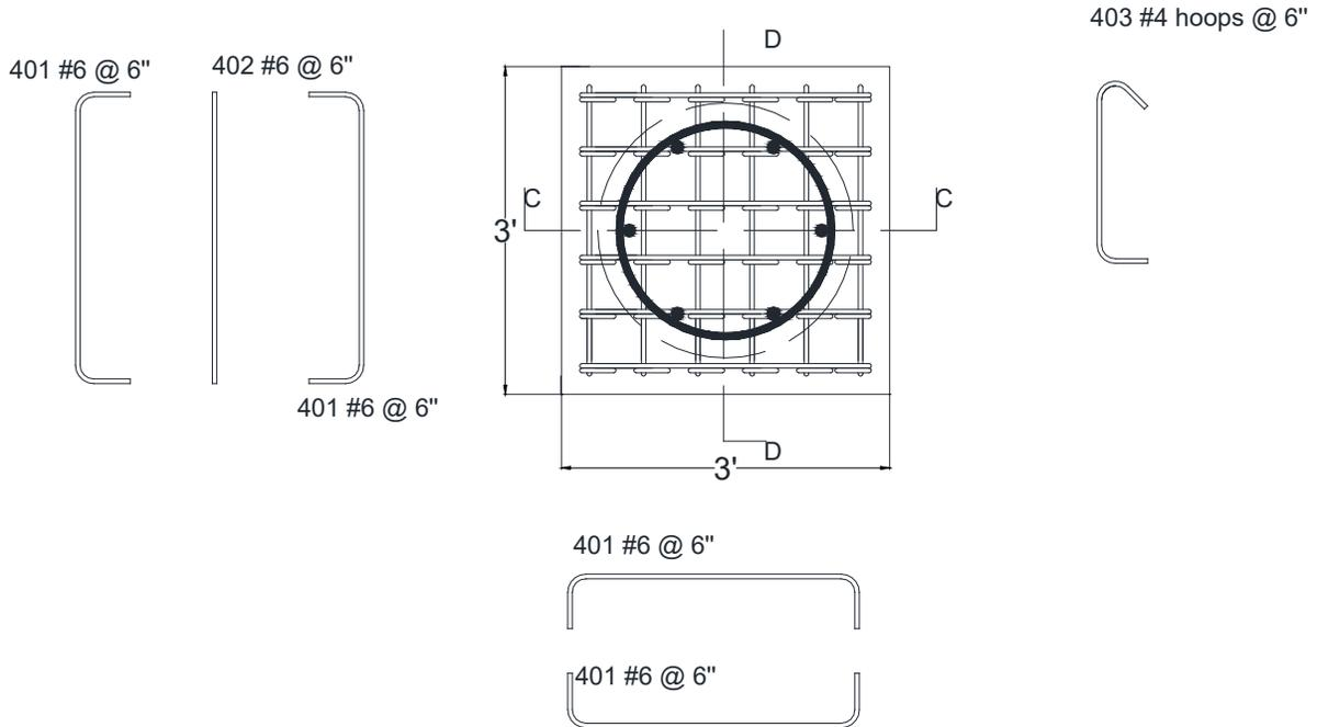
Figure 2.5 – Plan View of cap details
