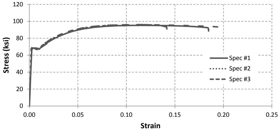
Figure 2.21 - Stress – strain curves for #9 longitudinal reinforcement
