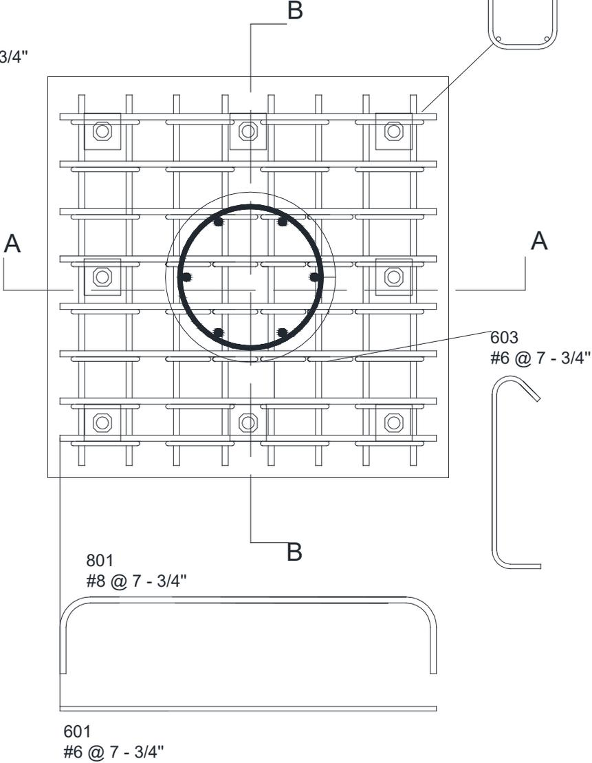
Figure 2.3- Plan view of footing details
