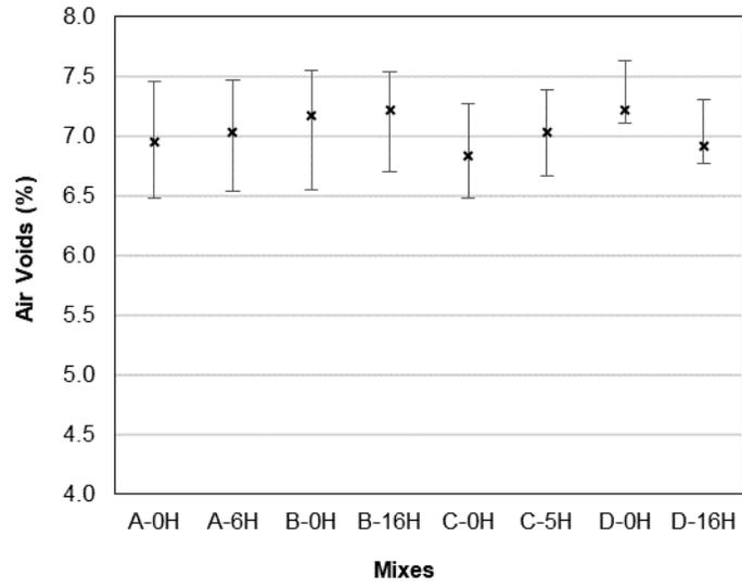
**Figure 3.10: Air void contents of flexural beam specimens.**
