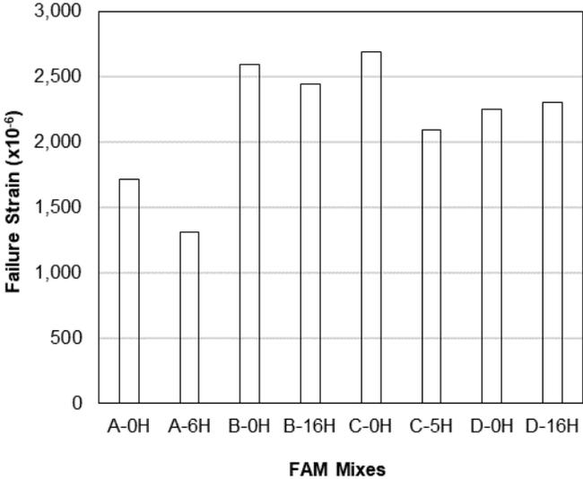
**Figure 7.6: Fatigue failure strain for all FAM mixes.**
