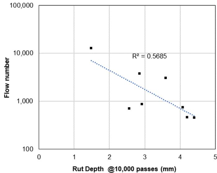
**Figure 4.21: Correlation between rut depth from HWT test and flow number from unconfined RLT for both silo storage conditions.**
