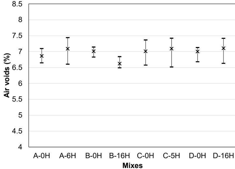
**Figure 3.9: Air void contents of IDEAL-CT specimens.**
