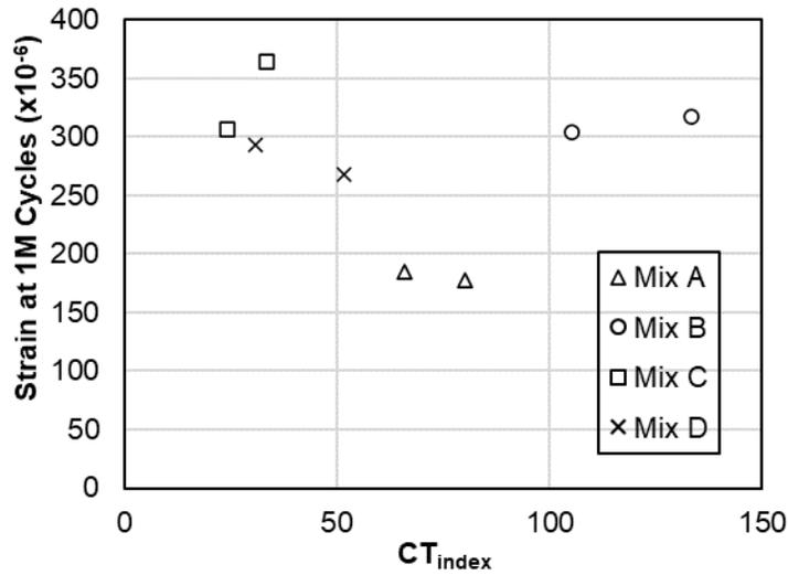
Figure 6.9: Strain at 1 million cycles from flexural beam test versus CT<sub>index</sub> from IDEAL-CT test for aged and unaged mixes.
