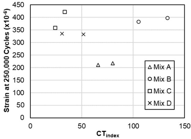
Figure 6.7: Strain at 250,000 cycles from flexural beam test versus CT<sub>index</sub> from IDEAL-CT test for aged and unaged mixes.
