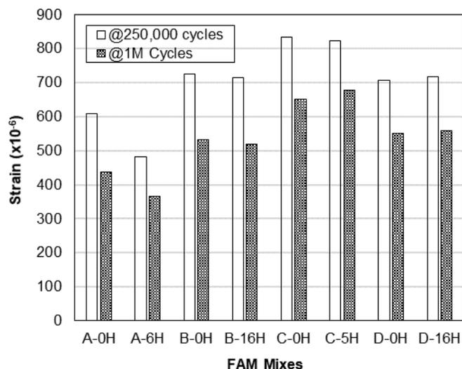
**Figure 7.7: Fatigue failure strain at 250,000 and 1 million cycles for FAM mixes.**
