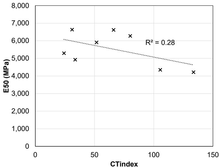
Figure 5.12: Flexural stiffness at 20°C (68°F) and 10Hz (E50) versus CT<sub>index</sub>.
