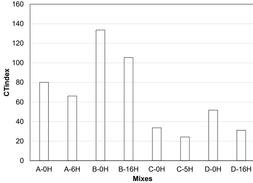
Figure 5.6: CT<sub>index</sub> from IDEAL-CT test for all mixes.
