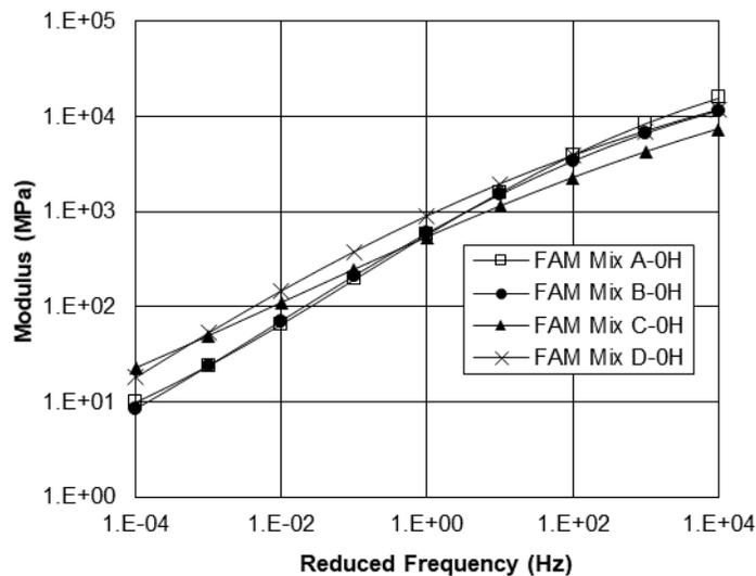
Figure 7.10: Modulus master curves for the FAM mixes.
