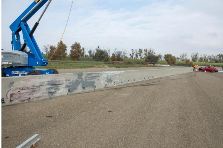
**Figure 5-8 Type 60 Barrier Post-Test Downstream of Impact**
