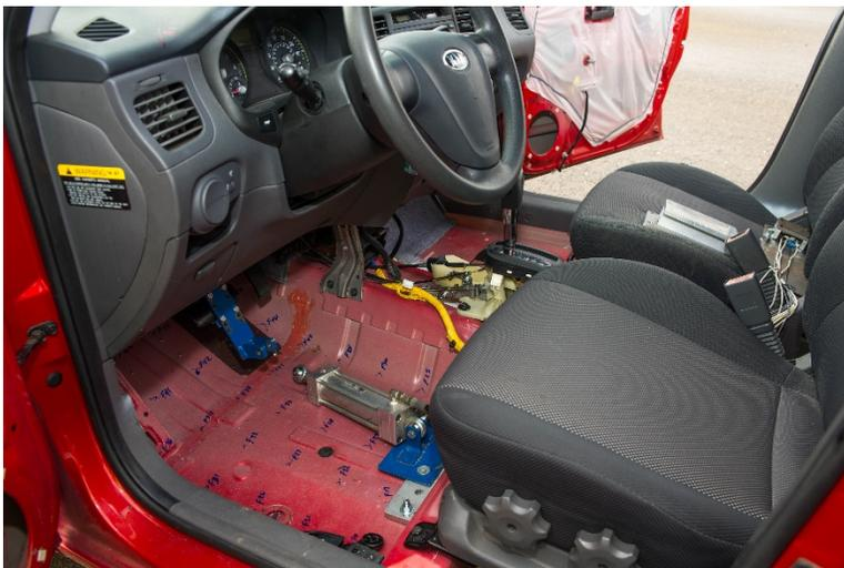
**Figure 7-4 Brake Pedal Actuator**
