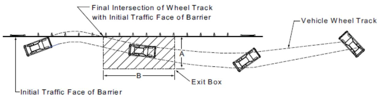
**Figure 5-18. Exit Box for Longitudinal Barriers**
