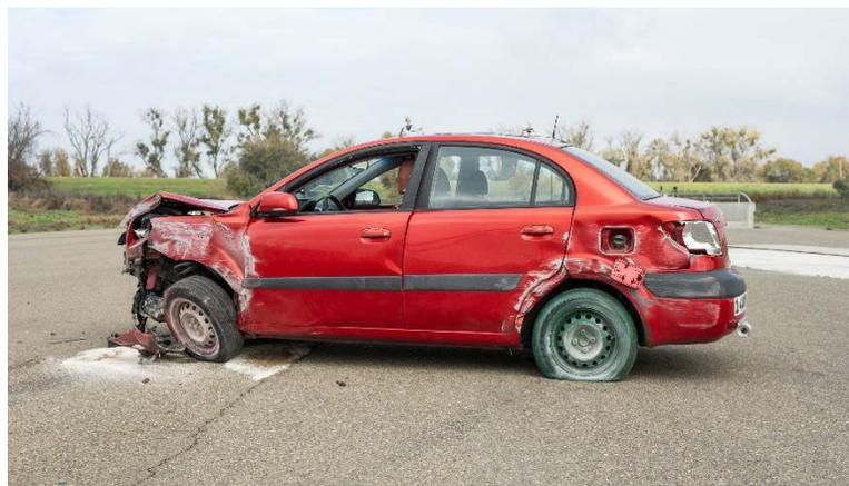
**Figure 5-11 140MASH3C16-04 Kia Rio Driver Side Damage**
