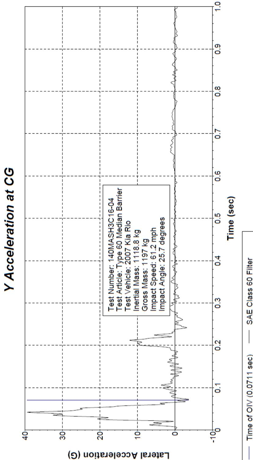
Figure 7-10 Lateral Acceleration at CG – Secondary
