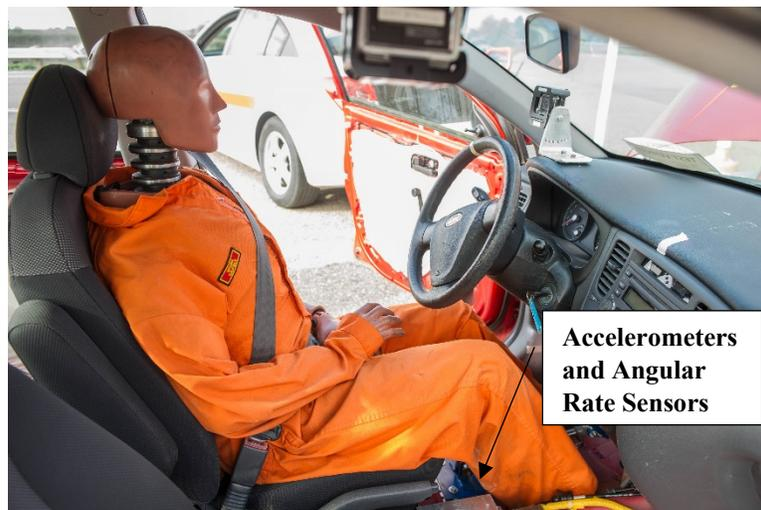
Figure 4-8 Test Vehicle Dummy and Instrumentation
