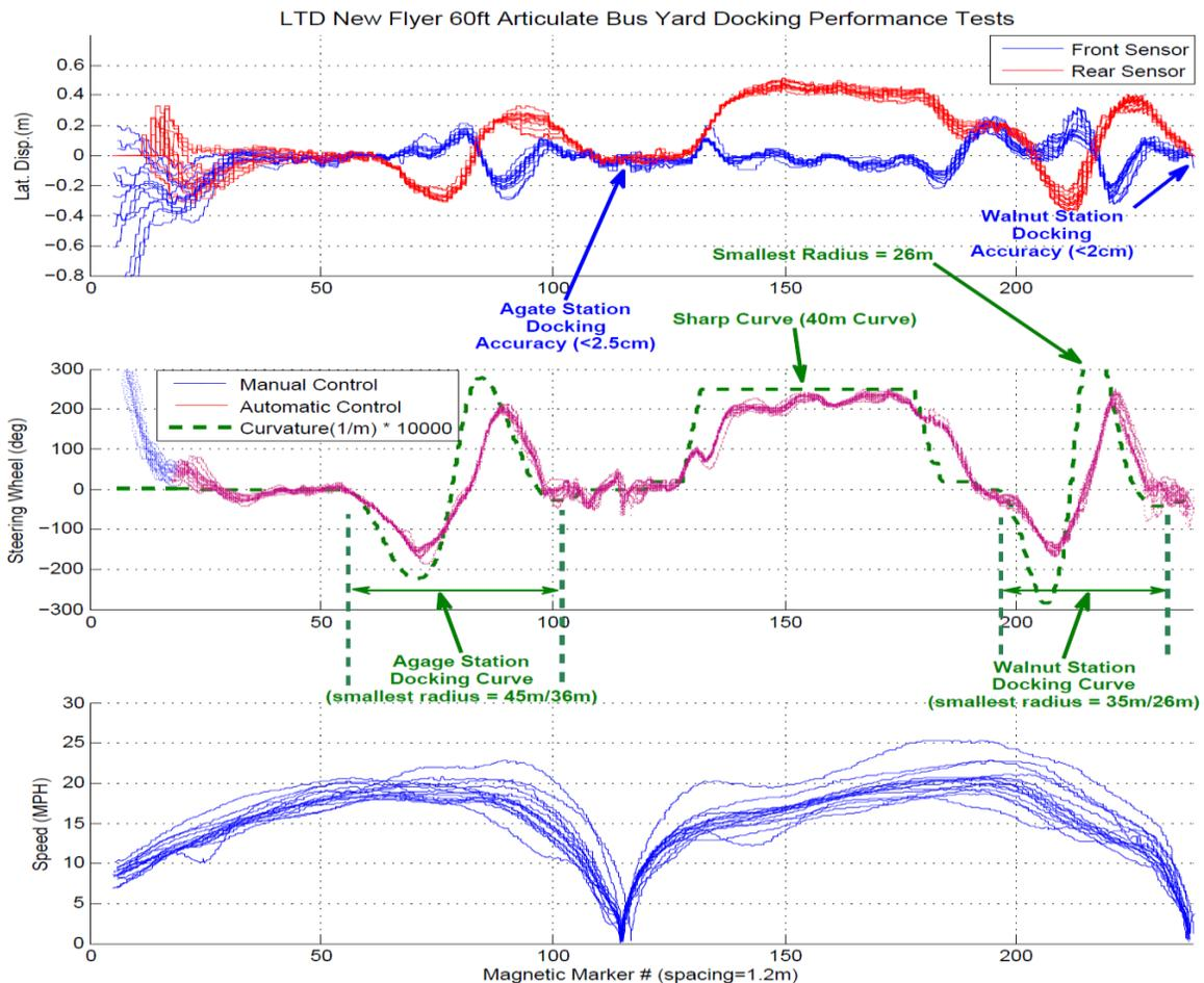
**Figure 5-8 VAA lane-keeping and docking performance at the LTD Yard test track**
