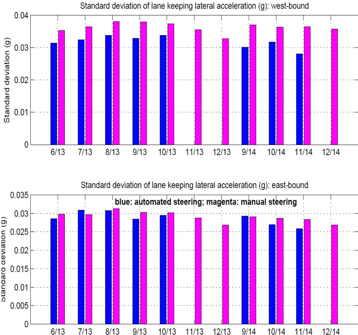
**Figure 5-47 Standard deviation of lane keeping lateral acceleration (g)**
