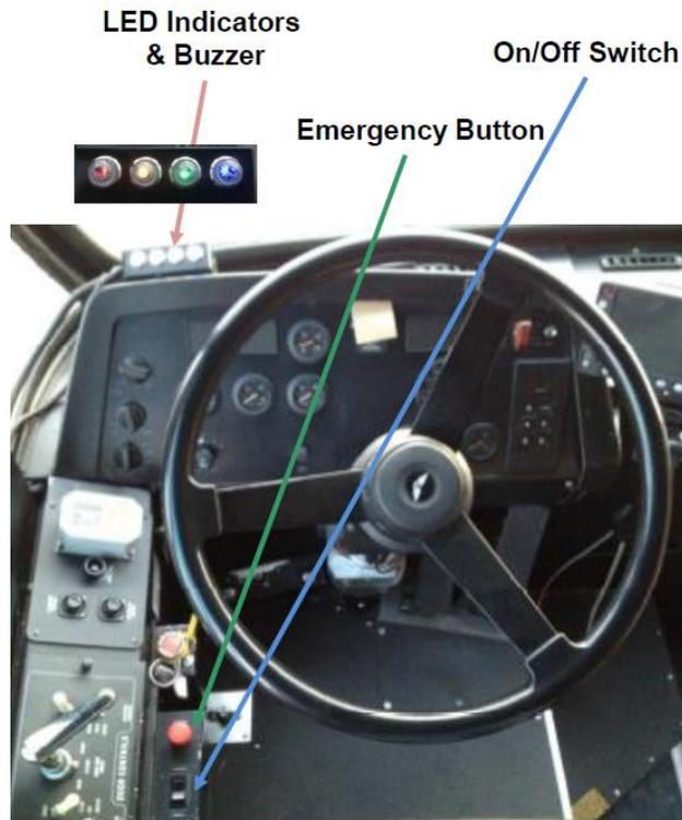
**Figure 3-5 Driver VAA Interface Components for the LTD New Flyer 60-ft Articulated Bus**
