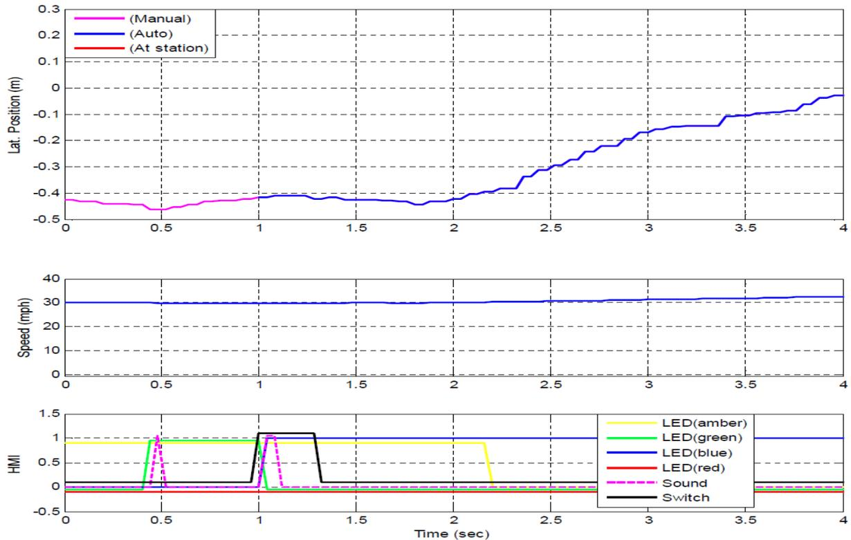
**Figure 5-30 EmX WB run: lateral position error, speed, and HMI LEDs & switch (time based - first four seconds)**
