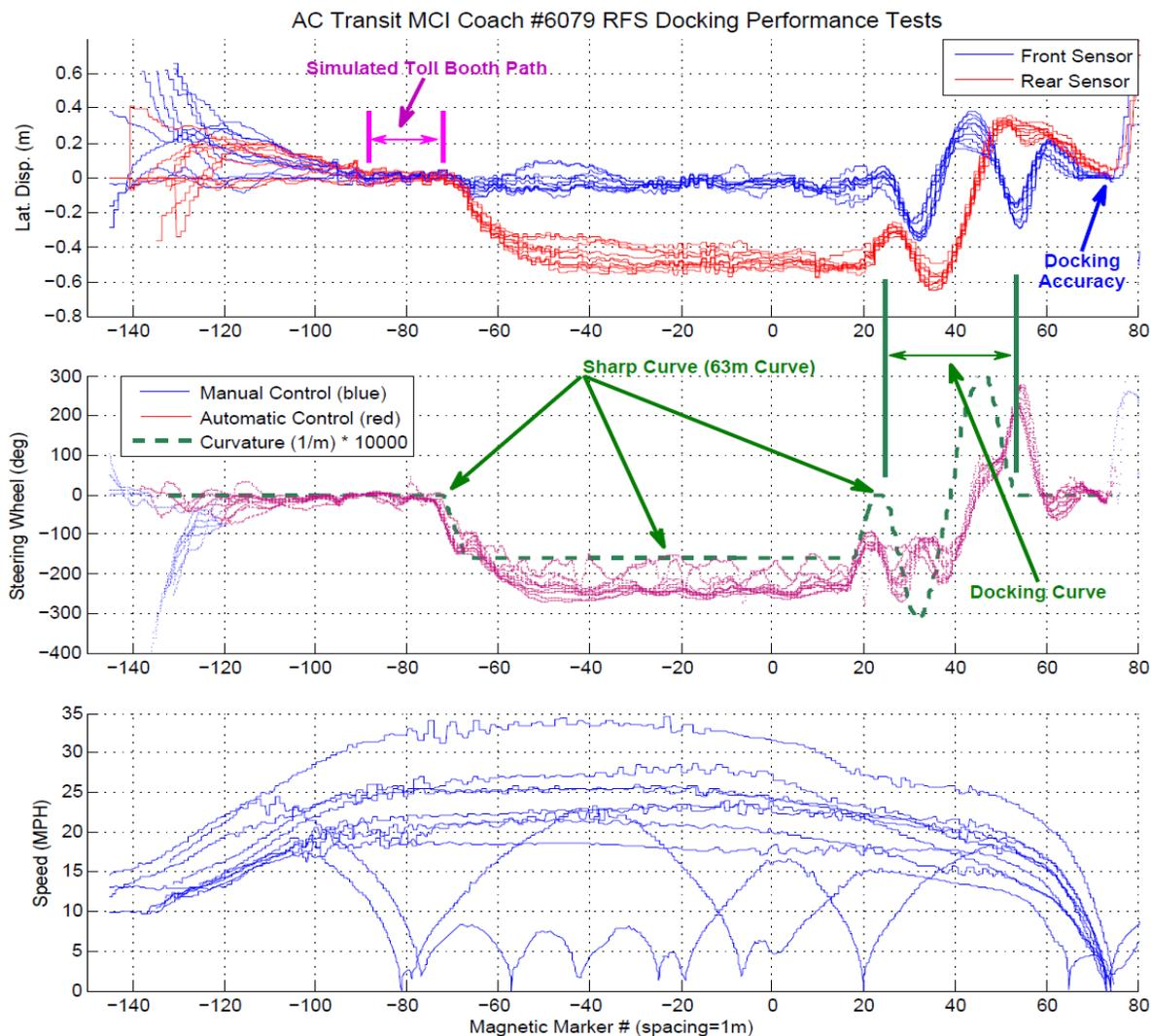
**Figure 5-22 VAA lane keeping and docking performance at the RFS test track**
