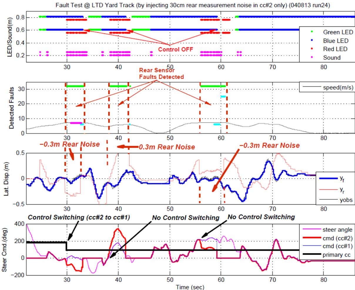
**Figure 5-11 Fault testing at the LTD yard track: fault in rear sensor (injecting rear sensor measurement noise in one control computer only)**
