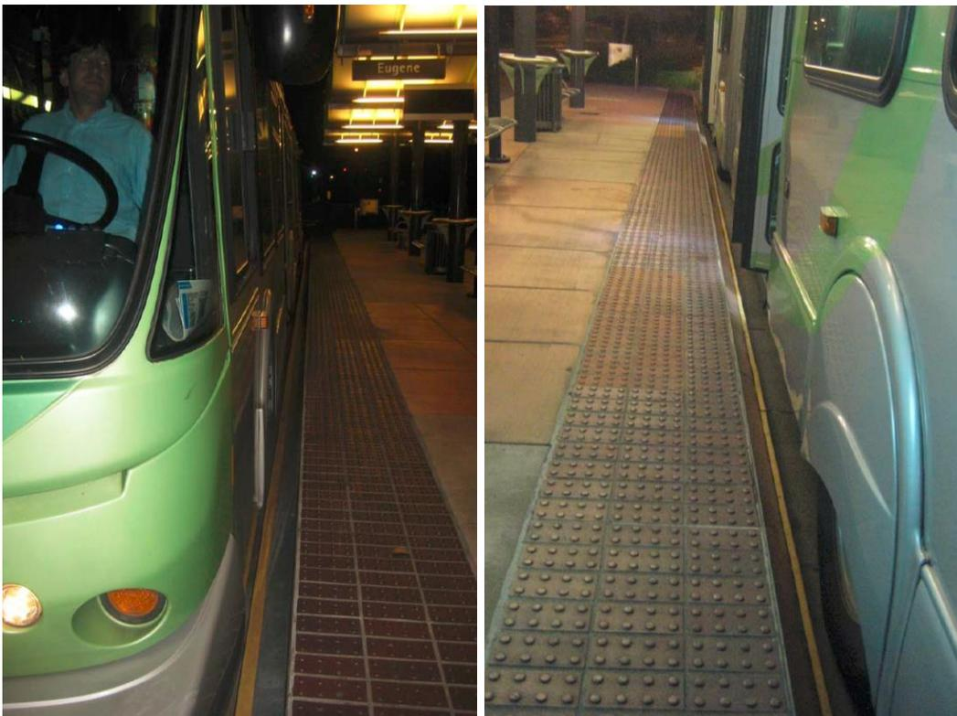
Figure 5-28 Precision docking at Dad's Gate Station (west-bound and east-bound)
