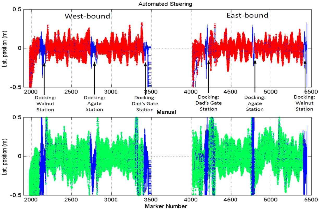
**Figure 5-29 Comparison of lateral positions (automated steering vs. manual driving)**
