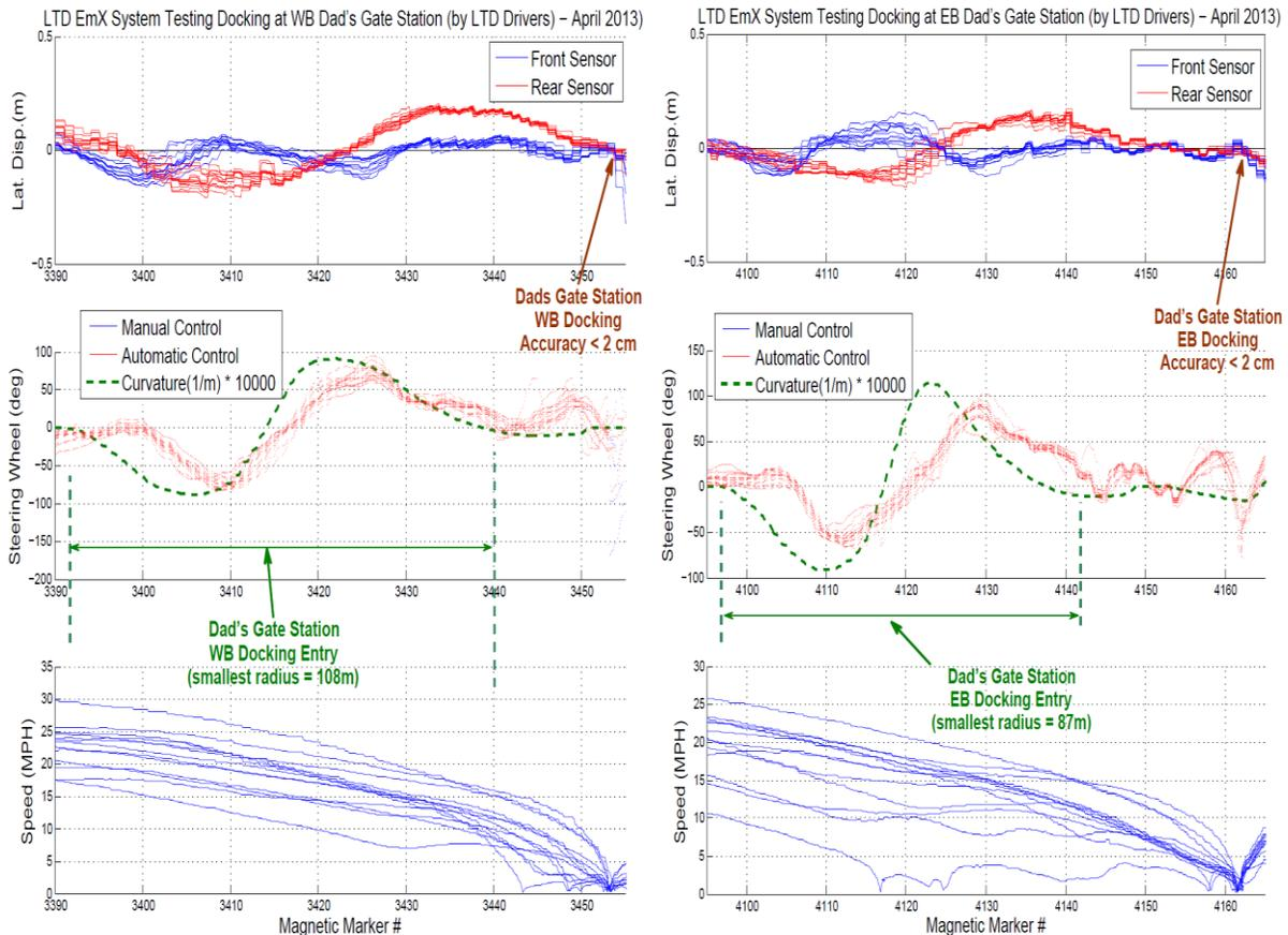
**Figure 5-20 Precision docking performance at EmX Track: Dad's Gate Station (WB & EB)**
