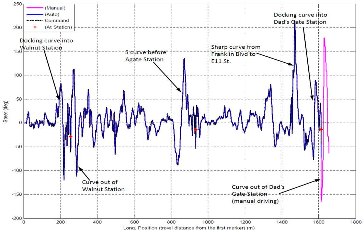
**Figure 5-34 EmX WB run: steering angle and command of the steering wheel (distance based)**
