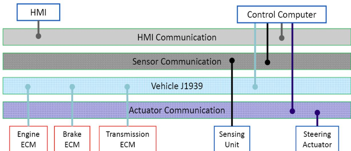
**Figure 2-1 Schematic for VAA communication network<sup>6</sup>**
