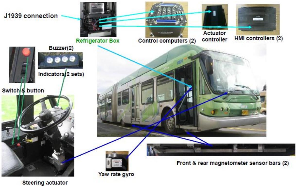
**Figure 3-8 VAA system components and installation on the LTD 60-ft New Flyer bus**
