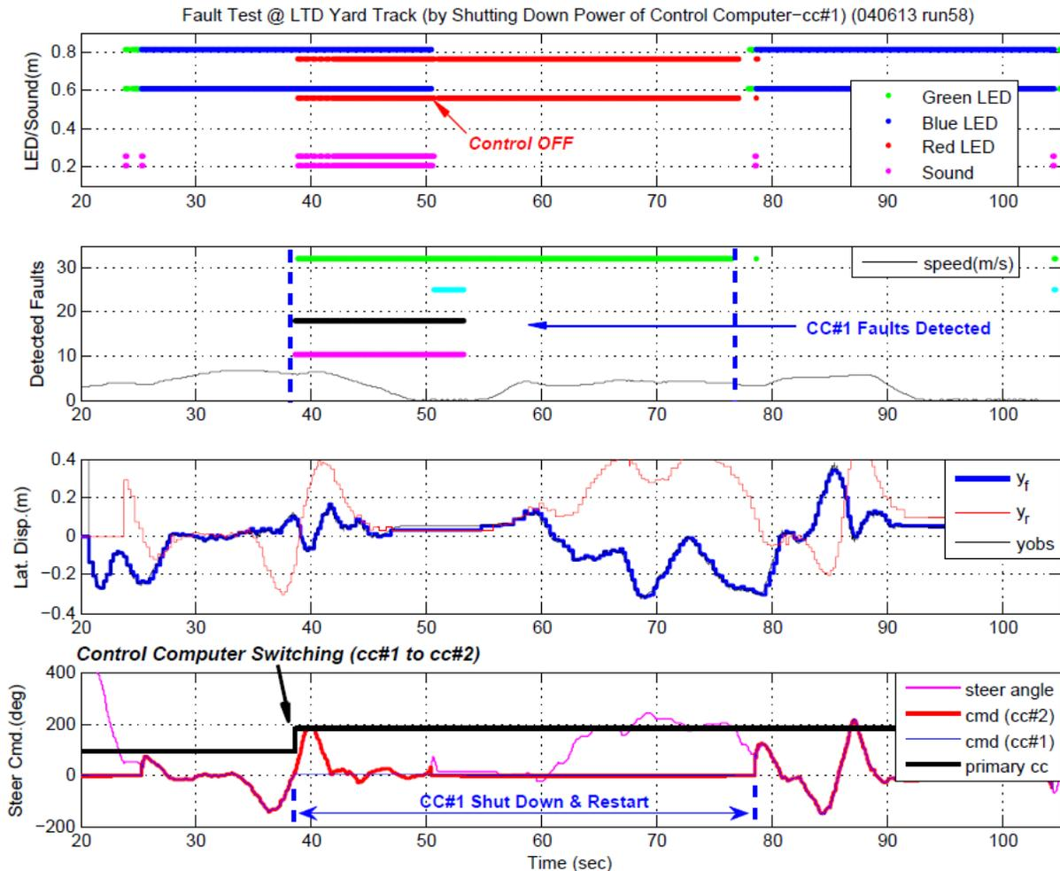
**Figure 5-12 Fault testing at the LTD yard track: fault in control computer (faults in shutting down one control computer)**
