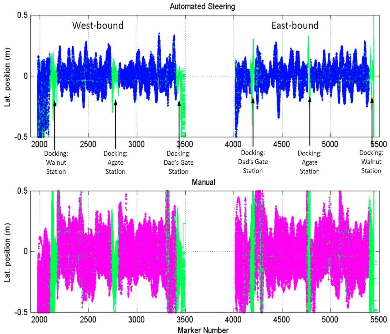
**Figure 5-43 Comparison of lateral positions: automated (upper plot) vs. manual driving (bottom plot)**
