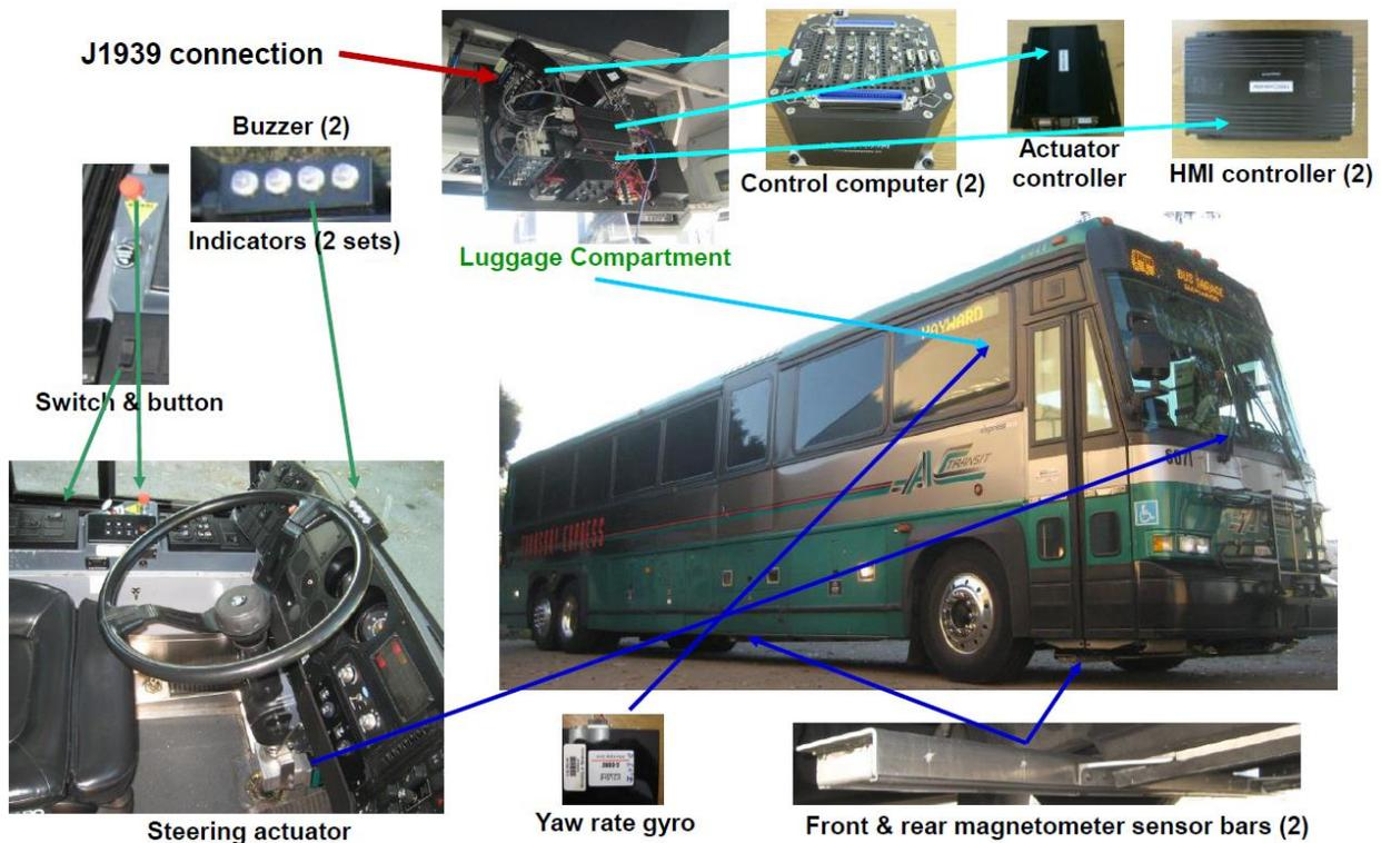
**Figure 3-9 VAA system components and installation on the AC Transit 50-ft MCI Coach**
