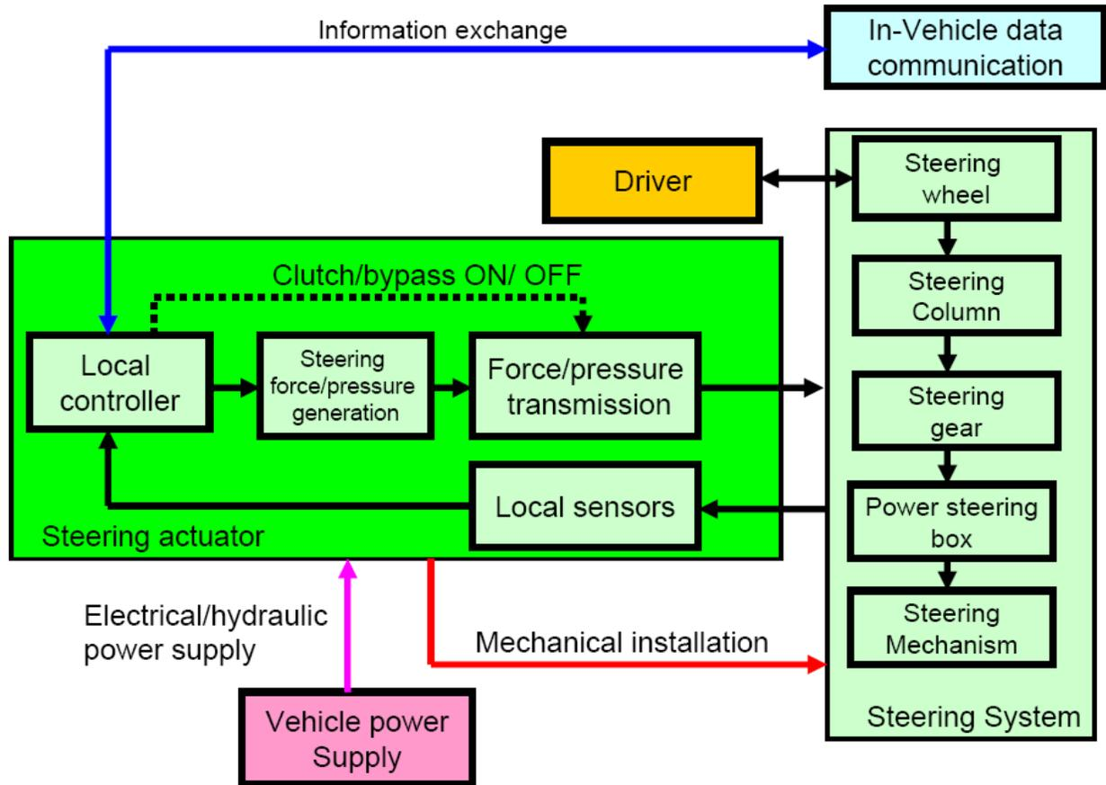
**Figure 2-3 Schematic of the Steering Actuator**
