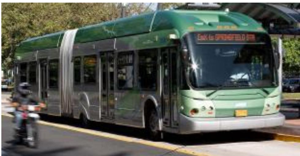
**Figure 3-3 New Flyer 60' Diesel Bus**
