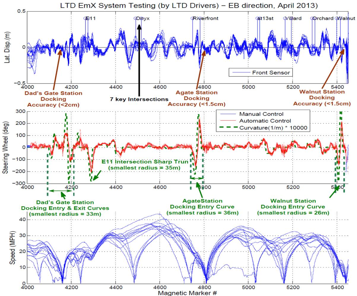
**Figure 5-14 Lane-keeping performance at EmX Track (Eastbound direction)**
