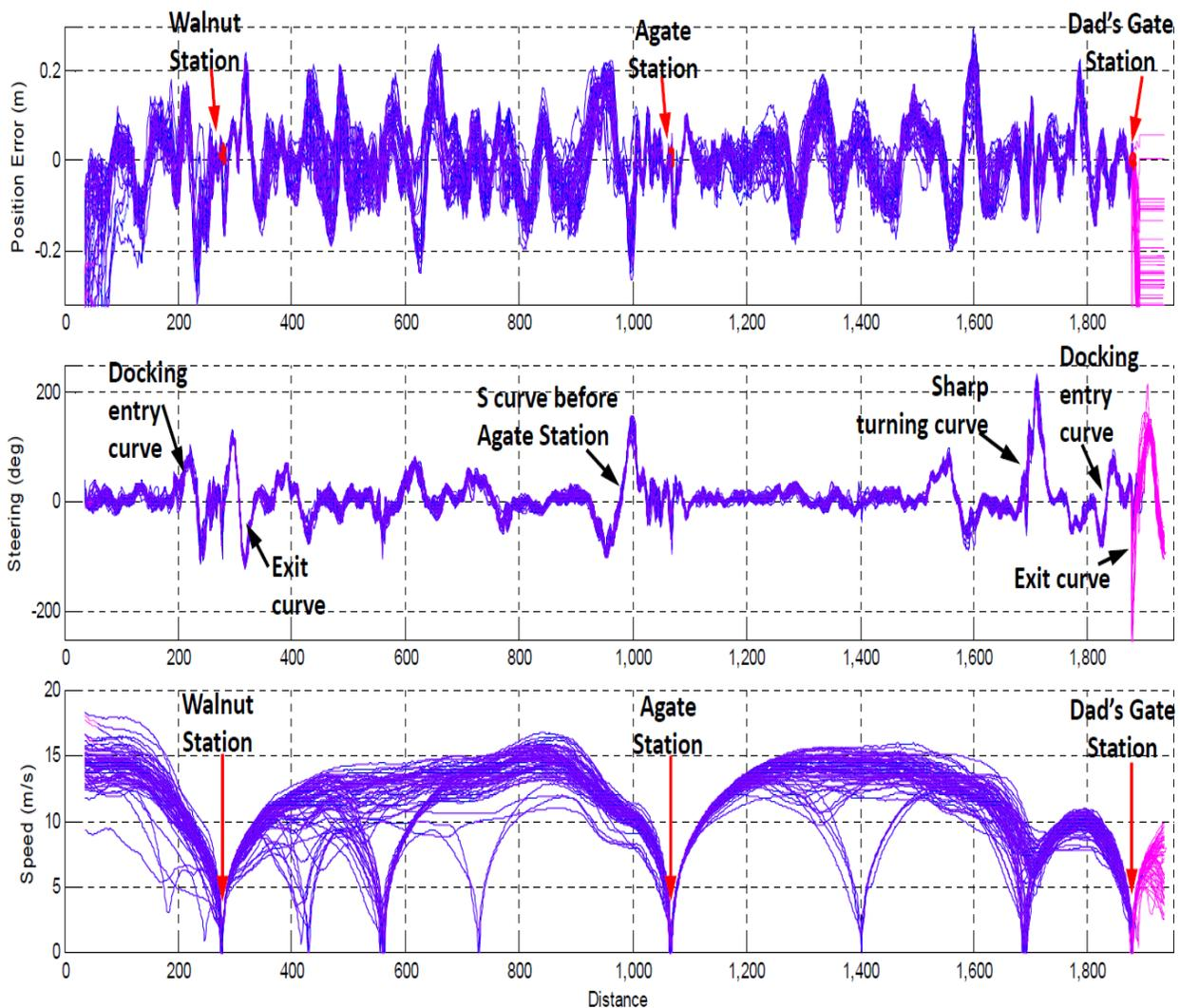
**Figure 5-41 EmX WB revenue service runs in July 2013: lateral position error, steering wheel angle, and vehicle speed (distance based)**
