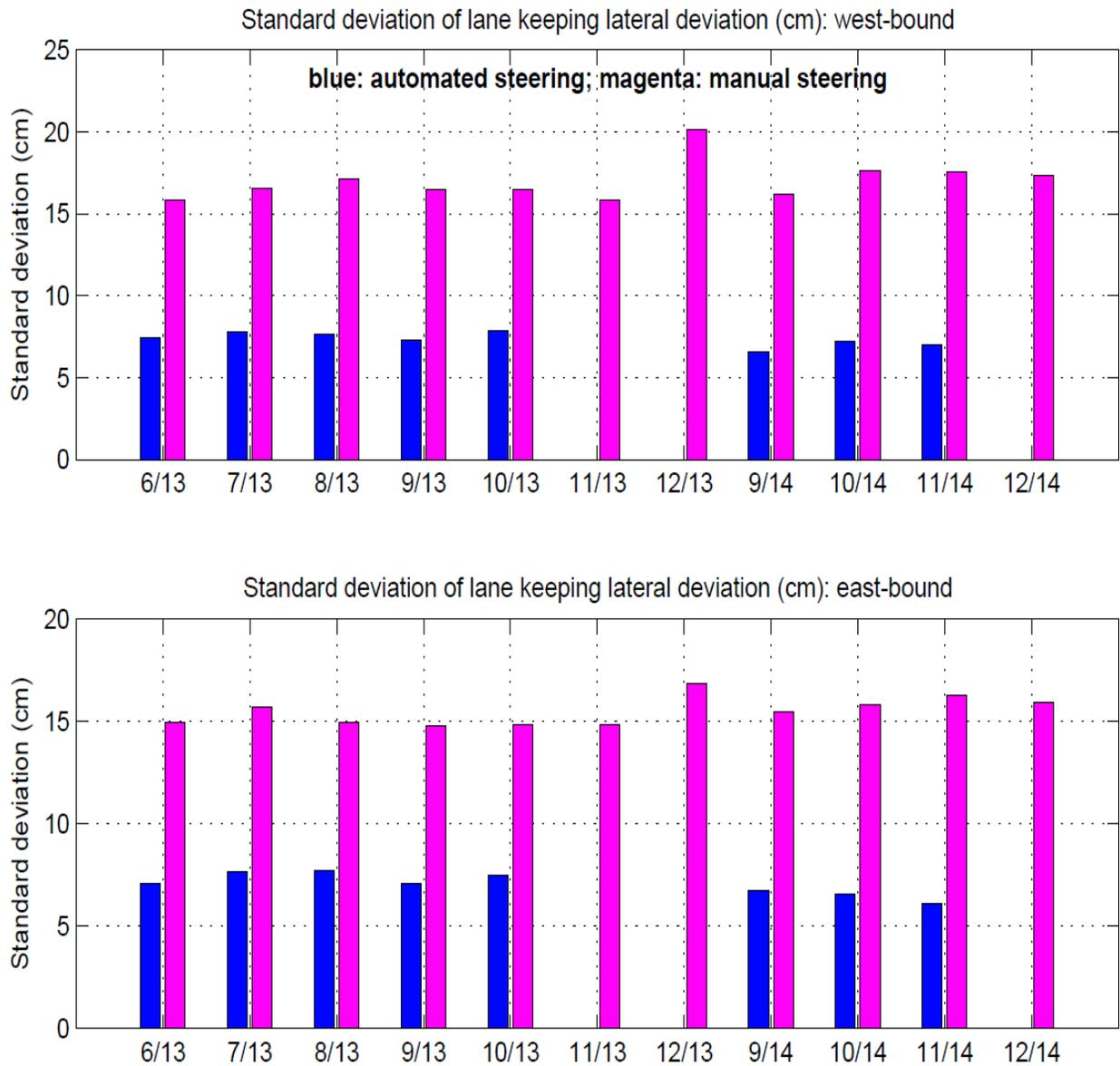
**Figure 5-45 Standard deviation of lane keeping deviation for each month of revenue service (blue: automated steering, magenta: manual steering)**
