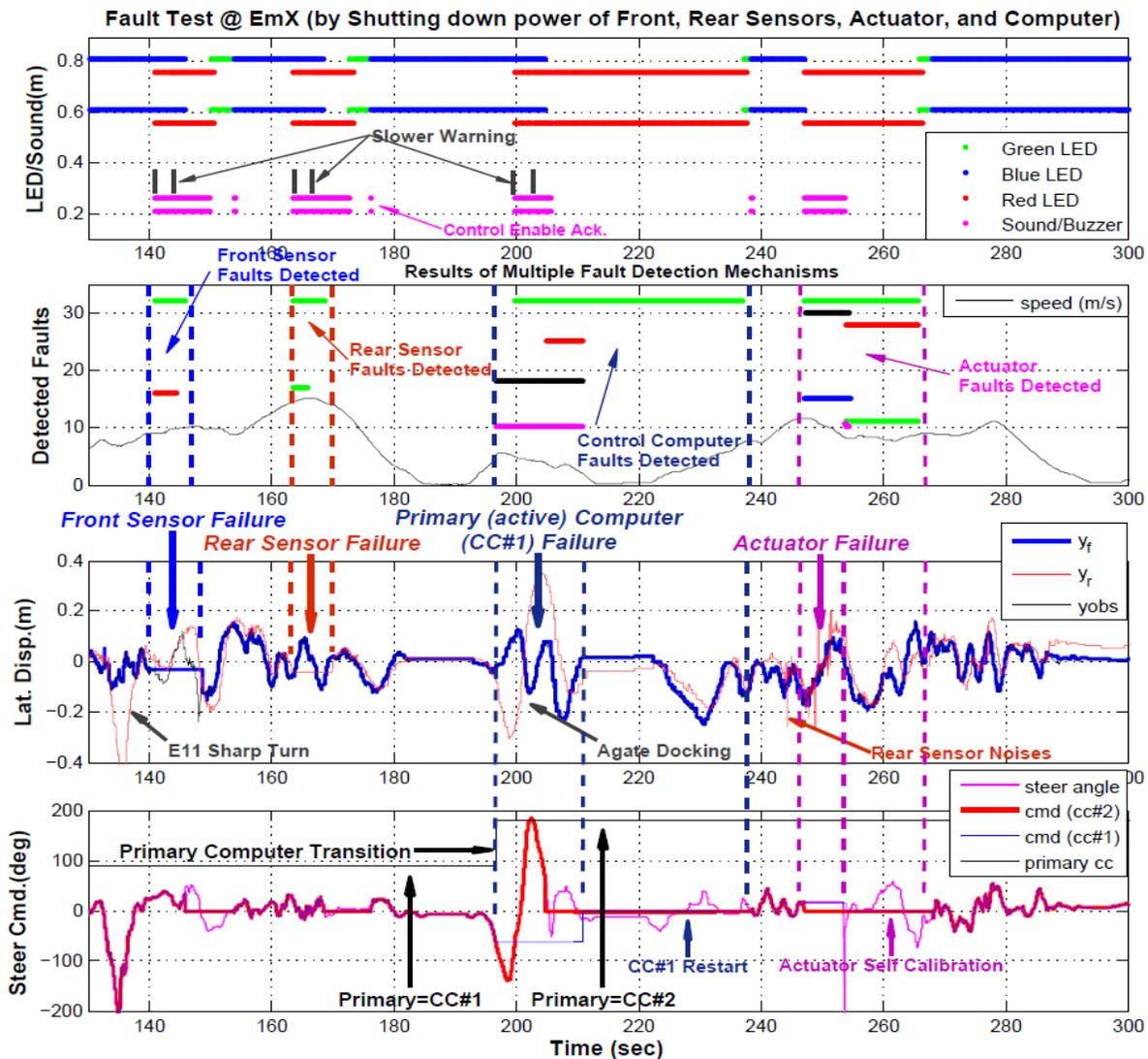
Figure 5-21 Fault testing on EmX conducted by the LTD instructors
