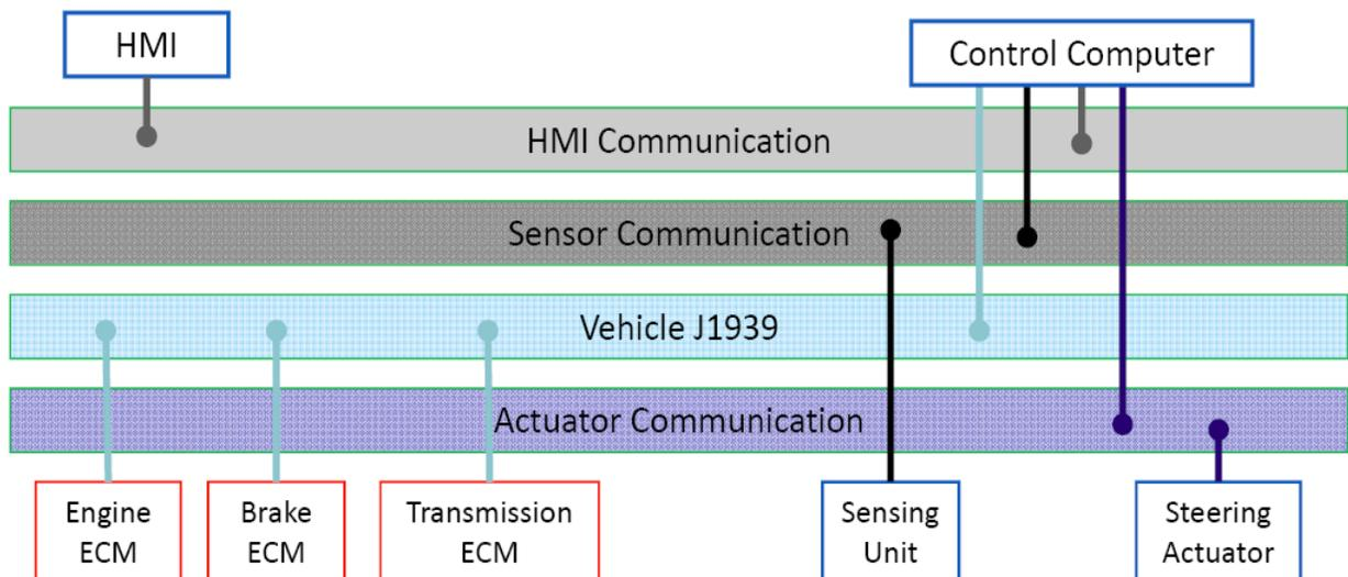
**Figure 2-1 Schematic for VAA communication network<sup>6</sup>**
