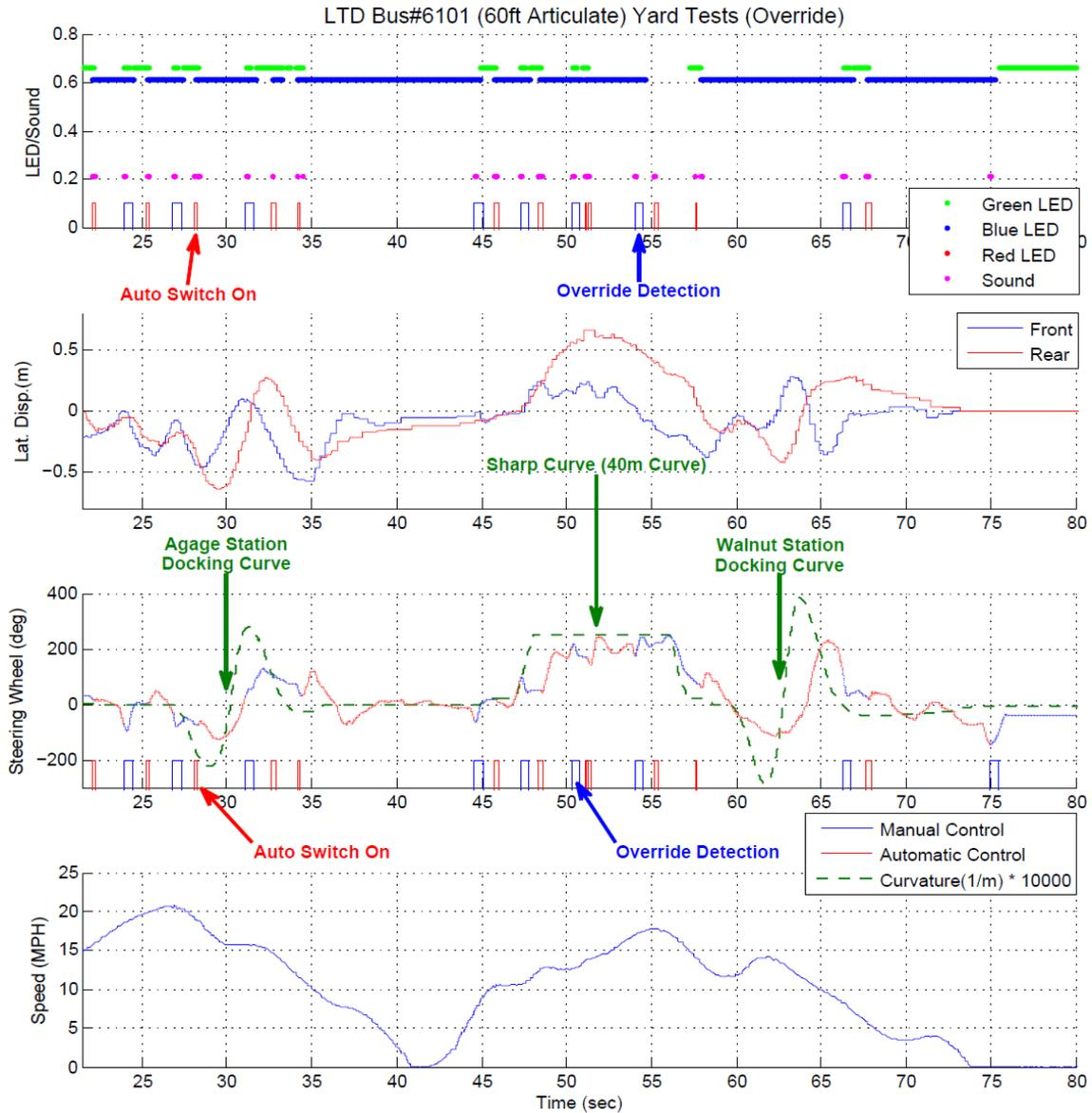
**Figure 5-9 VAA system automated-manual transitions using override (LTD yard)**
