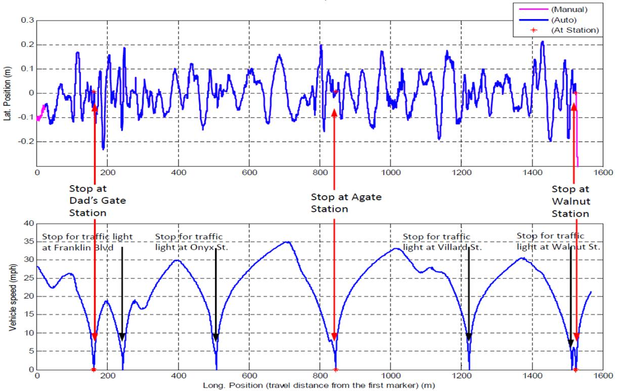
**Figure 5-36 EmX EB run: lateral position error and speed (distance based)**
