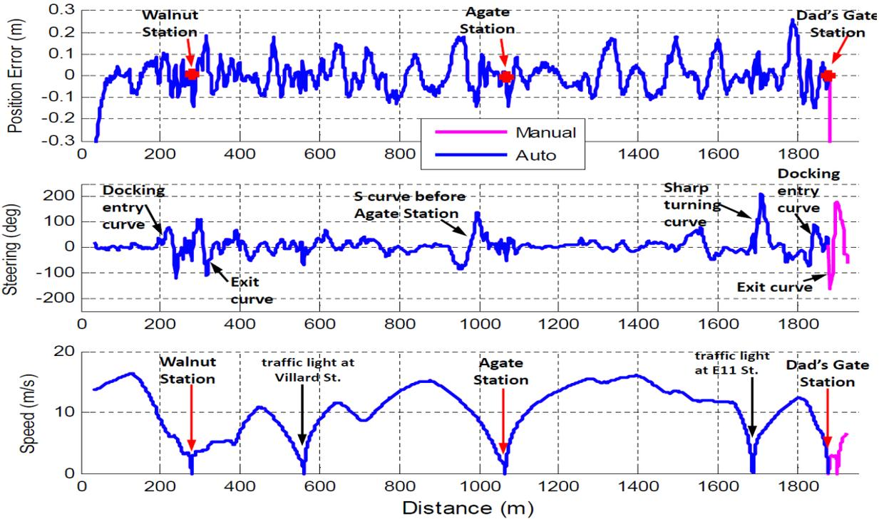
**Figure 5-39 EmX WB revenue service run: lateral position error, steering wheel angle, and speed (distance based)**
