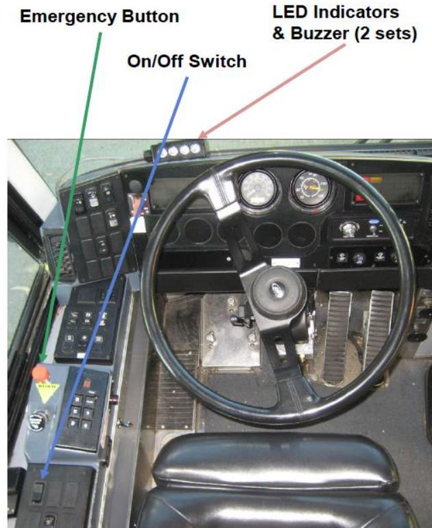
**Figure 3-6 Driver VAA Interface Components for the AC Transit MCI Coach**
