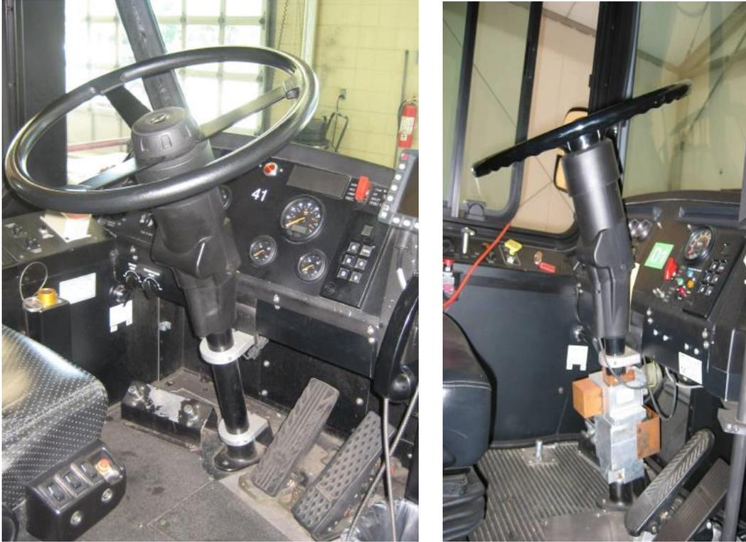
**Figure 3-4 New Flyer steering wheel and column (60' Diesel)**
