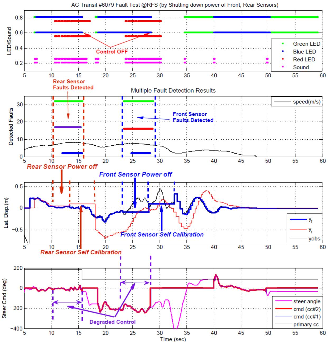
Figure 5-24 Fault testing at the RFS test track: faults in the front and rear sensors
