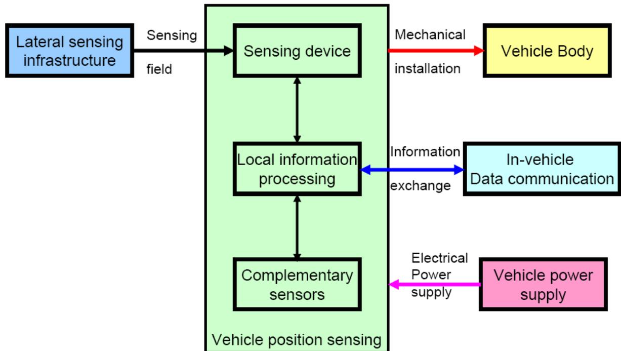
**Figure 2-2 Schematic for Vehicle Position Sensing**
