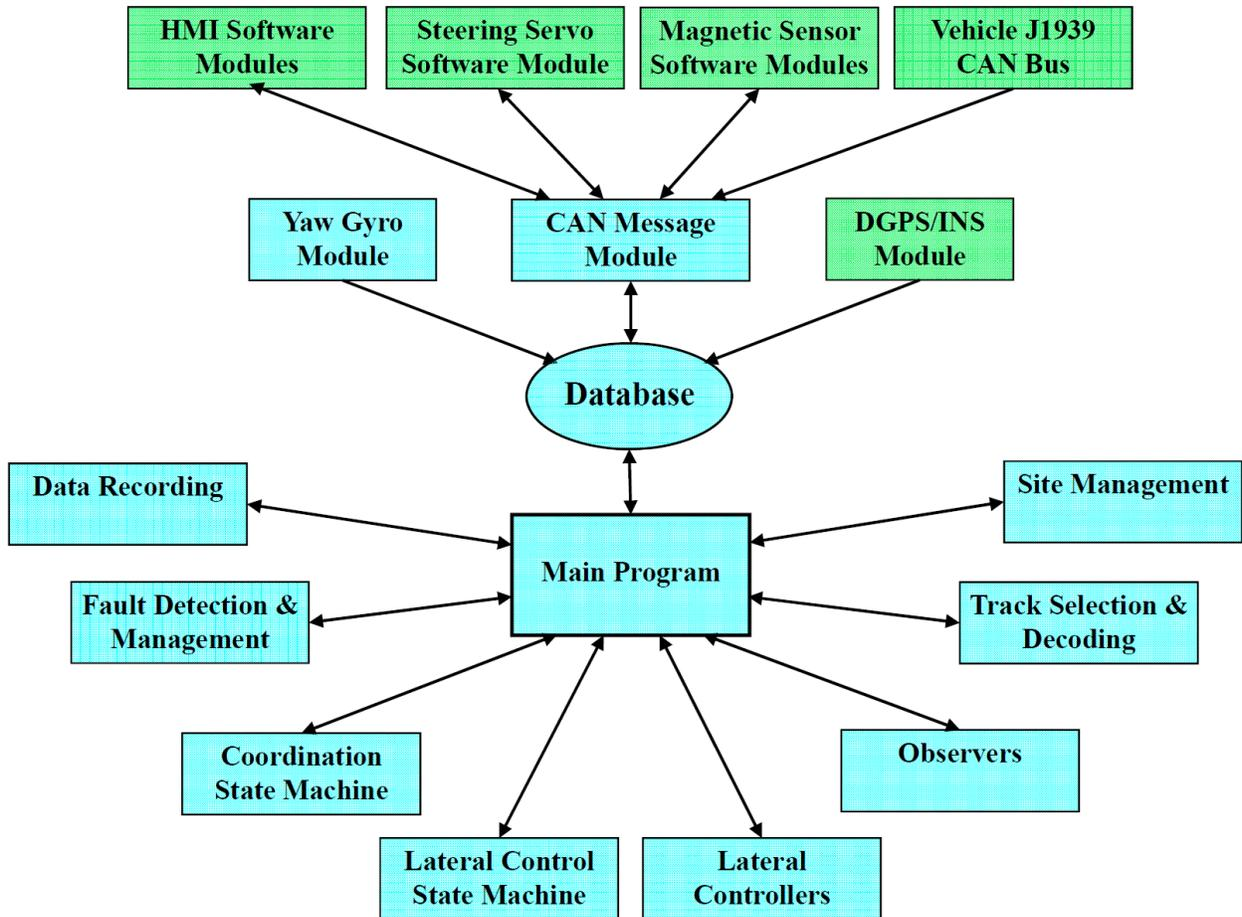
**Figure 3-7 VAA System Software Architecture**
