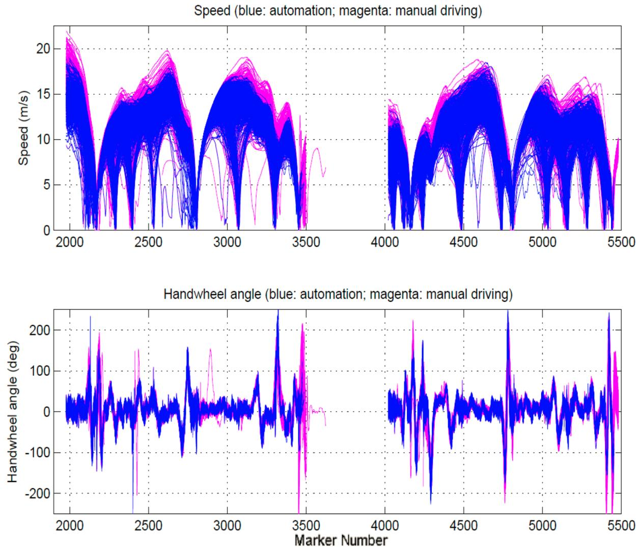
**Figure 5-44 Revenue Service: bus speed (upper plot) and steering wheel angle (bottom plot)**
