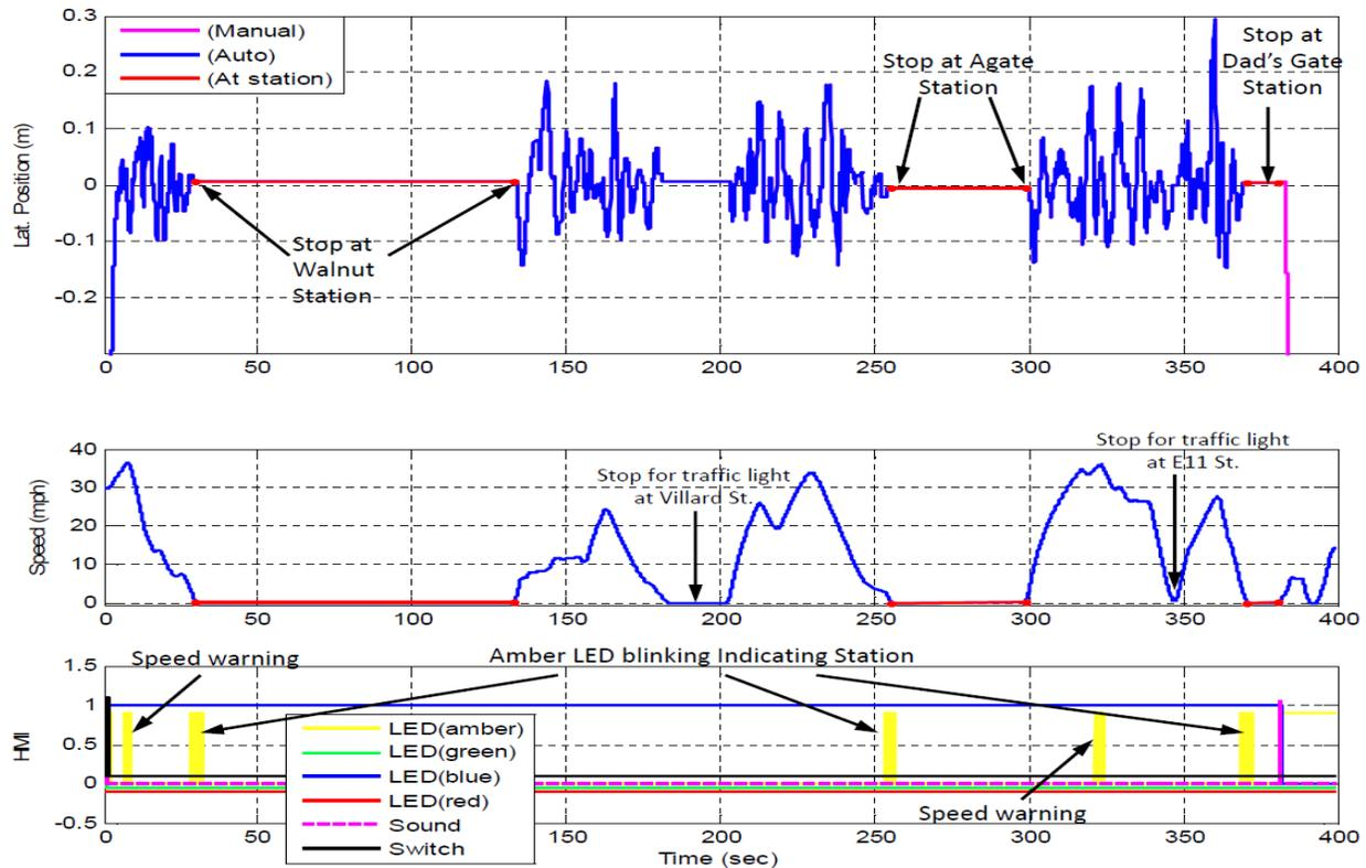
**Figure 5-31 EmX WB run: lateral position error, speed, and HMI LEDs & switch (time based)**
