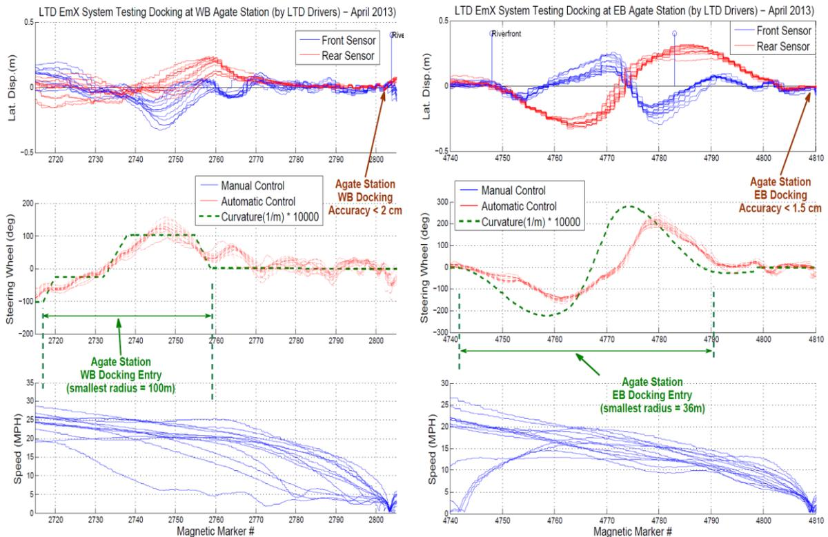
**Figure 5-19 Precision docking performance at EmX Track: Agate Station (WB & EB)**
