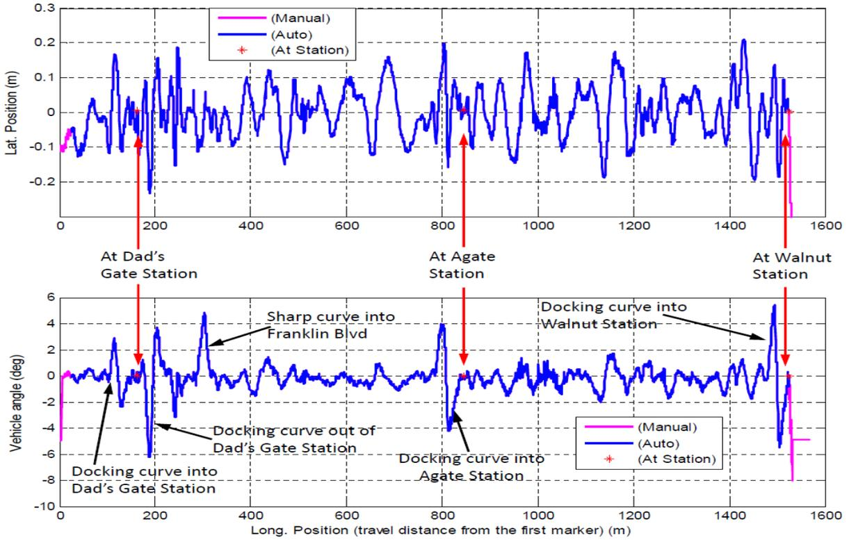
**Figure 5-37 EmX EB run: lateral position error and vehicle angle (distance based)**
