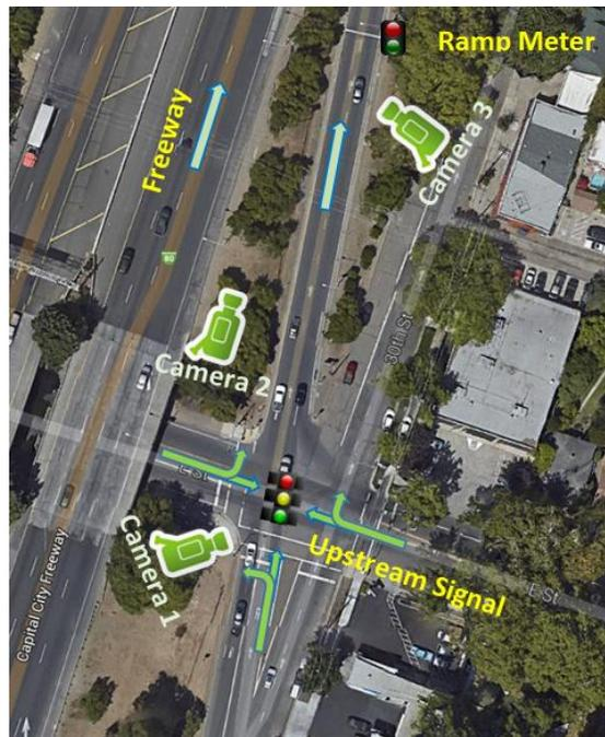
Figure 3-10 Typical Camera Layout for Queue Storage Data Collection
