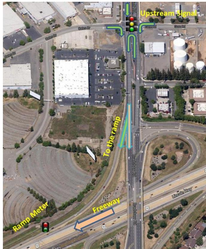
Figure 3-9 Slip Ramp with Diverging Movement (Bradshaw Road to WB 50, Caltrans District 3)
