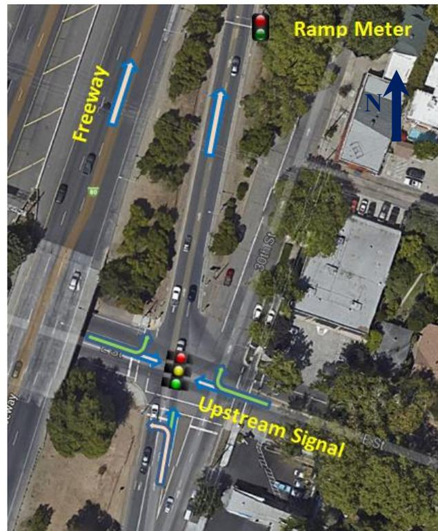
Figure 3-5 Diamond Ramp with Three Feeding Movements (E St. to NB 99, Caltrans District 3)
