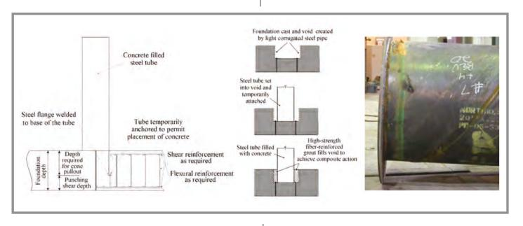
Construction of a CFT column and connection: (I) Overall configuration; (c) Construction procedure for grouted connection; (r) Welded annular ring at base of tube
