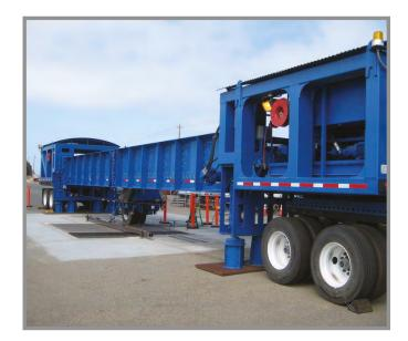
HVS testing on the deck joint
