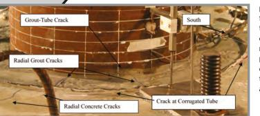
environment. Although CFTs offer many practical advantages, few studies have focused on the connections for CFT columns to the footings or cap beams, a critical element of bridge construction. This research investigated and developed design procedures for simple and economical connections of circular CFT piers or columns to reinforced concrete foundations, pile caps, and wide cap beams.
