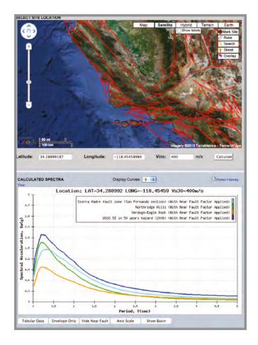
Engineers can quickly calculate the spectral acceleration by simply supplying the site's latitude and longitude and the shear-wave velocity in the top 30 meters of soil.
