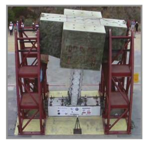
Beaten, but not broken, a full-scale Caltrans-designed bridge column on the UCSD/NEES Outdoor Shake Table maintains vertical support of more than 260 tons after undergoing six simulated earthquakes, each in excess of maximum design load.
