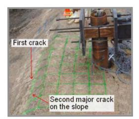
Crack pattern at 6-inch pile top displacement
