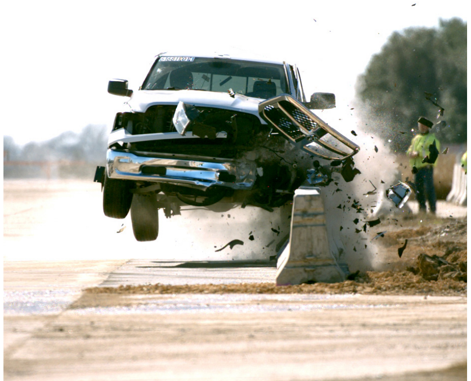
A pickup truck crashes into a concrete barrier during a controlled impact test, with debris flying and personnel watching from a safe distance.
