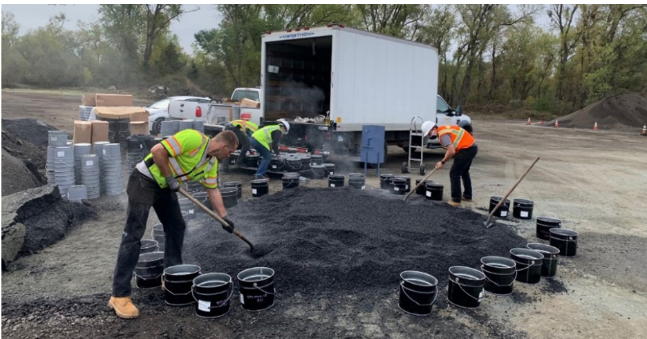
Crews sampling asphalt mixes from a pilot project for laboratory testing.
