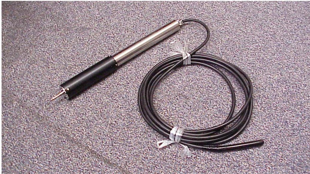
Figure 3.3.22 Displacement Sensor
