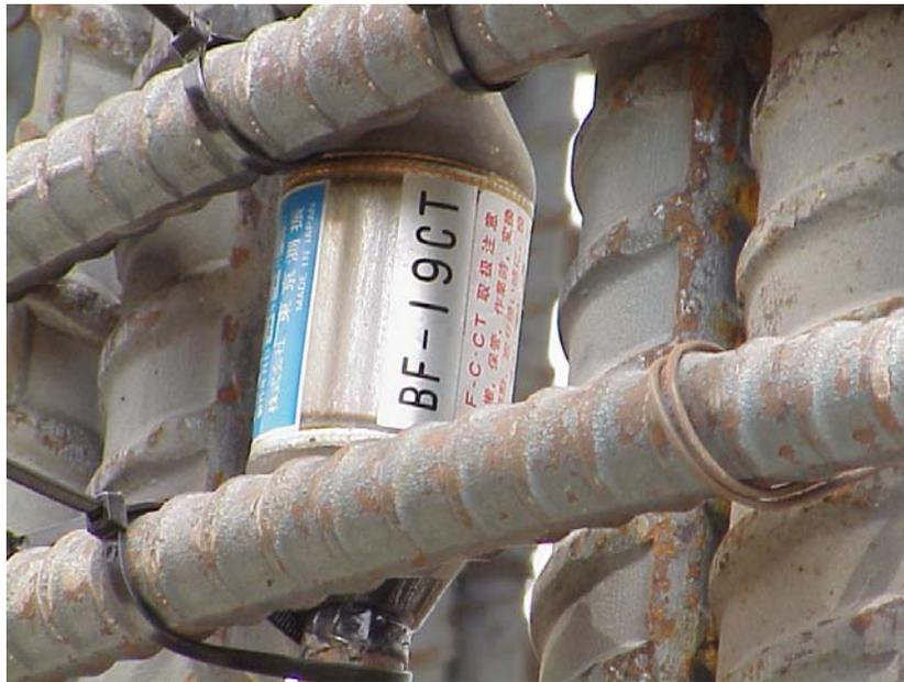
(b) LVDT Type Strain Meter Installed in the Column
