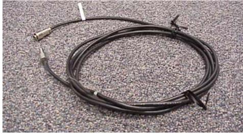
(a) Thermocouple Sensor head
