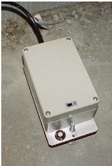
(a) A uni-axial accelerometer mounted in box-girder without bracket
