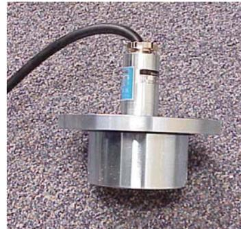
Figure 3.3.20 Soil Pressure Sensor
