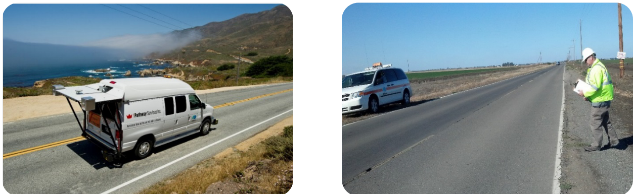
FIGURE 1. A.P.C.S. VEHICLE ON THE ROAD AND MANUAL PAVEMENT INSPECTION
