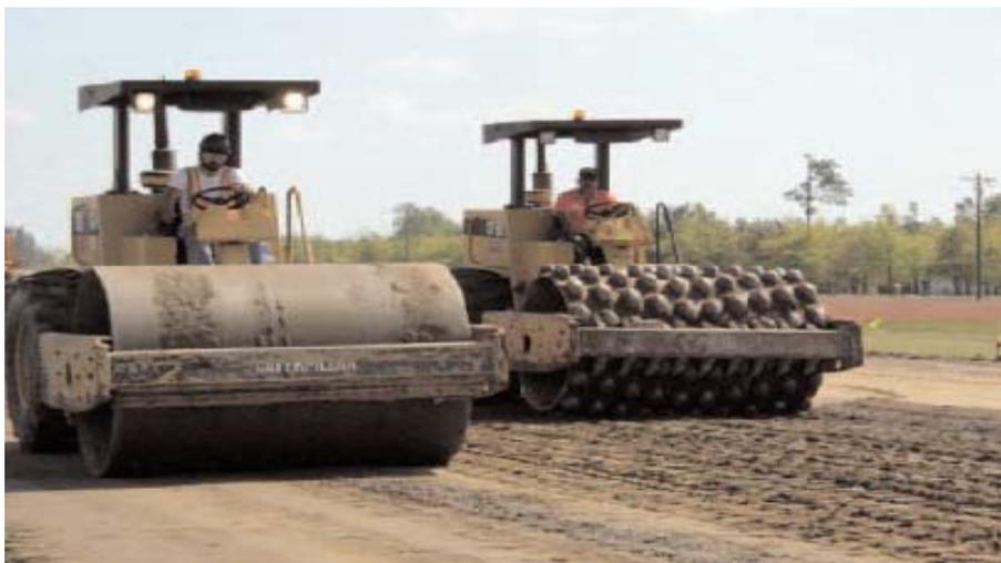
**Figure 3. Steel Drum Roller and Sheepfoot Roller (no blade)**
