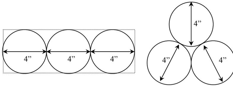
**Figure 6c. Examples of Clustered Coring Patterns**
