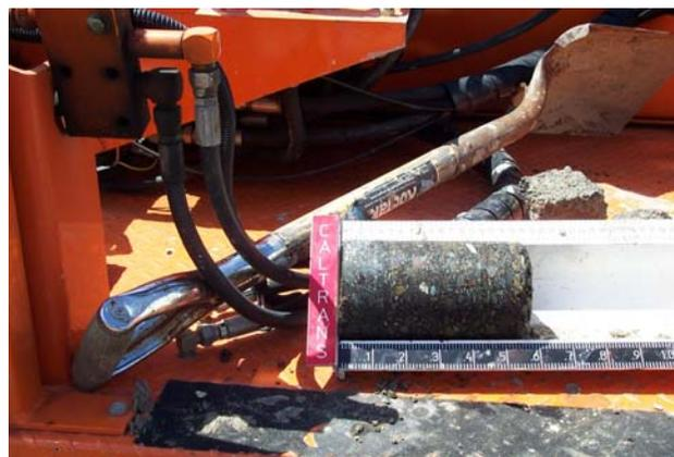
**Figure 6b. Core (4 Inch Diameter)**
