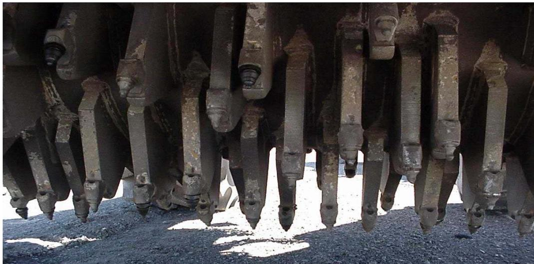
**Figure 8. Pulverizer Milling Teeth**
