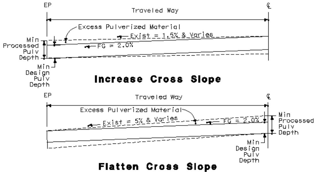
**Figure 9. Slope Corrections and Minimum Design Pulverization Depth**
