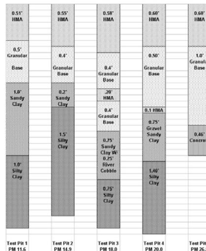
**Figure 7b. Example Test Pit Profile**
