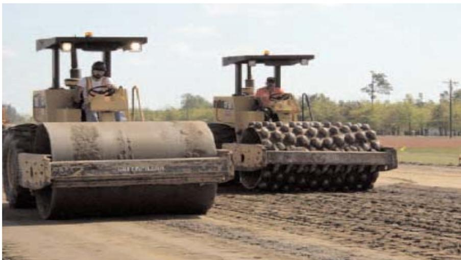
**Figure 3. Steel Drum Roller and Sheepfoot Roller (no blade)**
