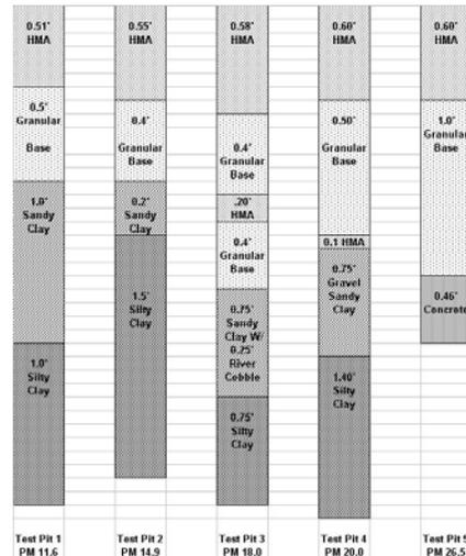
**Figure 7b. Example Test Pit Profile**
