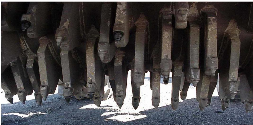
**Figure 8. Pulverizer Milling Teeth**
