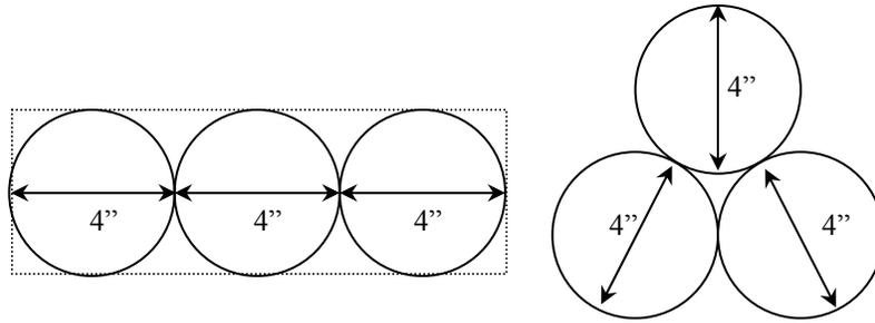
**Figure 6c. Examples of Clustered Coring Patterns**
