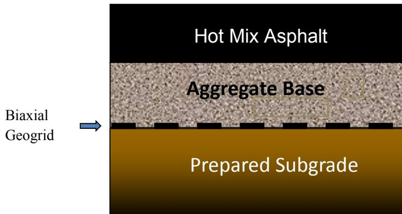
**Figure 1. Typical biaxial geogrid application**
