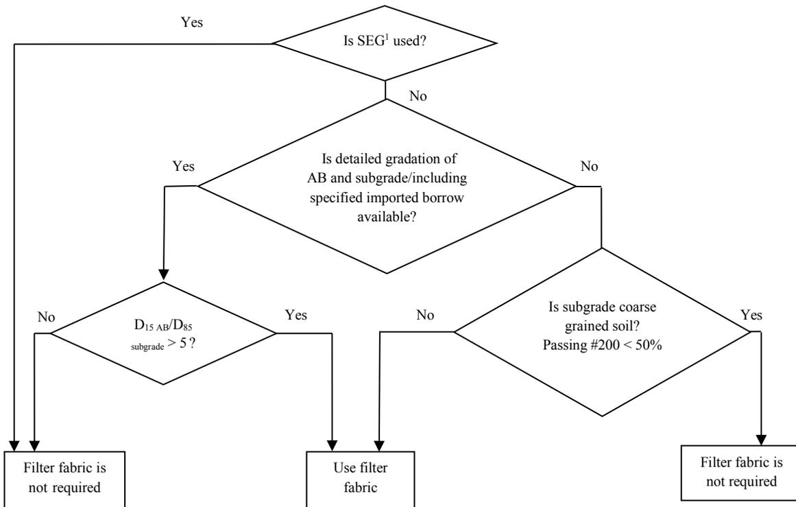
**Figure 2. Flowchart for Determining Filter Fabric Application**
