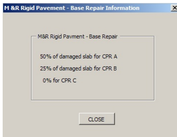
Figure 3-31 M&R Rigid Pavment – Base Repair Information Window
