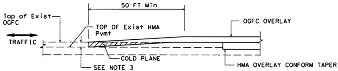
**TRANSVERSE OGFC TAPER TO EXISTING OGFC PAVEMENT**
