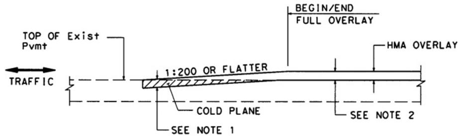
**TRANSVERSE HMA TAPER TO EXISTING HMA PAVEMENT**
