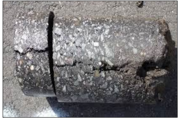
Figure 2.42: Bottom-up fatigue/reflected crack.
