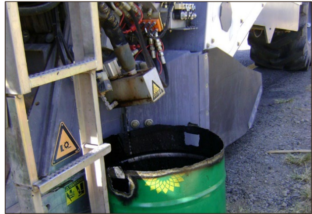
Figure 6.26: Nozzle for checking binder foaming characteristics.
