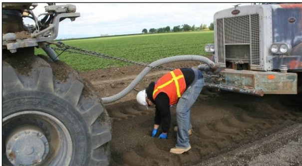
Figure 6.34: Sampling to check material consistency and gradation (FDR).
