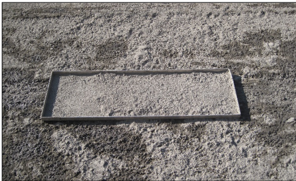
Figure 6.64: Pan after spreader has passed on a PDR-FA project (1% active filler).
