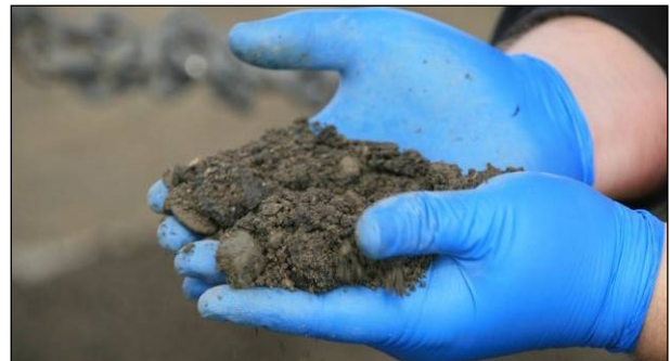
Figure 6.35: Checking material consistency and gradation (FDR).
