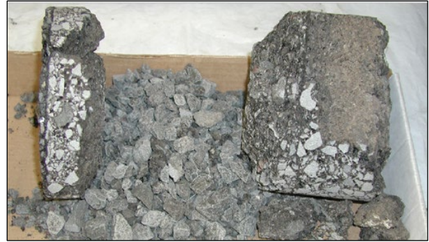
Figure 2.48: Stripped asphalt concrete layer.
