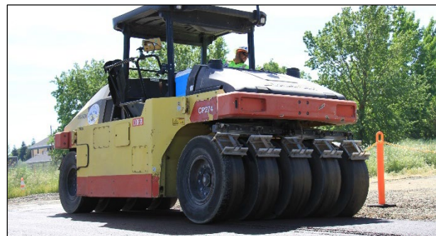
Figure 6.14: Pneumatic-tired roller on a PDR layer.
