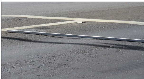
Figure 2.13: Example top-down distresses: Surface ruts/densification.
