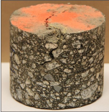
Figure 2.41: Top-down thermal crack.
