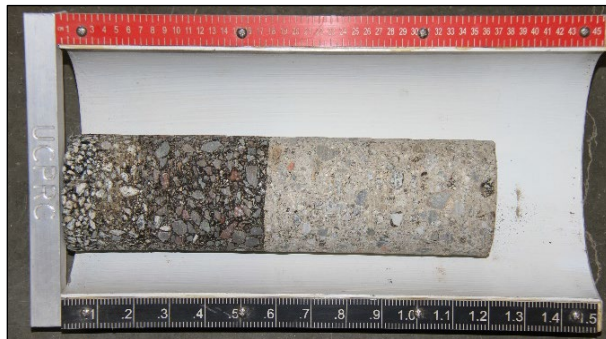
Figure 2.43: Concrete beneath asphalt layers (composite pavement).
