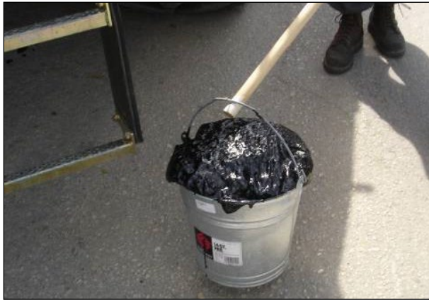
Figure 6.25: Checking binder foaming characteristics after tanker change.
