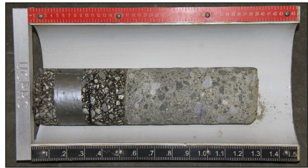
Figure 2.44: Asphalt on cement-treated base.
