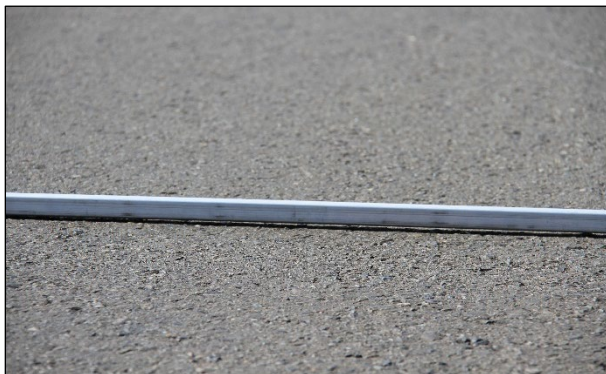
Figure 3.5: Minor early densification on a PDR project.
