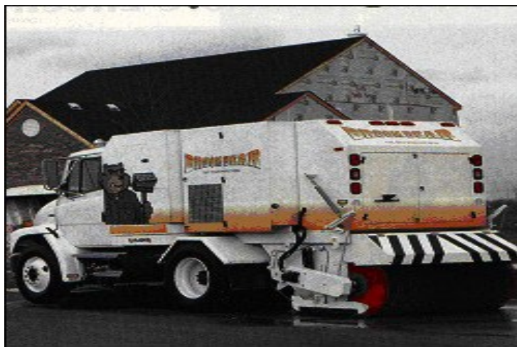
Figure 9-27 Sweeping with a Self-contained Sweeper
