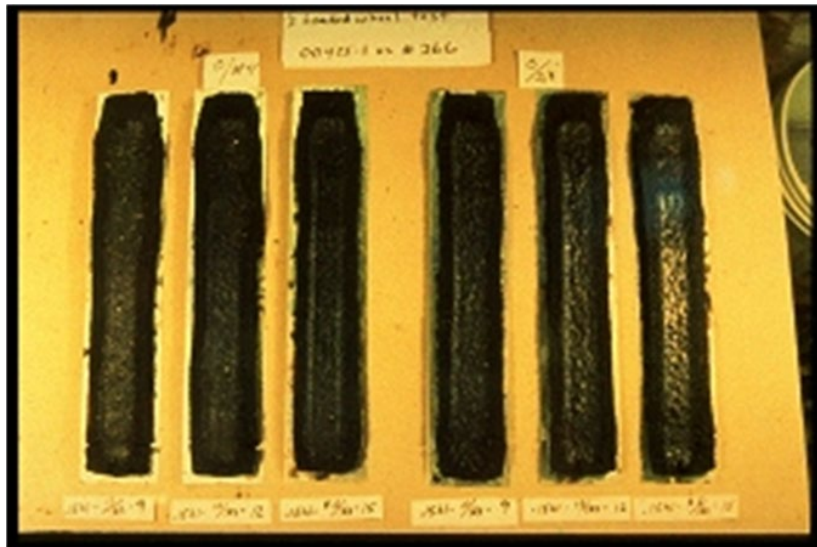
Figure 8-5 Tested Samples (TB 109) Showing Retained Sand from Loaded Wheel Test
