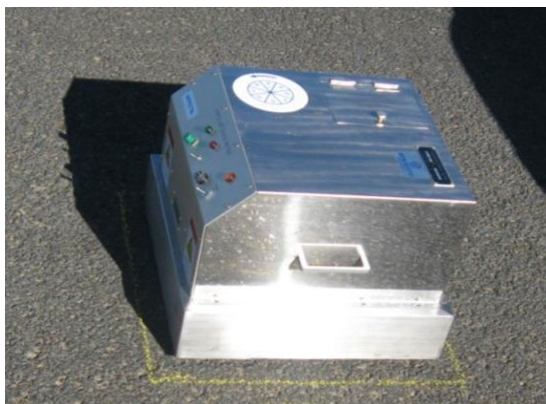
Figure 6-6 Circular Track Meter (CTM) for ASTM E2157-01
