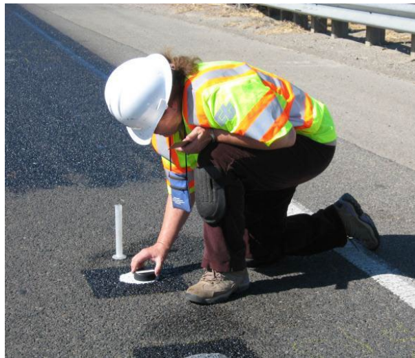
Figure 6-10 Sand Patch Test Being Performed ASTM E965 - 96 (2006)
