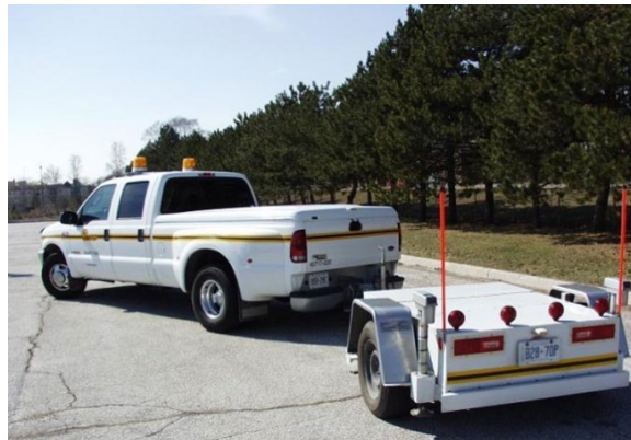
Figure 6-12 ASTM Skid Trailer (Ontario MTO 2010)
