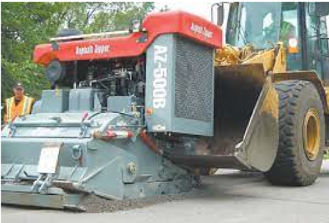
a) Milling Unit Mounted on Front Loader
