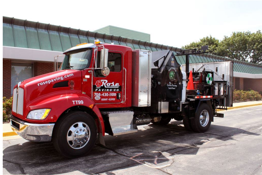
a) Truck-Mounted Heater (Rose Paving, 2013)
