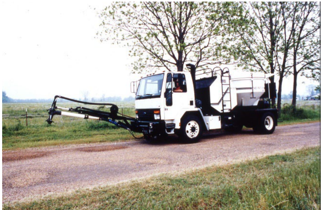
Figure 5-7 Spray Injection Patch Truck
