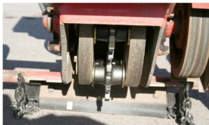
Figure 4-16 Crack Routing Operation and Equipment
