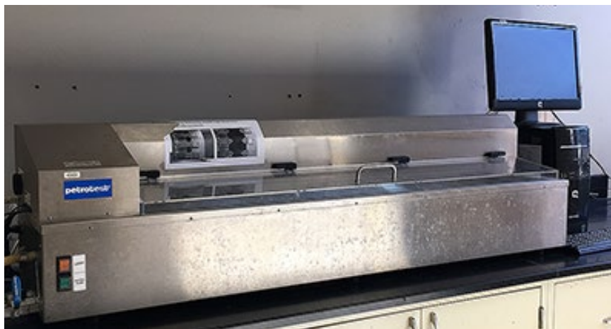
Figure 2-4 Ductility Meter (FHWA Research, Asphalt Binder and Mixtures Laboratory Overview)
