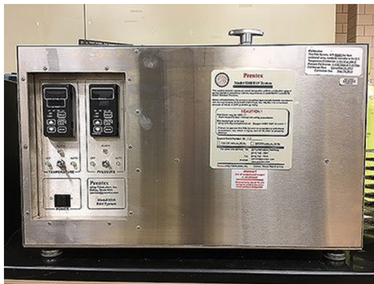
Figure 2-7 Pressure Aging Vessel (PAV) (FHWA Research, Asphalt Binder and Mixtures Laboratory Overview)
