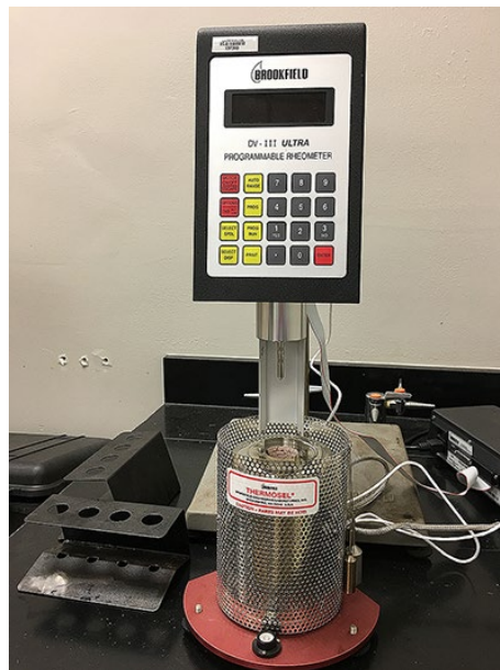
Figure 2-3 Rotational Viscometer (RV) (FHWA Research, Asphalt Binder and Mixtures Laboratory Overview)
