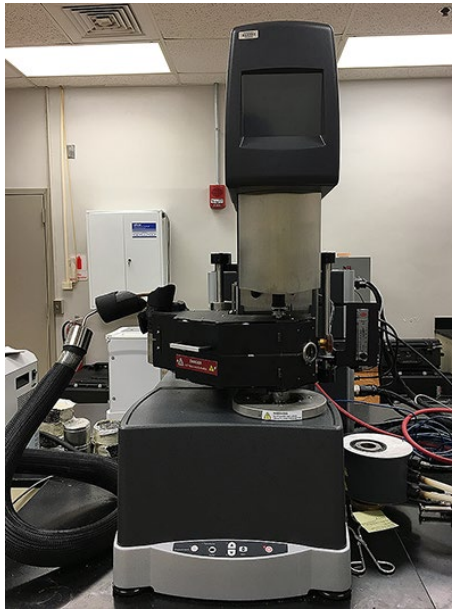
Figure 2-2 Dynamic Shear Rheometer (DSR), (FHWA Research, Asphalt Binder and Mixtures Laboratory Overview)
