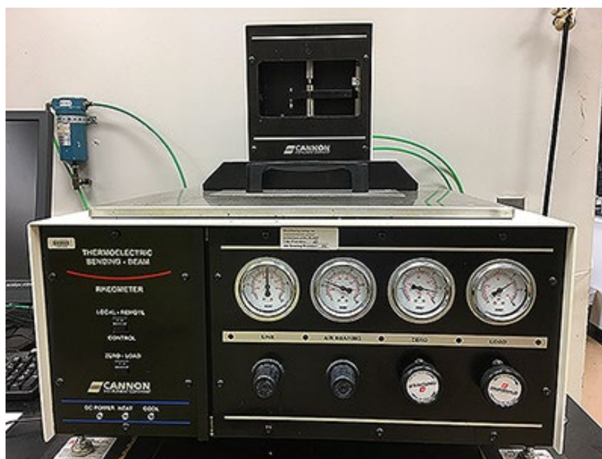
Figure 2-5 Bending Beam Rheometer (BBR) (FHWA Research, Asphalt Binder and Mixtures Laboratory Overview)
