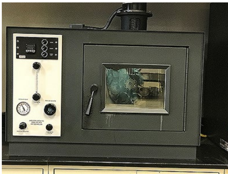
Figure 2-6 Rolling Thin Film Oven (RTFO) (FHWA Research, Asphalt Binder and Mixtures Laboratory Overview)
