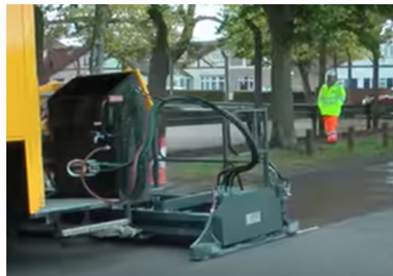
Figure 10-9 Micro Surfacing Rut Filling Machine (Lt.), Mounted Outrigger (Rt.)
