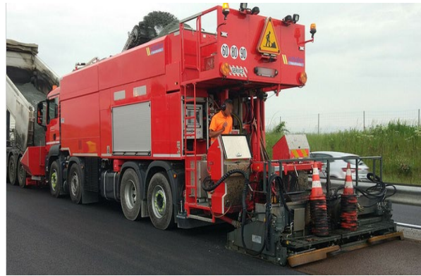
Figure 10-7 Micro Surfacing Machine
