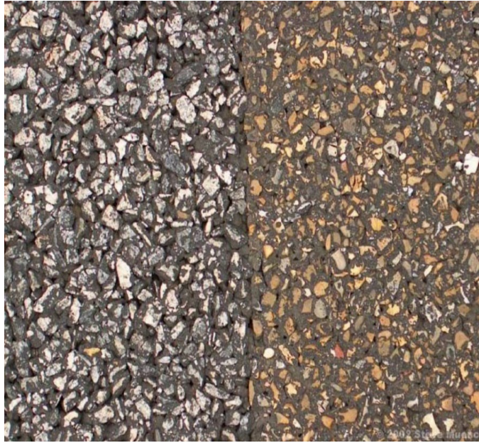
Figure 1-22 Non-polished (Lt.) Versus Polished Aggregate (Rt.)
