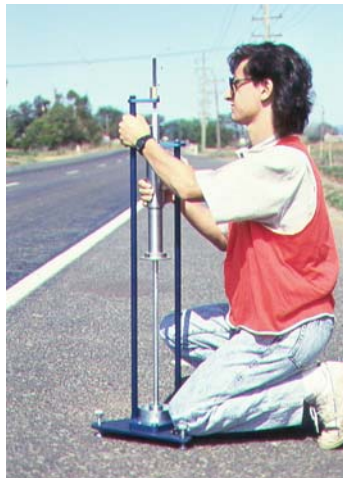
a) Ball Penetrometer Test
