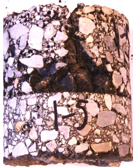
Figure 11-4 The bottom lift of the existing HMA layer is not cracked and the crack on the top layer is very wide at the interface. The crack in the OGFC layer is V shaped, indicative of raveling (Sebaaly, 2007).
