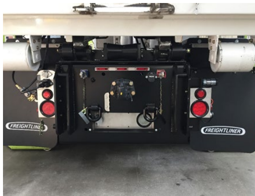
BODY AIR AND LIGHTING CONNECTIONS
